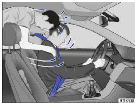
Fig. 49 Unbelted passengers in the rear seats are thrown forward on top of the belted driver.
