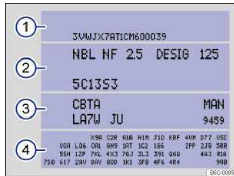
Fig. 18 Vehicle identification label: Shown in the example with engine identification code CBTA 3.
