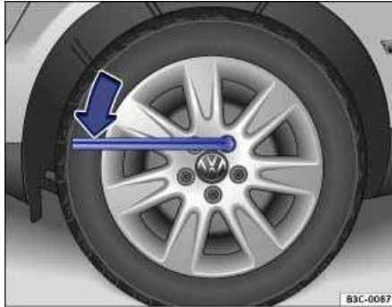
Fig. 160 Changing a wheel: Loosening wheel bolts.
