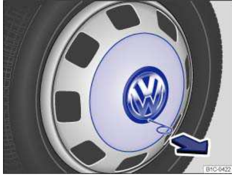
Fig. 159 Pulling the wheel cover off (Version 2).
