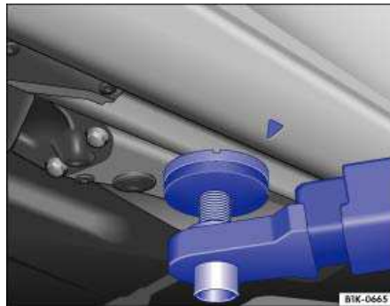
Fig. 146 Rear lift point for workshop hoist or floor jack.
