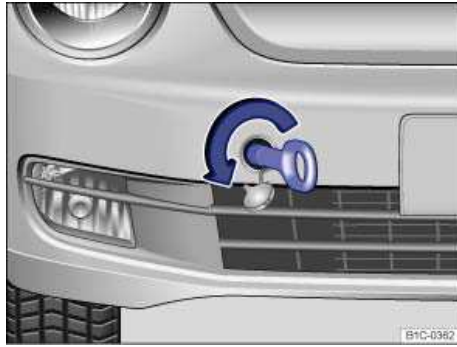
Fig. 184 In the right front bumper: Screwing in the towing eye.
