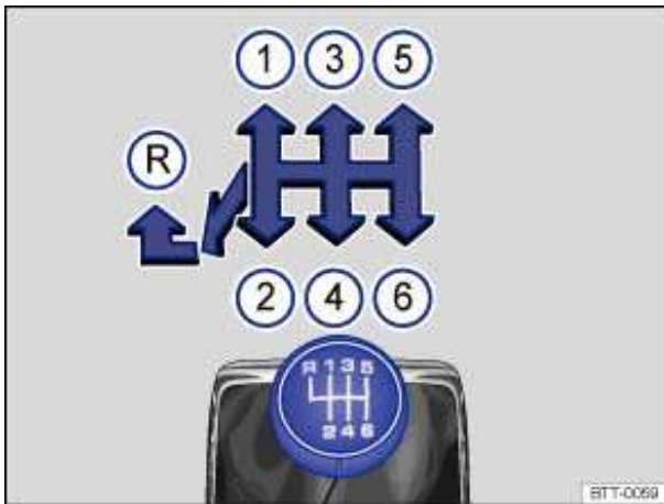
Fig. 99 Gearshift pattern of a 6-speed manual transmission.
