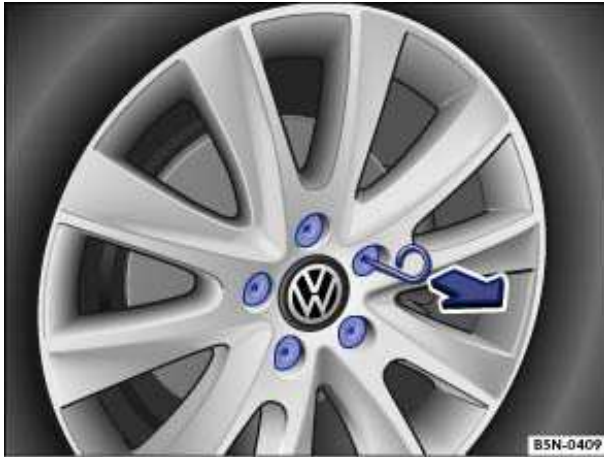
Fig. 141 Pulling cover caps off wheel bolts.
