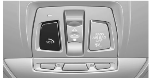
SOS button in the roofliner
