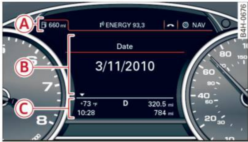
Fig. 4 Driver information system in the instrument cluster
