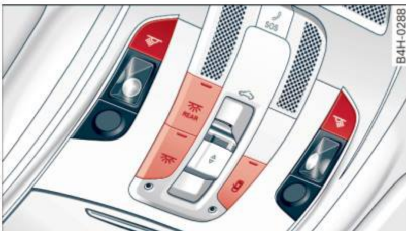
Fig. 41 Headliner: Front interior lights
