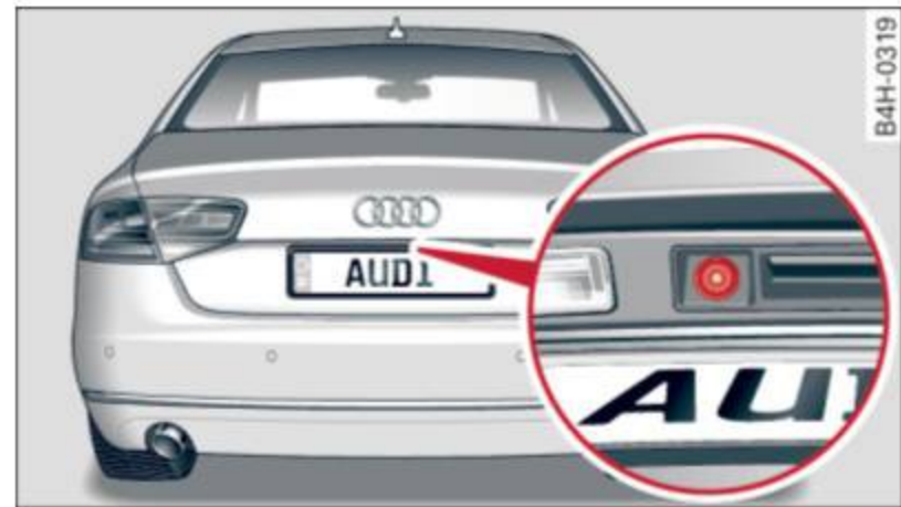
Fig. 131 Rear lid: Location of the rear view camera
