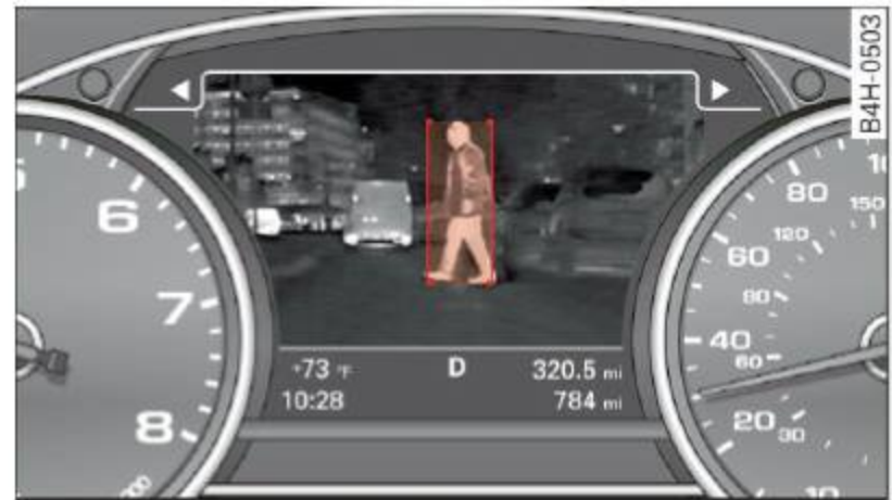
Fig. 117 Display: pedestrian warning
