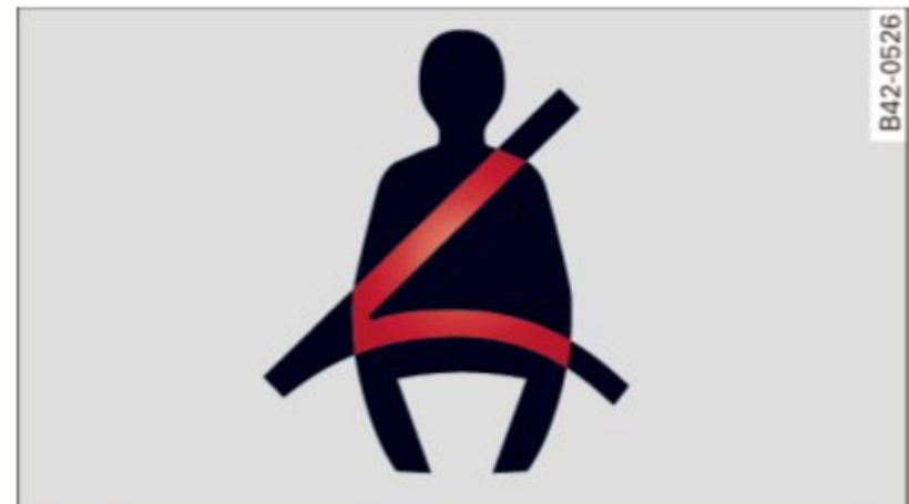
Fig. 155 Safety belt warning light in the instrument cluster - enlarged
