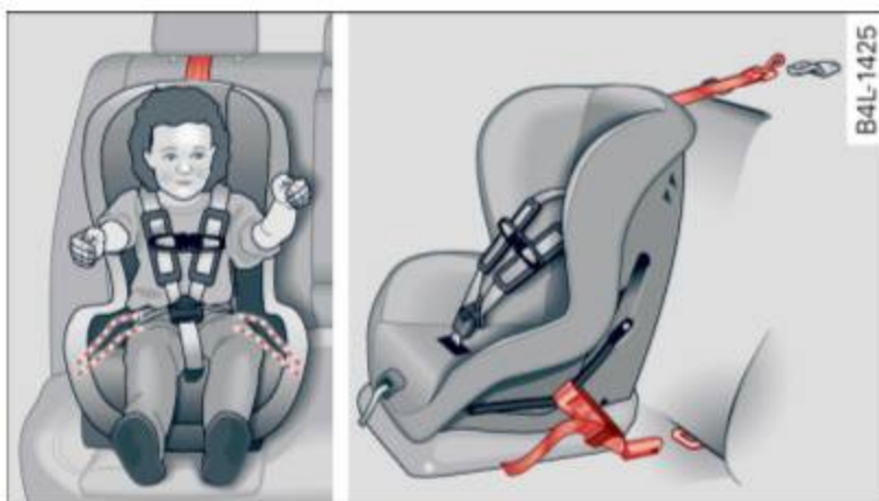
Fig. 177 Schematic overview: installation of the attachments applicable to a LATCH seat
