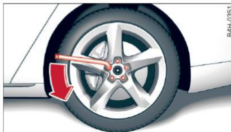
Fig. 223 Changing a wheel: loosening the wheel bolts
