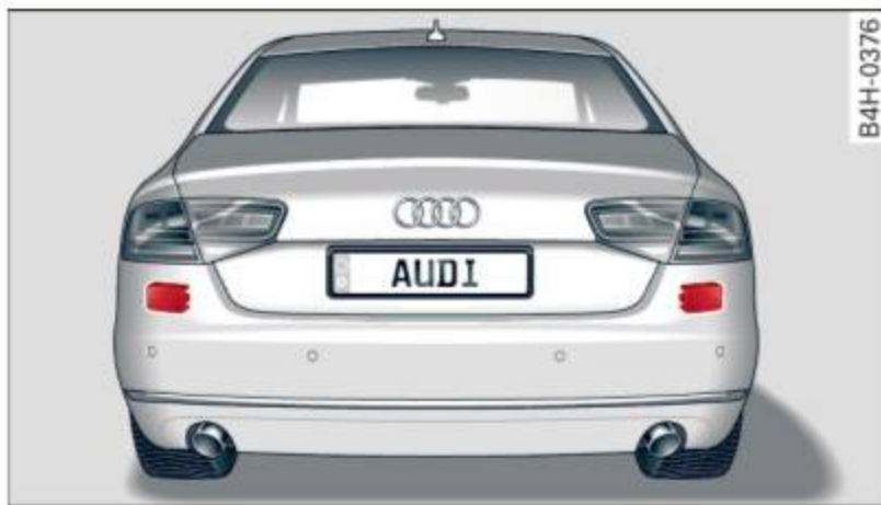
Fig. 111 Rear of the vehicle: position of the sensors
