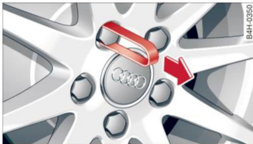
Fig. 222 Changing a wheel: removing the wheel bolt caps
