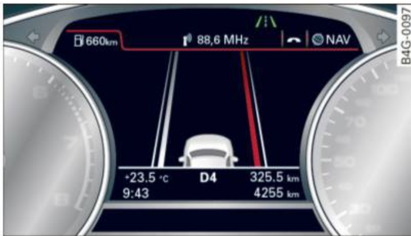
Fig. 106 Instrument cluster: lane assist is switched on and is warning
