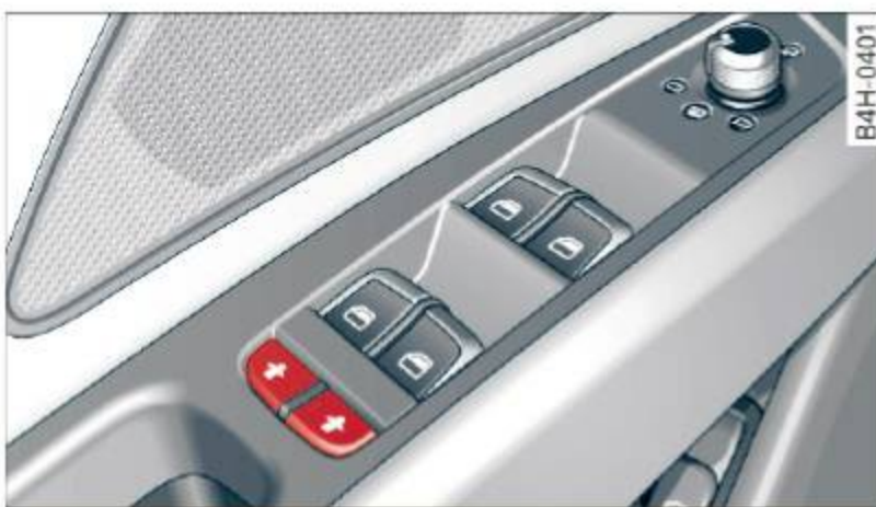
Fig. 31 Section from driver's door: controls
