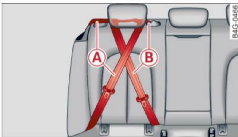
Fig. 175 Schematic overview: keep unused safety belts away from children in child safety seats. A - outer rear safety belt, B - center rear safety belt
