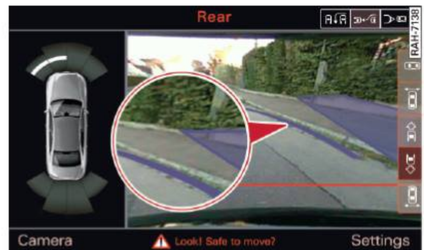
Fig. 149 Infotainment: contact of the blue curved line with the curb
