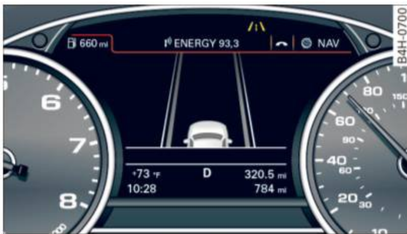
Fig. 107 Instrument cluster: lane assist is switched on but not ready to provide warnings
