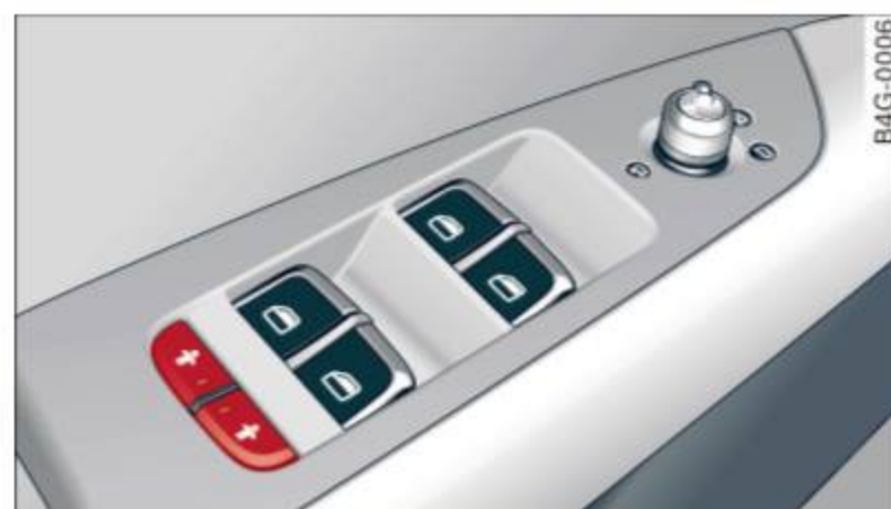
Fig. 33 Section from driver's door: child safety lock buttons
