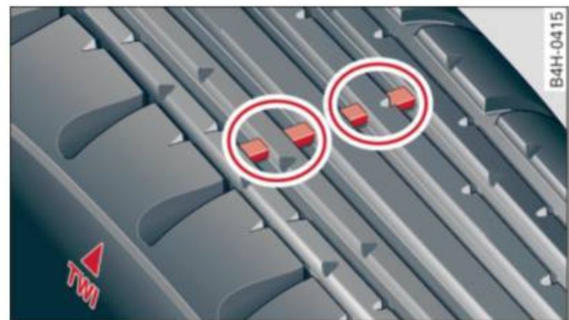
Fig. 197 Tire tread: tread wear indicators (TWI)
