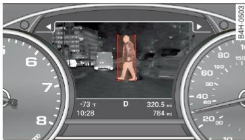
Fig. 110 Display: pedestrian warning
