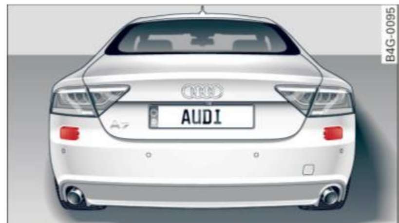
Fig. 104 Rear of the vehicle: position of the sensors
