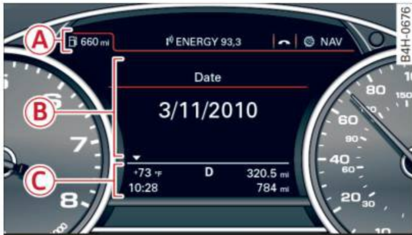
Fig. 4 Driver information system in the instrument cluster
