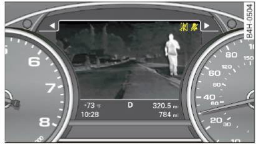
Fig. 114 Display: example of pedestrian detection and warning tone switched off
