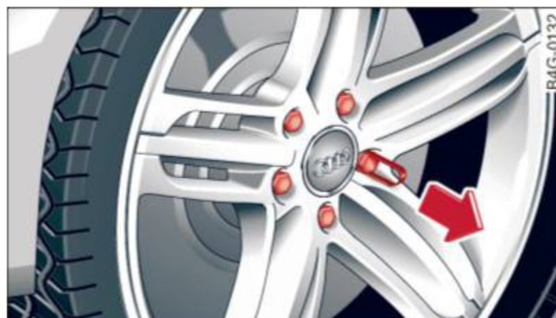
Fig. 208 Changing a wheel: removing the wheel bolt caps
