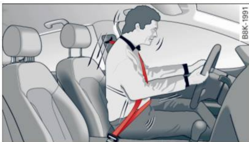
Fig. 153 Driver is correctly restrained in a sudden braking maneuver
