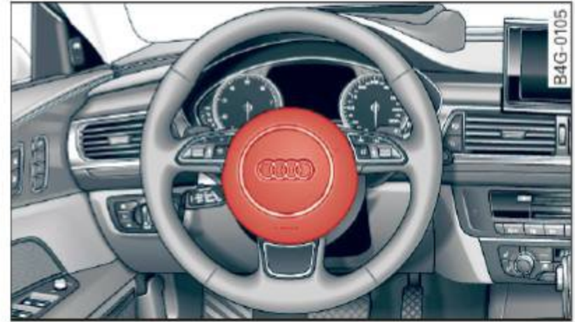
Fig. 159 Location of driver airbag: in steering wheel
