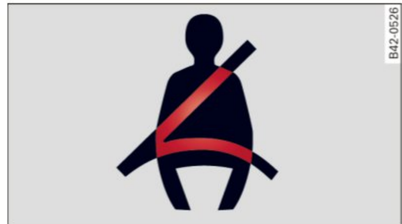
Fig. 148 Safety belt warning light in the instrument cluster - enlarged
