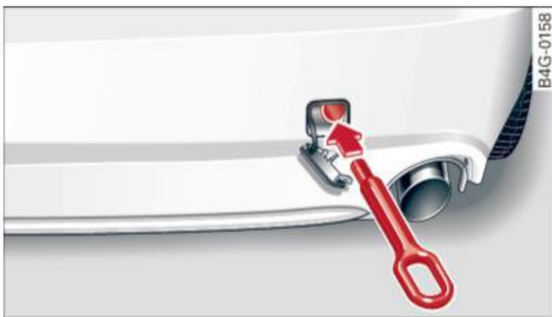
Fig. 224 Rear bumper: screwing in towing loop
