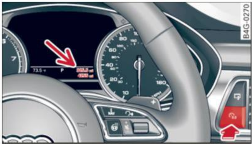
Fig. 11 Instrument cluster: Odometer and reset button
