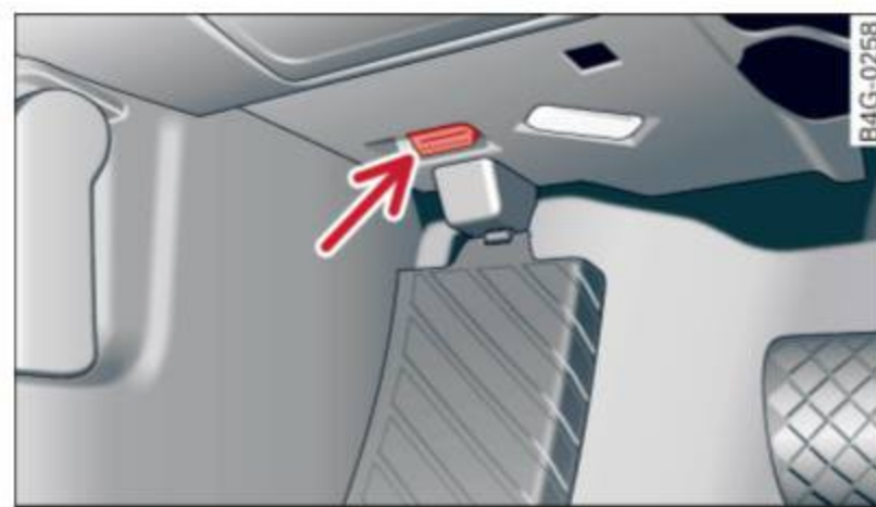
Fig. 19 Location of Data Link Connector (DLC)
