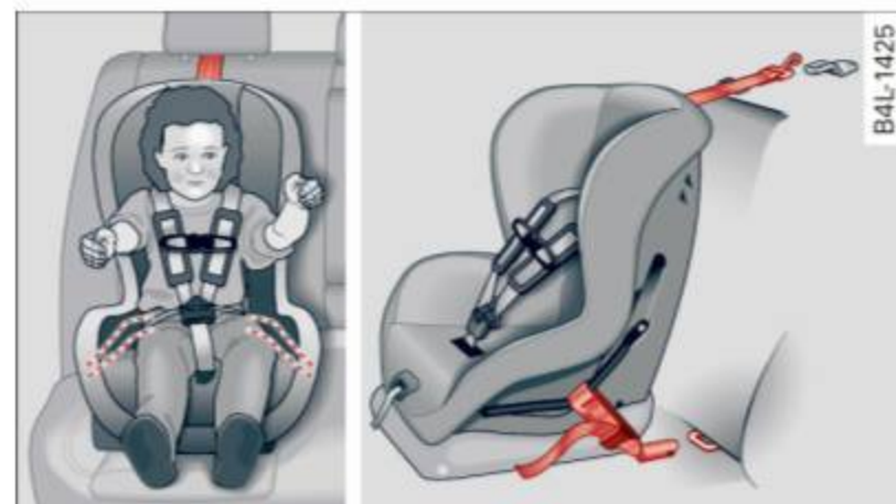
Fig. 171 Schematic overview: installation of the attachments applicable to a LATCH seat
