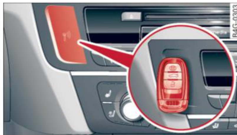
Fig. 82 Center console/master key: starting the engine if there is a malfunction
