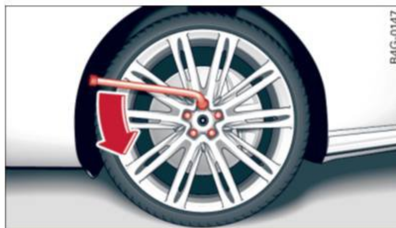
Fig. 209 Changing a wheel: loosening the wheel bolts
