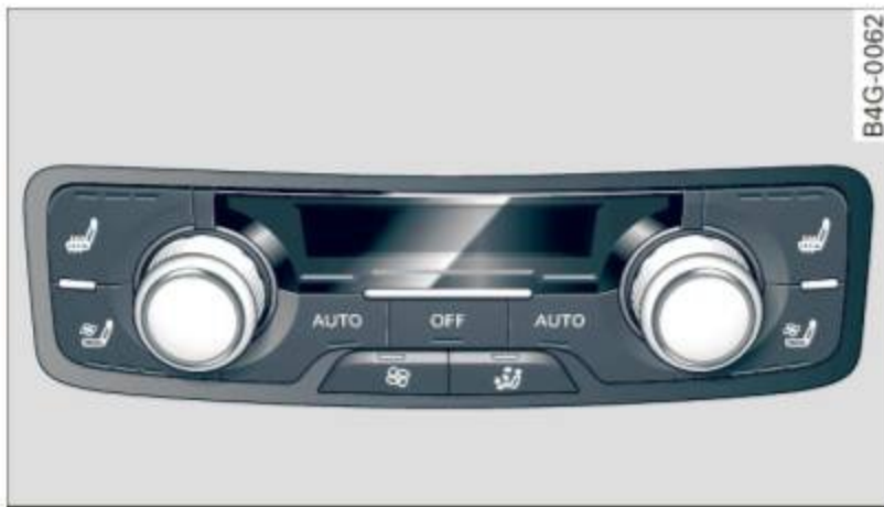
Fig. 77 Four-zone automatic climate control: rear controls
