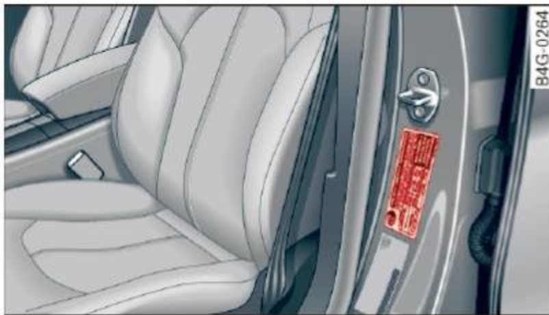
Fig. 195 Tire pressure label: located on driver's side B-pillar
