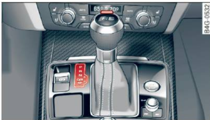
Fig. 117 Shift gate on the center console: selector lever with release button
