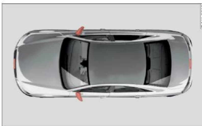
Fig. 132 Location of peripheral cameras
