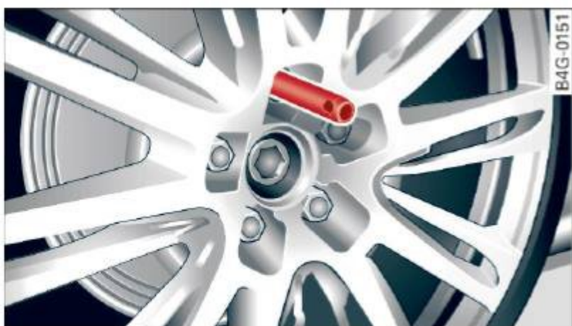
Fig. 214 Changing a wheel: alignment pin inside the top hole
