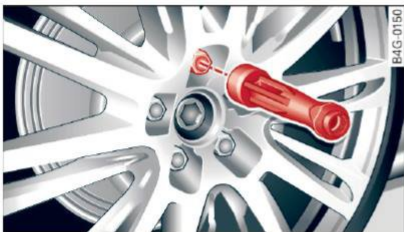
Fig. 213 Changing a wheel: using the screwdriver handle (with the blade removed) to turn the bolts
