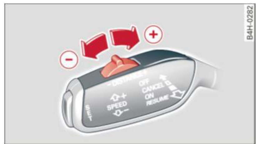
Fig. 94 Selector lever: setting the distance
