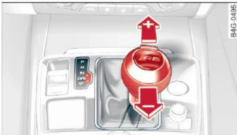
Fig. 118 Center console: shifting the gears manually
