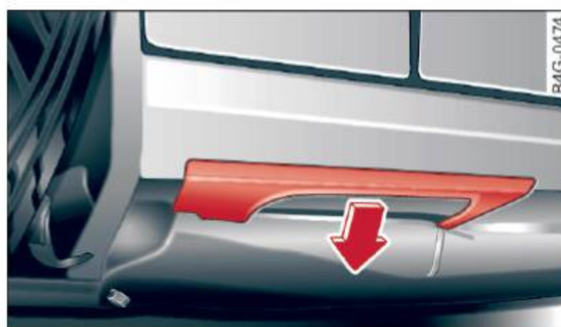
Fig. 212 Sill: removing the cover
