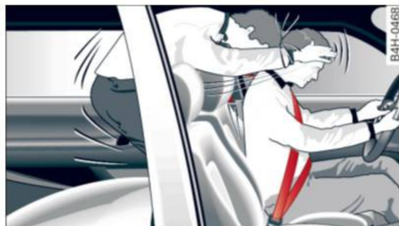
Fig. 152 A rear passenger not wearing a safety belt will fly forward and strike the driver
