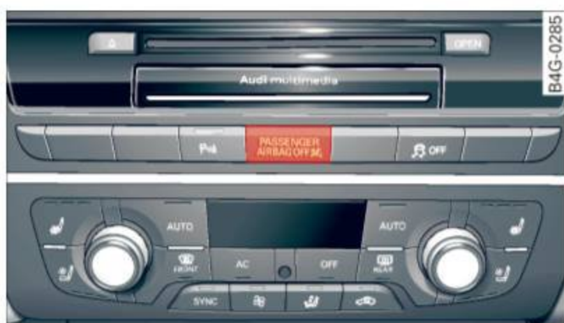
Fig. 162 Section from the instrument panel: PASSENGER AIR BAG OFF light
