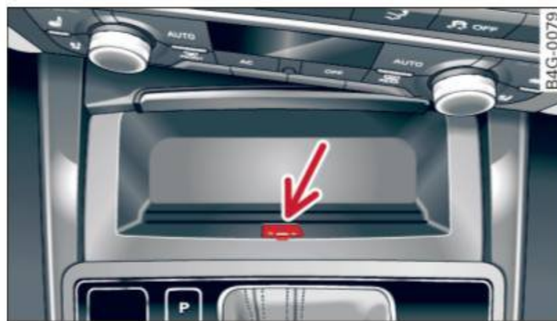
Fig. 120 Front center console: selector lever emergency release
