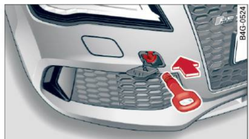
Fig. 222 Front bumper: installing the towing loop
