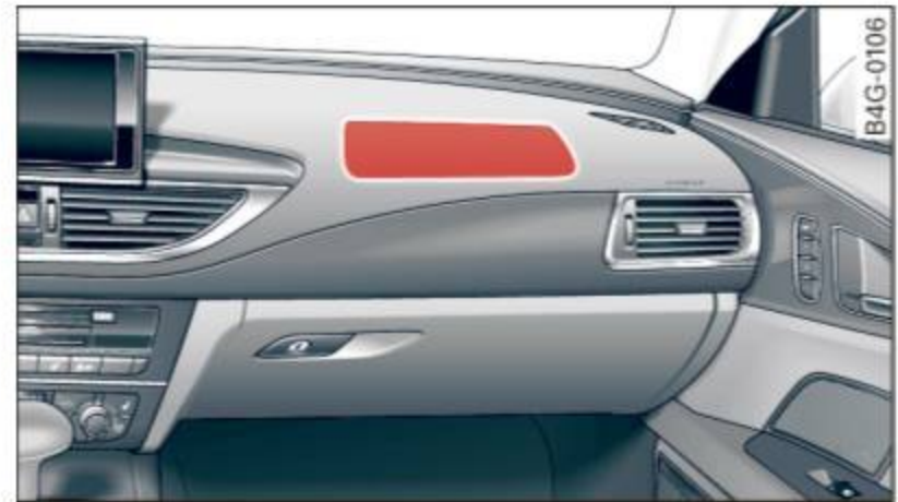
Fig. 160 Location of front passenger's airbag: in the instrument panel
