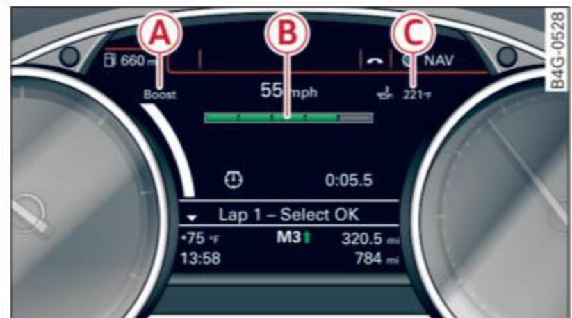
Fig. 16 Instrument cluster: boost, shifting and engine oil temperature indicators
