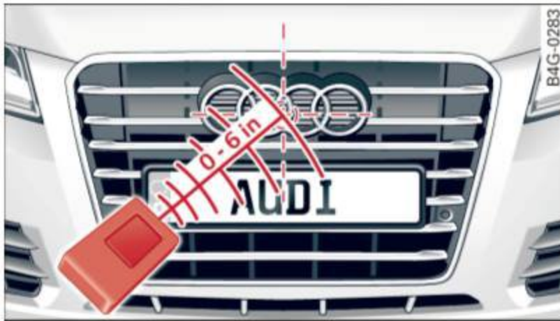
Fig. 145 Distance between the radiator grille and the hand transmitter
