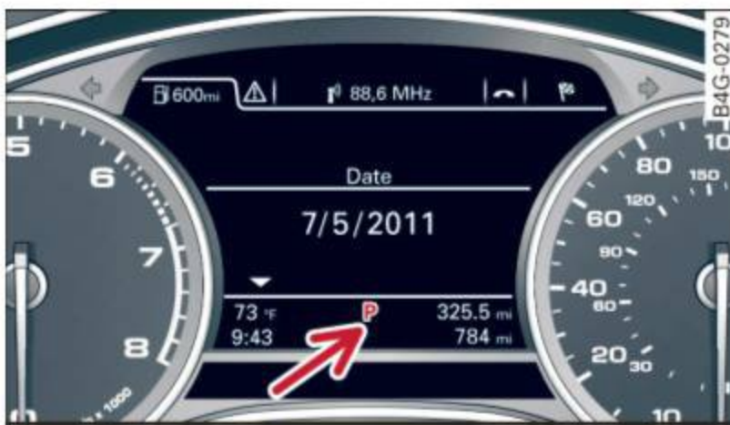
Fig. 115 Display in the instrument cluster: selector lever position
