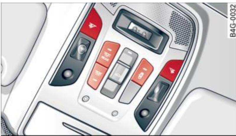
Fig. 40 Headliner: Front interior lights
