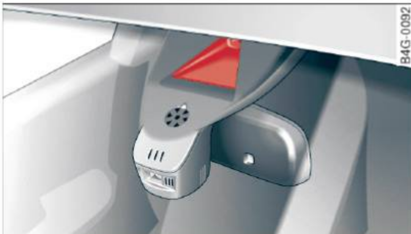
Fig. 98 Windshield: Active lane assist camera viewing window
