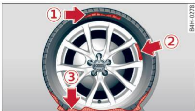
Fig. 205 Tire damage for which the Tire Mobility System is not suited
