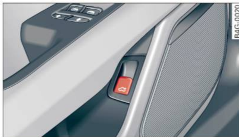
Fig. 29 Driver's door: Unlocking the rear lid
