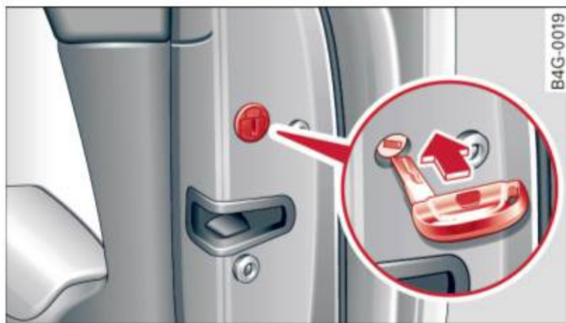
Fig. 28 Door: Emergency locking
