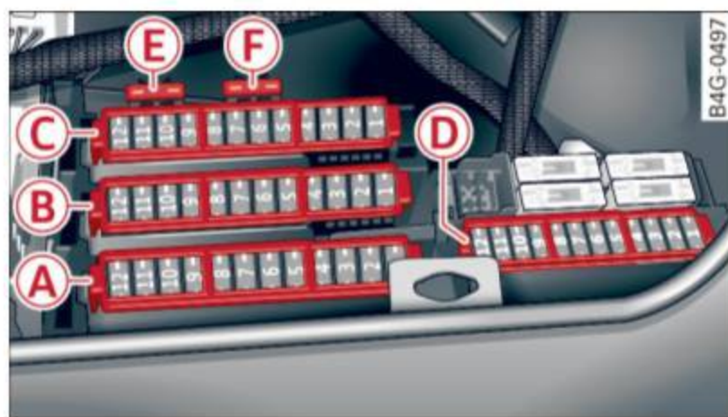
Fig. 218 Luggage compartment: fuse panel with plastic bracket
