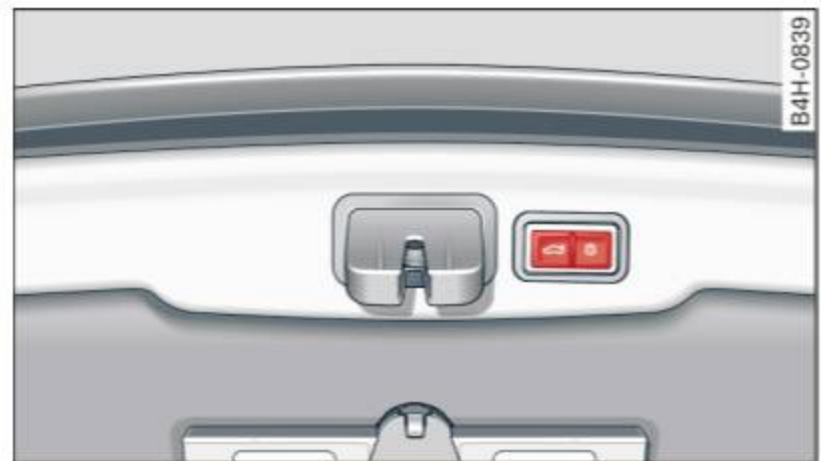
Fig. 30 Closing and locking button in the luggage compartment lid (vehicles with convenience key*)
