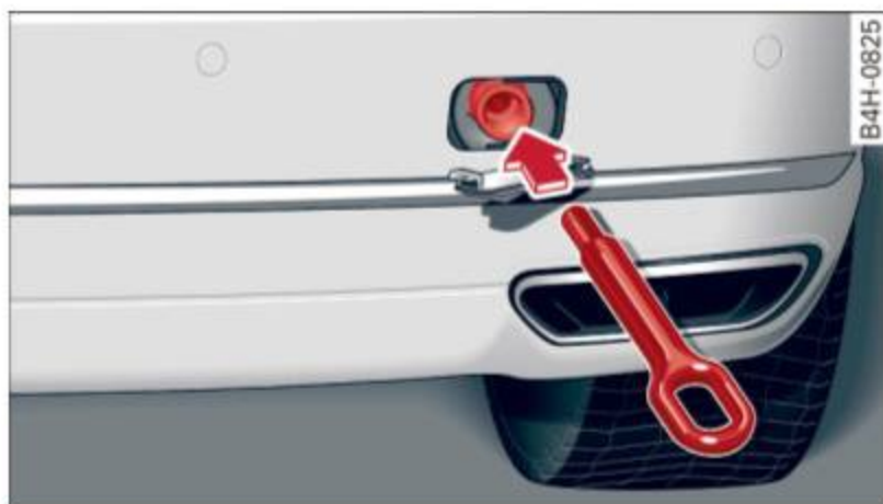
Fig. 240 Rear bumper: screwing in towing loop
