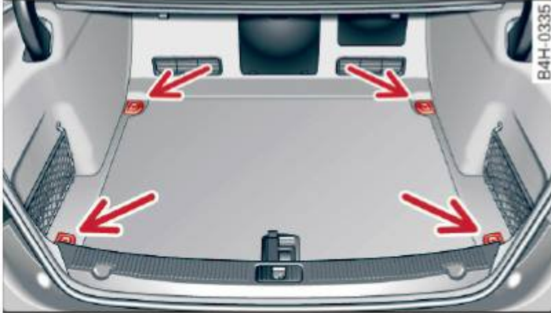
Fig. 71 Location of the fastening eyes in the luggage compartment
