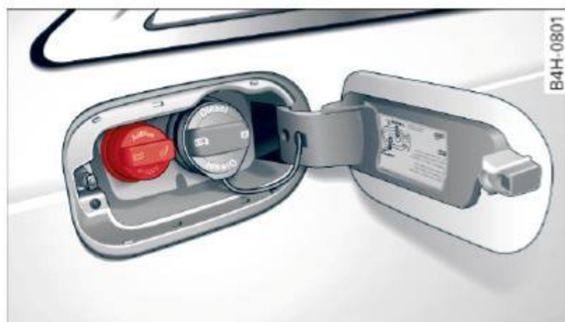
Fig. 195 Right rear vehicle side: removing the AdBlue filler cap
