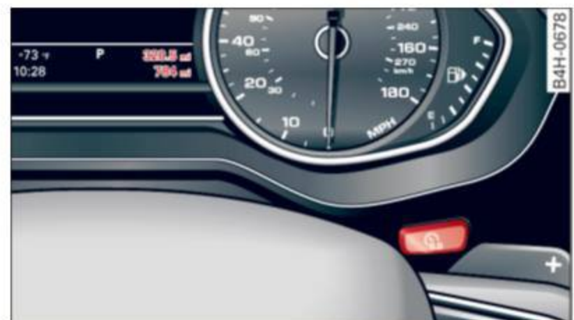
Fig. 11 Instrument cluster Odometer and reset button
