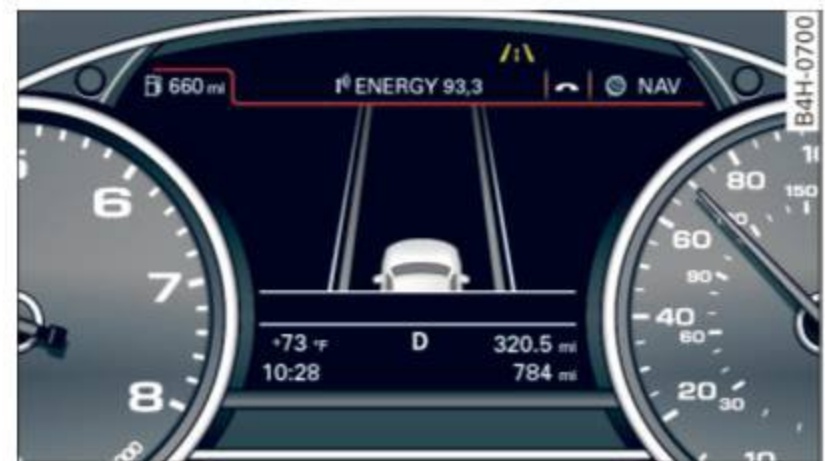
Fig. 110 Instrument cluster: Active lane assist is switched on but not ready to provide warnings
