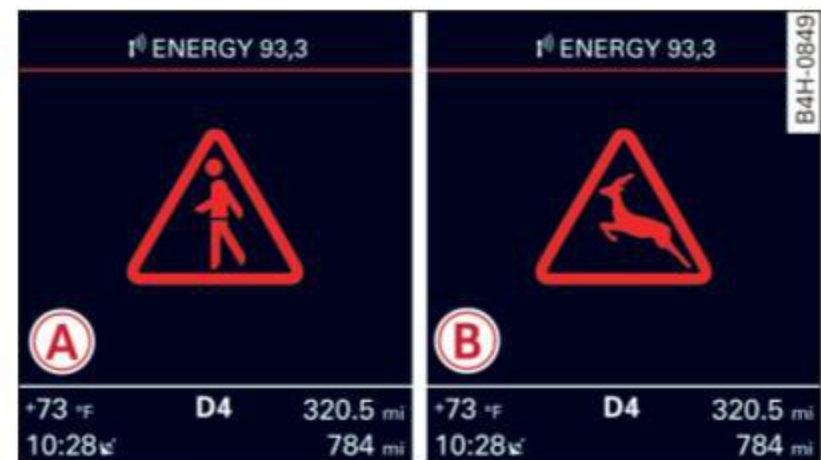
Fig. 120 Instrument cluster: (A) pedestrian warning/ (B) wild animal warning when the night vision assistant image is not selected in the instrument cluster display
