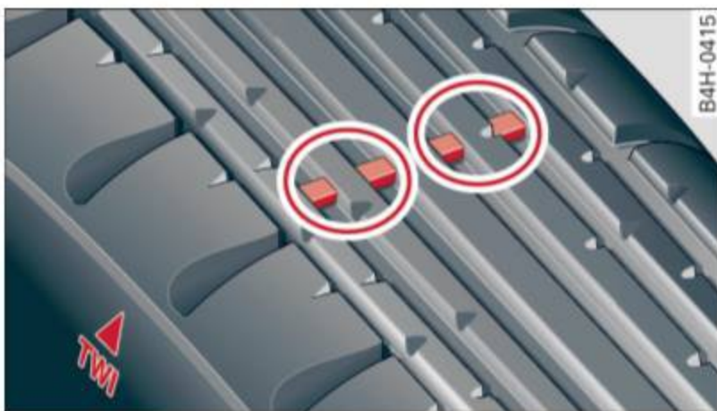
Fig. 210 Tire tread: tread wear indicators (TWI)
