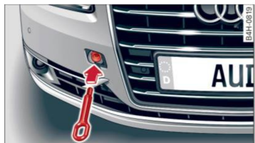
Fig. 238 Front bumper: screwing in the towing loop
