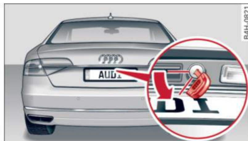
Fig. 32 Luggage compartment lid: mechanical key in the lock cylinder
