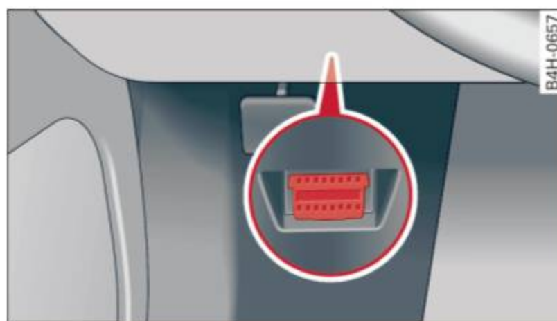
Fig. 17 Location of Data Link Connector (DLC)
