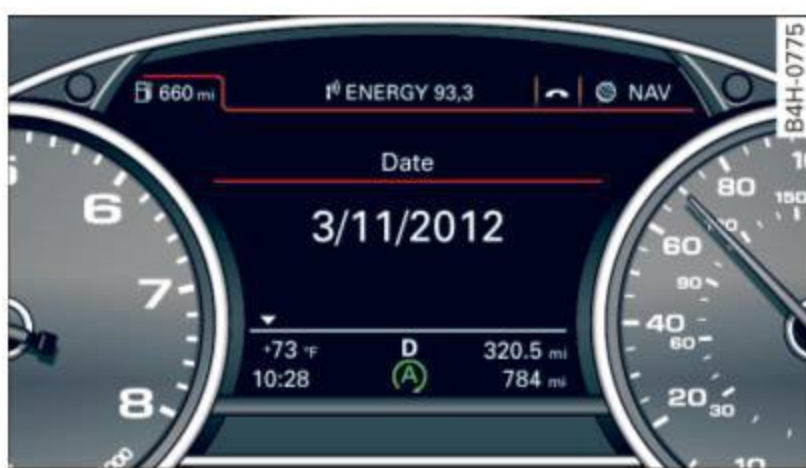
Fig. 91 Instrument cluster: engine switched off (stop phase)
