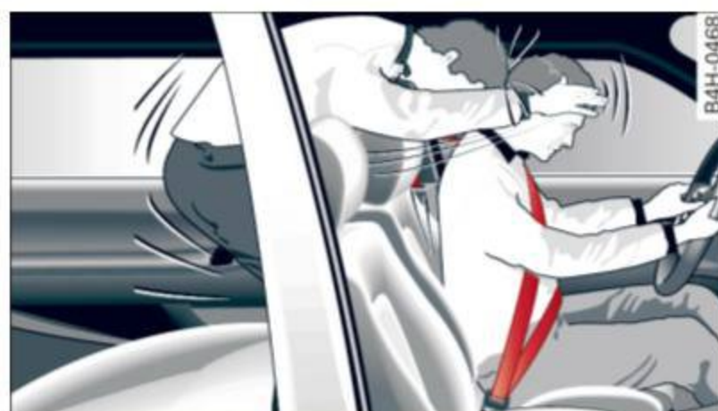
Fig. 159 A rear passenger not wearing a safety belt will fly forward and strike the driver
