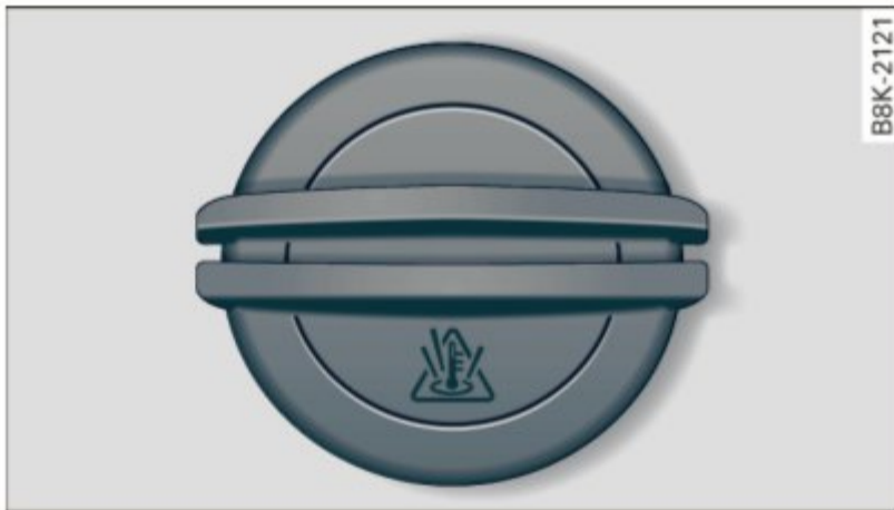
Fig. 204 Engine compartment: cover on the coolant expansion tank
