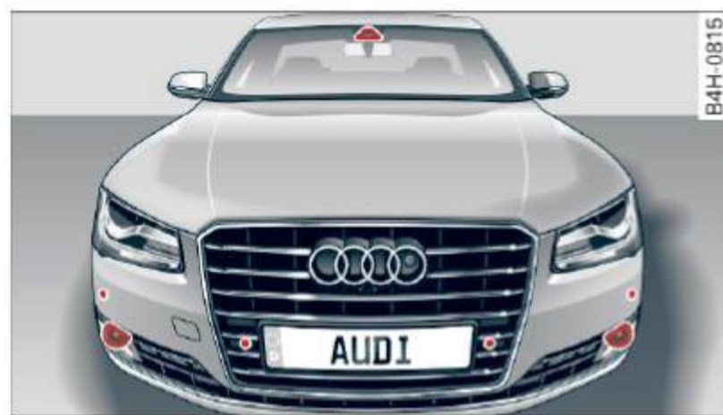
Fig. 96 Front of the vehicle: sensors and video camera
