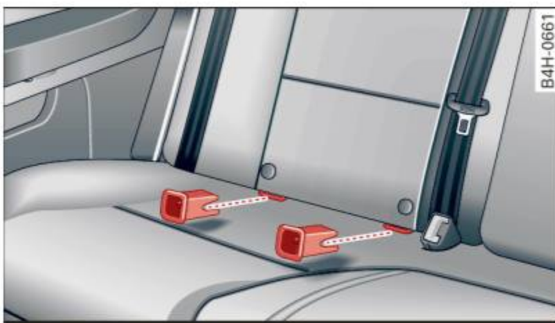
Fig. 183 Outer rear seats: installing the guidance fixtures
