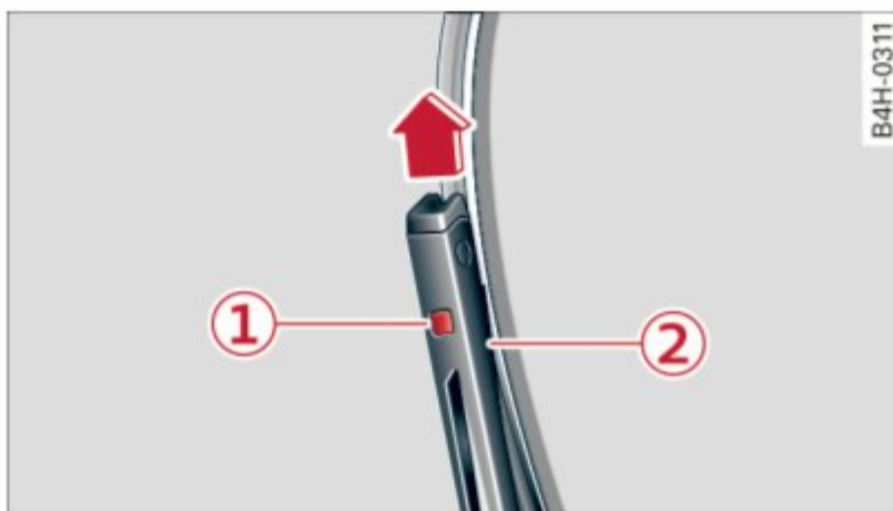
Fig. 52 Removing windshield wiper blades
