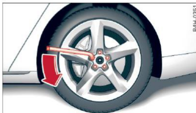
Fig. 223 Changing a wheel: loosening the wheel bolts
