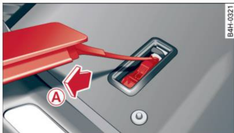
Fig. 127 Driver's side footwell: releasing the parking lock using the emergency release
