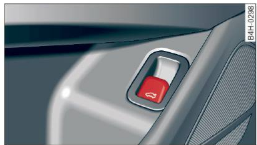
Fig. 27 Driver's door: remote luggage compartment lid release
