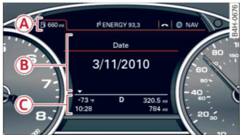
Fig. 4 Driver information system in the instrument cluster
