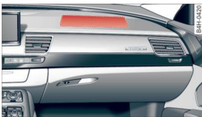
Fig. 166 Location of front passenger's airbag: in the instrument panel
