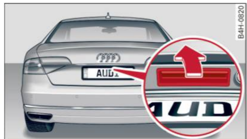
Fig. 28 Position of lock and handle in the luggage compartment lid
