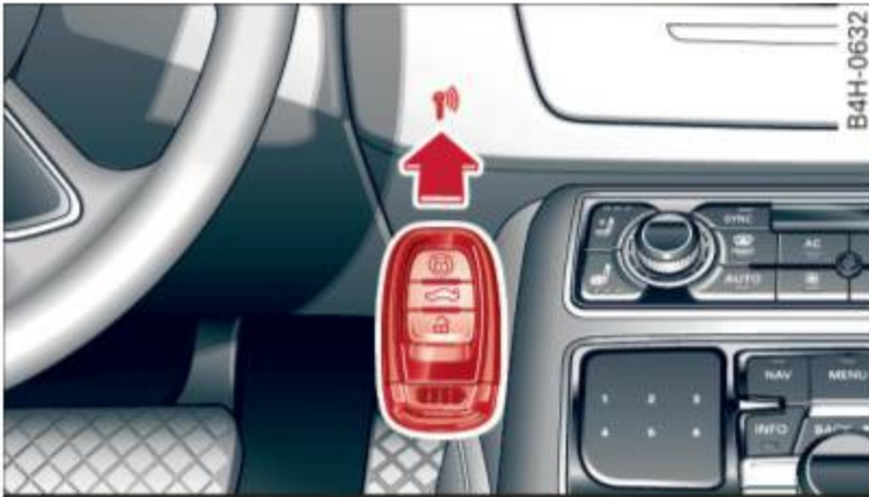
Fig. 89 Center console/master key: starting the engine if there is a malfunction
