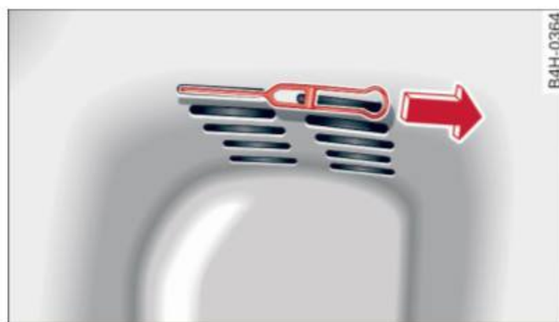
Fig. 193 Right side trim panel in the luggage compartment: emergency release mechanism
