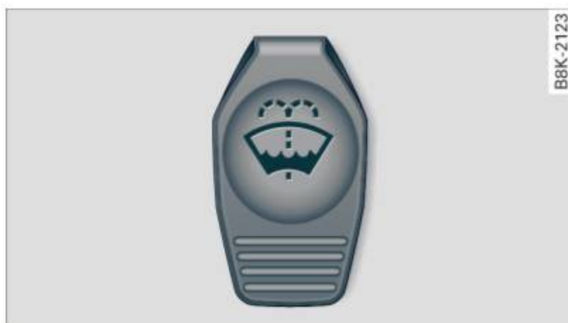
Fig. 207 Engine compartment: cover on the windshield washer fluid reservoir
