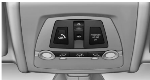
SOS button in the roofliner
