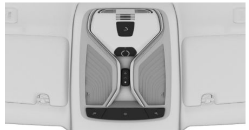
SOS button in the roofliner.
