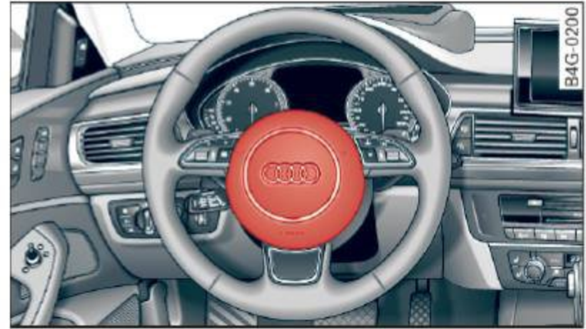
Fig. 156 Location of driver airbag: in steering wheel
