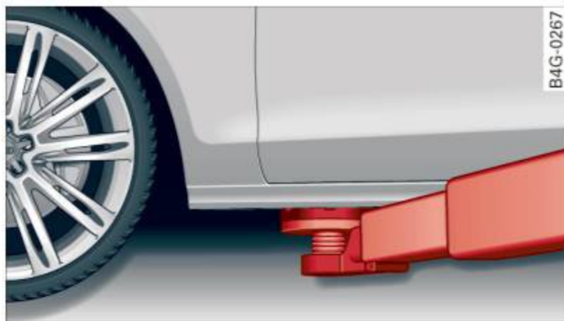
Fig. 221 Front lifting point
