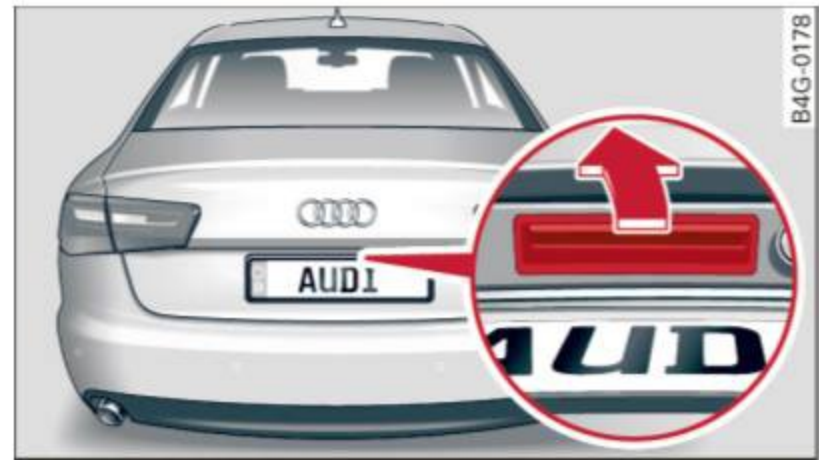
Fig. 27 Position of handle in the rear lid
