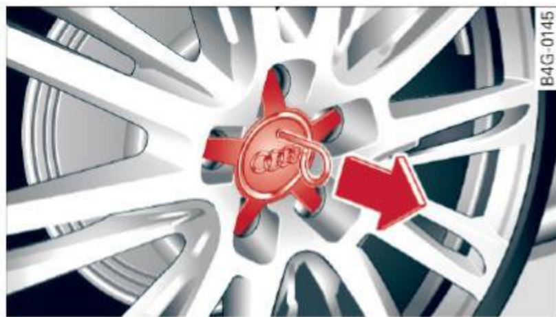
Fig. 202 Changing a wheel: Removing the wheel cover
