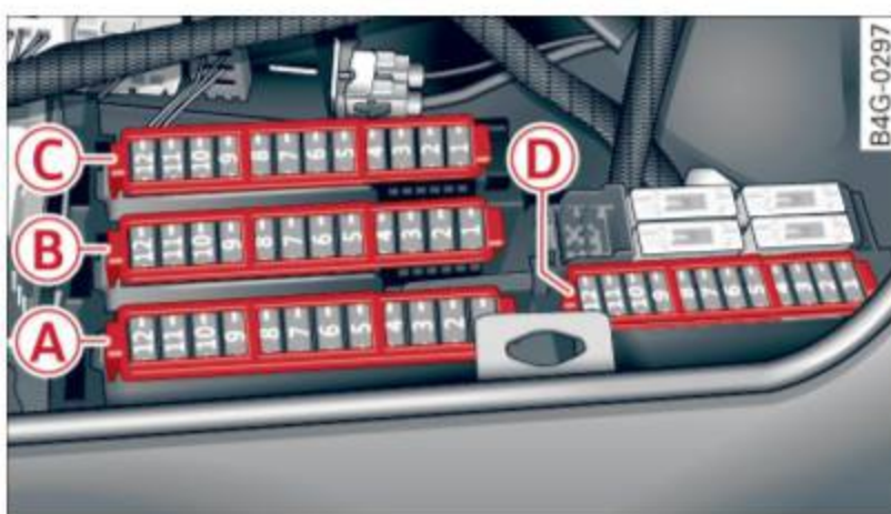
Fig. 213 Luggage compartment: fuse panel with plastic bracket
