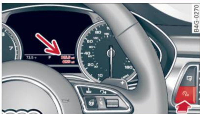
Fig. 11 Instrument cluster: Odometer and reset button
