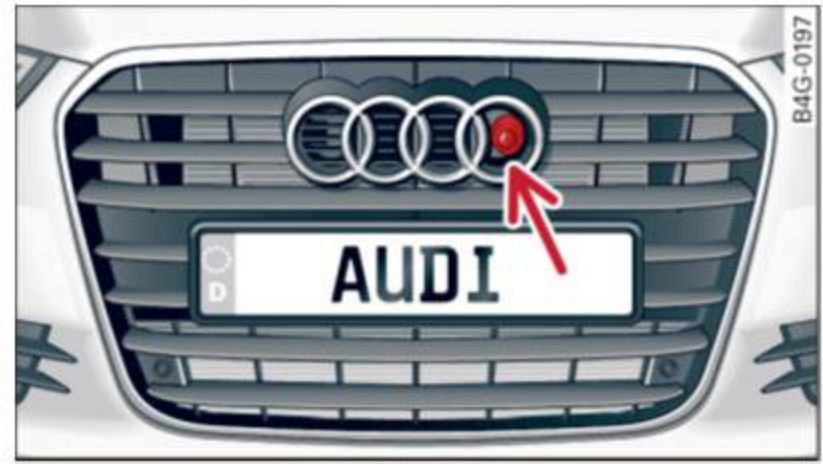
Fig. 108 Front of the vehicle: night vision assistant camera
