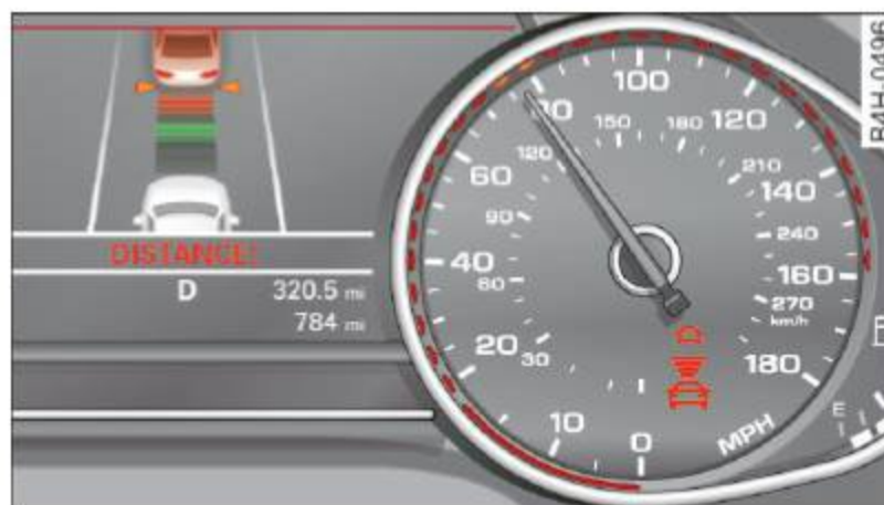
Fig. 91 Instrument cluster: request for driver intervention
