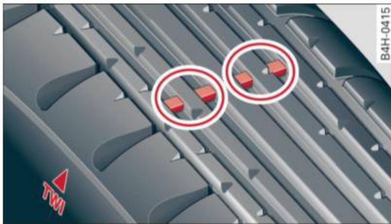
Fig. 193 Tire tread: tread wear indicators (TWI)
