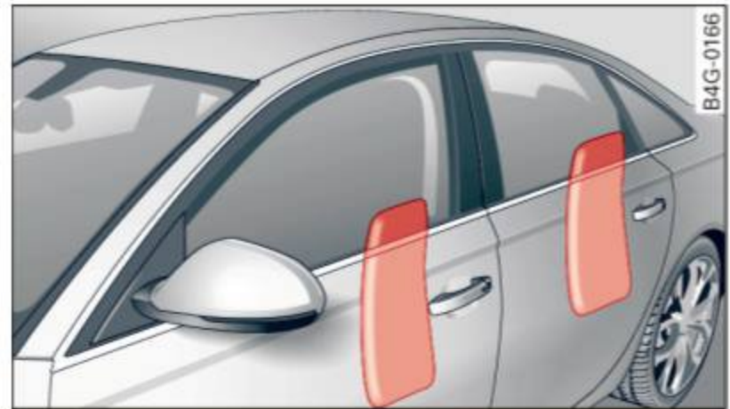
Fig. 163 Inflated side airbags on left side of vehicle, rear side airbag
