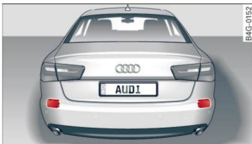
Fig. 100 Rear of the vehicle: position of the sensors
