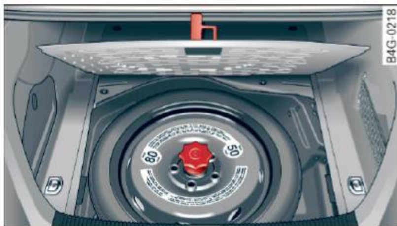
Fig. 200 Luggage compartment: cargo floor cover folded upward/spare tire
