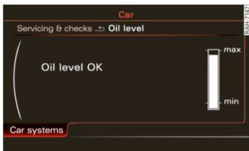
Fig. 185 Display: oil level indicator
