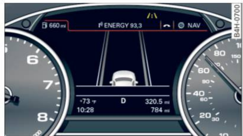
Fig. 96 Instrument cluster: Active lane assist is switched on but not ready to provide warnings
