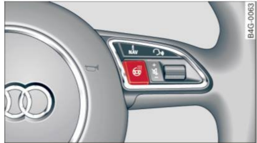
Fig. 71 Steering column: steering wheel heating button
