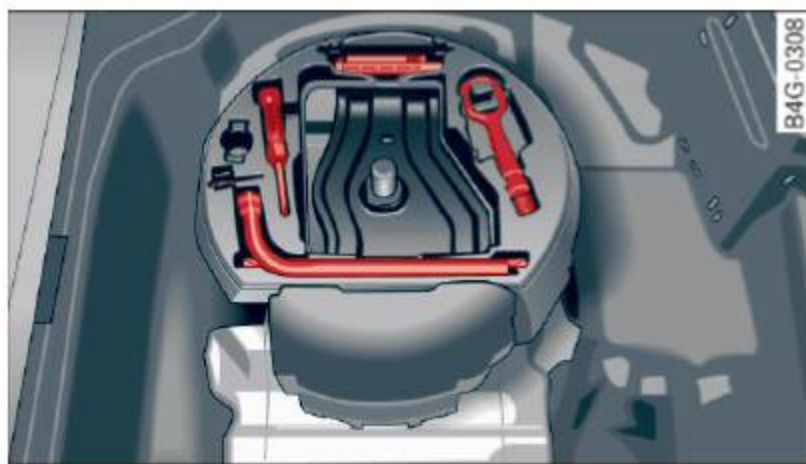
Fig. 201 Trunk lid: Vehicle tool kit
