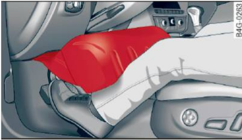
Fig. 161 Inflated airbags protecting in a frontal collision
