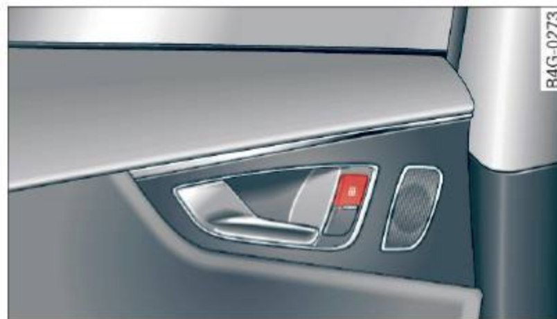
Fig. 24 Rear power locking switch
