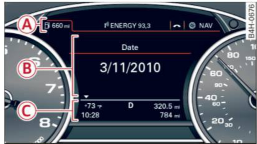
Fig. 4 Driver information system in the instrument cluster
