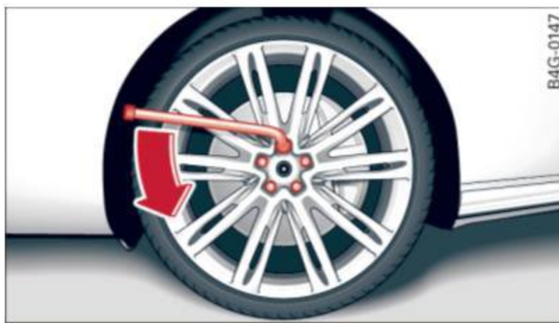
Fig. 204 Changing a wheel: loosening the wheel bolts
