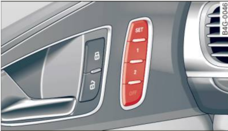
Fig. 52 Driver's door: memory function buttons
