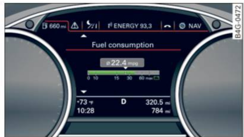
Fig. 10 Instrument cluster: fuel consumption
