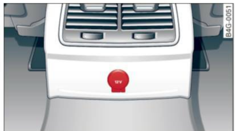
Fig. 57 Rear center console: 12-volt socket
