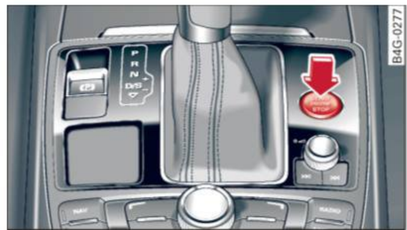
Fig. 74 Center console: START ENGINE STOP button
