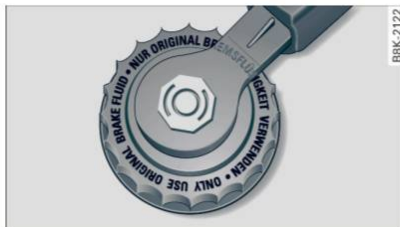
Fig. 188 Engine compartment: cover on the brake fluid reservoir
