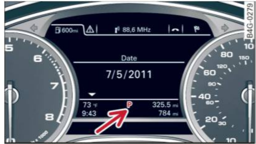
Fig. 111 Display in the instrument cluster: selector lever position
