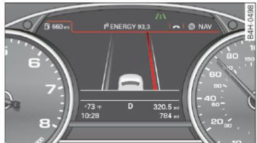
Fig. 95 Display: Active lane assist is switched on and is warning
