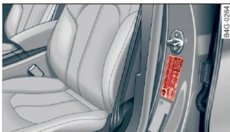
Fig. 191 Tire pressure label: located on driver's side B-pillar
