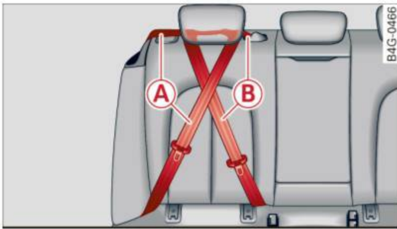
Fig. 166 Schematic overview: keep unused safety belts away from children in child safety seats. A - outer rear safety belt, B - center rear safety belt*
