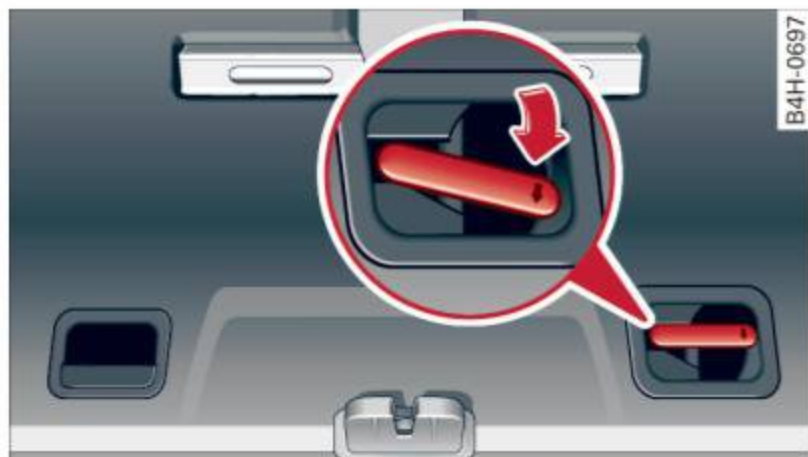
Fig. 198 Trunk escape handle: View from inside the closed trunk
