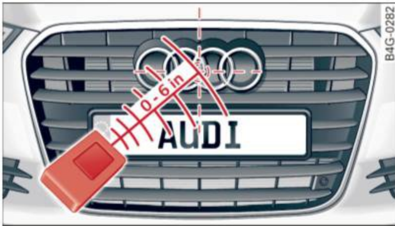
Fig. 142 Distance between the radiator grille and the hand transmitter
