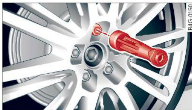
Fig. 208 Changing a wheel: using the screwdriver handle (with the blade removed) to turn the bolts
