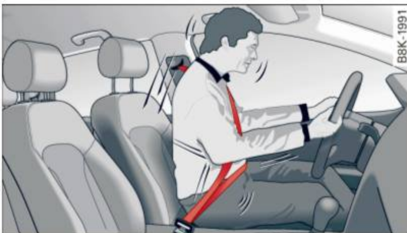
Fig. 150 Driver is correctly restrained in a sudden braking maneuver
