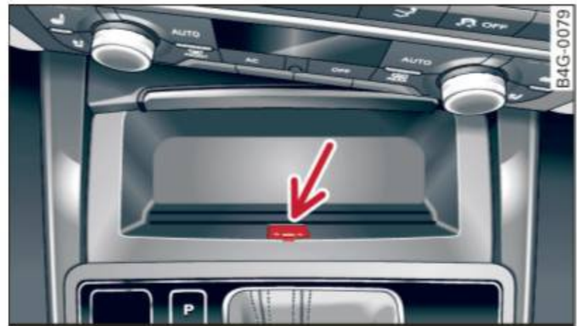
Fig. 116 Front center console: selector lever emergency release
