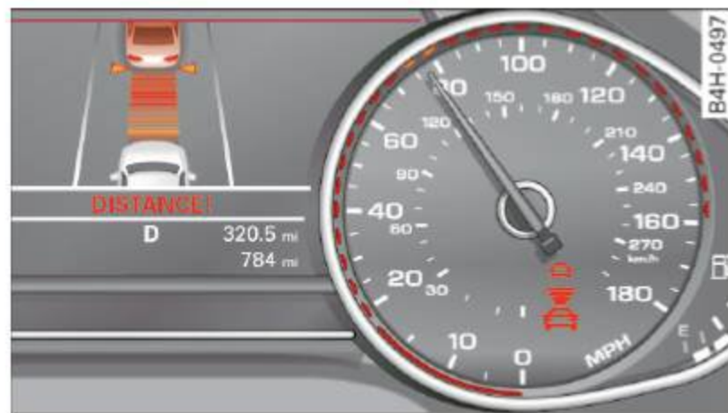
Fig. 92 Instrument cluster: approach warning
