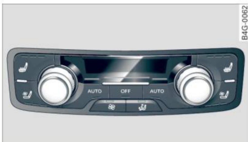
Fig. 70 Four-zone automatic climate control: rear controls
