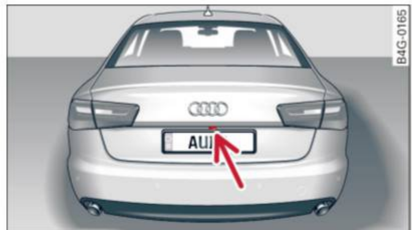
Fig. 123 Rear lid: Location of the rear view camera
