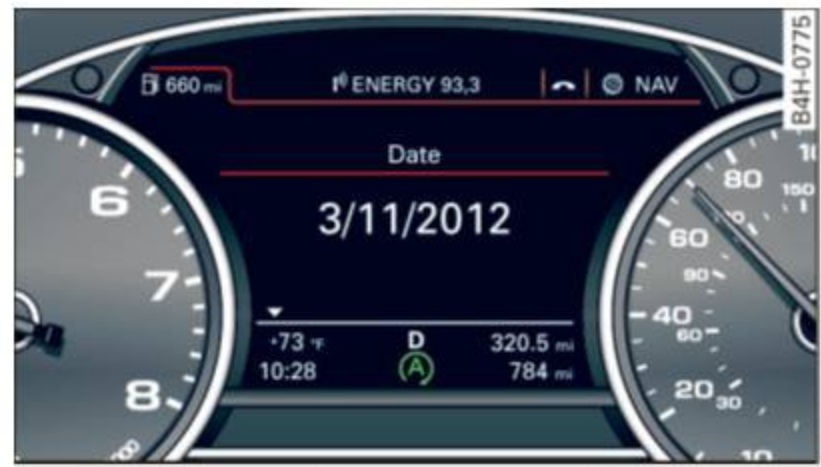
Fig. 77 Instrument cluster: engine switched off (stop phase)
