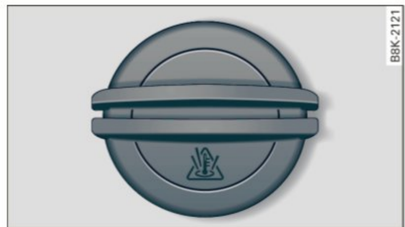
Fig. 187 Engine compartment: cover on the coolant expansion tank
