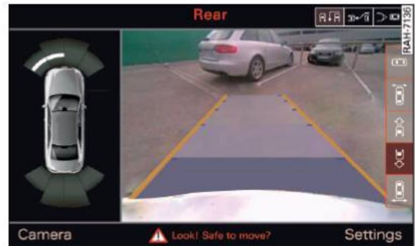
Fig. 137 Infotainment: aligning the vehicle
