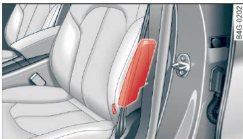
Fig. 162 Side airbag location in the driver's seat
