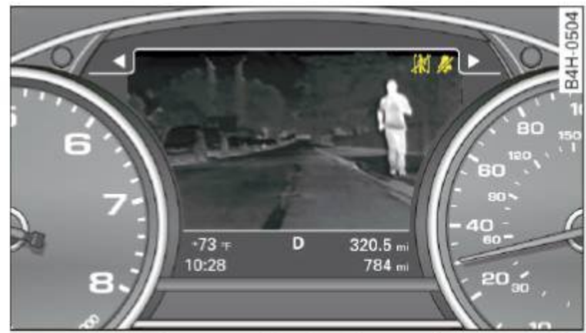
Fig. 110 Display: example of pedestrian detection and warning tone switched off
