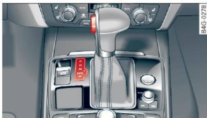
Fig. 113 Shift gate on the center console: selector lever with release button
