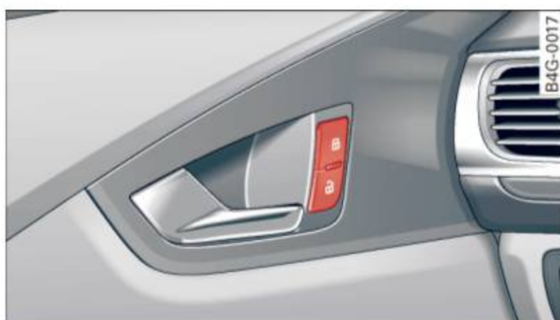
Fig. 23 Driver's door: power locking switch
