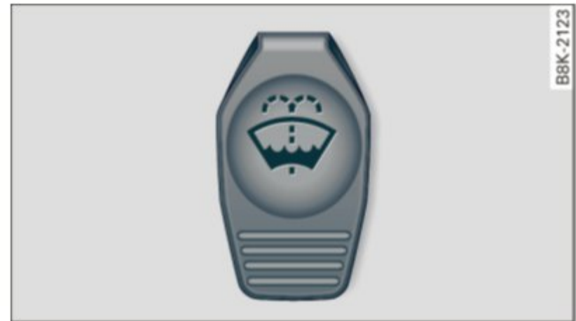
Fig. 190 Engine compartment: cover on the windshield and headlight* washer fluid reservoir
