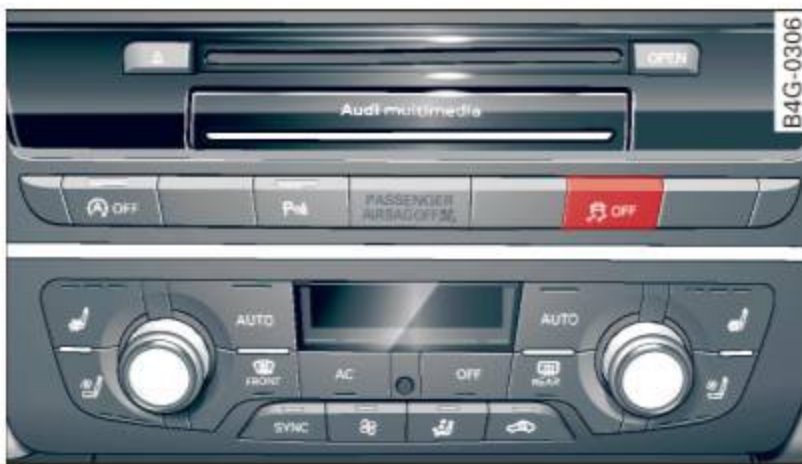
Fig. 177 Center console with ESC OFF button
