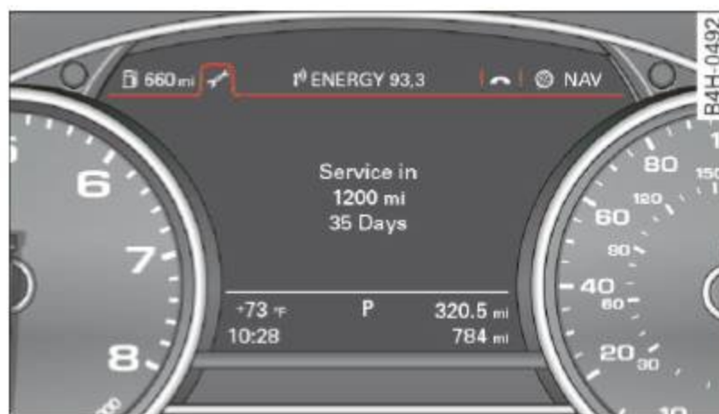
Fig. 13 Instrument cluster: Service interval display
