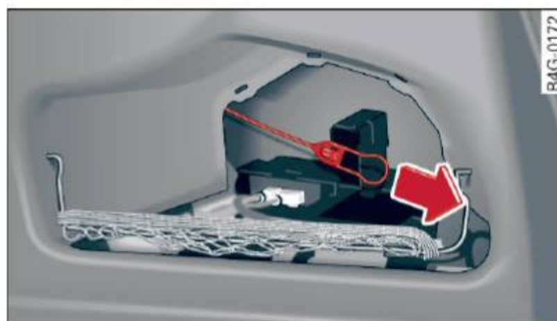
Fig. 181 Right side trim panel in the luggage compartment: emergency release mechanism
