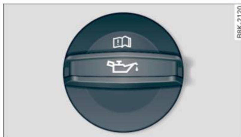
Fig. 186 Engine compartment: cover on the engine oil filler neck
