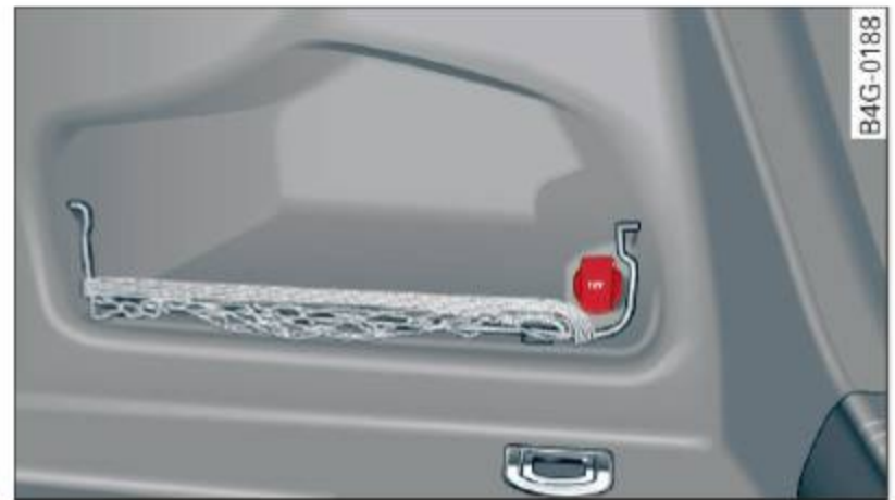
Fig. 56 Section of the trim panel of the luggage compartment: 12-volt socket
