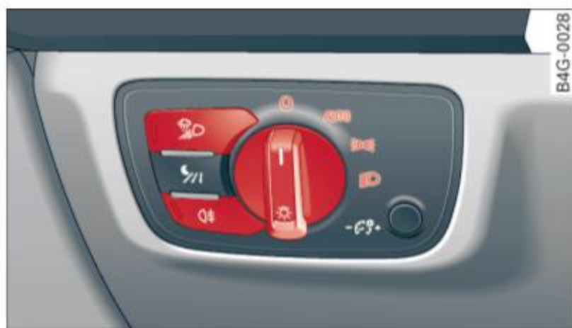
Fig. 33 Instrument panel: light switch with all-weather lights*
