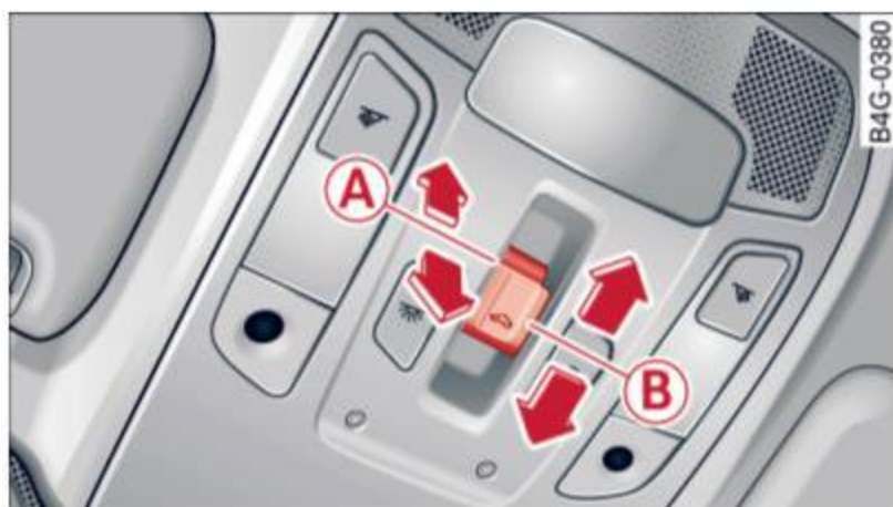
Fig. 32 Section of the headliner: Sliding/tilting sunroof button
