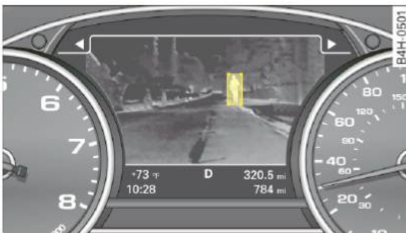
Fig. 104 Display: yellow pedestrian marking
