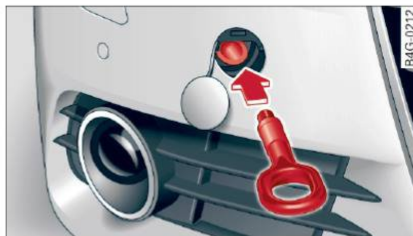
Fig. 217 Front bumper: installing the towing loop
