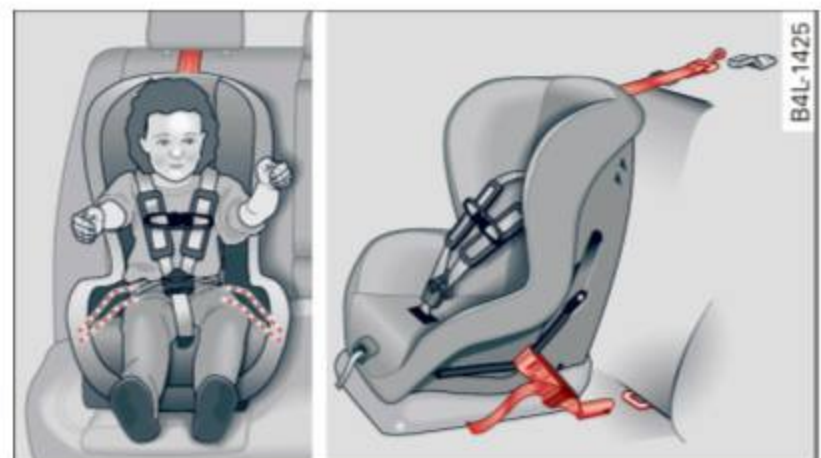
Fig. 168 Schematic overview: installation of the attachments applicable to a LATCH seat
