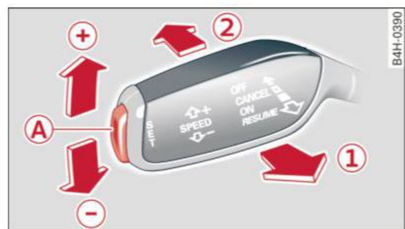
Fig. 80 Control lever with set button
