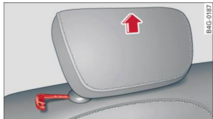
Fig. 51 Rear head restraints: release
