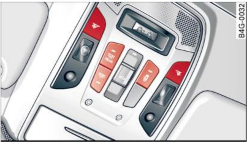
Fig. 36 Headliner: Front interior lights
