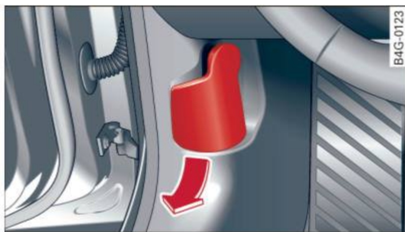
Fig. 182 Driver footwell: release lever
