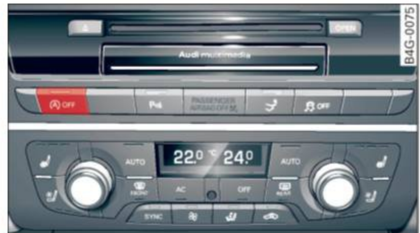
Fig. 79 Center console: Start-Stop-System button
