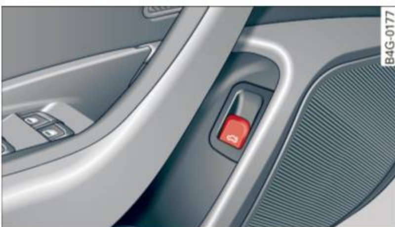
Fig. 26 Driver's door: remote rear lid release
