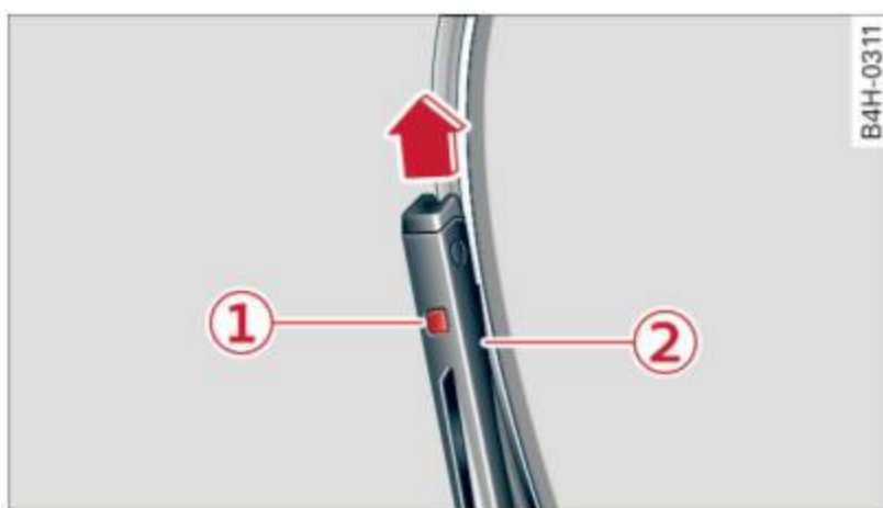
Fig. 43 Removing windshield wiper blades
