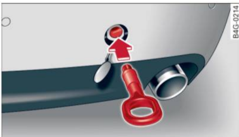
Fig. 219 Rear bumper: towing loop installed
