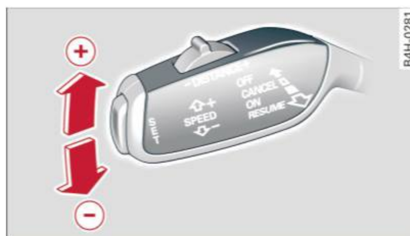
Fig. 88 Selector lever: changing the speed
