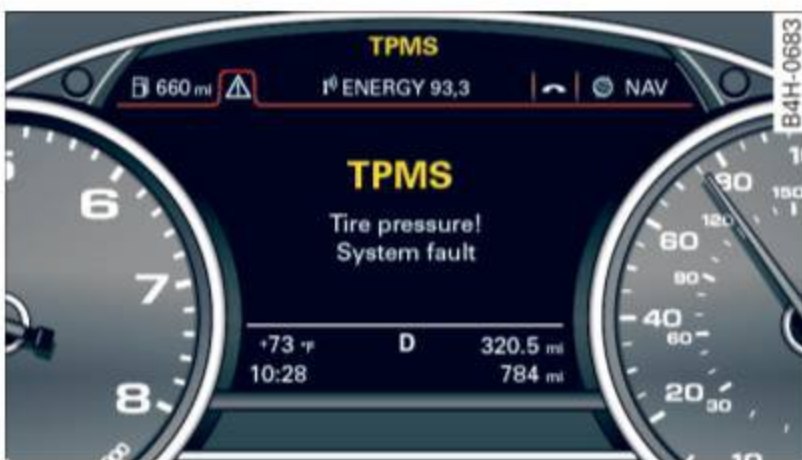
Fig. 197 Display: System malfunction
