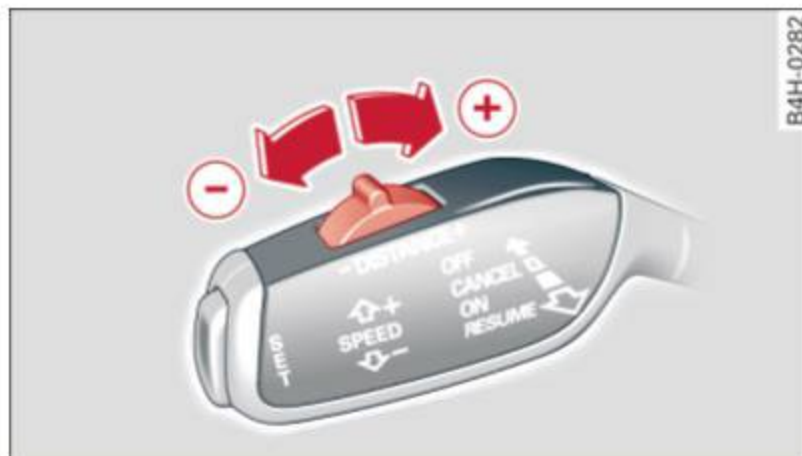
Fig. 90 Selector lever: setting the distance
