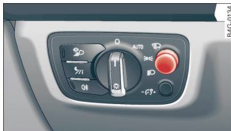
Fig. 15 Instrument panel: knob for the Head-up Display
