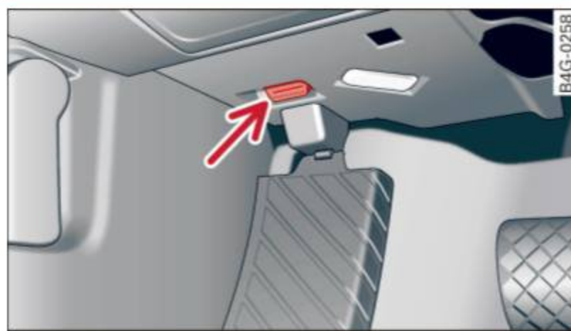
Fig. 16 Location of Data Link Connector (DLC)
