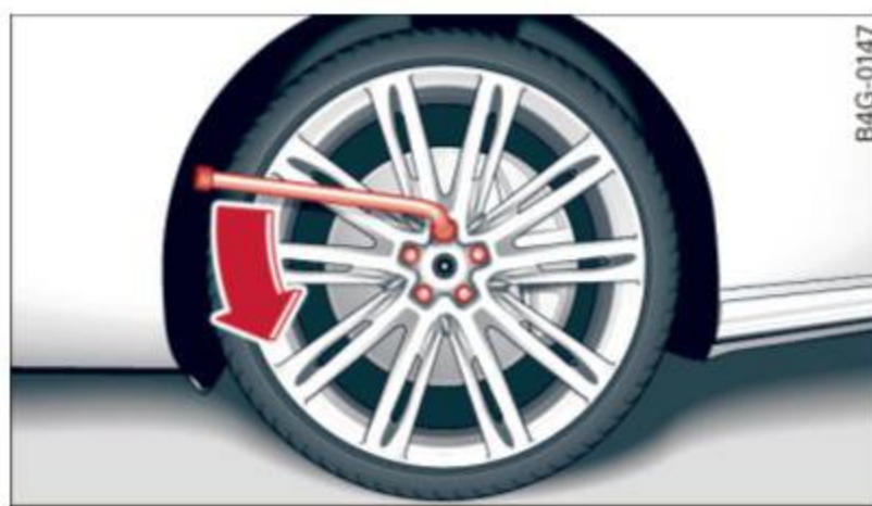
Fig. 208 Changing a wheel: loosening the wheel bolts
