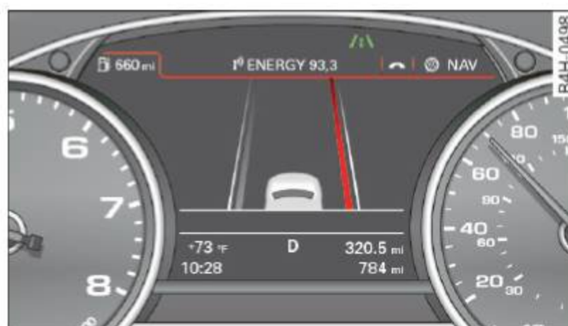
Fig. 98 Display: Active lane assist is switched on and is warning
