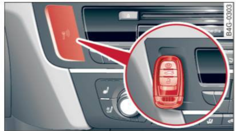
Fig. 78 Center console/master key: starting the engine if there is a malfunction
