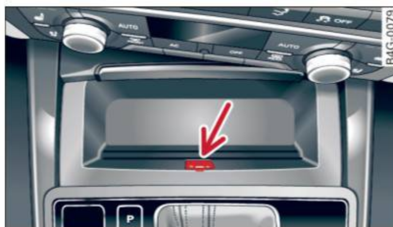
Fig. 119 Front center console: selector lever emergency release
