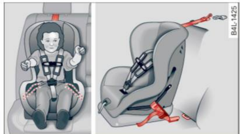
Fig. 169 Schematic overview: installation of the attachments applicable to a LATCH seat
