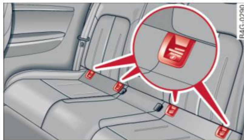
Fig. 174 Rear seats: lower anchorage bracket locations
