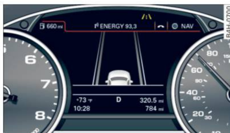
Fig. 99 Instrument cluster: Active lane assist is switched on but not ready to provide warnings
