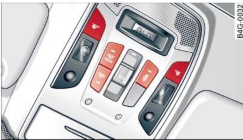
Fig. 39 Headliner: Front interior lights
