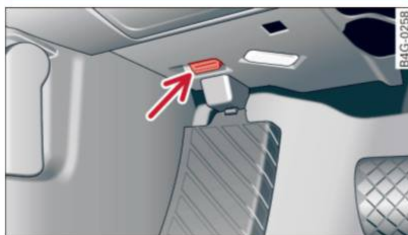
Fig. 16 Location of Data Link Connector (DLC)
