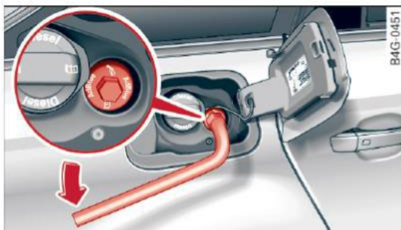
Fig. 184 Right rear vehicle side: removing the AdBlue cap
