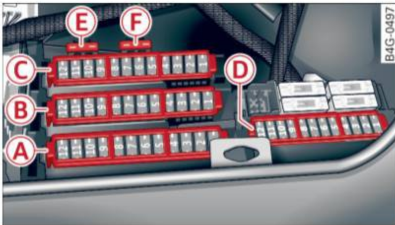
Fig. 217 Luggage compartment: fuse panel with plastic bracket
