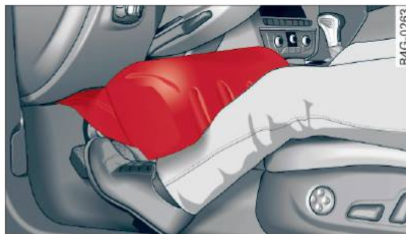
Fig. 162 Inflated airbags protecting in a frontal collision
