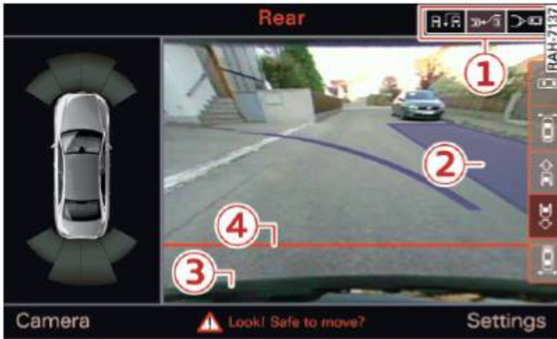
Fig. 141 Infotainment: blue surfaces aligned in the parking space
