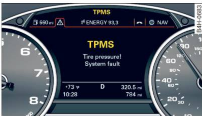
Fig. 201 Display: System malfunction
