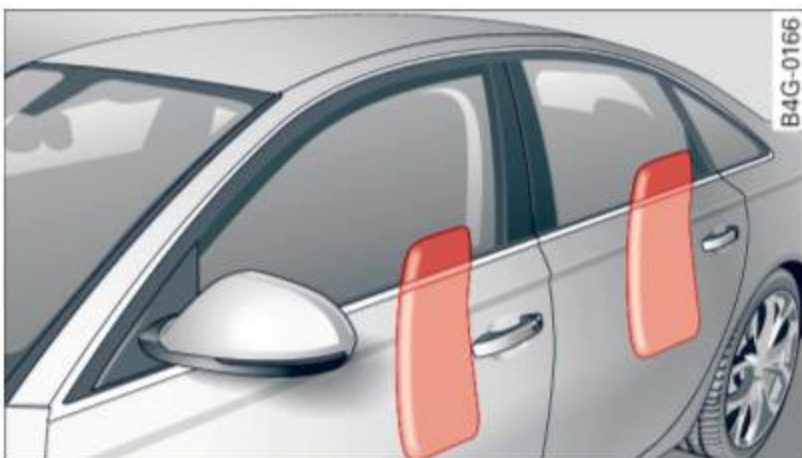
Fig. 164 Inflated side airbags on left side of vehicle, rear side airbag
