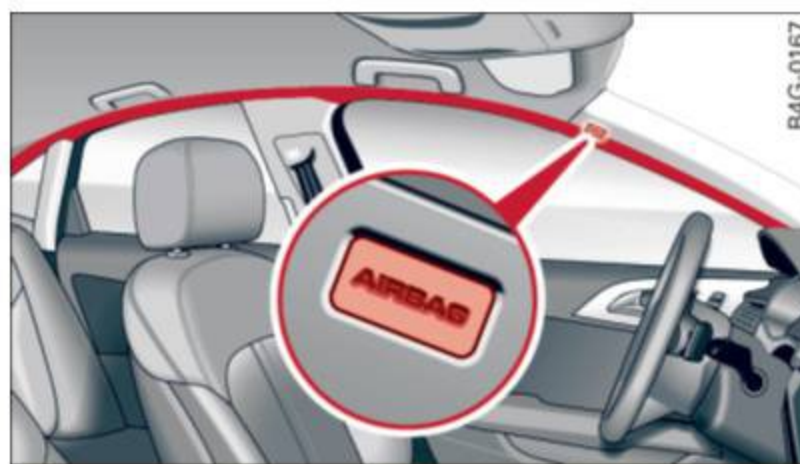
Fig. 165 Side curtain airbags, driver's side: side curtain airbag location
