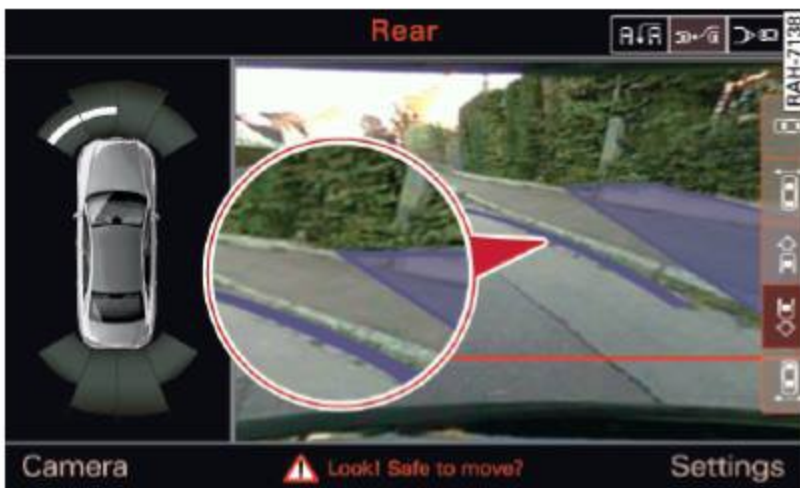
Fig. 142 Infotainment: contact of the blue curved line with the curb
