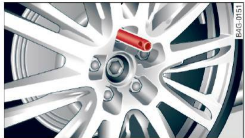
Fig. 213 Changing a wheel: alignment pin inside the top hole
