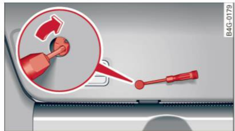
Fig. 29 Section of the luggage compartment: access to emergency release
