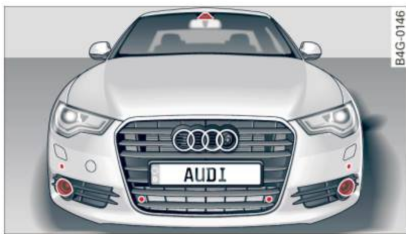
Fig. 85 Front of the vehicle: sensors and video camera
