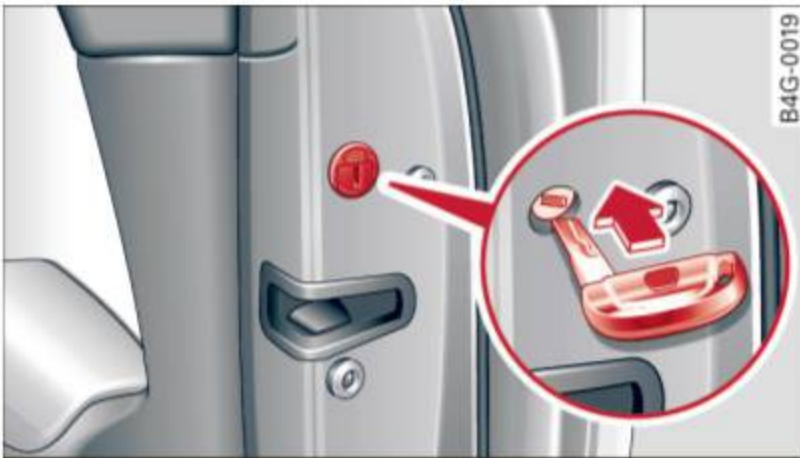
Fig. 25 Door: Emergency locking
