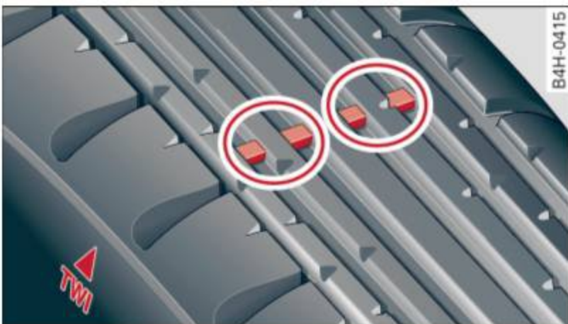
Fig. 197 Tire tread: tread wear indicators (TWI)
