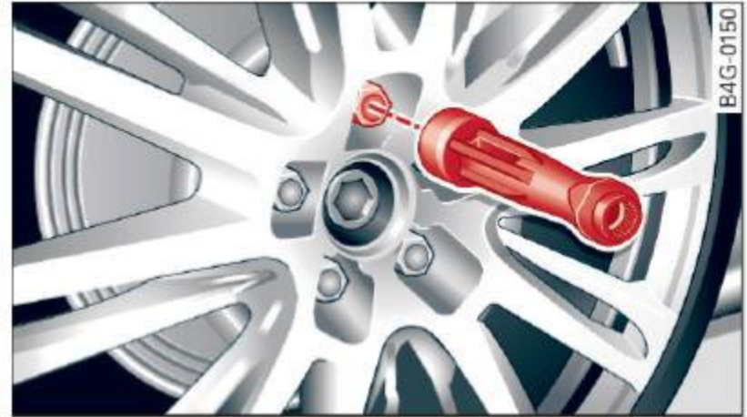
Fig. 212 Changing a wheel: using the screwdriver handle (with the blade removed) to turn the bolts
