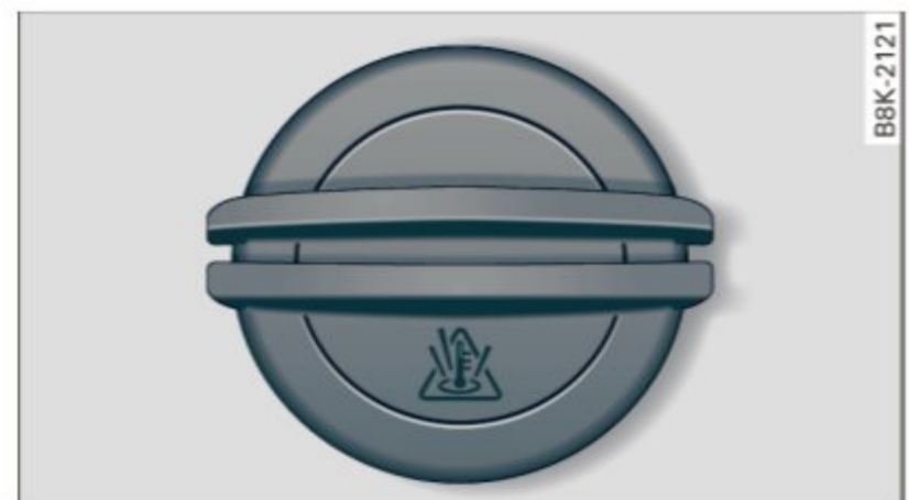
Fig. 191 Engine compartment: cover on the coolant expansion tank
