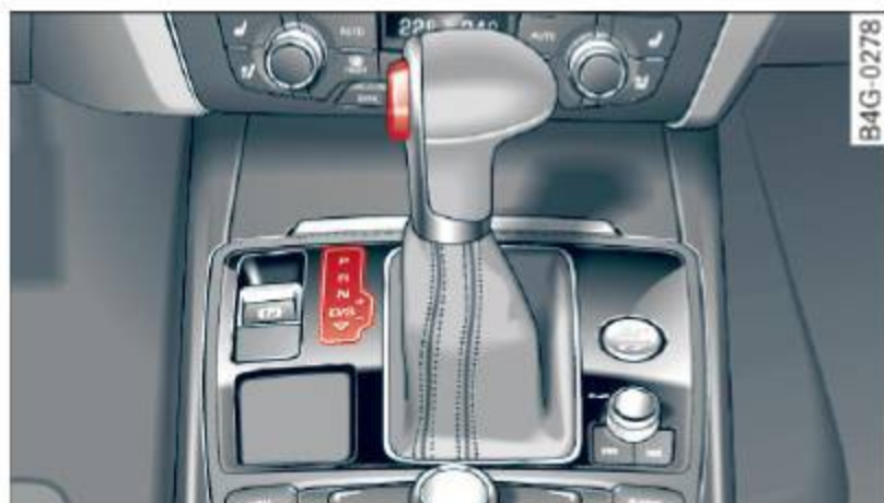
Fig. 116 Shift gate on the center console: selector lever with release button
