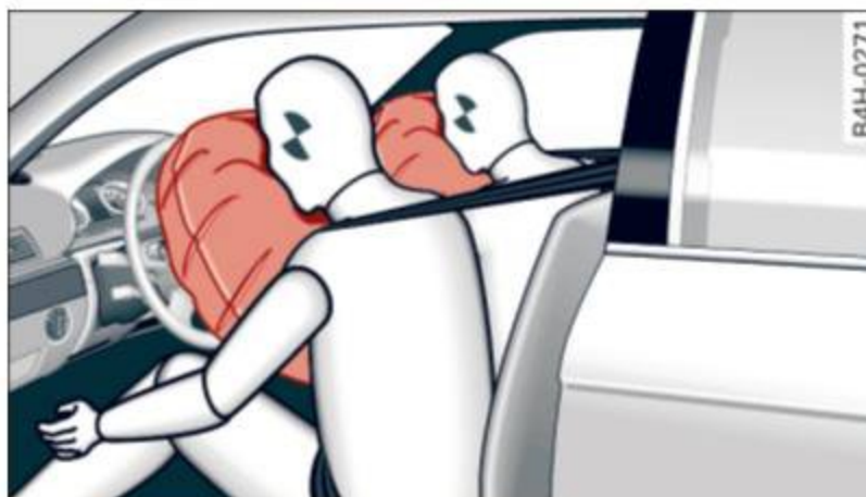
Fig. 159 Inflated front airbags
