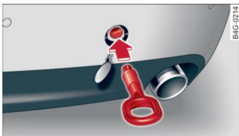
Fig. 223 Rear bumper: towing loop installed
