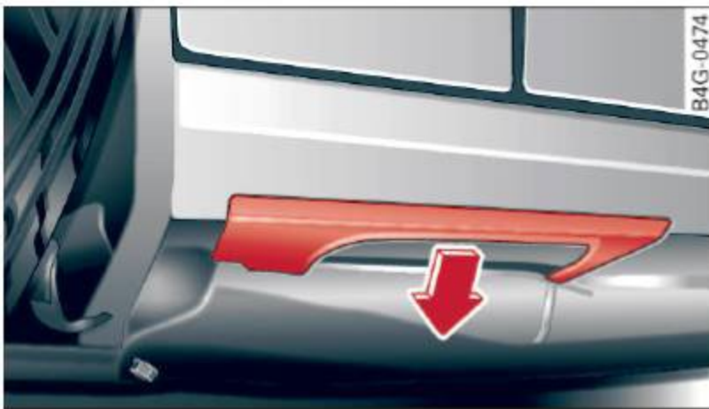
Fig. 211 Sill: removing the cover
