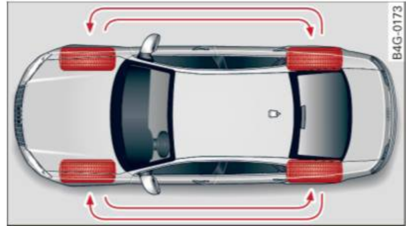
Fig. 198 Rotating tires for more even wear
