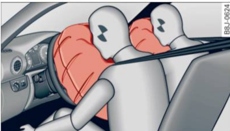
Fig. 106 Inflated front airbags
