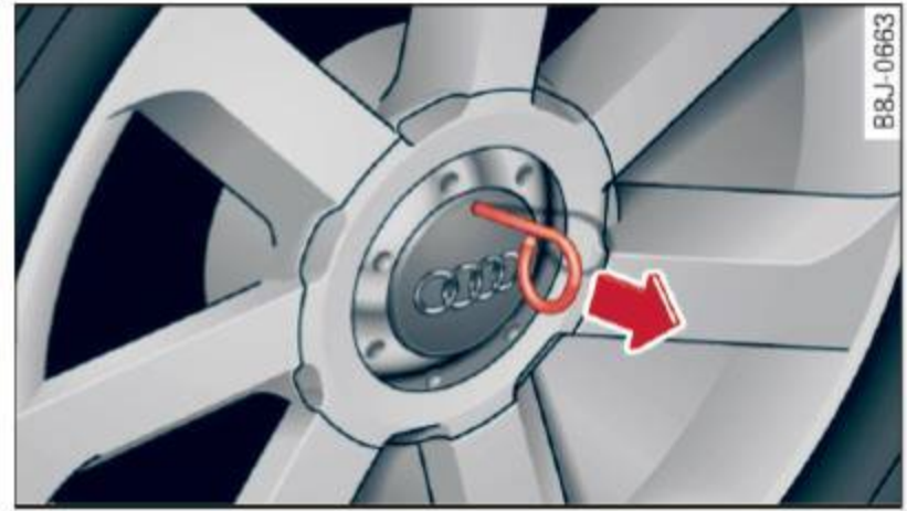
Fig. 158 Wheel change: removing the wheel cover
