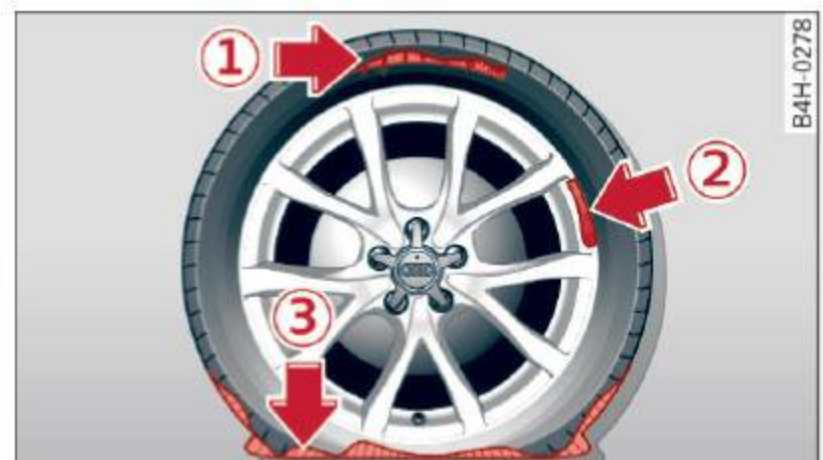
Fig. 153 Tire damage for which the Tire Mobility System is not suited
