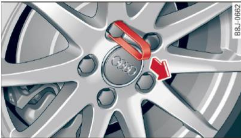
Fig. 157 Wheel change: removing the wheel bolt caps
