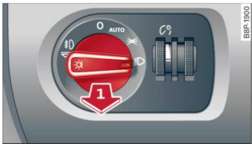
Fig. 42 Fog light activation: light switch position on vehicles WITHOUT sensor light
