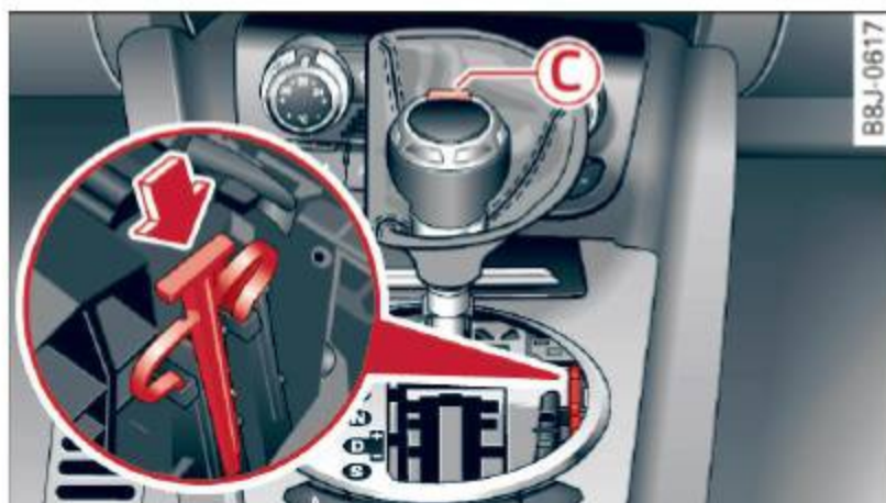
Fig. 87 Selector lever: Using the emergency release to move out of the Park position
