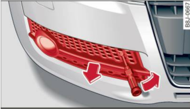
Fig. 170 Front bumper: removing the grill
