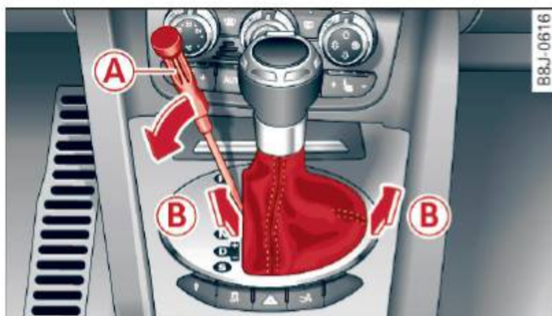
Fig. 86 Selector lever: Removing the selector lever boot
