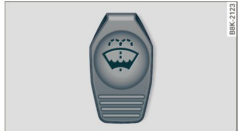
Fig. 141 Fender, left: cover on the windshield and headlight* washer fluid reservoir
