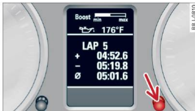
Fig. 20 Display: boost and engine oil temperature indicator
