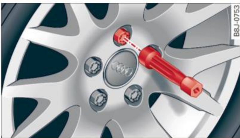
Fig. 162 Wheel change: using the screwdriver handle (with the blade removed) to turn the bolts
