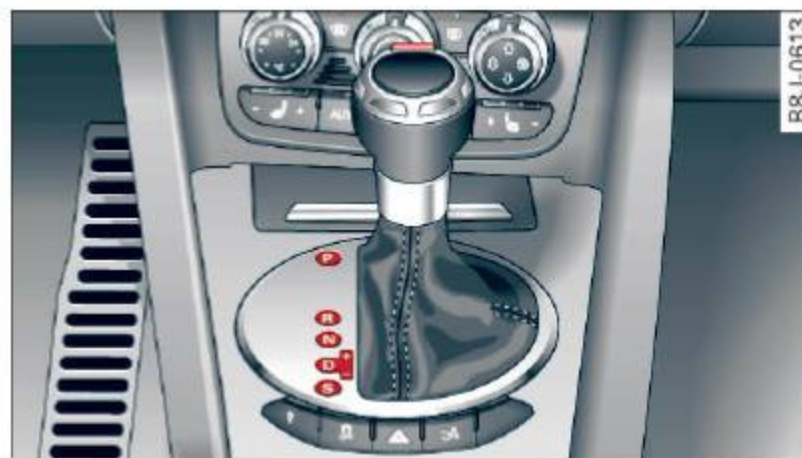
Fig. 82 Section from center console: Selector lever with release button
