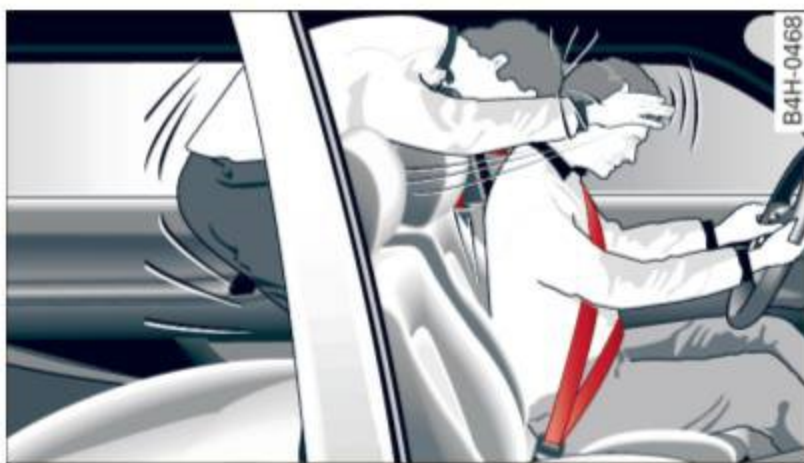
Fig. 98 A rear passenger not wearing a safety belt will fly forward and strike the driver
