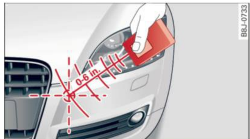
Fig. 89 Front bumper, driver side: location of transmitter unit
