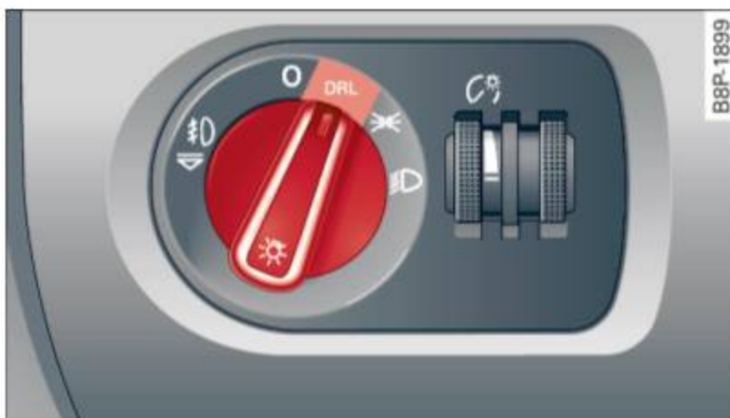
Fig. 40 Instrument panel: light switch with daytime running lights (DRL)
