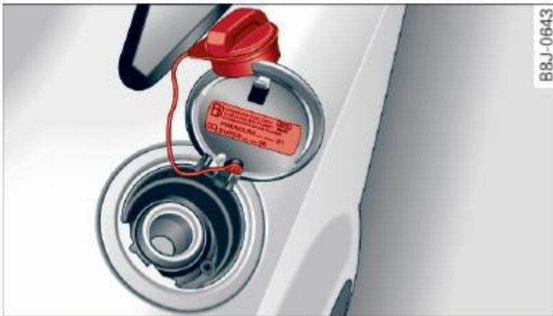
Fig. 130 Fuel cap hooked on the opened fuel filler flap
