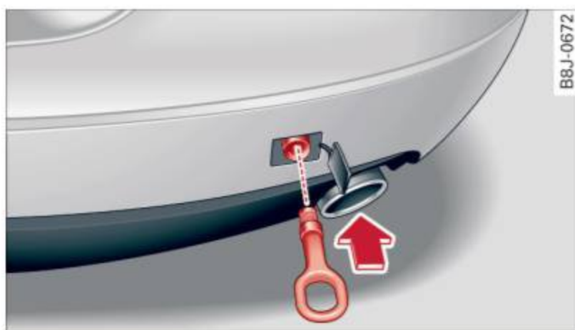
Fig. 175 Rear bumper: screwing in the towing loop
