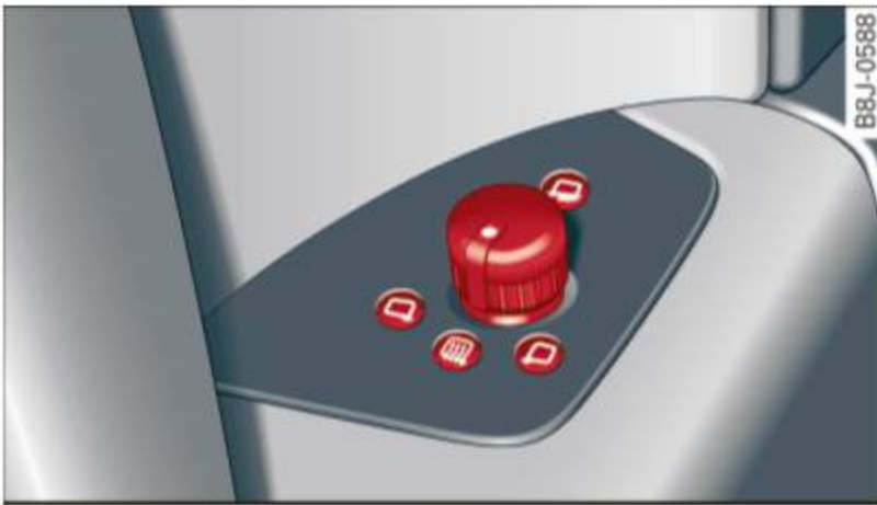
Fig. 48 Forward section of driver's armrest: power mirror controls
