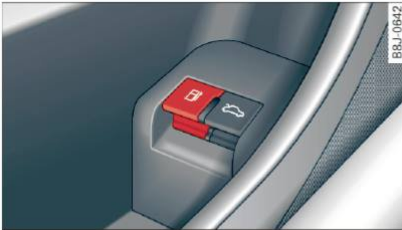
Fig. 129 Driver's door: Unlocking fuel filler flap
