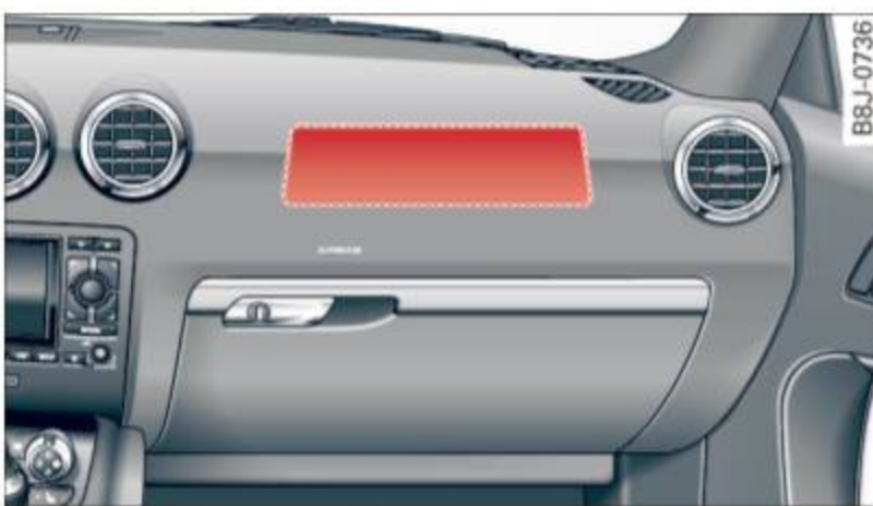
Fig. 105 Location of front passenger's airbag: in the instrument panel
