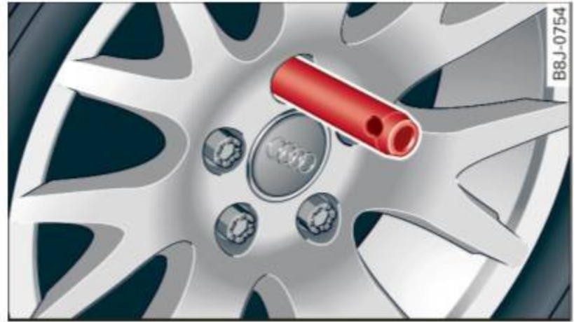
Fig. 163 Wheel change: alignment pin inside the top hole
