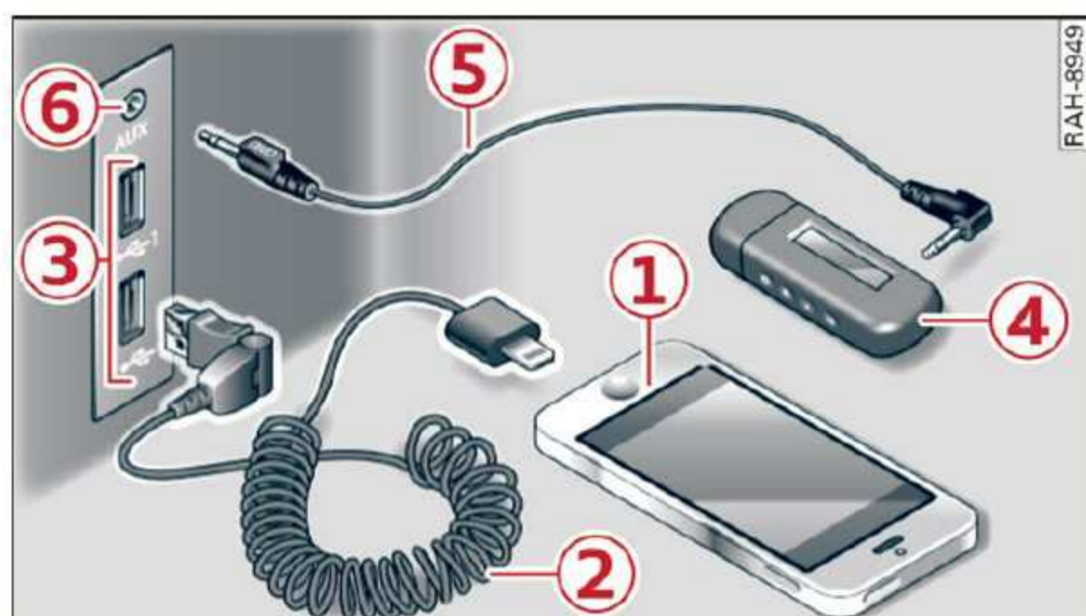
Fig. 136 Storage compartment in the center console: connecting mobile devices
