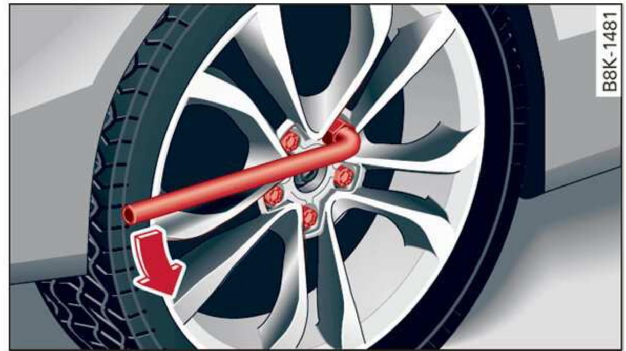
Fig. 192 Changing a tire: loosen the wheel bolts
