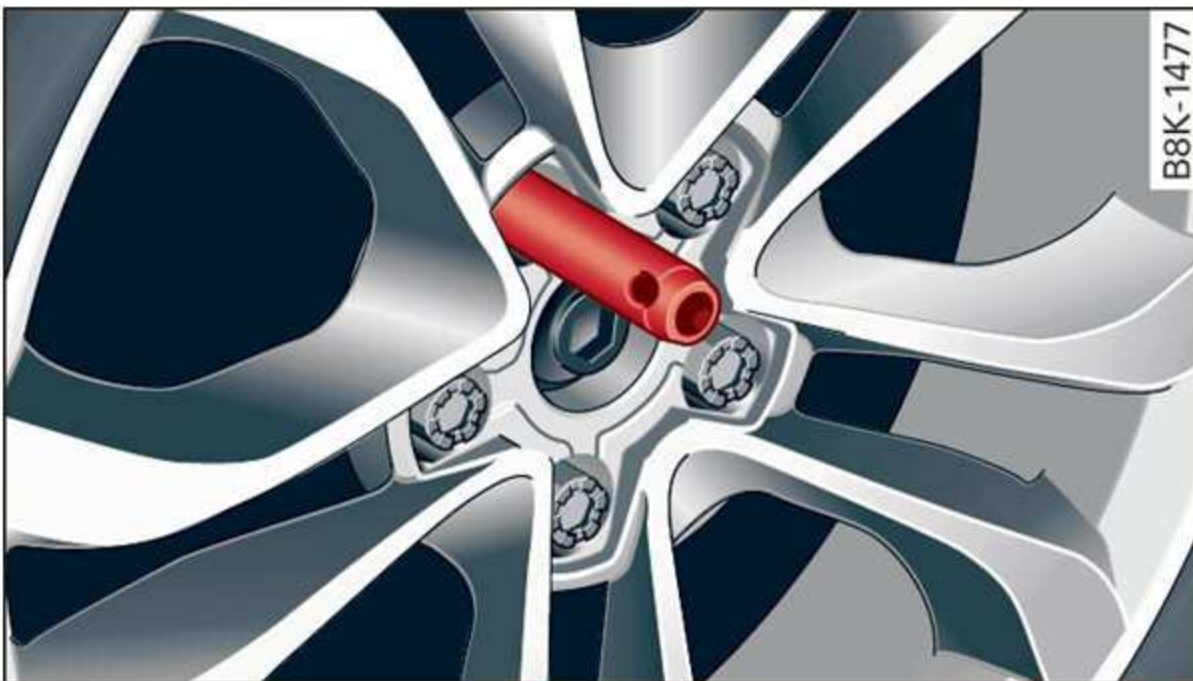
Fig. 196 Wheel: alignment pin in the top hole
