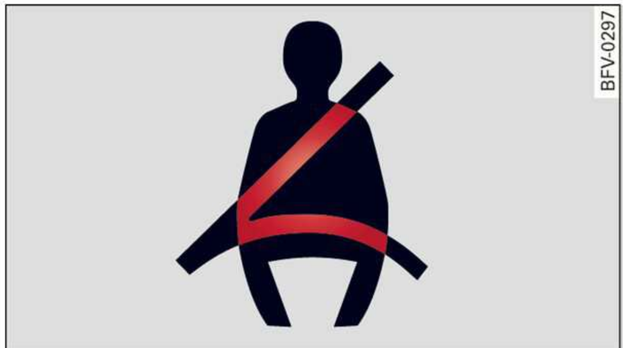
Fig. 146 Safety belt warning light in the instrument cluster - enlarged
