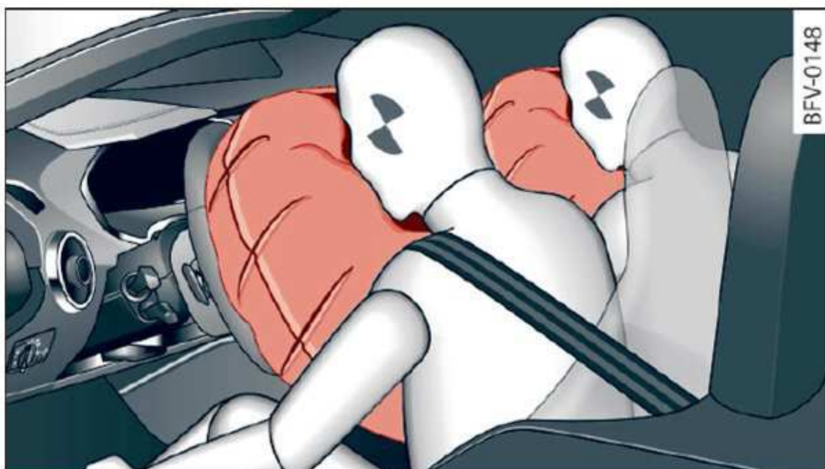
Fig. 157 Inflated front airbags
