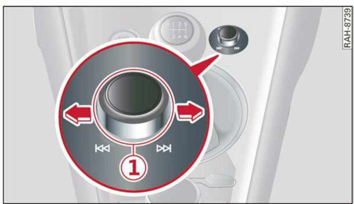
Fig. 94 MMI On/Off knob with joystick function
