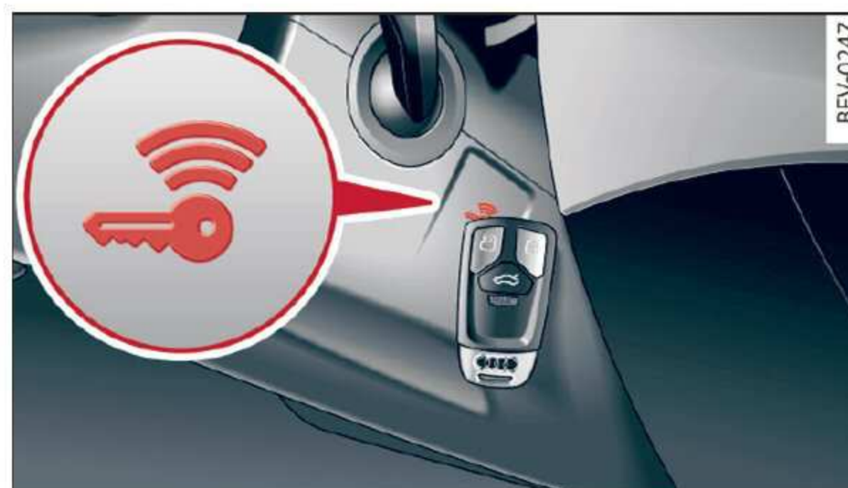
Fig. 66 Steering column/remote control key: starting the engine if there is a malfunction
