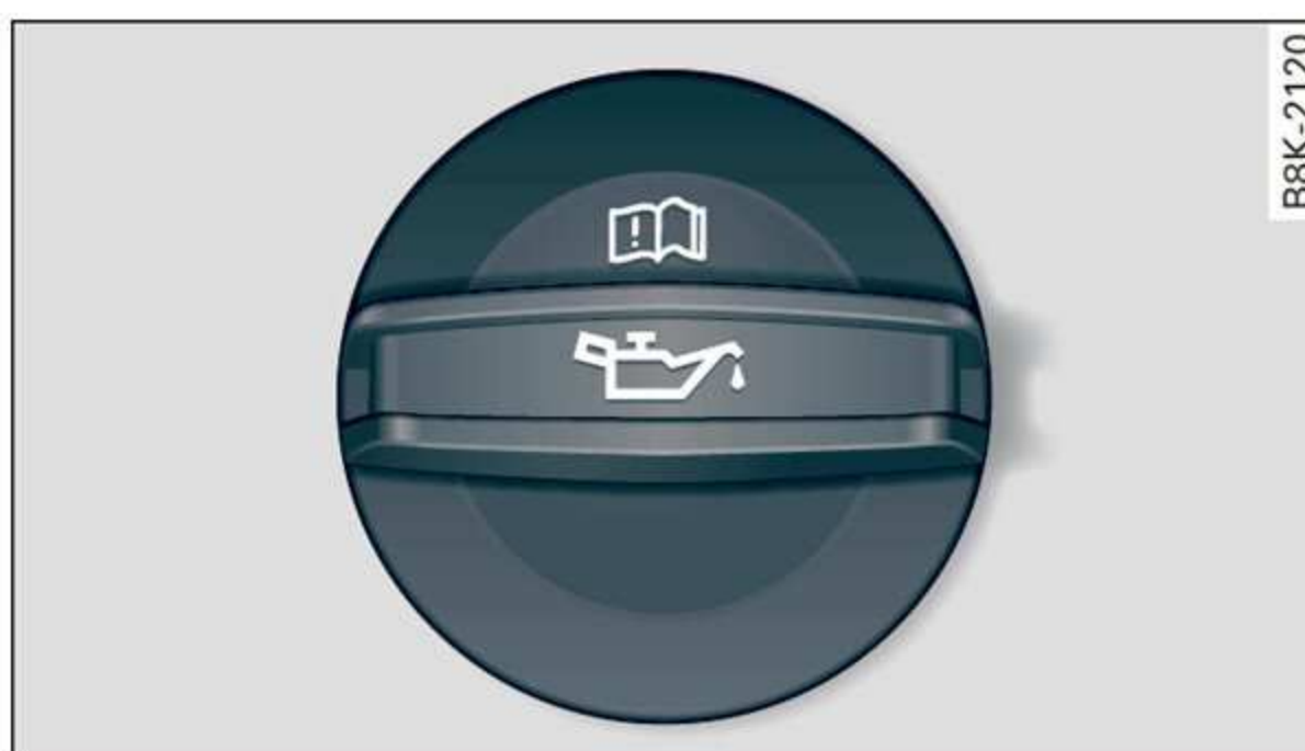
Fig. 176 Engine compartment: engine oil filler opening cover
