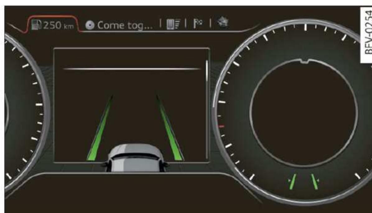
Fig. 77 Instrument cluster: active lane assist is switched on and ready to provide warnings
