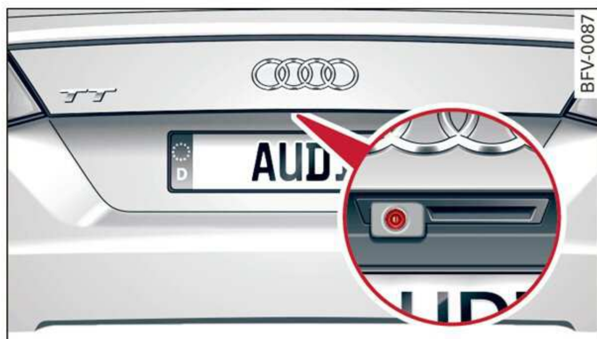
Fig. 88 Luggage compartment lid: location of the rear-view camera
