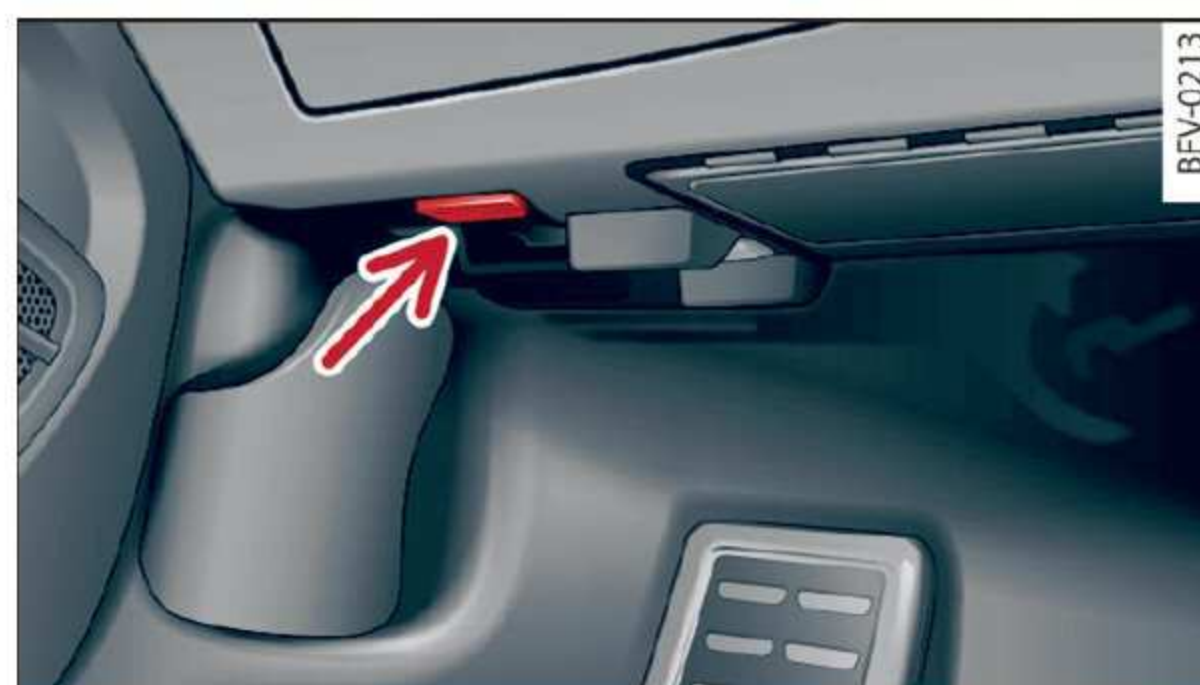
Fig. 171 Footwell on left side of the vehicle: connection port for the On Board Diagnostic System (OBD)
