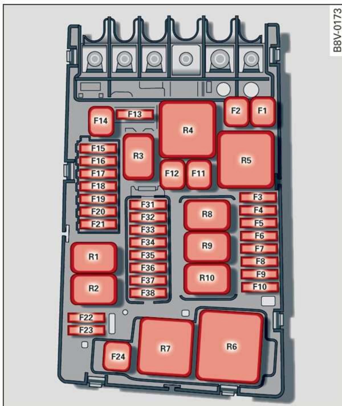
Fig. 203 Left side of engine compartment: fuse assignment
