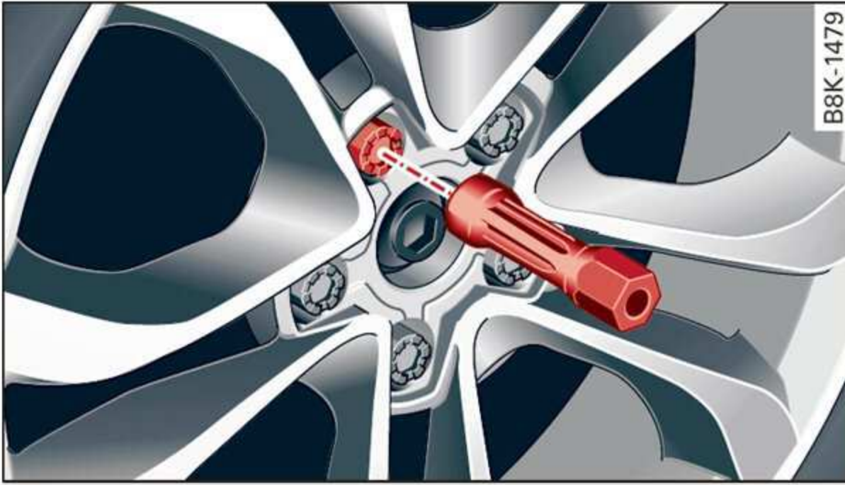
Fig. 195 Wheel: internal hex socket to turn the wheel bolts
