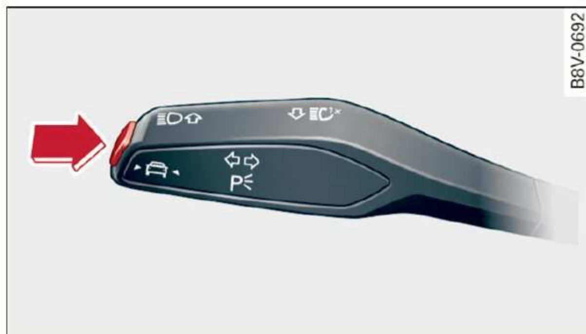
Fig. 75 Turn signal lever: button for active lane assist
