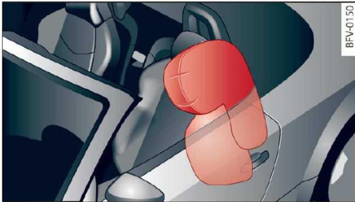
Fig. 162 Inflated side airbag on left side of vehicle
