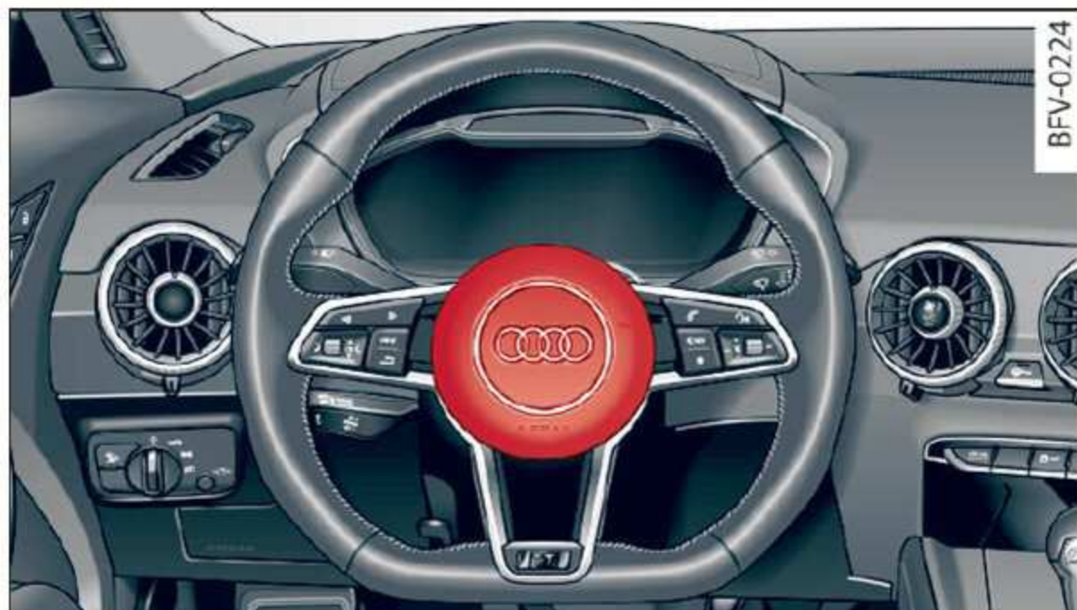
Fig. 155 Location of driver airbag: in steering wheel
