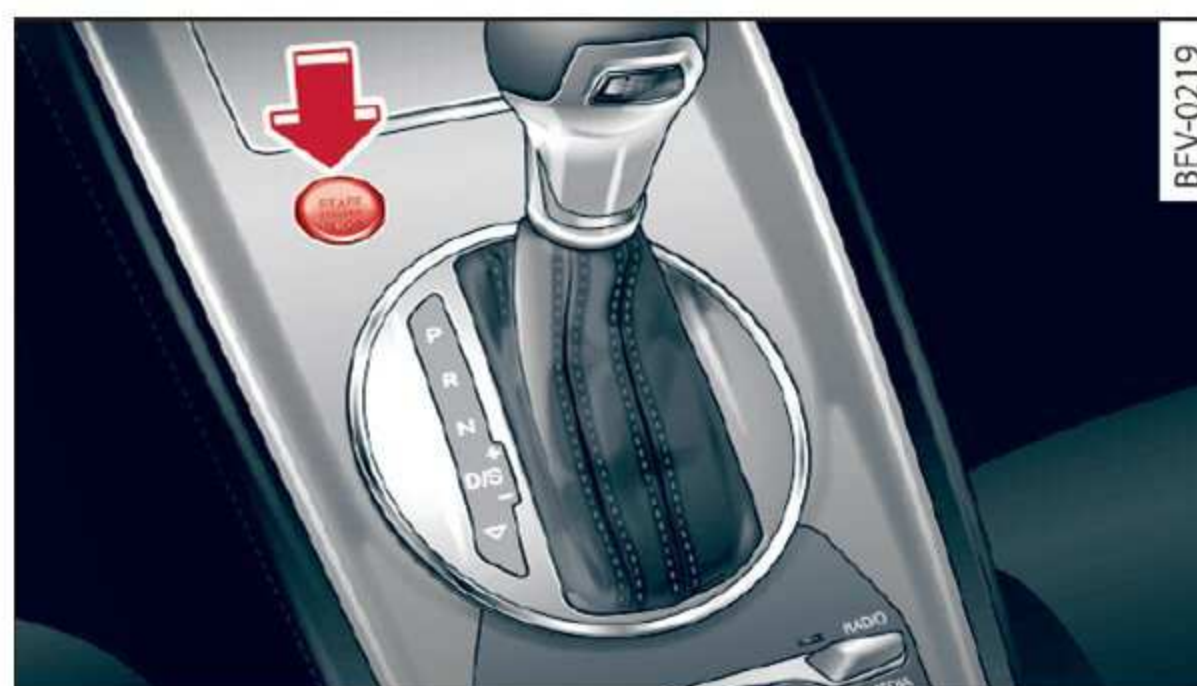
Fig. 65 Center console: START ENGINE STOP button
