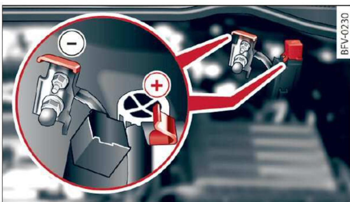
Fig. 179 Engine compartment: connectors for a charger or jump start cables
