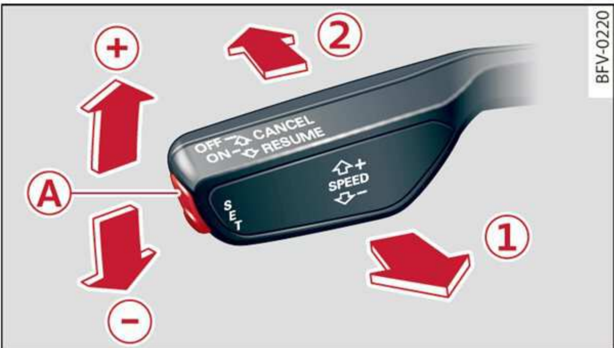
Fig. 74 Lever: switching on the cruise control system
