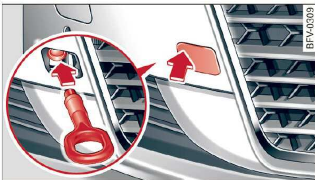
Fig. 198 Front bumper: installing the towing loop
