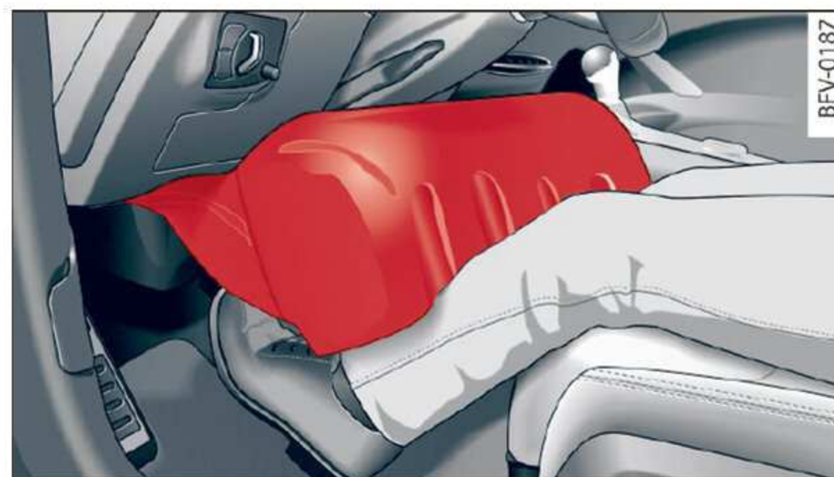
Fig. 160 Inflated airbags protecting in a frontal collision
