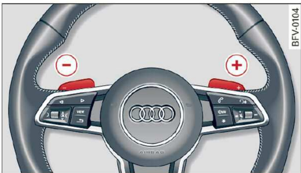
Fig. 71 Steering wheel: shifting manually with the shift paddles*
