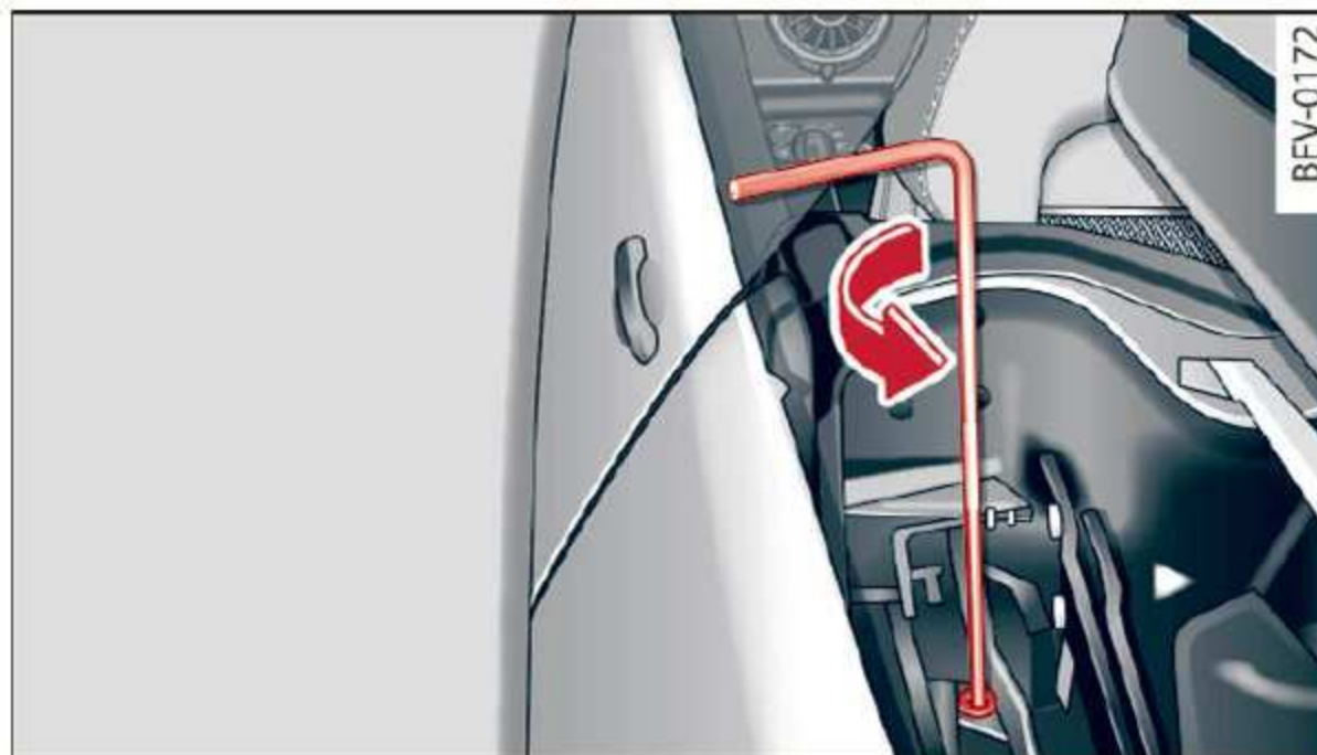
Fig. 33 Driver's side: inserted hex socket wrench
