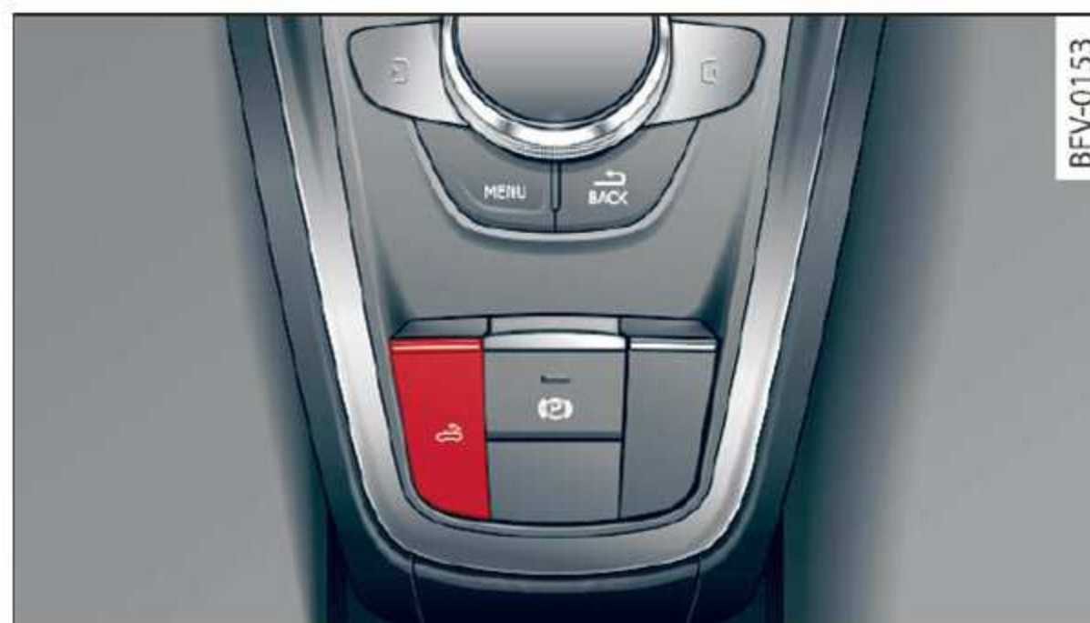
Fig. 27 Center console: power top switch (example)
