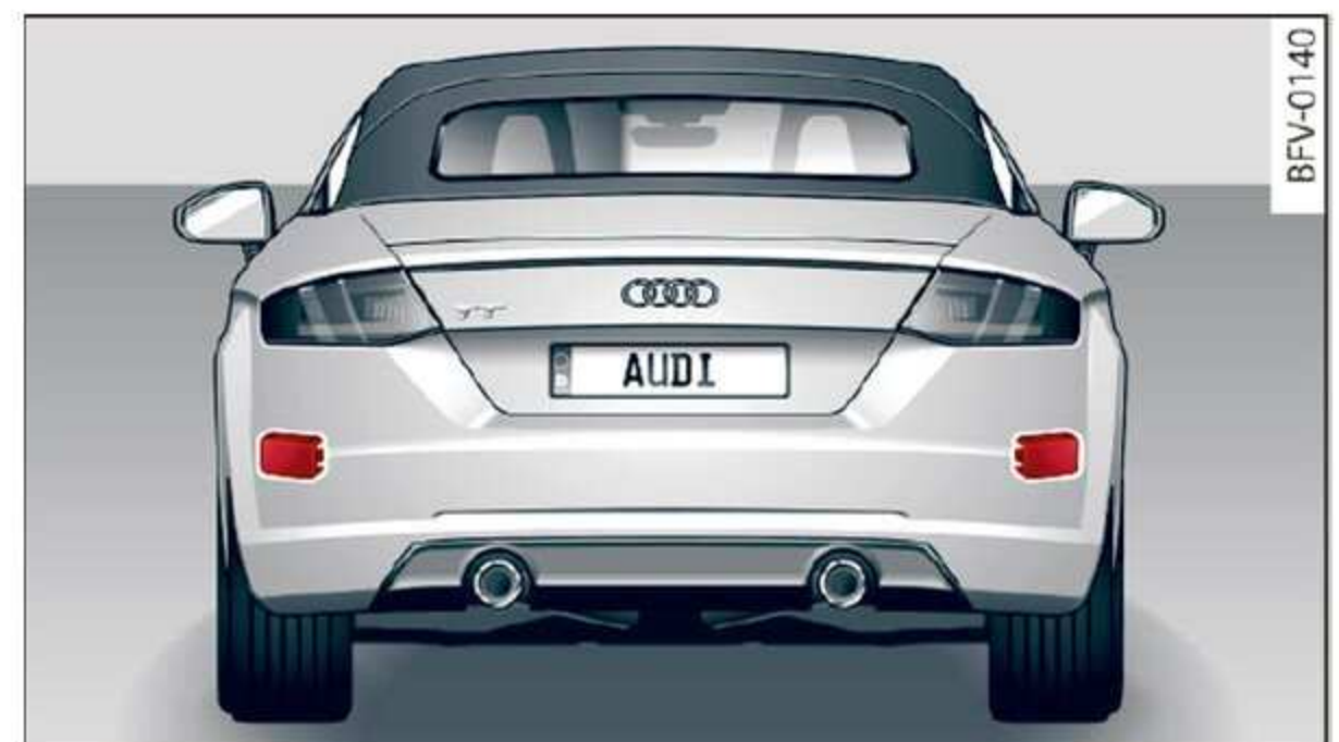
Fig. 81 Rear of the vehicle: position of the sensors (example)
