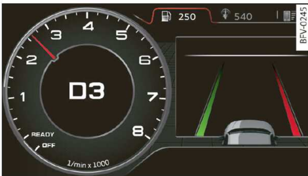
Fig. 67 Instrument cluster: selector lever positions
