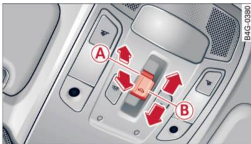
Fig. 32 Section of the headliner: Sliding/tilting sunroof button
