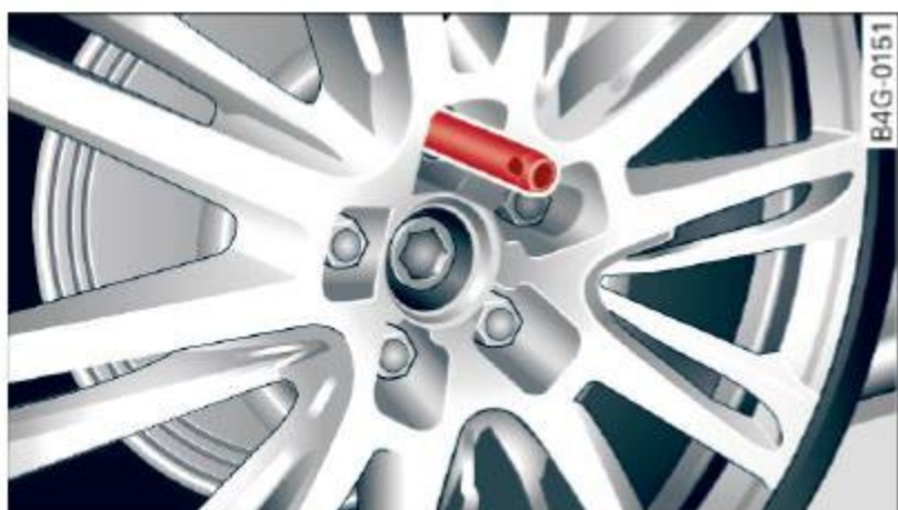
Fig. 213 Changing a wheel: alignment pin inside the top hole
