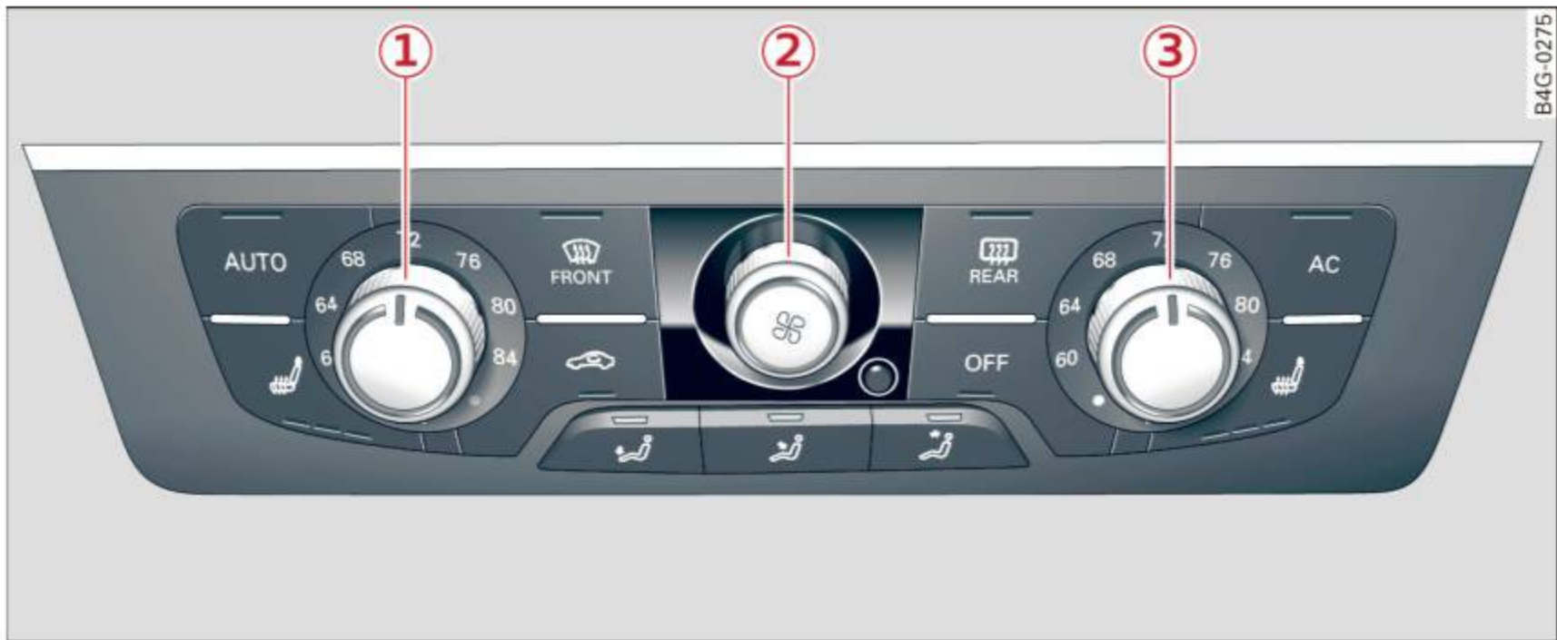
Fig. 72 Three-zone climate control: controls
