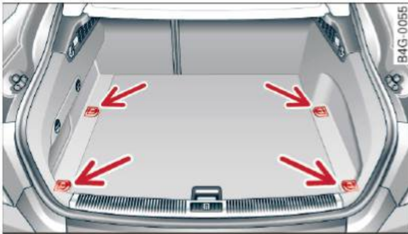
Fig. 65 Location of the tie-downs in the luggage compartment
