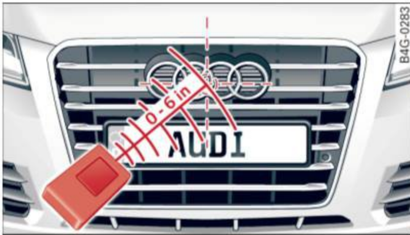
Fig. 146 Distance between the radiator grille and the hand transmitter
