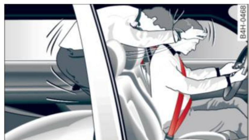
Fig. 153 A rear passenger not wearing a safety belt will fly forward and strike the driver
