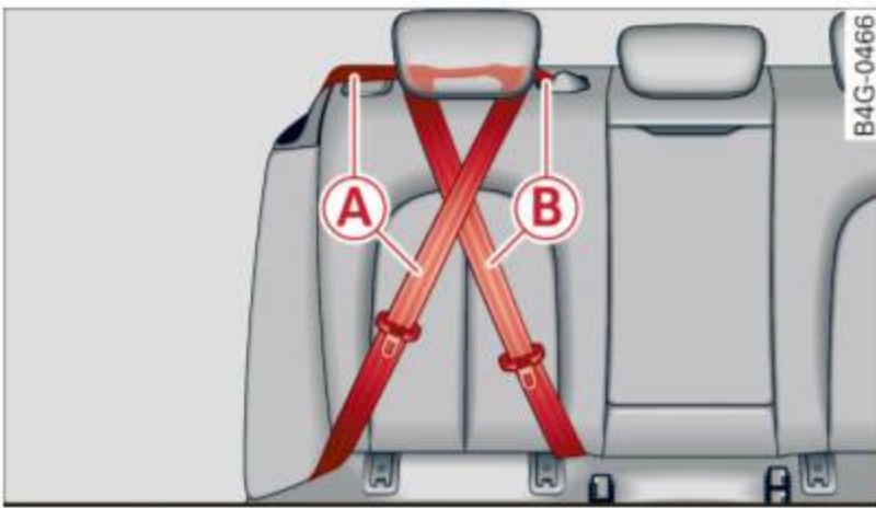
Fig. 170 Schematic overview: keep unused safety belts away from children in child safety seats. A - outer rear safety belt, B - center rear safety belt*
