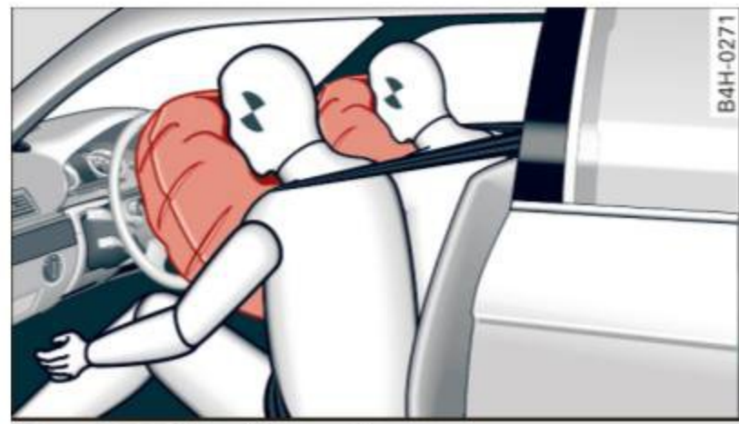
Fig. 162 Inflated front airbags
