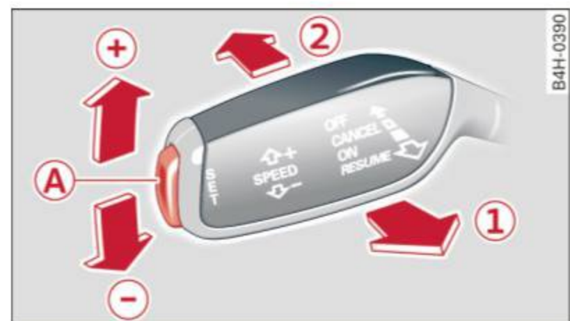
Fig. 84 Control lever with set button
