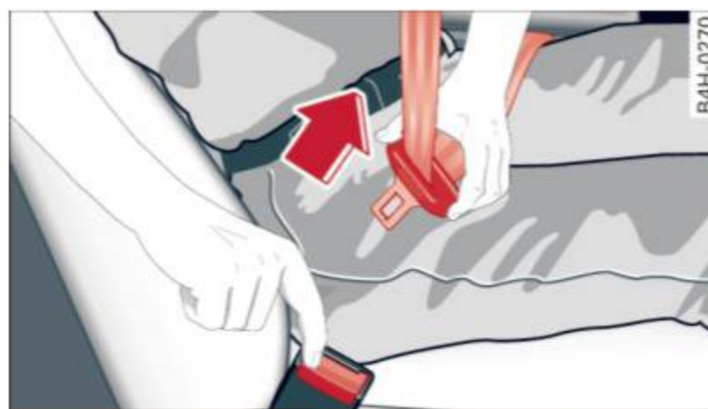
Fig. 158 Releasing the tongue from the buckle
