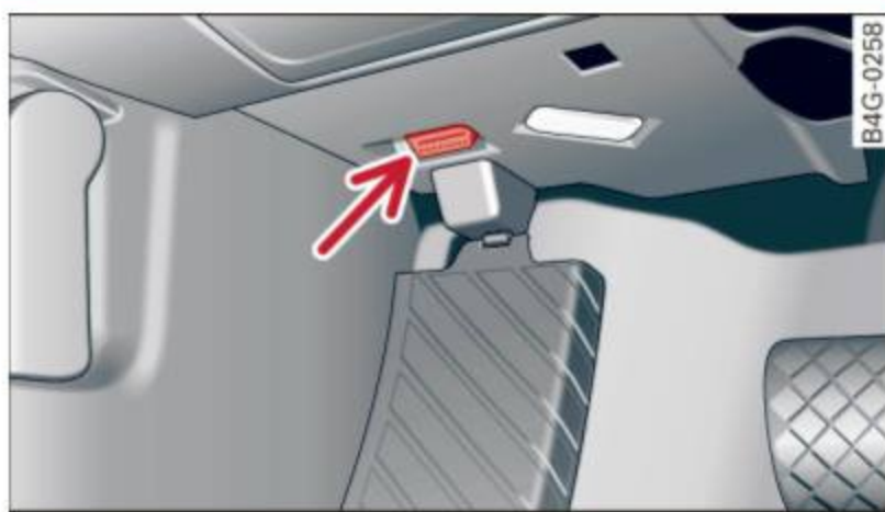
Fig. 16 Location of Data Link Connector (DLC)
