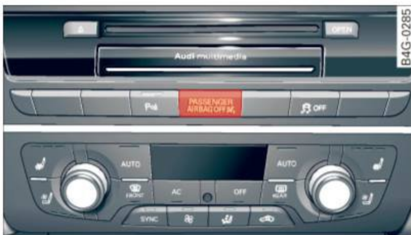
Fig. 163 Section from the instrument panel: PASSENGER AIR BAG OFF light
