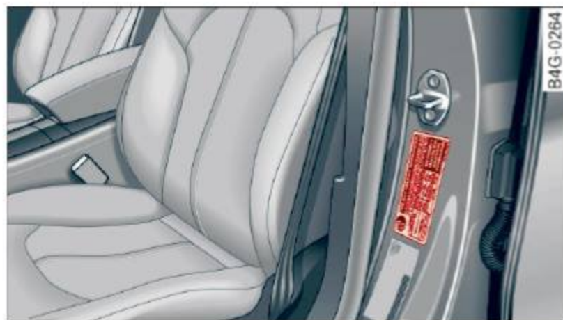
Fig. 196 Tire pressure label: located on driver's side B-pillar
