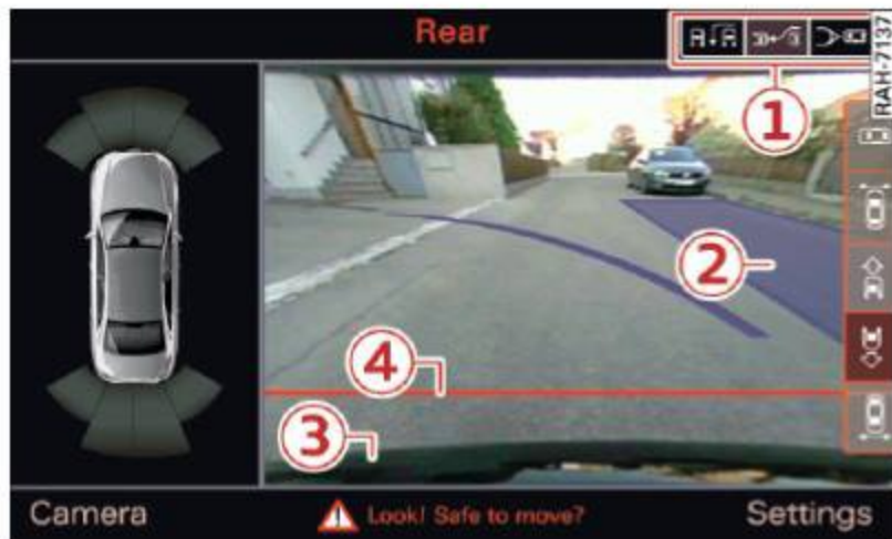
Fig. 142 Infotainment: blue surfaces aligned in the parking space
