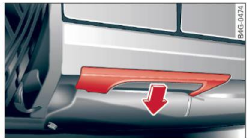
Fig. 211 Sill: removing the cover
