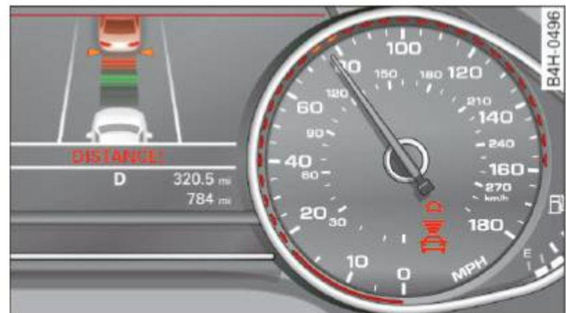
Fig. 95 Instrument cluster: request for driver intervention
