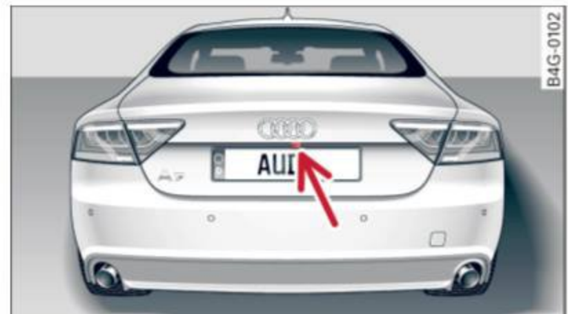
Fig. 127 Rear lid: Location of the rear view camera
