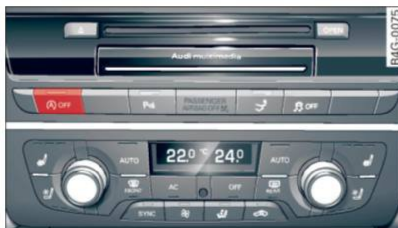
Fig. 83 Center console: Start-Stop-System button
