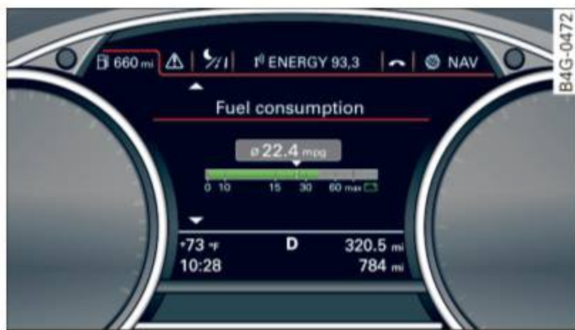
Fig. 10 Instrument cluster: fuel consumption
