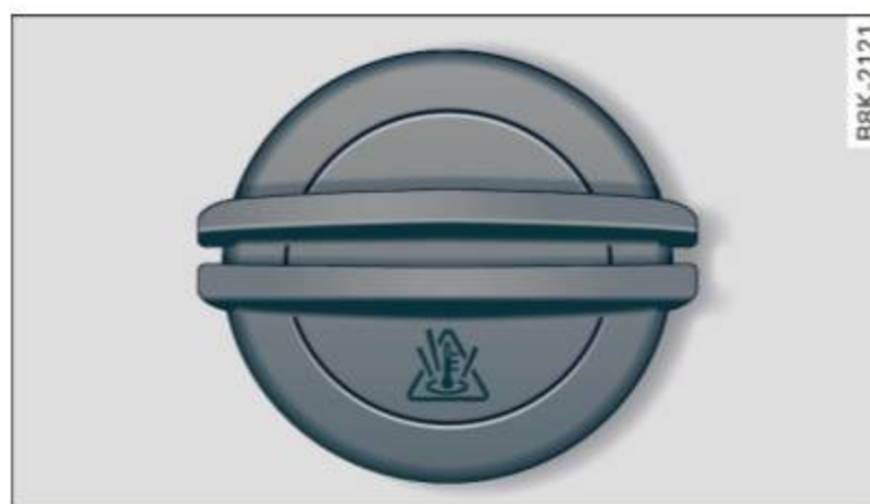
Fig. 192 Engine compartment: cover on the coolant expansion tank
