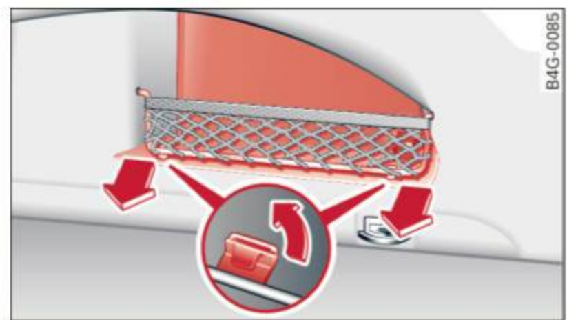
Fig. 185 Luggage compartment: opening the side trim
