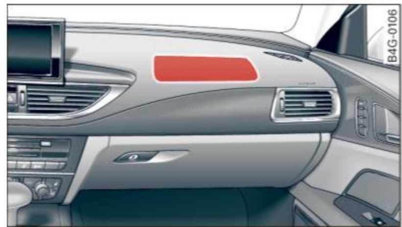
Fig. 161 Location of front passenger's airbag: in the instrument panel
