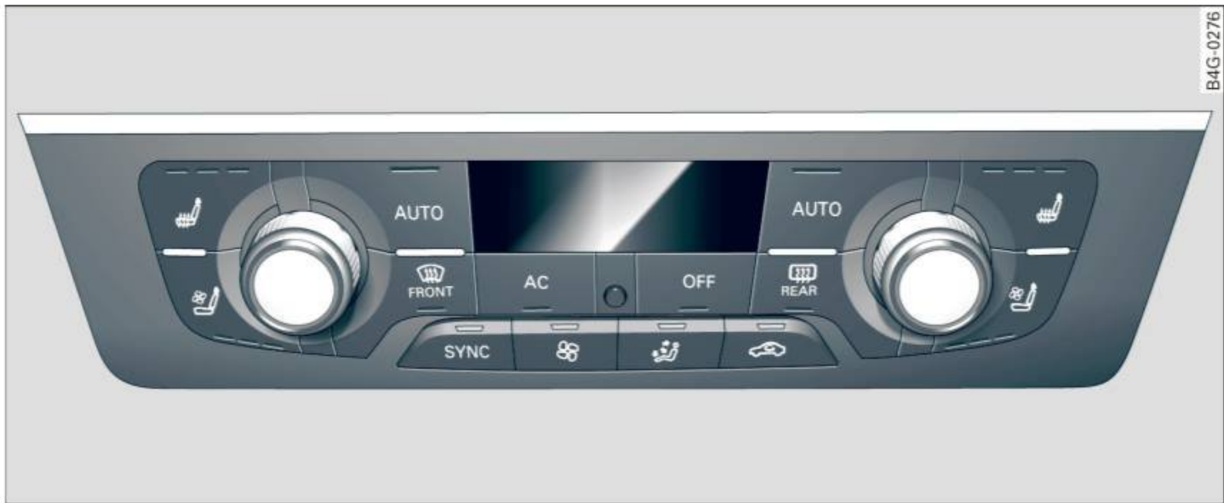
Fig. 73 Four-zone automatic climate control: controls
