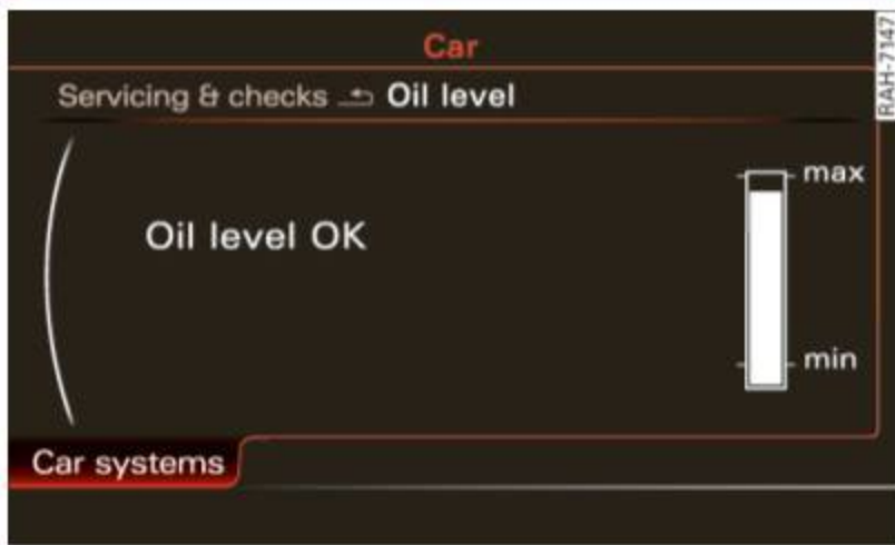
Fig. 190 Display: oil level indicator
