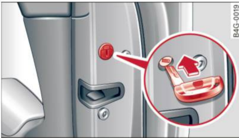
Fig. 25 Door: Emergency locking
