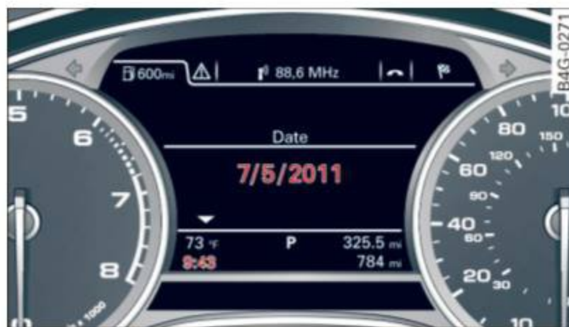
Fig. 12 Instrument cluster: clock and date
