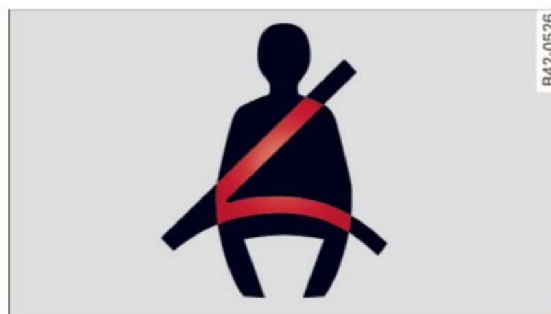
Fig. 149 Safety belt warning light in the instrument cluster - enlarged
