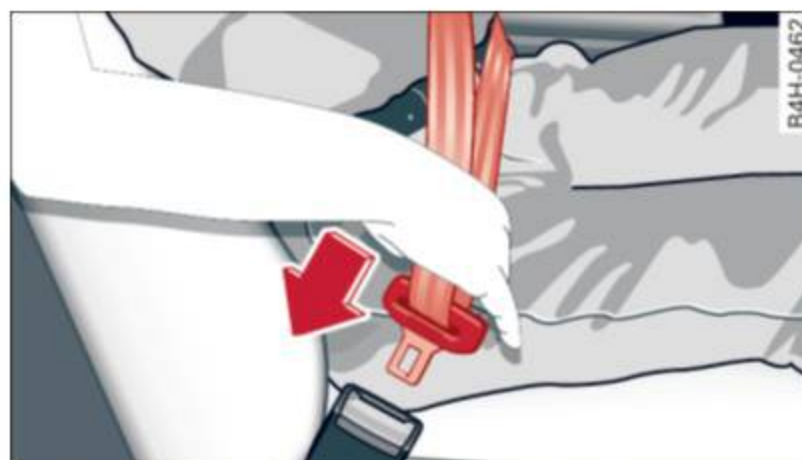
Fig. 155 Belt buckle and tongue on the driver's seat
