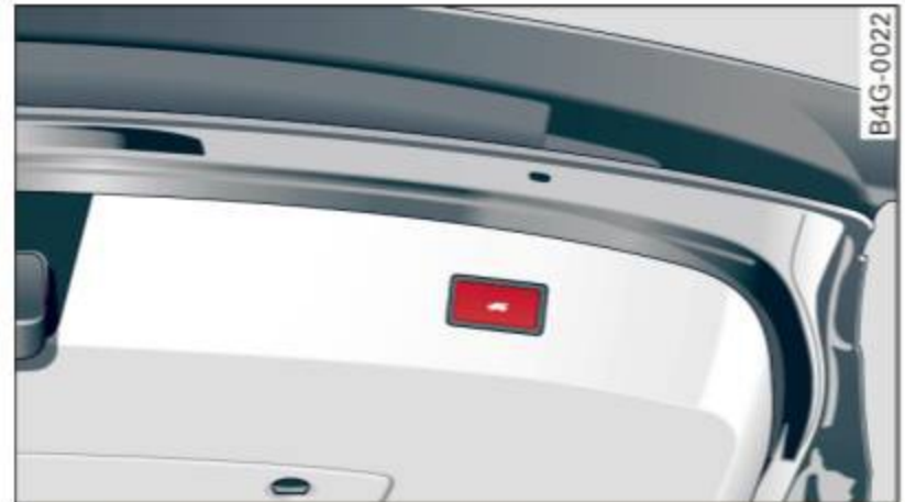
Fig. 27 Locking switch in the rear lid
