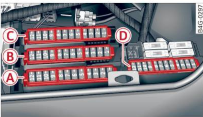
Fig. 217 Luggage compartment: fuse panel with plastic bracket
