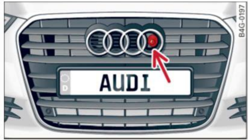
Fig. 112 Front of the vehicle: night vision assistant camera
