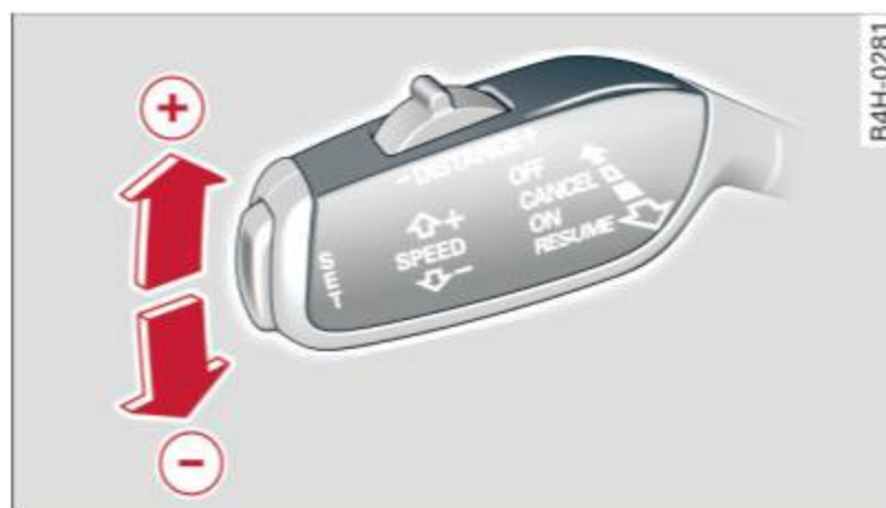
Fig. 92 Selector lever: changing the speed
