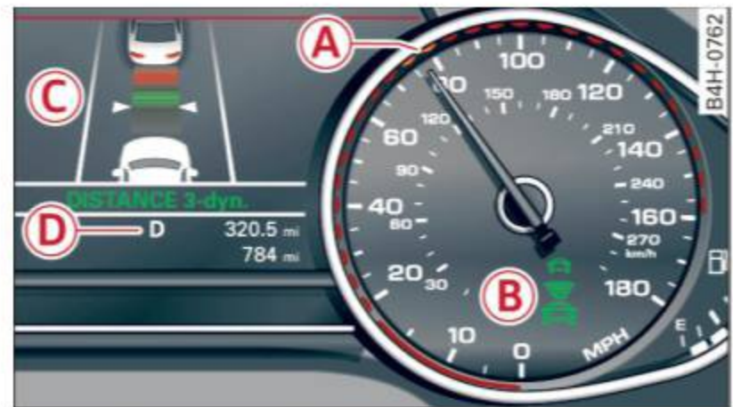
Fig. 91 Instrument cluster: adaptive cruise control
