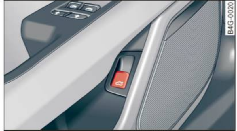
Fig. 26 Driver's door: Unlocking the rear lid
