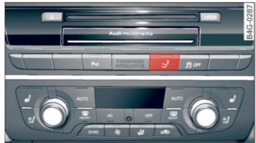
Fig. 182 Center console: Switch for rear spoiler
