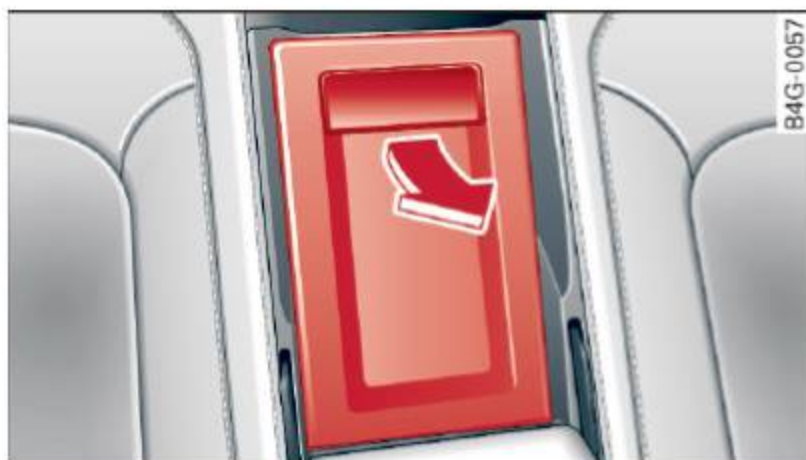
Fig. 69 Rear bench seat: opening the pass-through
