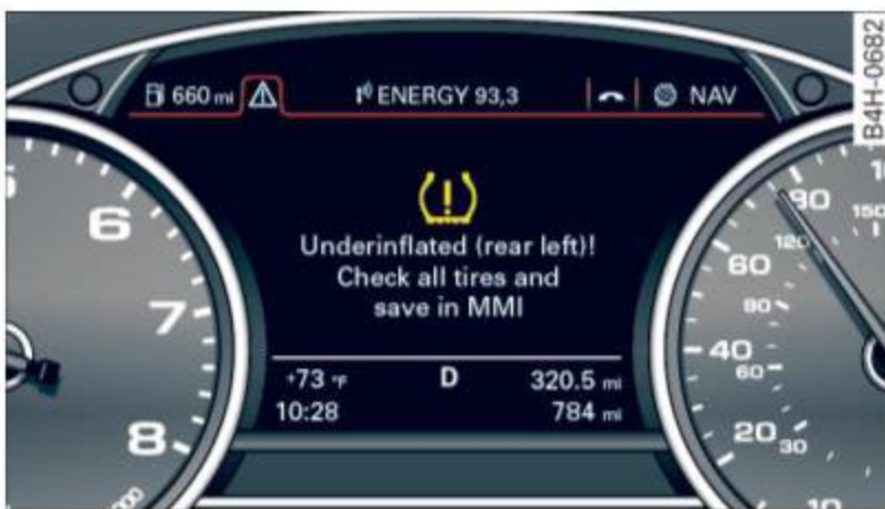
Fig. 201 Display: underinflation warning
