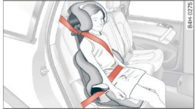
Fig. 174 Rear seat: child properly restrained in a booster seat
