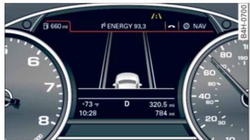
Fig. 100 Instrument cluster: Active lane assist is switched on but not ready to provide warnings
