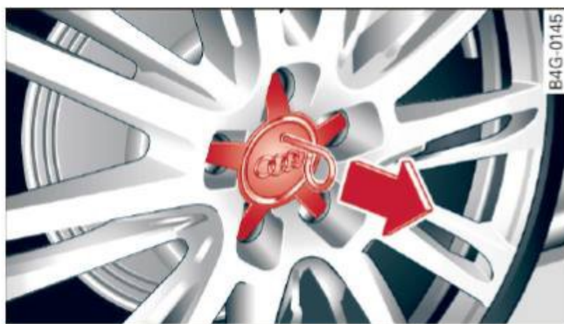
Fig. 206 Changing a wheel: Removing the wheel cover
