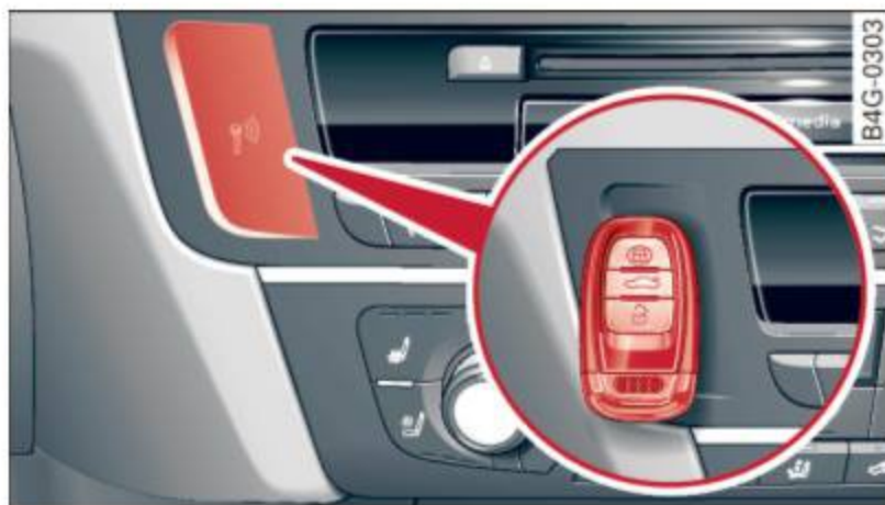
Fig. 79 Center console/master key: starting the engine if there is a malfunction
