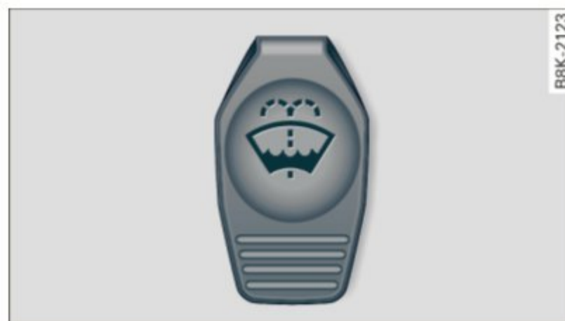
Fig. 195 Engine compartment: cover on the windshield and headlight* washer fluid reservoir
