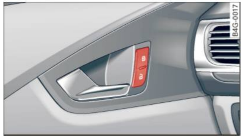
Fig. 23 Driver's door: power locking switch
