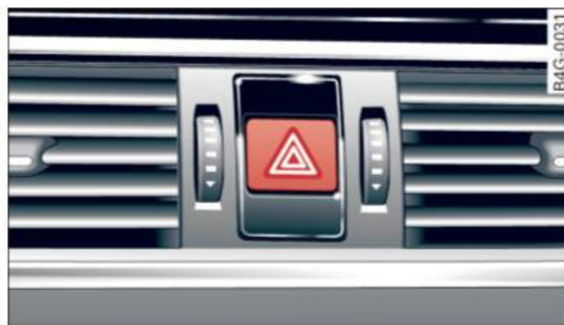
Fig. 34 Center console: emergency flasher switch
