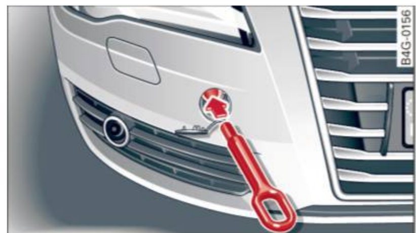
Fig. 221 Front bumper: installing the towing loop
