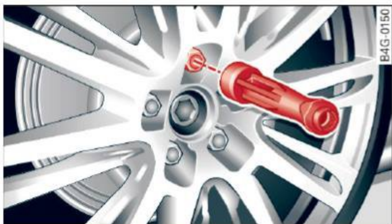
Fig. 212 Changing a wheel: using the screwdriver handle (with the blade removed) to turn the bolts
