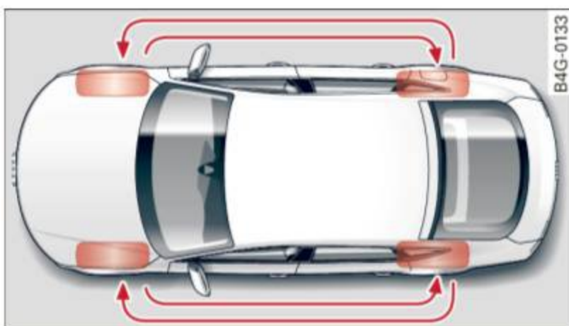
Fig. 199 Rotating tires for more even wear
