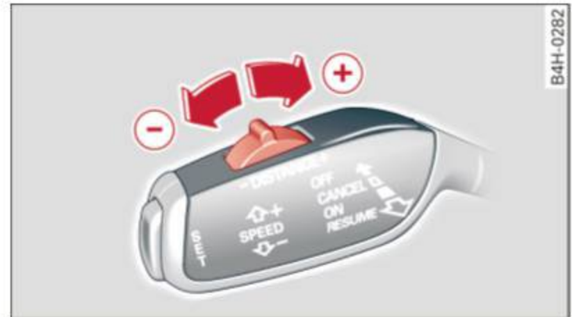
Fig. 94 Selector lever: setting the distance
