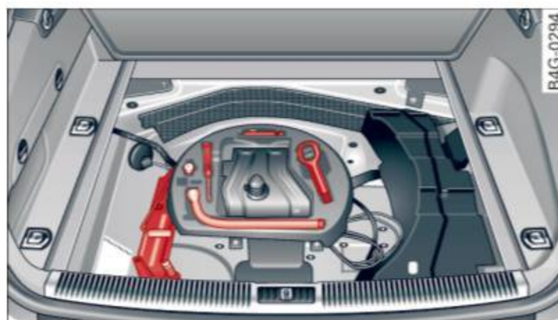
Fig. 205 Trunk lid: Vehicle tool kit
