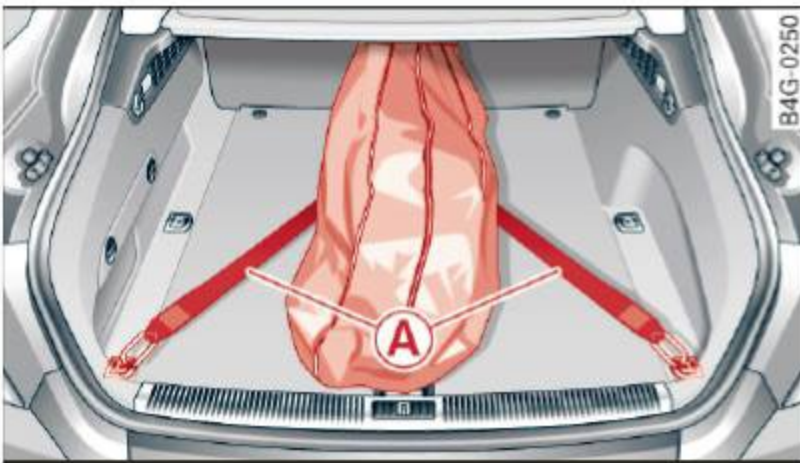
Fig. 70 Luggage compartment: Securing the bag
