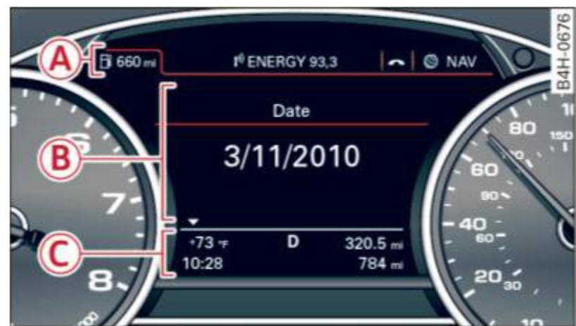
Fig. 4 Driver information system in the instrument cluster
