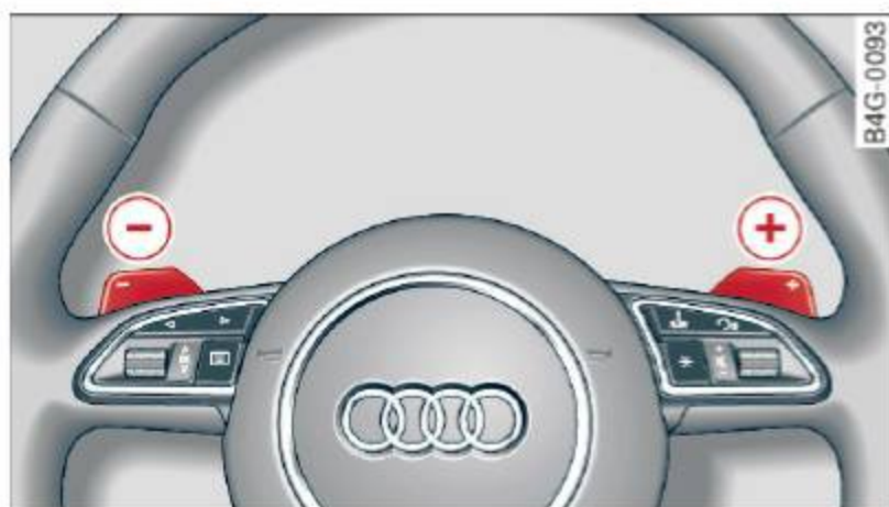
Fig. 119 Steering wheel: shifting the tiptronic manually using shift buttons*
