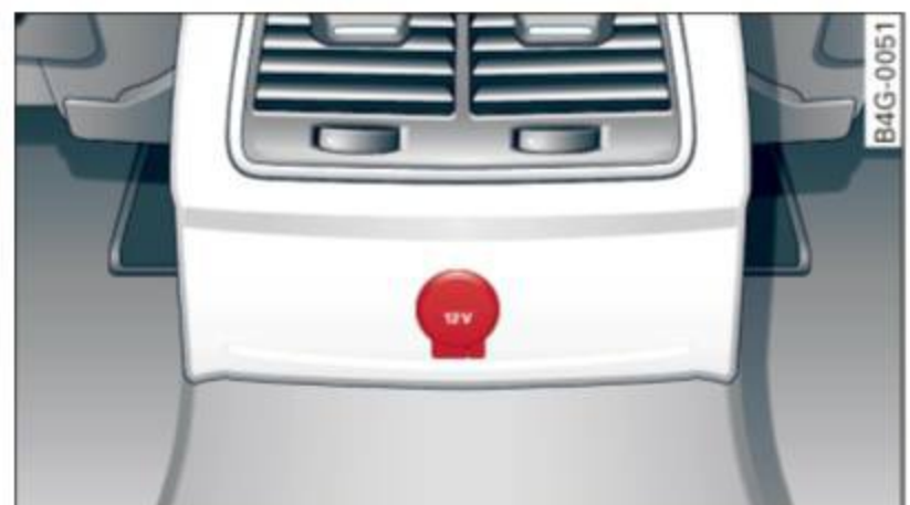
Fig. 56 Rear center console: 12-volt socket
