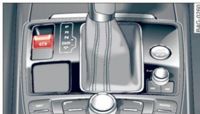
Fig. 80 Center console: Parking brake
