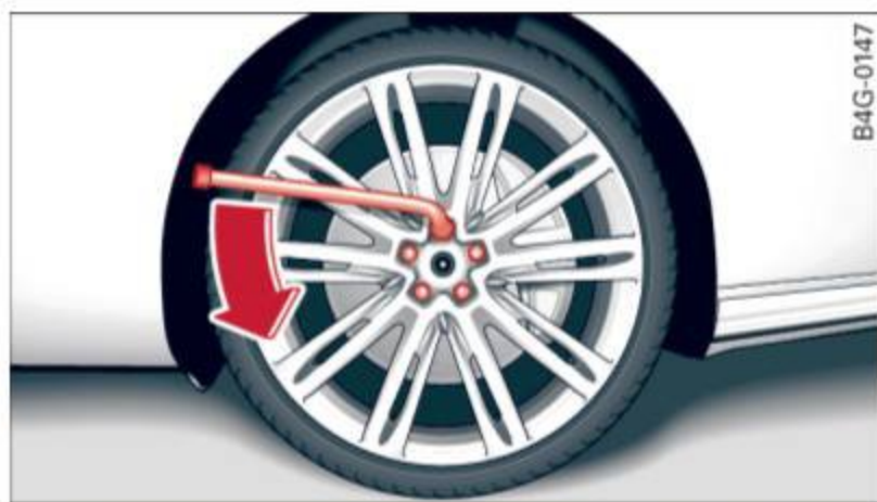
Fig. 208 Changing a wheel: loosening the wheel bolts
