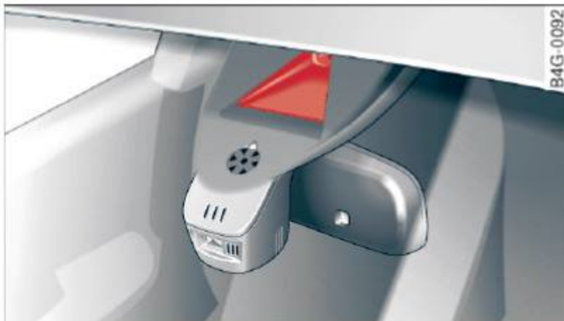
Fig. 98 Windshield: Active lane assist camera viewing window
