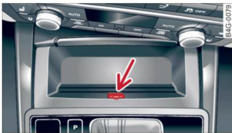
Fig. 120 Front center console: selector lever emergency release
