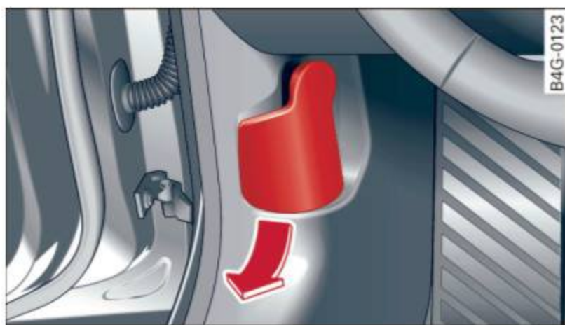
Fig. 187 Driver footwell: release lever
