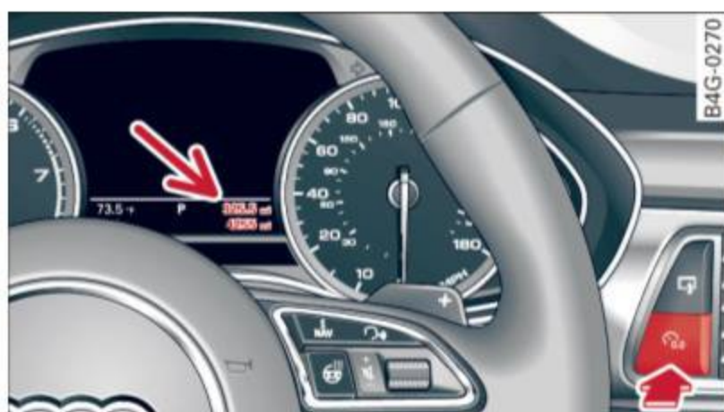
Fig. 11 Instrument cluster: Odometer and reset button
