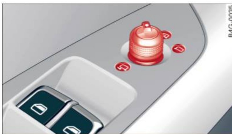
Fig. 43 Forward section of driver's armrest: power mirror controls
