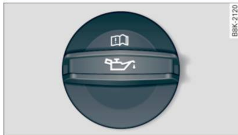
Fig. 191 Engine compartment: cover on the engine oil filler neck
