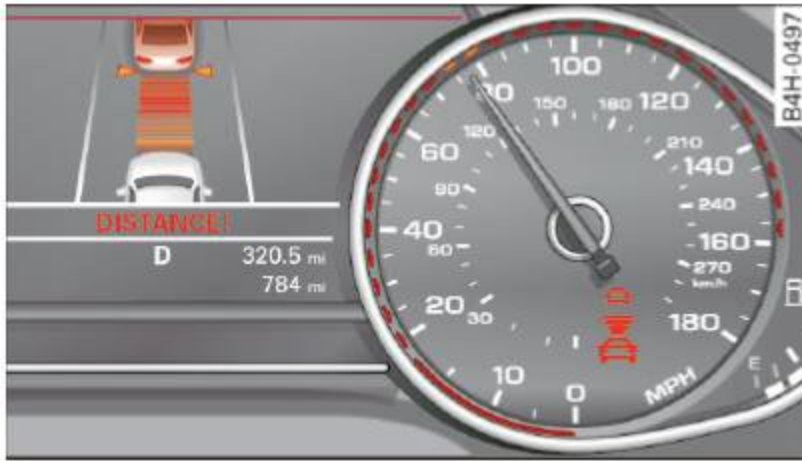
Fig. 96 Instrument cluster: approach warning
