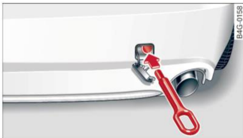
Fig. 223 Rear bumper: screwing in towing loop
