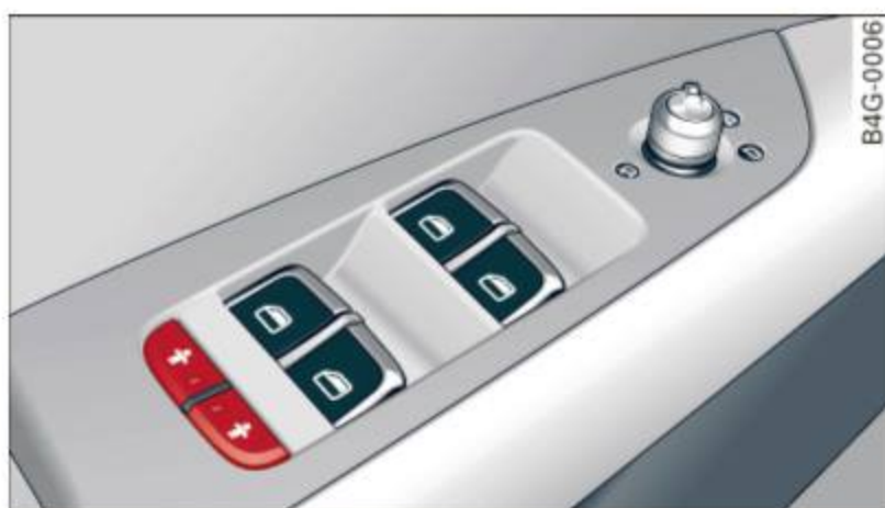
Fig. 29 Section from driver's door: child safety lock buttons
