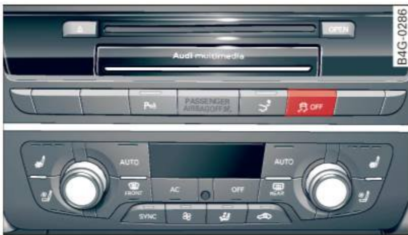
Fig. 181 Center console with ESC OFF button
