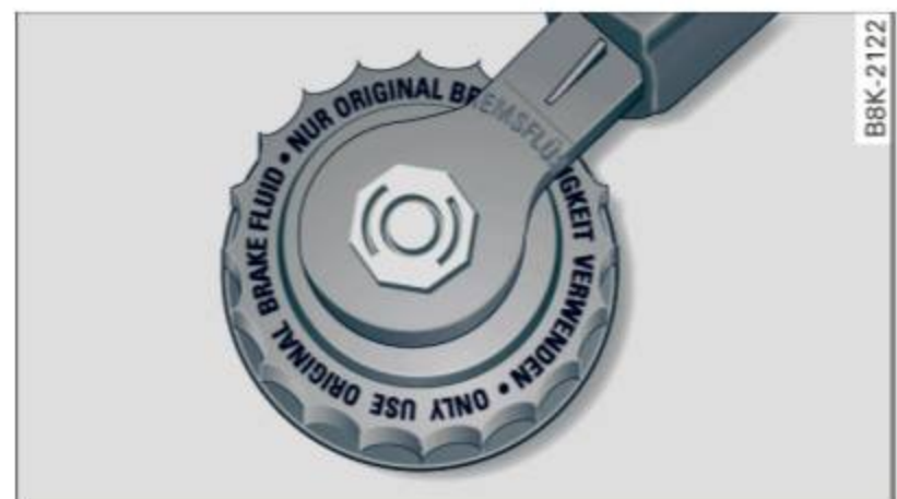
Fig. 193 Engine compartment: cover on the brake fluid reservoir
