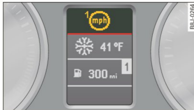
Fig. 23 Display: speed warning system
