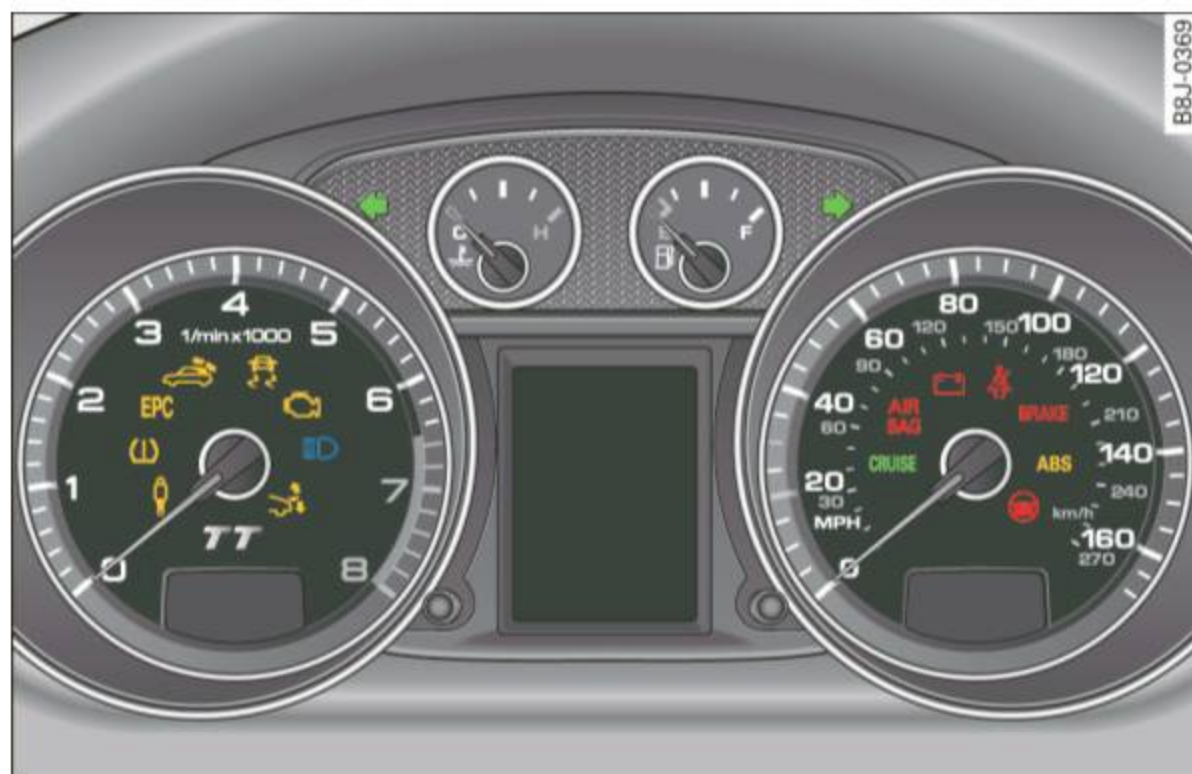
Fig. 6 Instrument cluster with warning/indicator lights
