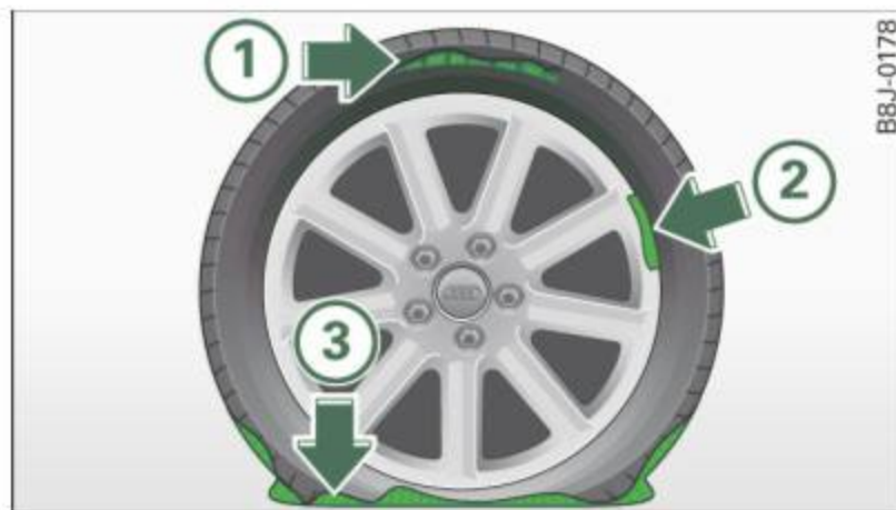
Fig. 167 Tire damage for which the Tire Mobility System is not suited
