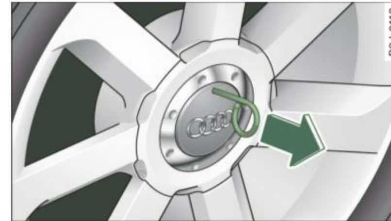
Fig. 171 Wheel change: removing the wheel cover
