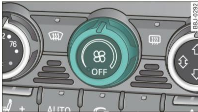
Fig. 95 Rotary knob to switch air conditioning on and off and to regulate fan speed
