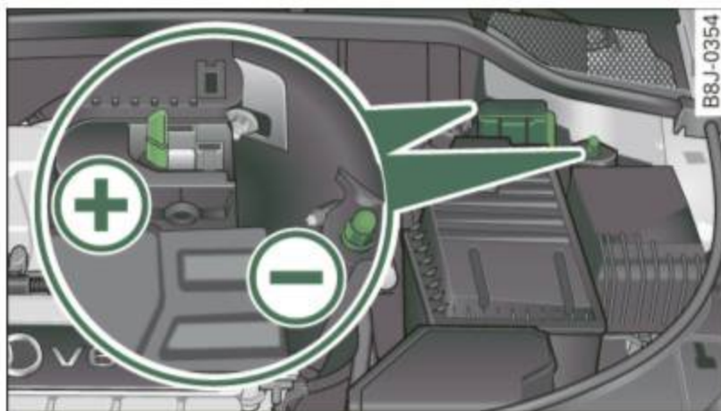
Fig. 182 For jump starting or charging the battery, there is a jump start connection on the left side of the engine compartment.
