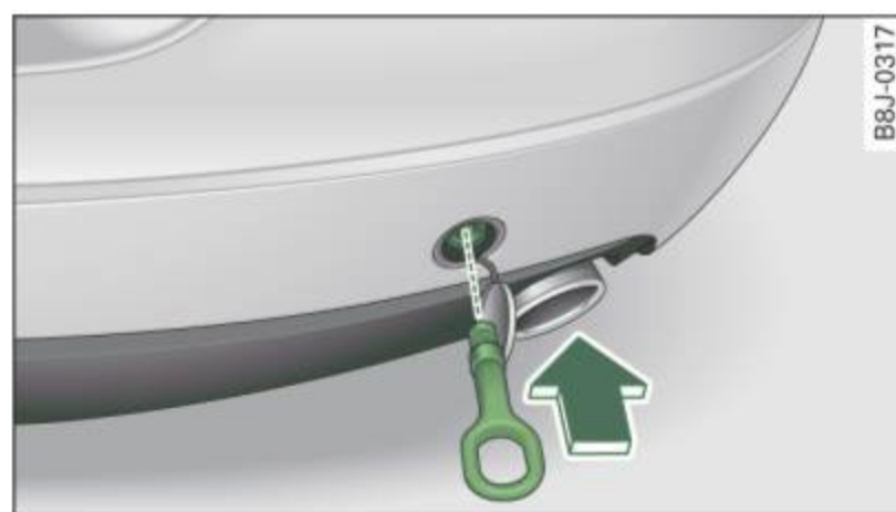
Fig. 186 Rear bumper: screwing in the towing loop
