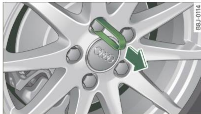
Fig. 172 Wheel change: removing the wheel bolt caps
