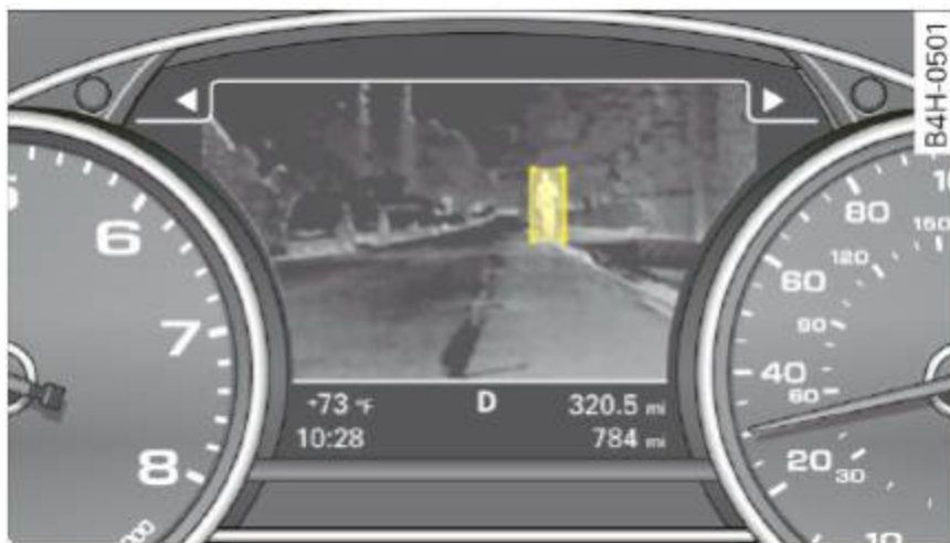
Fig. 110 Instrument cluster: Yellow pedestrian highlighting
