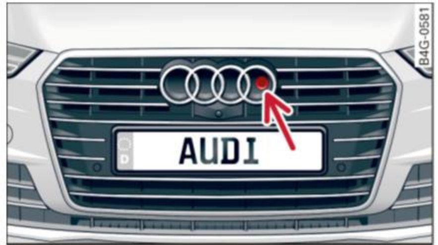
Fig. 114 Front of the vehicle: night vision camera
