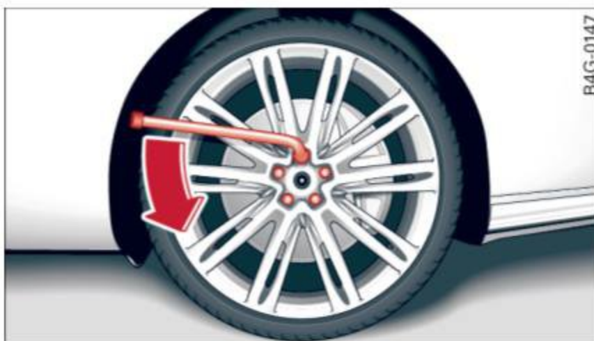
Fig. 205 Changing a wheel: loosening the wheel bolts
