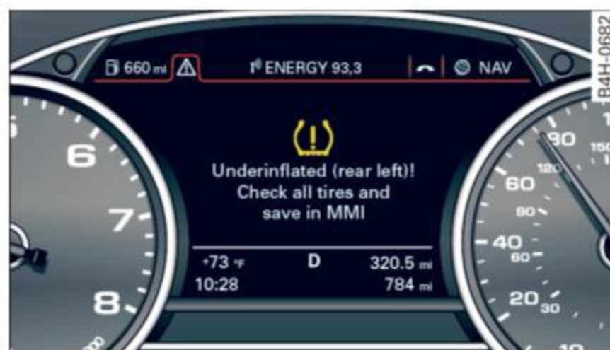
Fig. 199 Instrument cluster: indicator light with message
