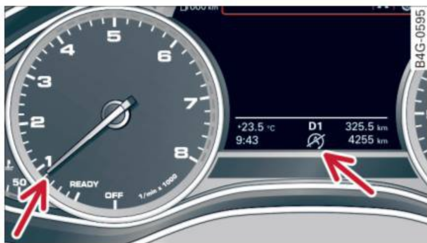
Fig. 85 Instrument cluster: Engine stop temporarily unavailable
