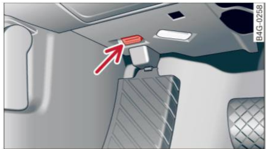
Fig. 16 Location of Data Link Connector (DLC)
