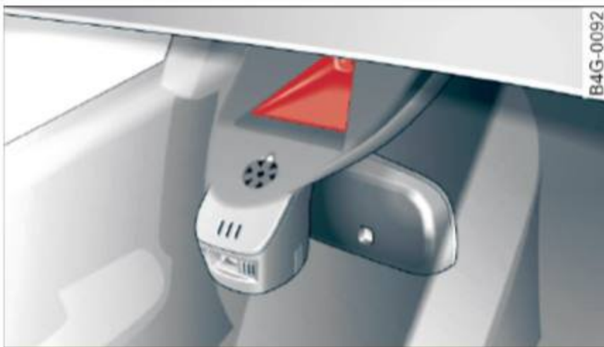
Fig. 101 Windshield: camera window for active lane assist
