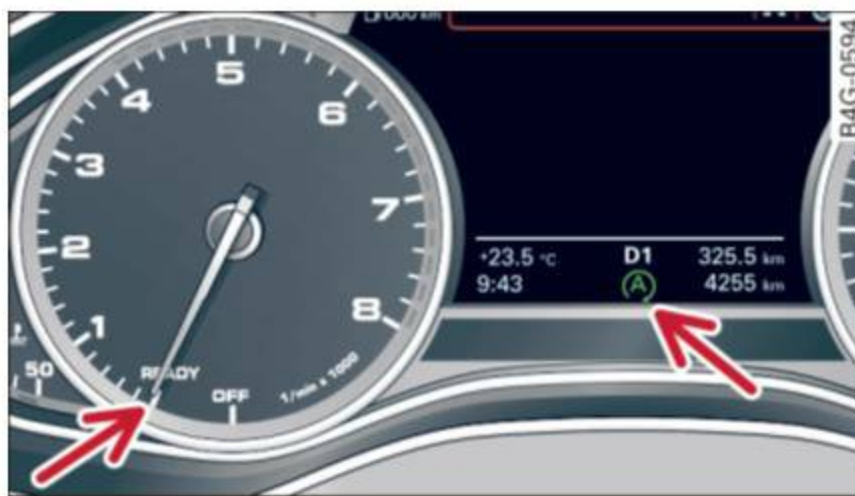
Fig. 84 Instrument cluster: engine stopped (stop phase)
