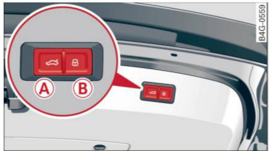
Fig. 27 Luggage compartment lid: (A) closing button, (B) lock button (vehicles with convenience key*)
