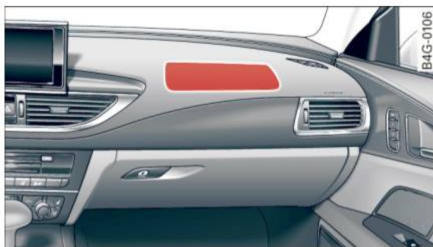
Fig. 158 Location of front passenger's airbag: in the instrument panel
