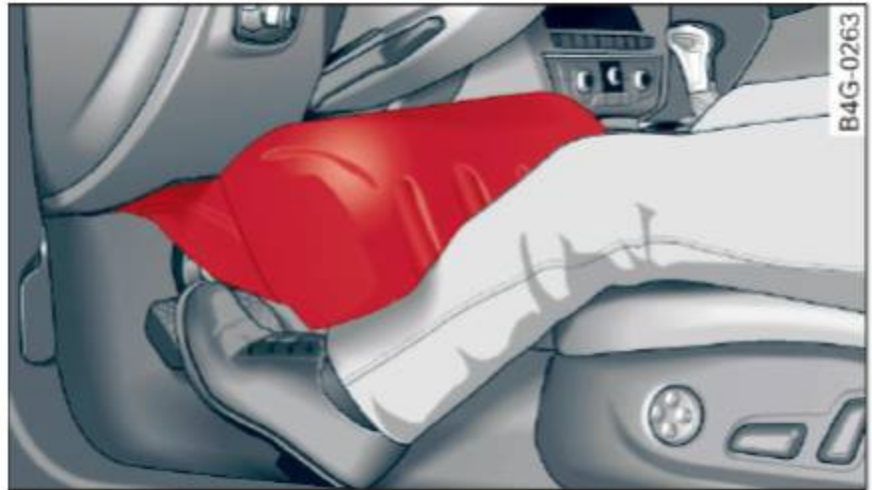
Fig. 162 Inflated airbags protecting in a frontal collision
