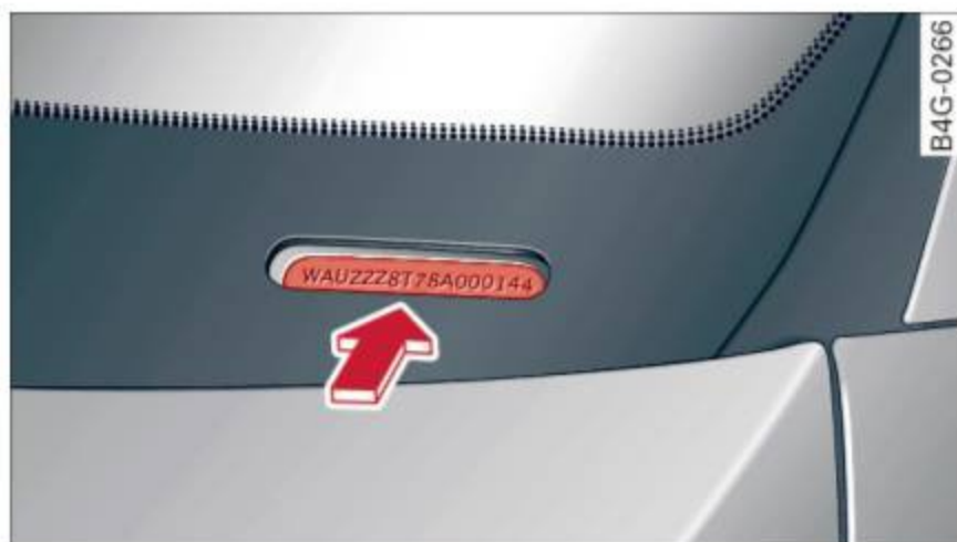
Fig. 224 Vehicle Identification Number (VIN) plate: location on driver's side dash panel
