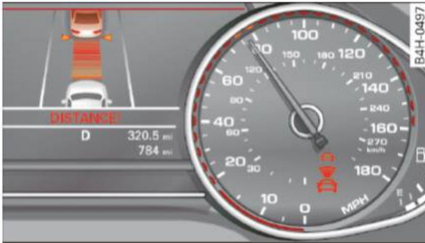
Fig. 99 Instrument cluster: approach warning
