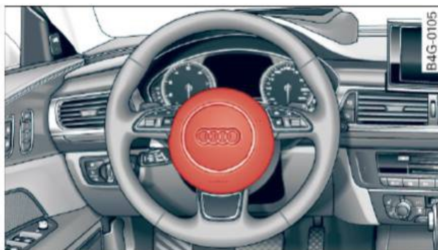
Fig. 157 Location of driver airbag: in steering wheel
