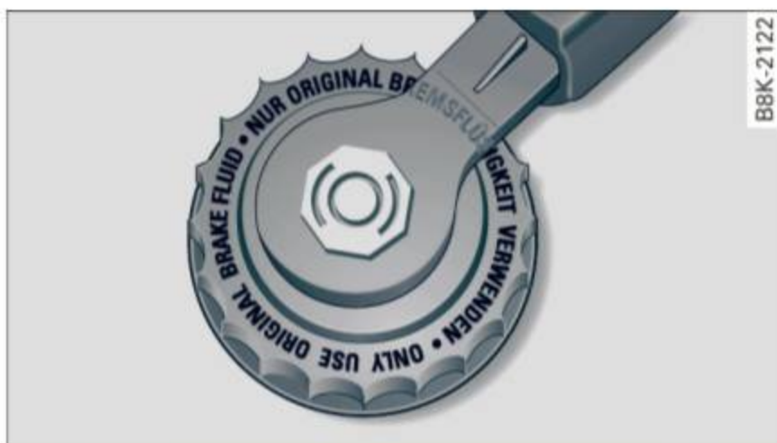
Fig. 192 Engine compartment: cover on the brake fluid reservoir
