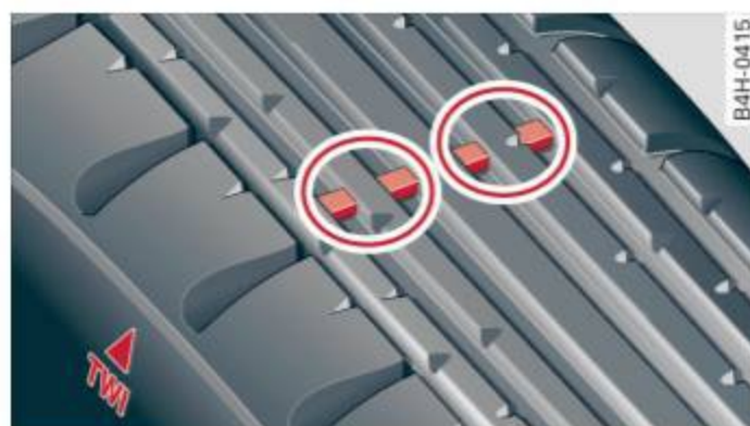
Fig. 196 Tire profile: Treadwear indicator
