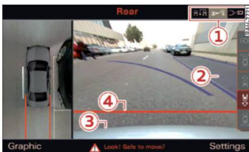
Fig. 141 Infotainment: blue surface aligned with parking spot
