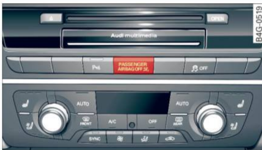
Fig. 160 Section from the instrument panel: PASSENGER AIR BAG OFF light
