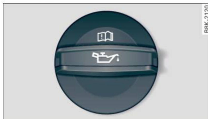
Fig. 190 Engine compartment: cover on the engine oil filler neck
