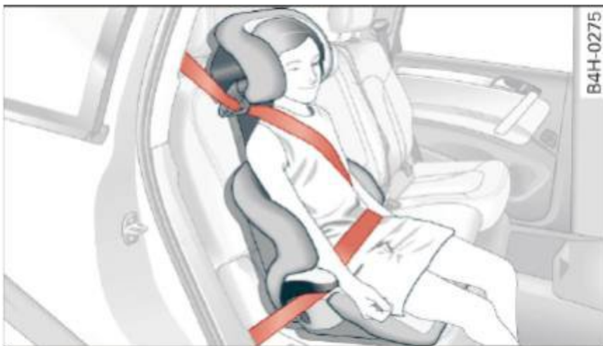
Fig. 171 Rear seat: child properly restrained in a booster seat
