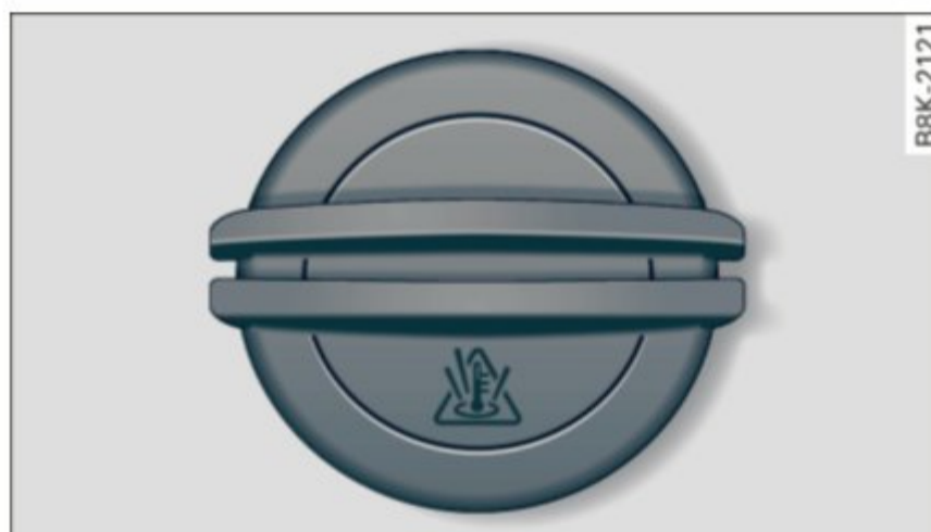
Fig. 191 Engine compartment: cover on the coolant expansion tank
