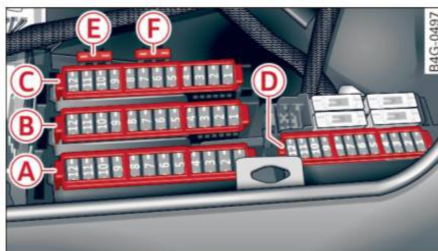
Fig. 214 Luggage compartment: fuse panel with plastic clip
