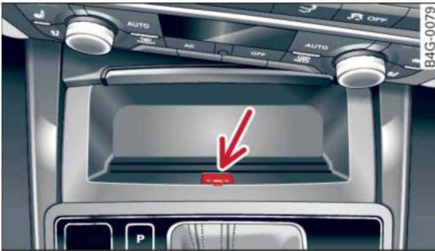
Fig. 120 Front center console: Selector lever emergency release
