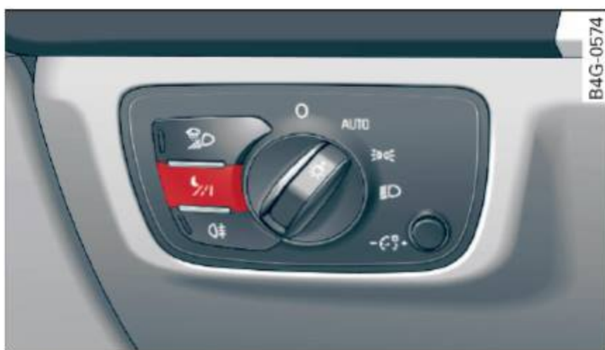
Fig. 115 Area around the light switch: night vision assist button
