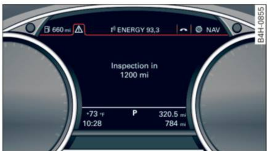
Fig. 13 Instrument cluster display: service interval display (example)
