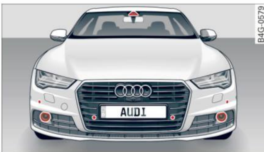
Fig. 89 Front of the vehicle: sensors and video camera
