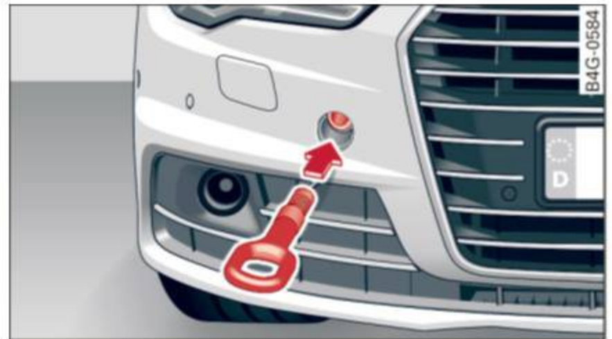
Fig. 218 Front bumper: installing the towing loop
