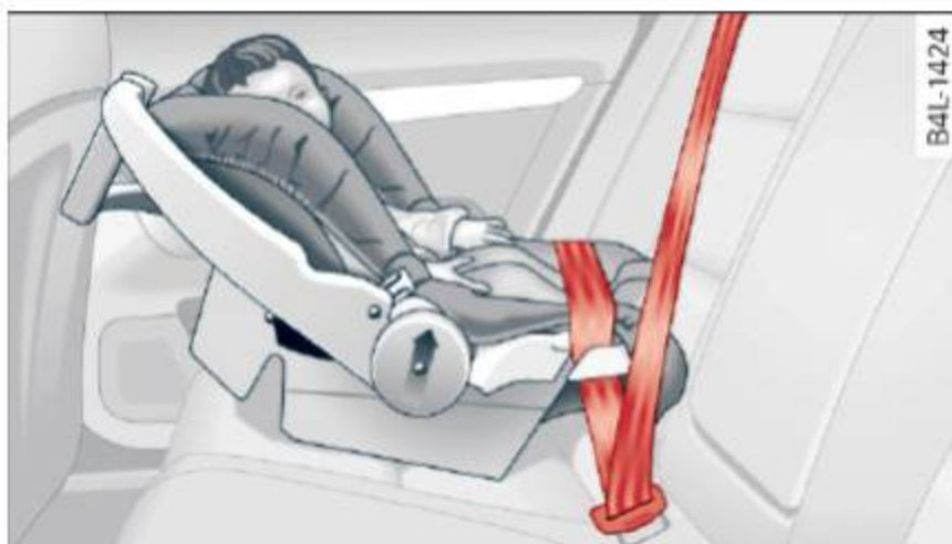
Fig. 168 Schematic overview: rearward-facing infant seat, properly installed on the rear seat
