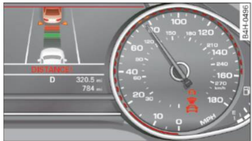
Fig. 98 Instrument cluster: request for driver intervention
