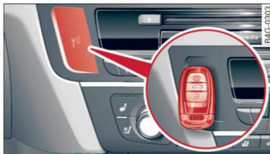
Fig. 82 Center console/master key: starting the engine when there is a malfunction
