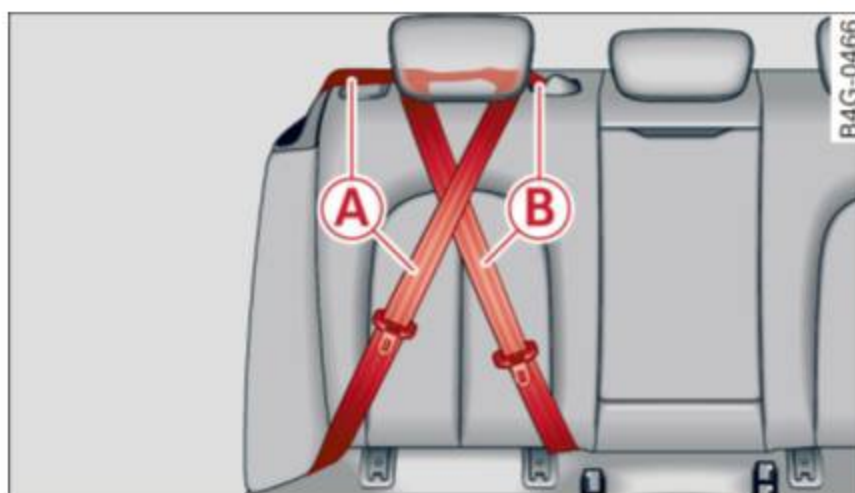
Fig. 167 Schematic overview: keep unused safety belts away from children in child safety seats. A - outer rear safety belt, B - center rear safety belt*
