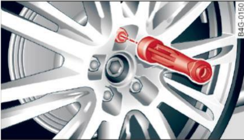
Fig. 209 Changing a wheel: using the screwdriver handle (with the blade removed) to turn the bolts
