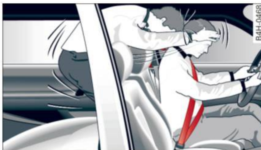
Fig. 150 A rear passenger not wearing a safety belt will fly forward and strike the driver
