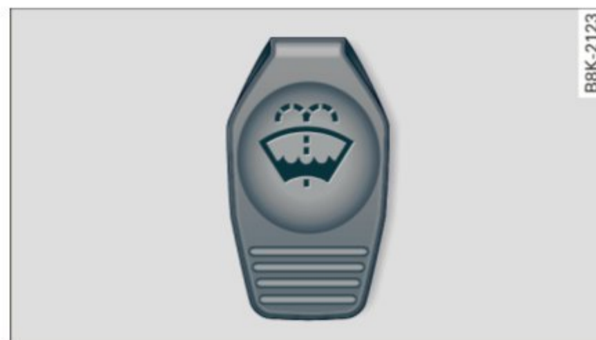
Fig. 194 Engine compartment: cover on the windshield and headlight* washer fluid reservoir
