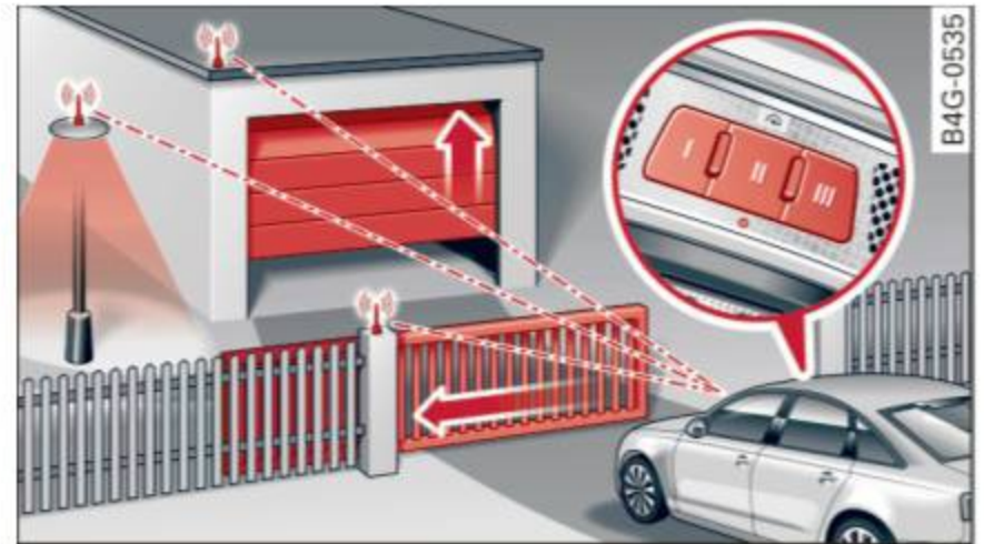
Fig. 33 Garage door opener: examples of using with different systems
