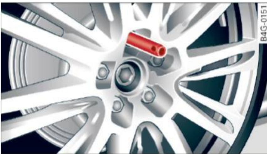
Fig. 210 Changing a wheel: alignment pin inside the top hole
