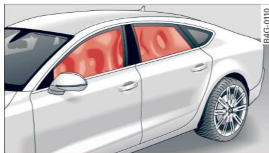
Fig. 166 Illustration of principle: Inflated side curtain airbags on the left side
