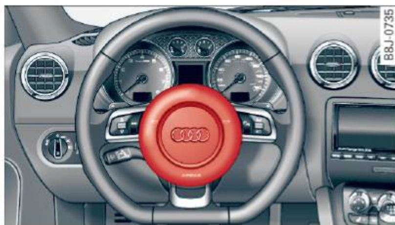
Fig. 112 Location of driver airbag: in steering wheel
