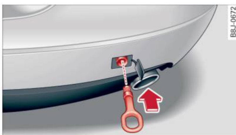
Fig. 184 Rear bumper: screwing in the towing loop
