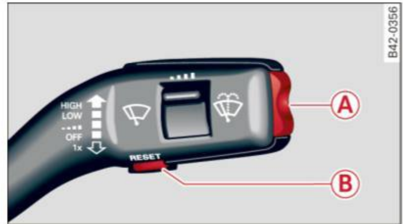
Fig. 25 Wiper lever: Trip computer controls
