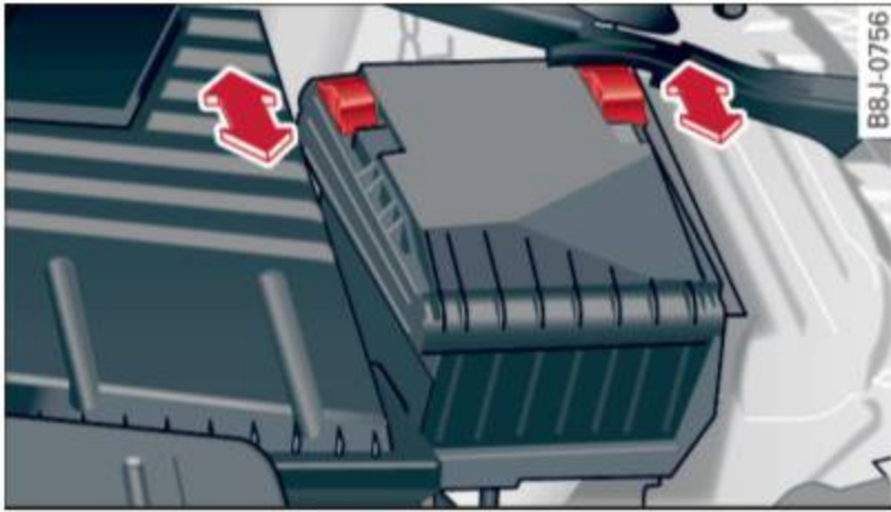
Fig. 174 Left side of engine compartment: fuse cover
