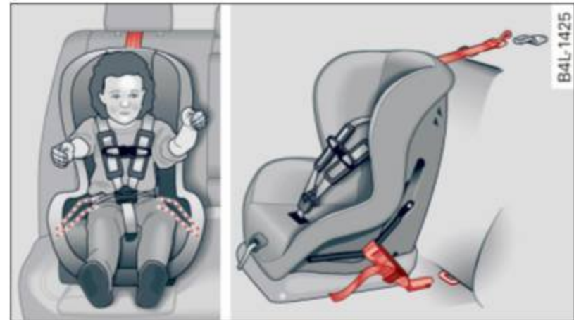
Fig. 121 Schematic overview: installation of the attachments applicable to a LATCH seat
