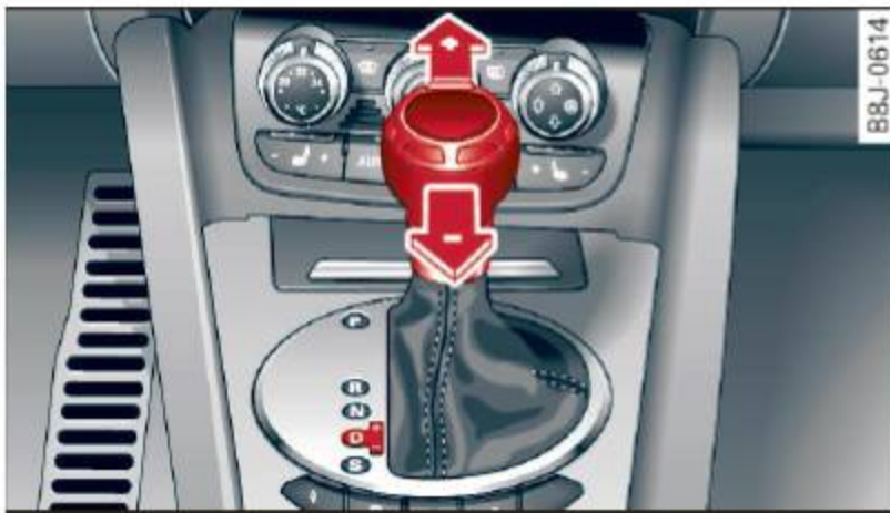
Fig. 90 Center console: Manual shifting (tiptronic)
