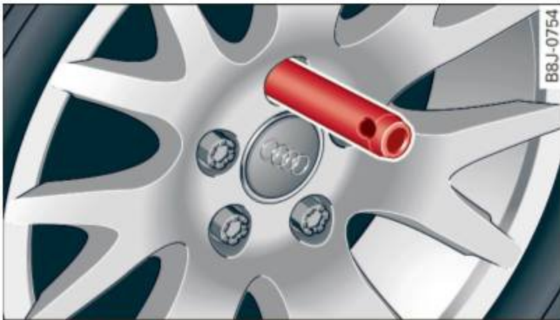
Fig. 172 Wheel change: alignment pin inside the top hole
