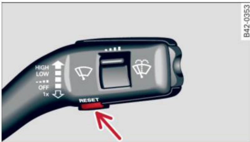
Fig. 7 Wiper lever: controls for the menu display
