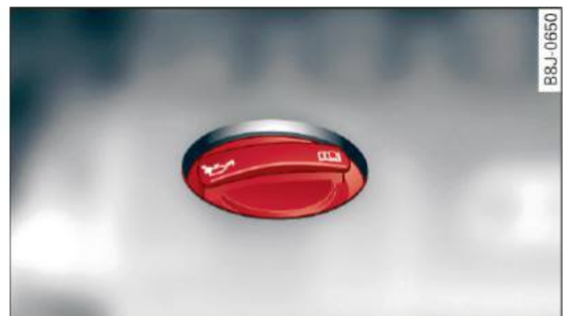
Fig. 144 Engine compartment: Oil filler cap location
