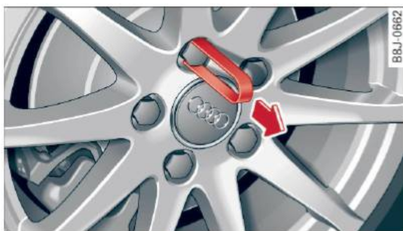
Fig. 167 Wheel change: removing the wheel bolt caps
