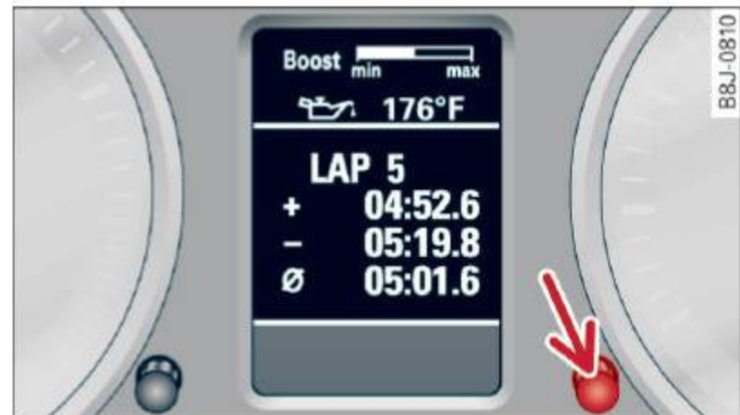
Fig. 20 Display: boost and engine oil temperature indicator
