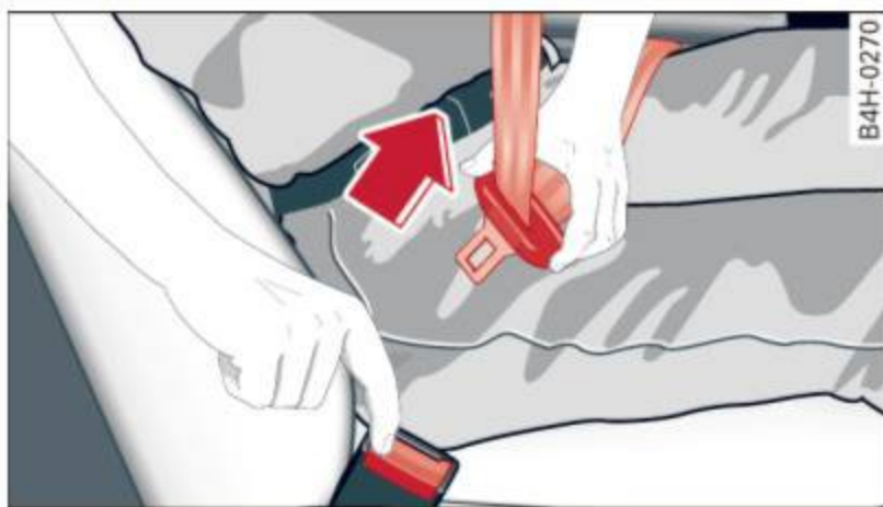
Fig. 111 Releasing the tongue from the buckle
