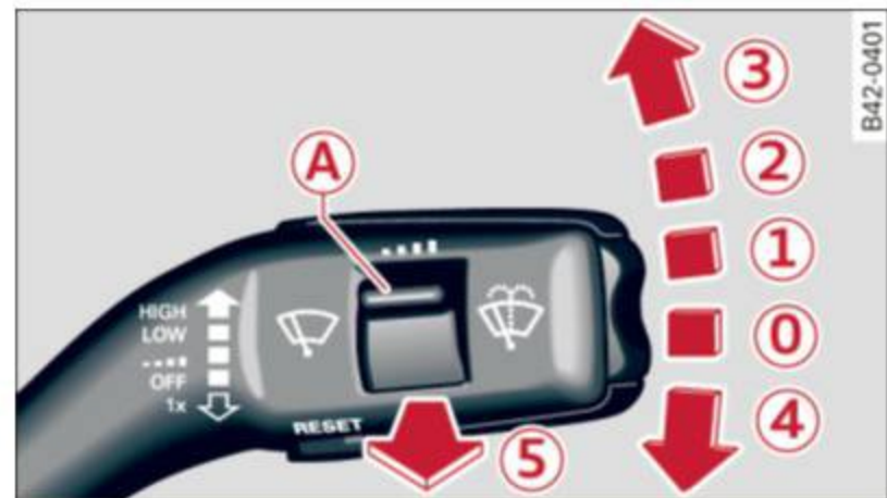
Fig. 55 Wiper lever: windshield wiper lever positions
