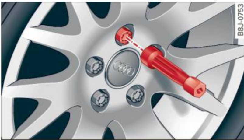
Fig. 171 Wheel change: using the screwdriver handle (with the blade removed) to turn the bolts
