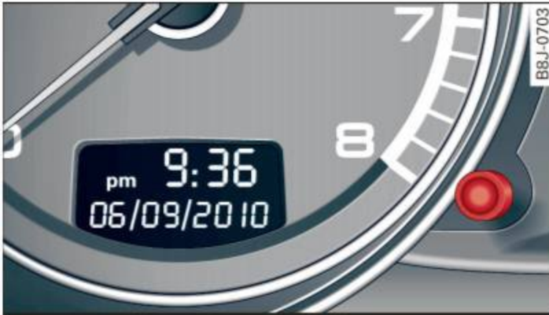
Fig. 24 Section of instrument cluster: Set/Check button
