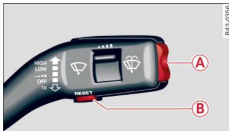
Fig. 12 Wiper lever: Controls for the menu display
