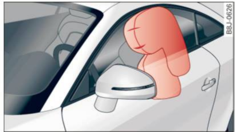
Fig. 119 Inflated side airbags on left side of vehicle
