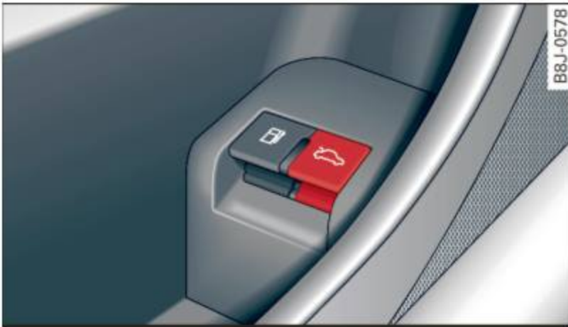
Fig. 36 Driver's door: remote rear lid release
