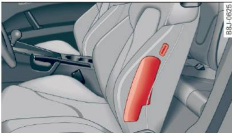
Fig. 118 Side airbag location in the driver's seat
