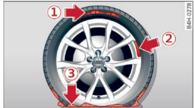
Fig. 162 Tire damage for which the Tire Mobility System is not suited
