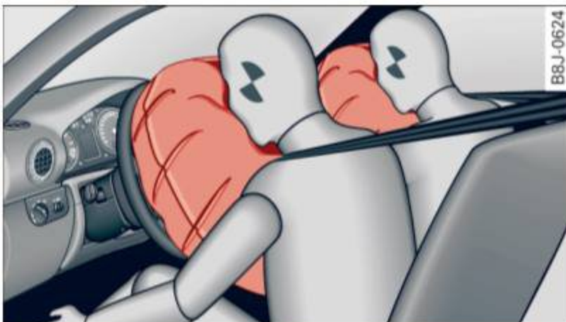
Fig. 114 Inflated front airbags
