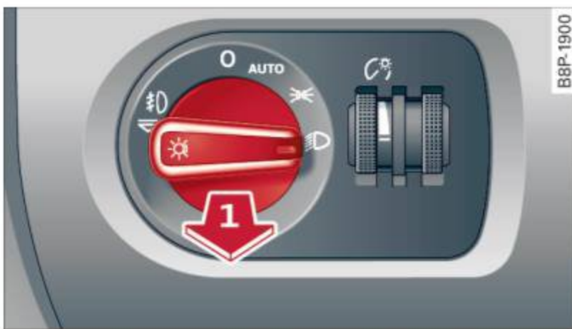
Fig. 47 Fog light activation: light switch position on vehicles WITHOUT sensor light
