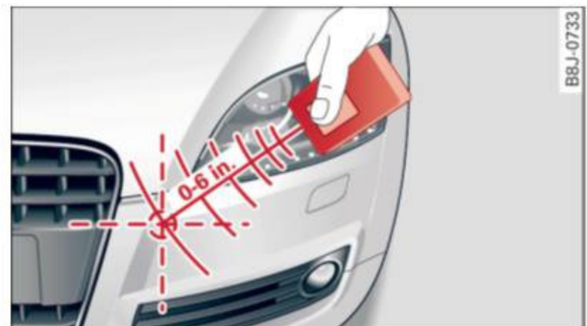
Fig. 96 Front bumper, driver side: location of transmitter unit
