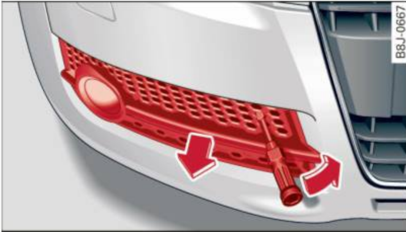
Fig. 179 Front bumper: removing the grill
