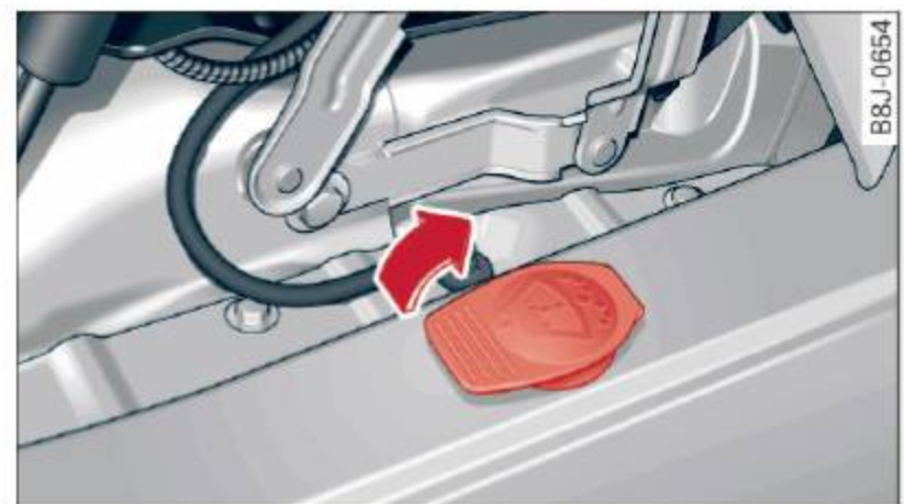
Fig. 149 Fender, left: Windshield washer fluid reservoir
