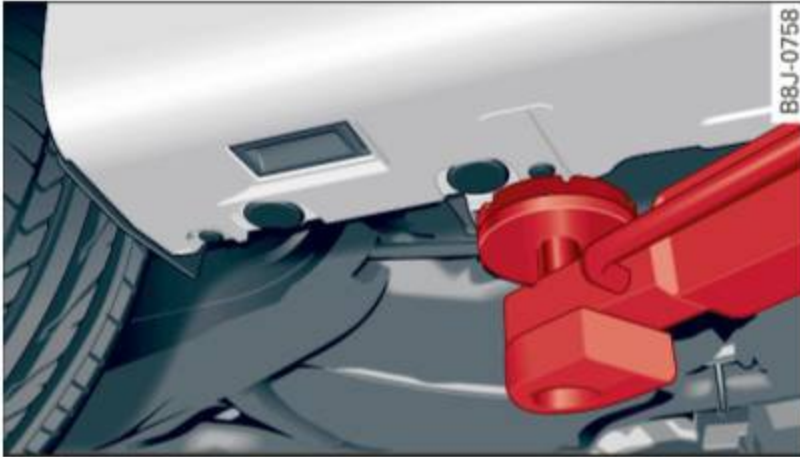
Fig. 186 Rear lifting point (right side)
