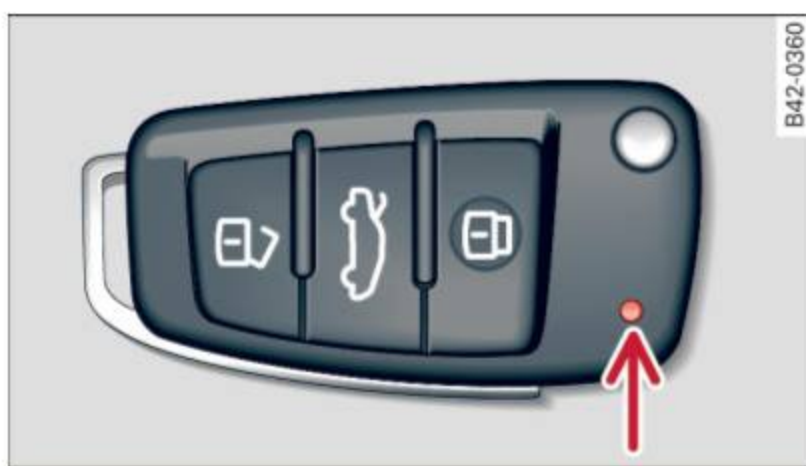
Fig. 29 Check light in the master key
