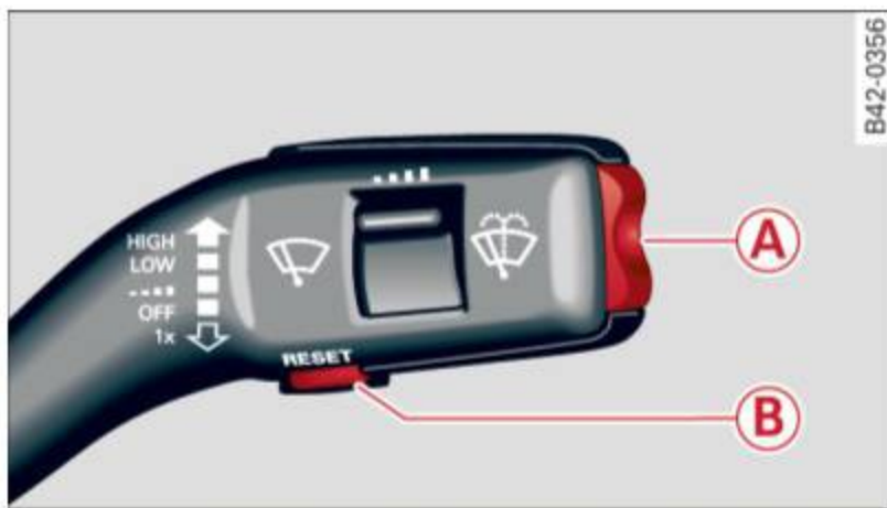
Fig. 10 Wiper arm/wiper lever: controls for the trip computer
