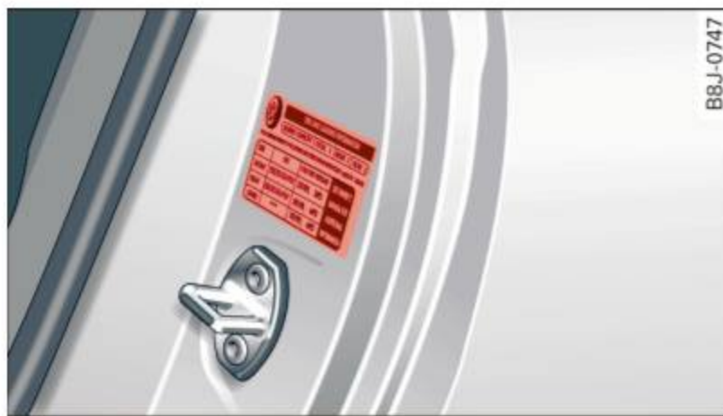
Fig. 150 Tire pressure label: located on driver's side B-pillar
