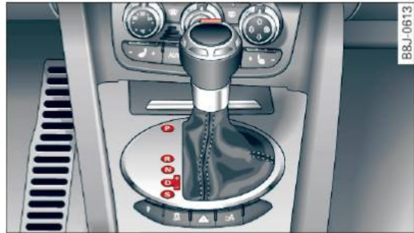
Fig. 89 Section from center console: Selector lever with release button
