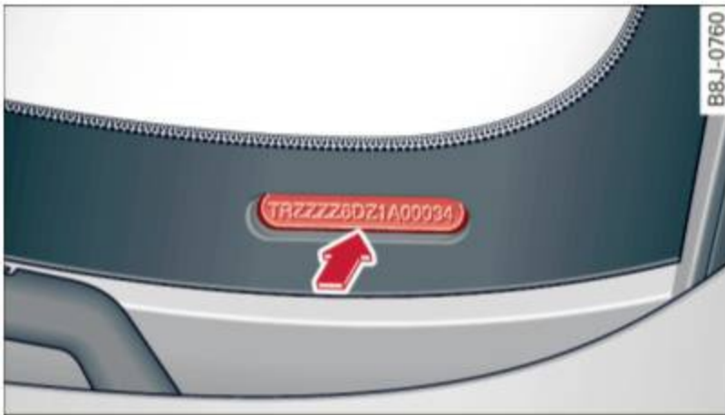
Fig. 188 Vehicle Identification Number (VIN) plate: location on driver's side dash panel
