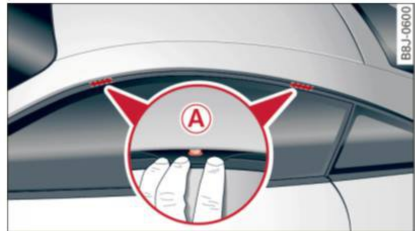
Fig. 71 Mounting locations for roof rack
