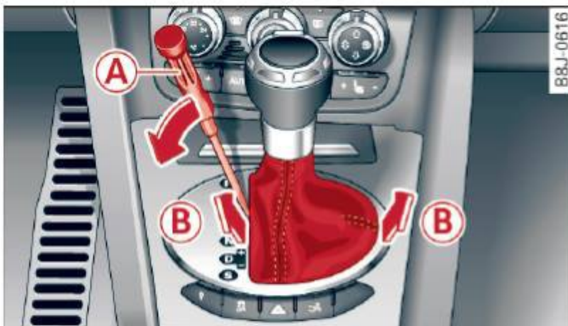
Fig. 93 Selector lever: Removing the selector lever boot
