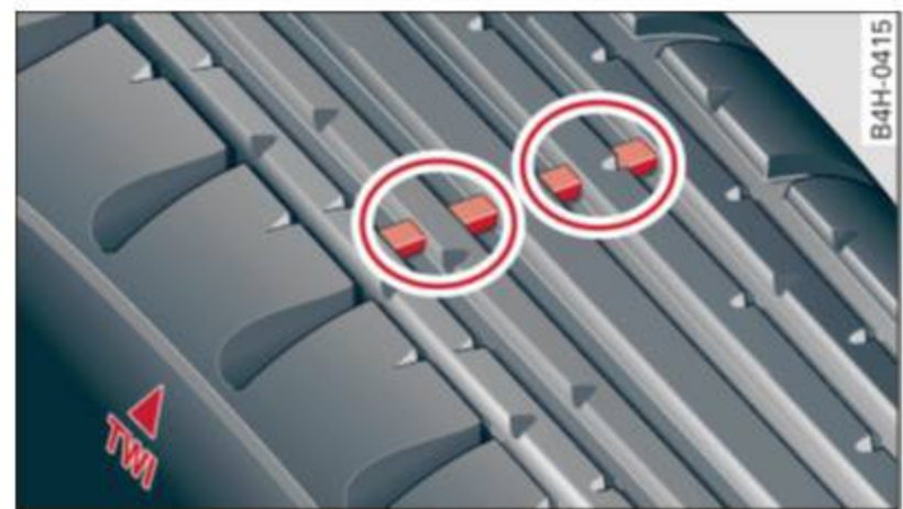
Fig. 152 Tire tread: tread wear indicators (TWI)
