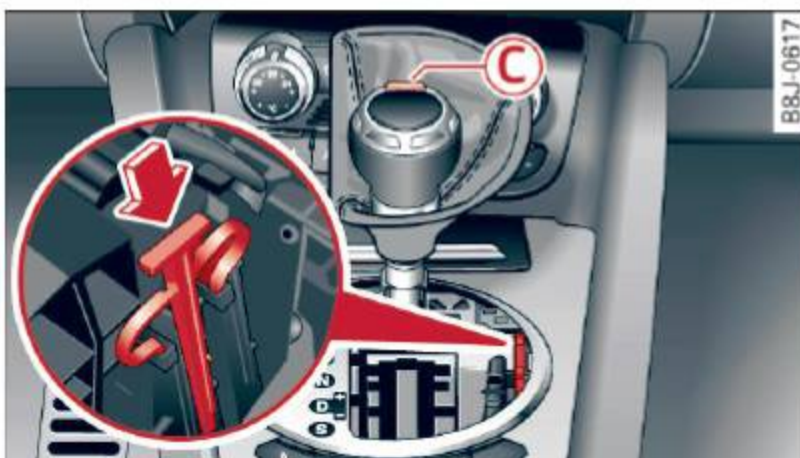
Fig. 94 Selector lever: Using the emergency release to move out of the Park position
