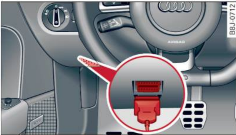
Fig. 26 Location of Data Link Connector (DLC)
