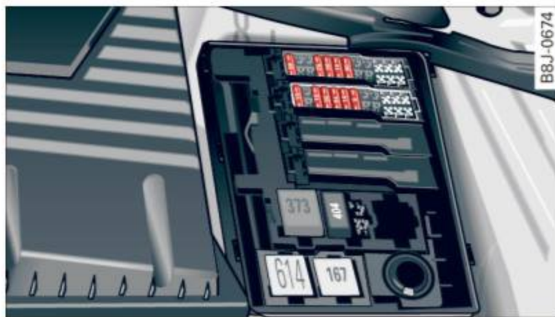
Fig. 176 Illustration of fuse holder on left side of engine compartment: fuses (without fuse cover)
