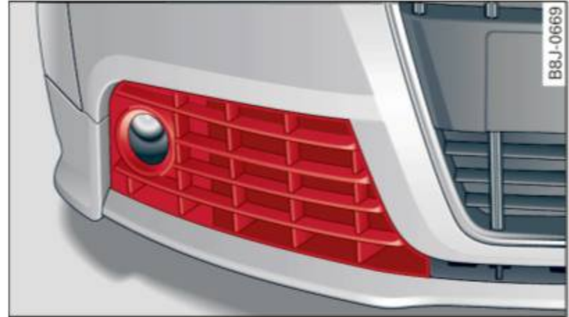
Fig. 181 Right front section: removing the air intake grille
