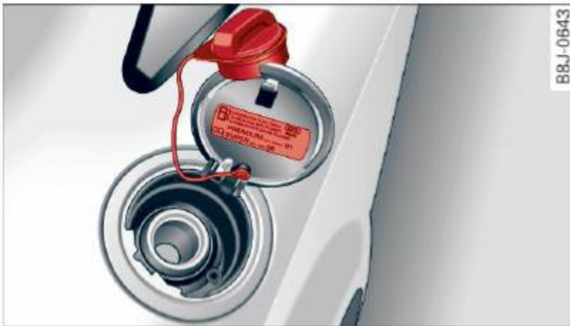
Fig. 137 Fuel cap hooked on the opened fuel filler flap
