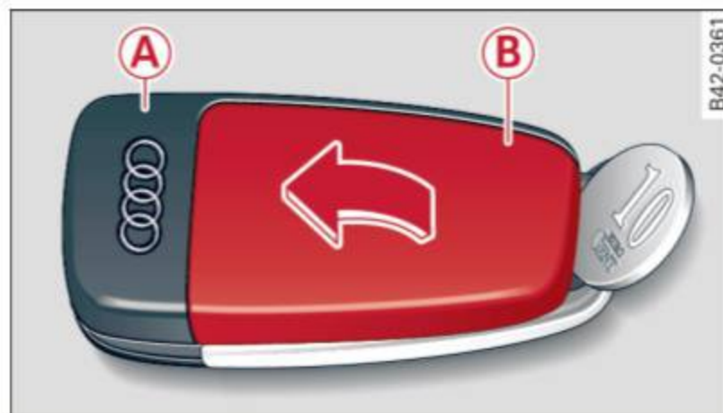
Fig. 30 Master key: opening the cover
