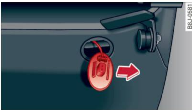
Fig. 39 Section: Interior luggage compartment: Emergency release
