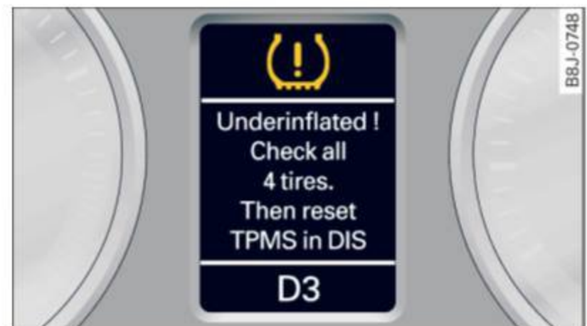
Fig. 155 Display: underinflation warning
