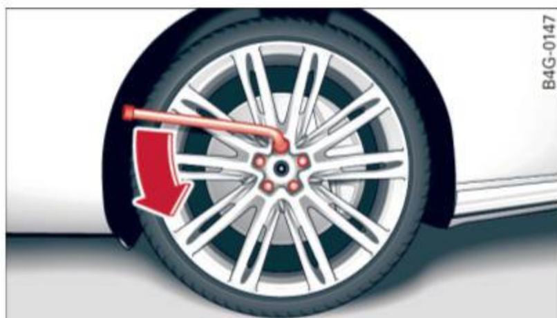
Fig. 212 Changing a wheel: loosening the wheel bolts
