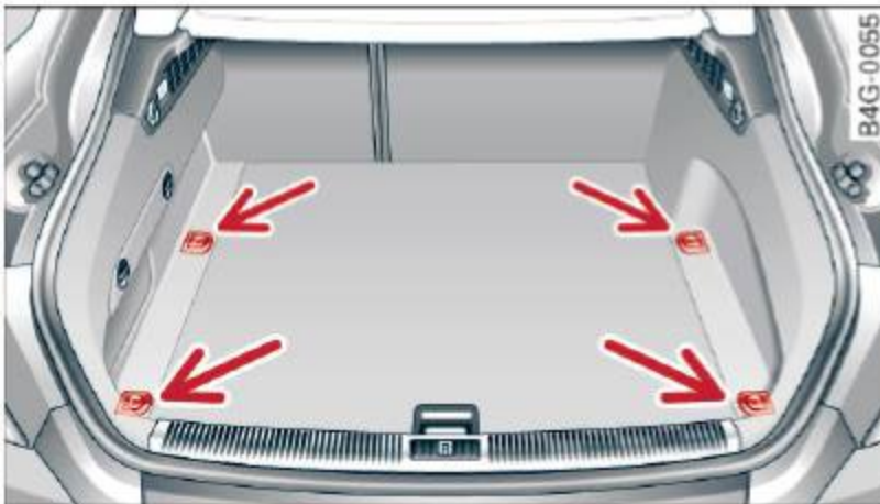
Fig. 66 Location of the tie-downs in the luggage compartment
