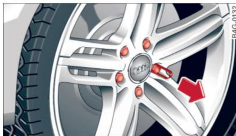
Fig. 211 Changing a wheel: removing the wheel bolt caps
