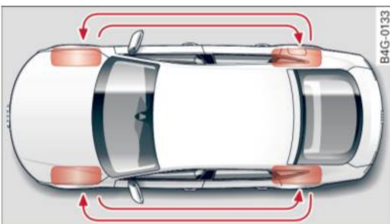
Fig. 203 Rotating tires for more even wear
