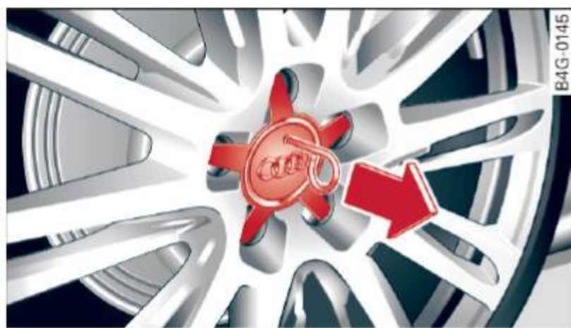
Fig. 210 Changing a wheel: Removing the wheel cover
