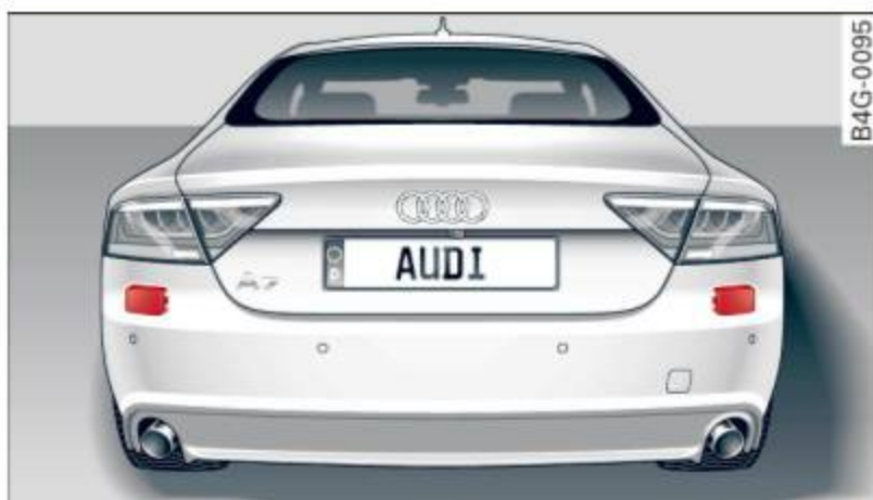
Fig. 105 Rear of the vehicle: position of the sensors
