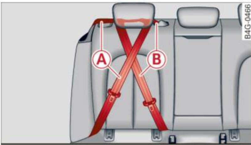
Fig. 171 Schematic overview: keep unused safety belts away from children in child safety seats. A - outer rear safety belt, B - center rear safety belt*
