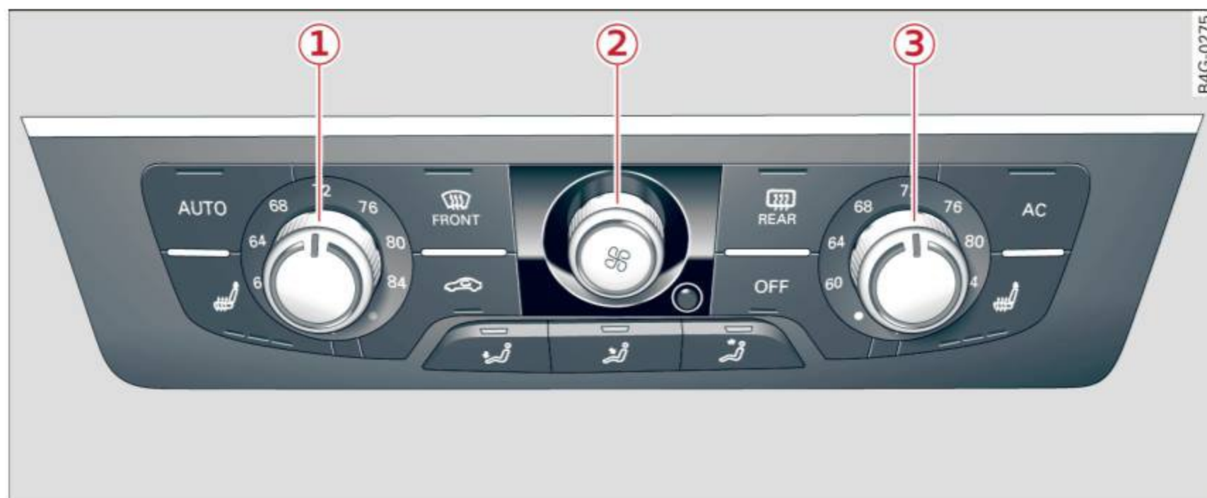
Fig. 73 Three-zone climate control: controls
