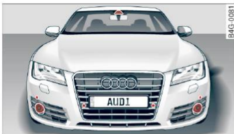
Fig. 87 Front of the vehicle: sensors and video camera
