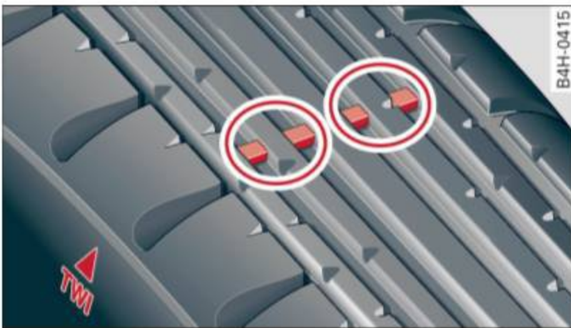
Fig. 202 Tire tread: tread wear indicators (TWI)
