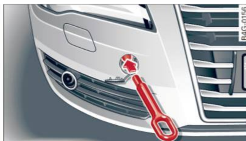
Fig. 225 Front bumper: installing the towing loop
