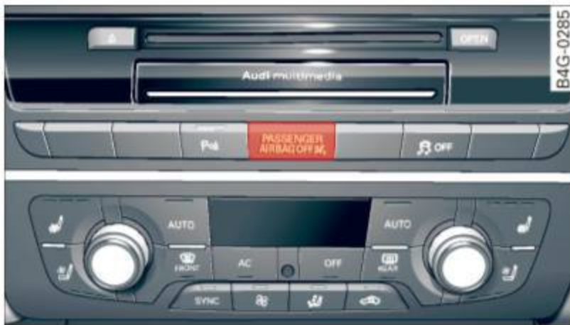
Fig. 164 Section from the instrument panel: PASSENGER AIR BAG OFF light
