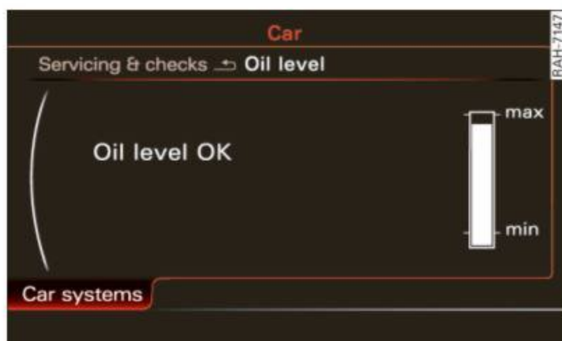
Fig. 194 Display: oil level indicator
