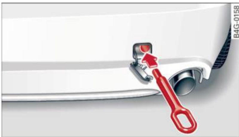
Fig. 227 Rear bumper: screwing in towing loop
