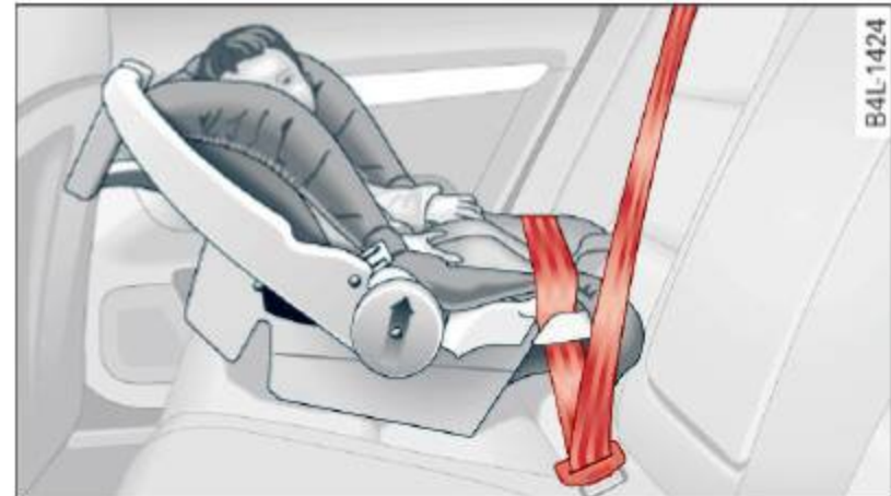
Fig. 172 Schematic overview: rearward-facing infant seat, properly installed on the rear seat
