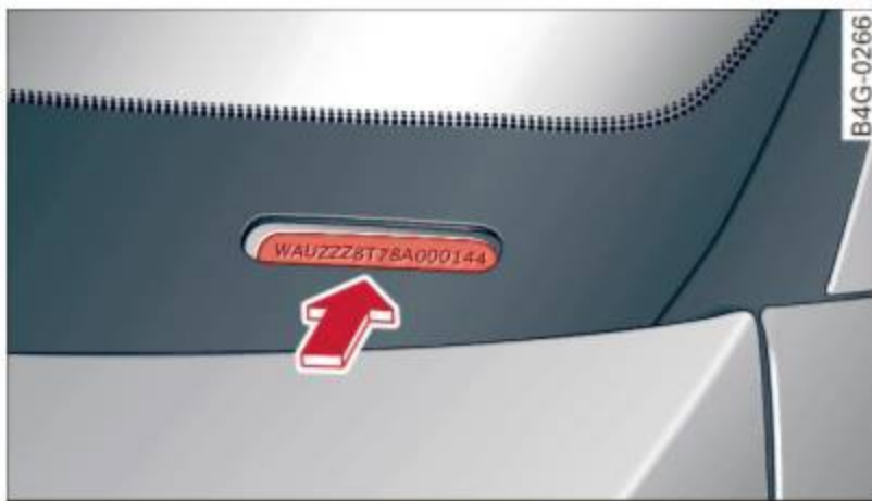
Fig. 231 Vehicle Identification Number (VIN) plate: location on driver's side dash panel
