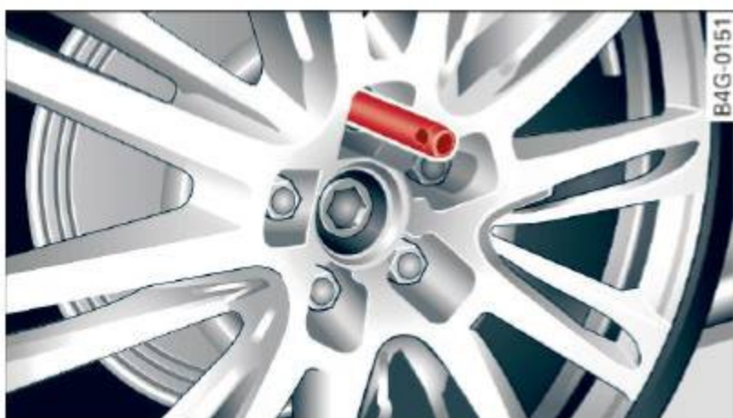
Fig. 217 Changing a wheel: alignment pin inside the top hole
