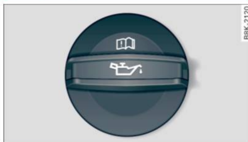
Fig. 195 Engine compartment: cover on the engine oil filler neck
