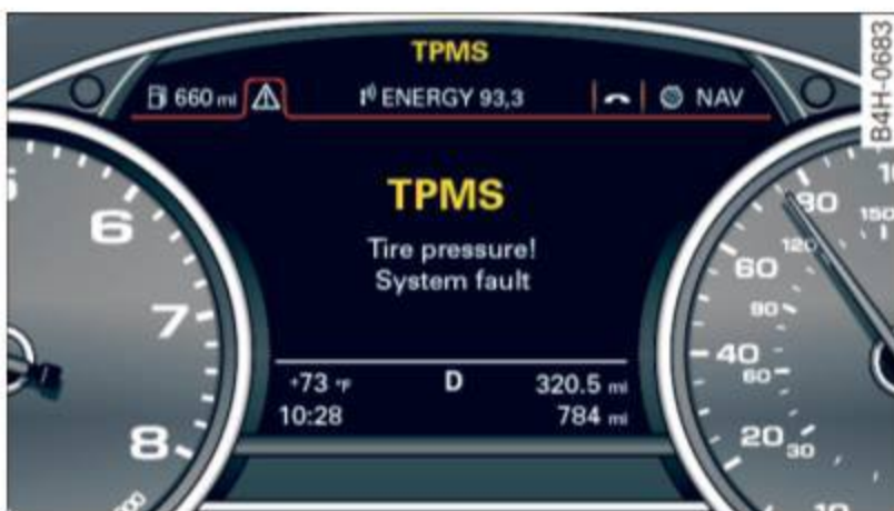
Fig. 206 Display: System malfunction
