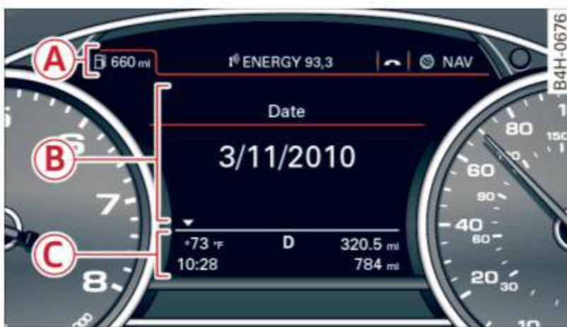
Fig. 4 Driver information system in the instrument cluster
