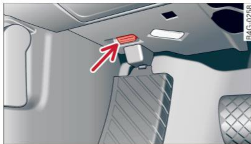
Fig. 16 Location of Data Link Connector (DLC)
