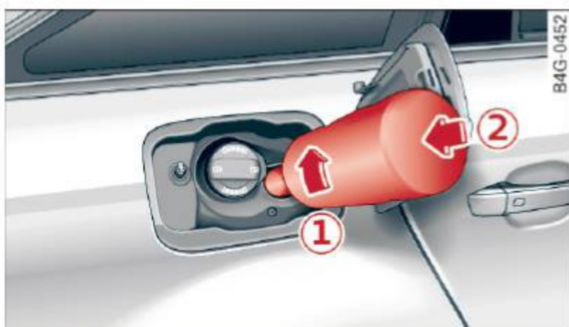
Fig. 190 AdBlue filler tube: inserting the refill bottle
