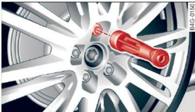
Fig. 216 Changing a wheel: using the screwdriver handle (with the blade removed) to turn the bolts
