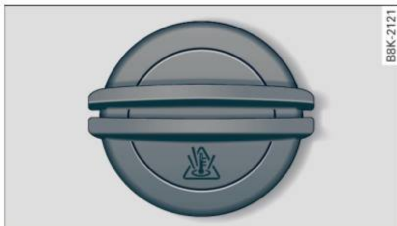
Fig. 196 Engine compartment: cover on the coolant expansion tank
