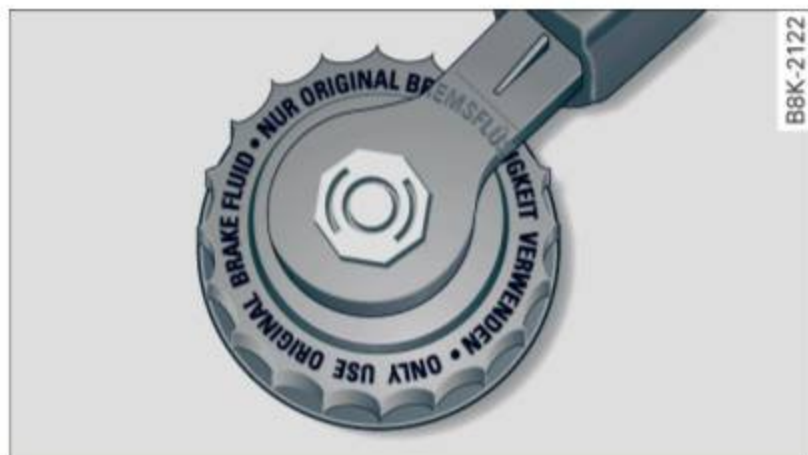
Fig. 197 Engine compartment: cover on the brake fluid reservoir
