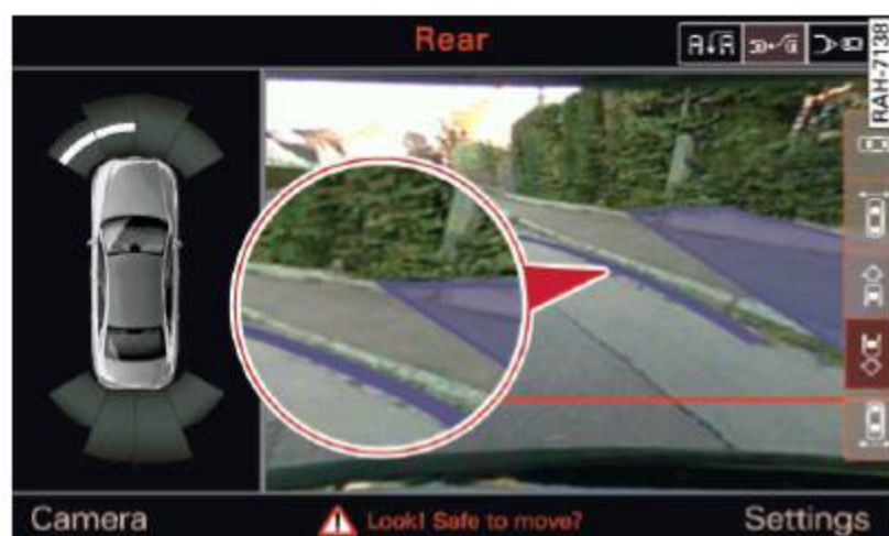
Fig. 144 Infotainment: contact of the blue curved line with the curb
