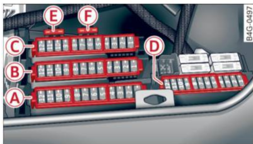
Fig. 221 Luggage compartment: fuse panel with plastic bracket
