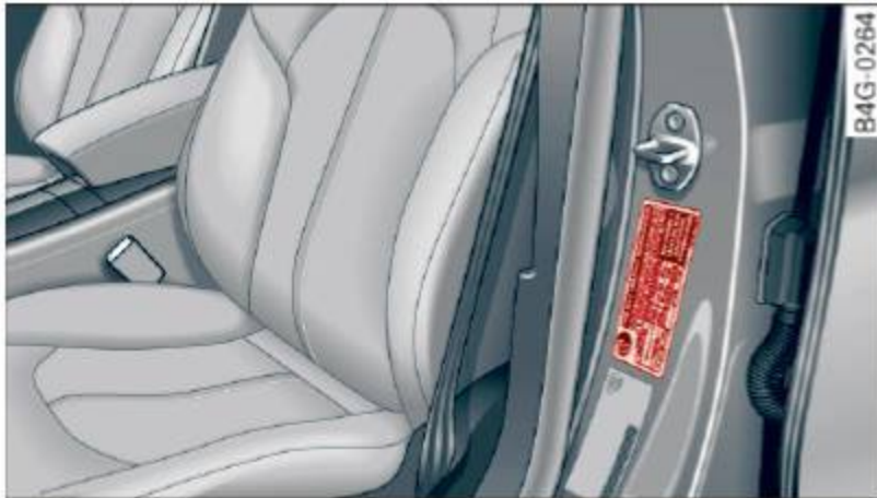
Fig. 200 Tire pressure label: located on driver's side B-pillar
