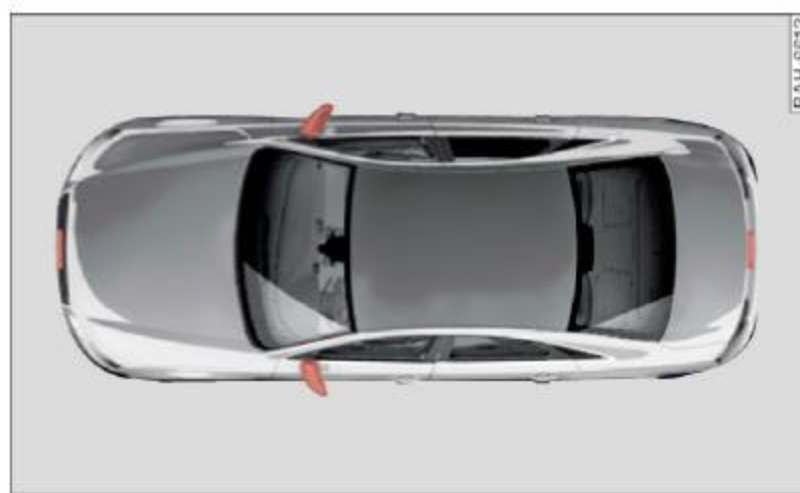
Fig. 133 Location of peripheral cameras
