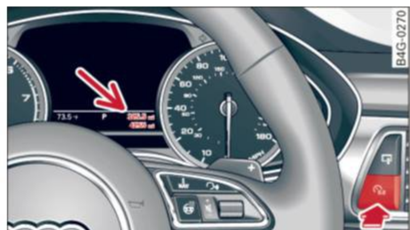
Fig. 11 Instrument cluster: Odometer and reset button
