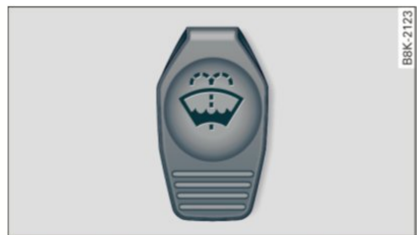
Fig. 199 Engine compartment: cover on the windshield and headlight* washer fluid reservoir
