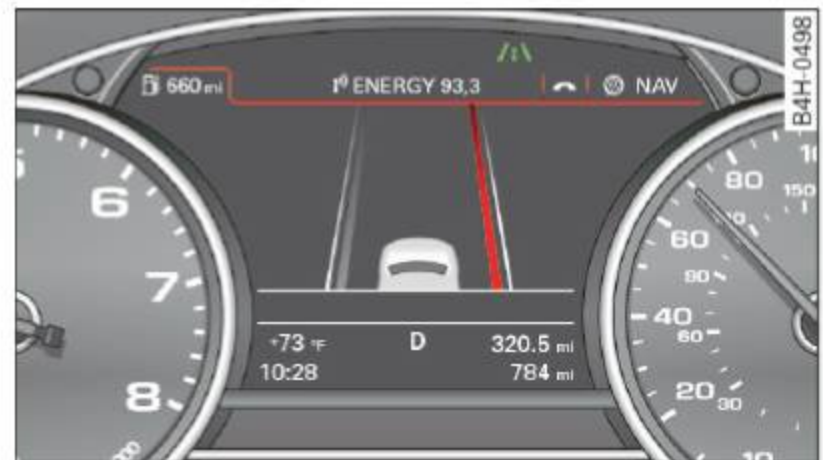
Fig. 100 Display: Active lane assist is switched on and is warning
