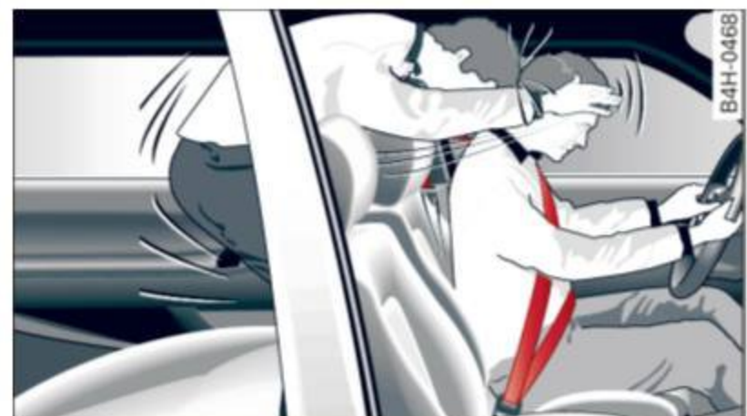
Fig. 154 A rear passenger not wearing a safety belt will fly forward and strike the driver
