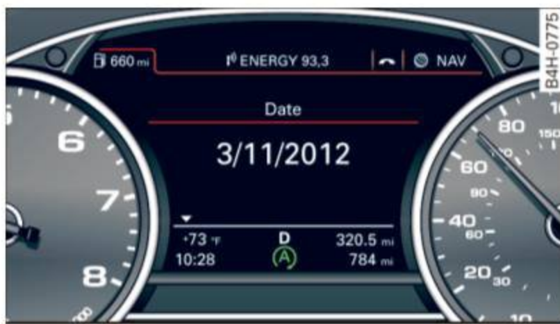
Fig. 82 Instrument cluster: engine switched off (stop phase)
