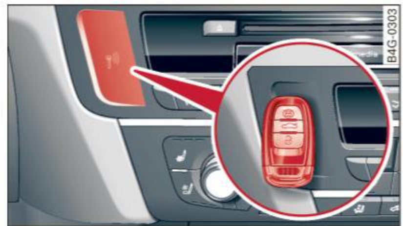
Fig. 80 Center console/master key: starting the engine if there is a malfunction
