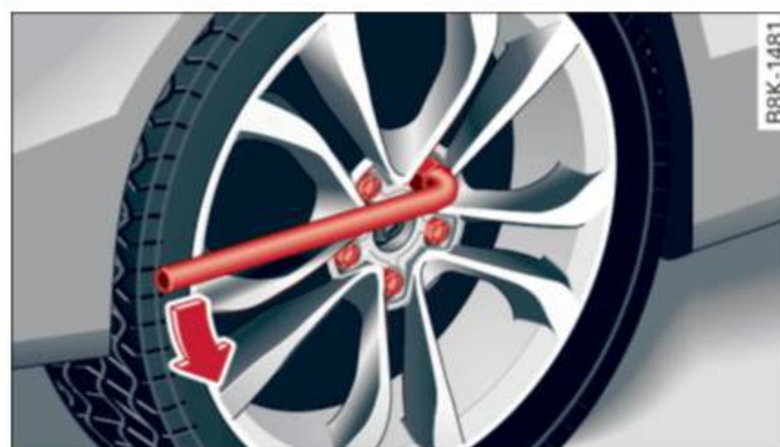
Fig. 206 Changing a tire: loosen the wheel bolts
