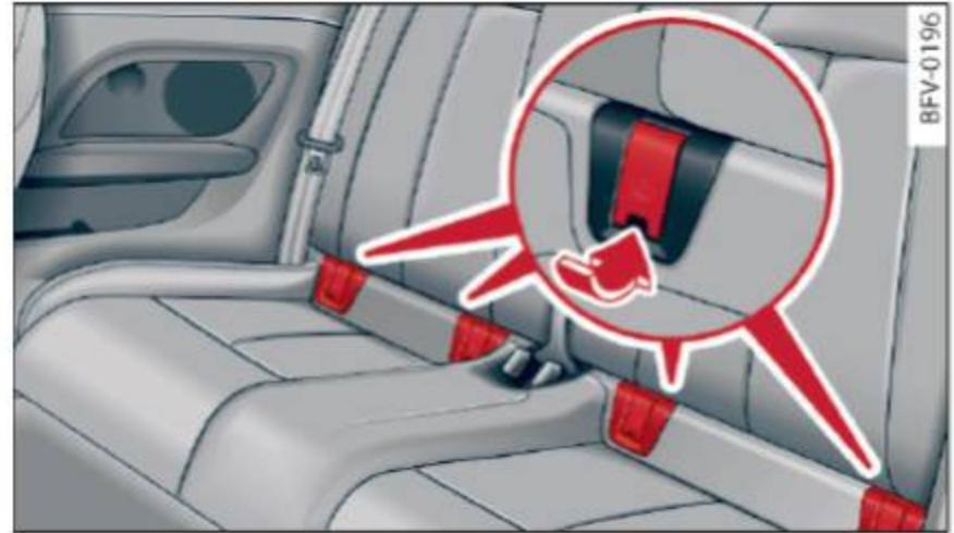
Fig. 176 Lower anchorages, covers marked
