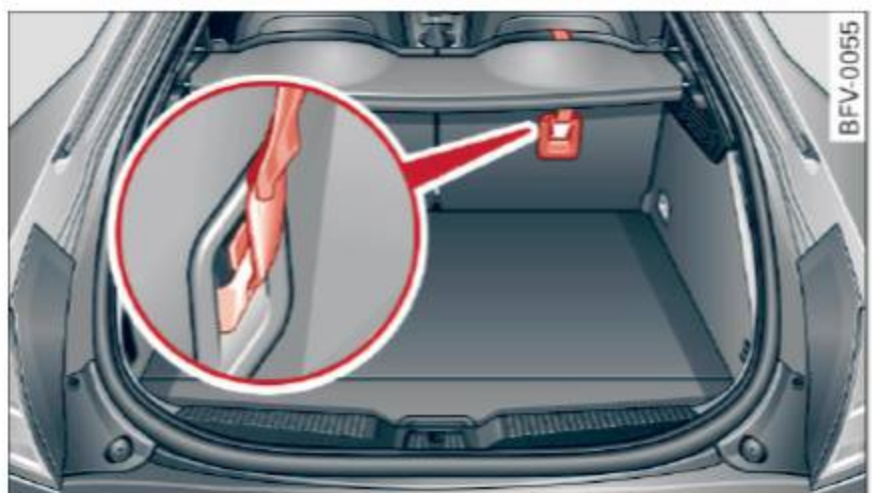
Fig. 181 Tether strap: proper routing and mounting
