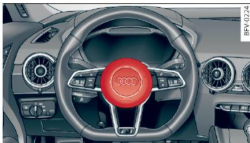
Fig. 160 Location of driver airbag: in steering wheel
