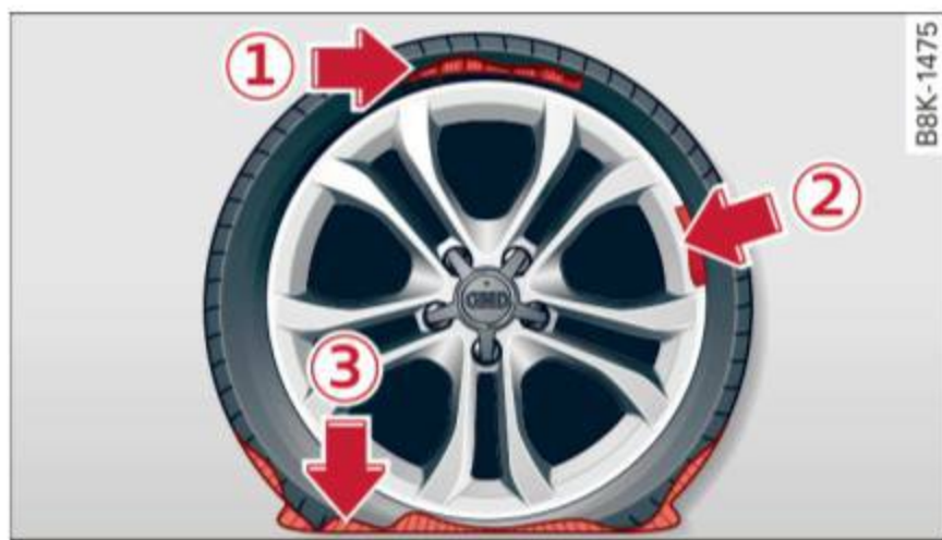
Fig. 201 Tire: tire damage that cannot be repaired
