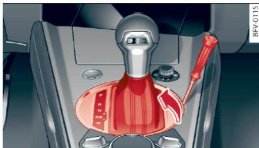
Fig. 68 Selector lever: removing the cover
