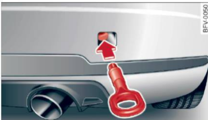
Fig. 222 Rear bumper: installing the towing loop
