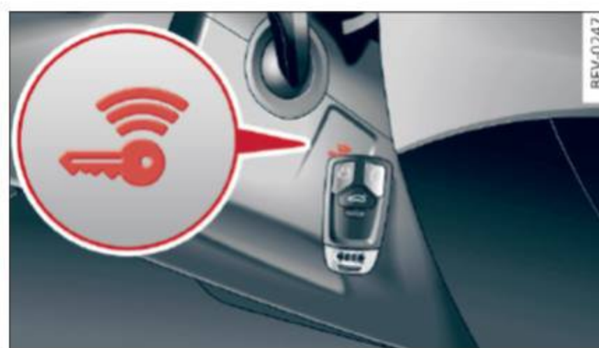
Fig. 61 Steering column/remote control key: starting the engine if there is a malfunction
