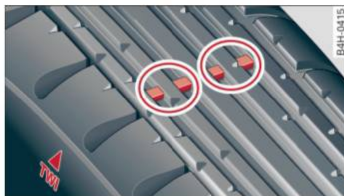
Fig. 197 Tire profile: treadwear indicator
