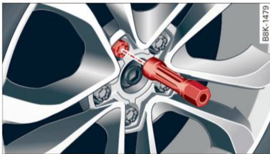
Fig. 209 Wheel: internal hex socket to turn the wheel bolts
