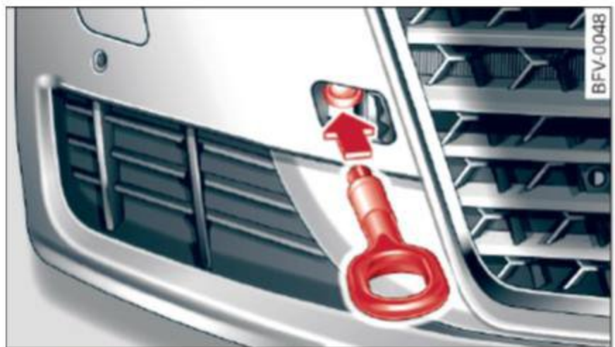
Fig. 220 Front bumper: installing the towing loop
