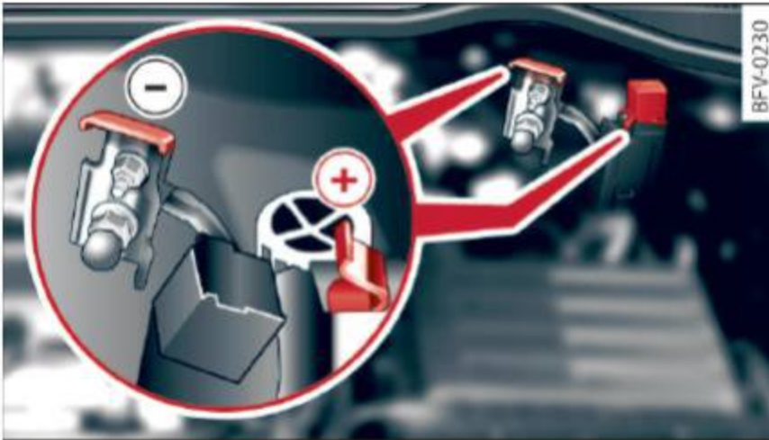
Fig. 217 Engine compartment: connectors for jump start cables and charger
