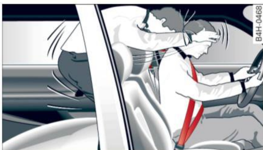
Fig. 154 A rear passenger not wearing a safety belt will fly forward and strike the driver
