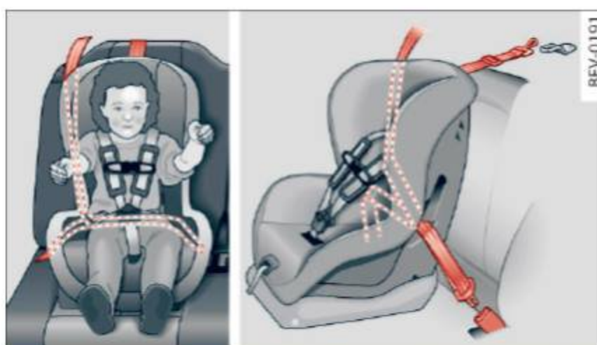
Fig. 173 Schematic overview: installation of the seat using the vehicle's safety belt system
