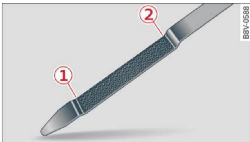
Fig. 190 Oil dipstick (example): checking the engine oil level
