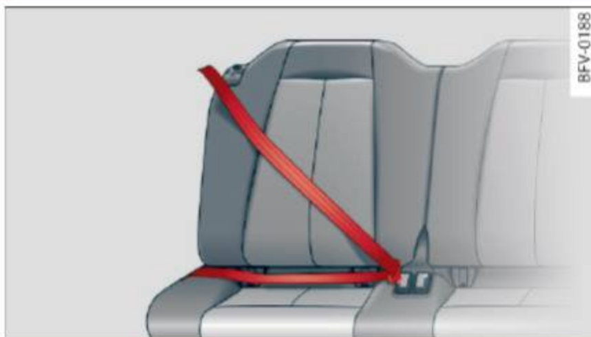
Fig. 170 Schematic overview: keep unused safety belts away from children in child safety seats. - outer rear safety belt,
