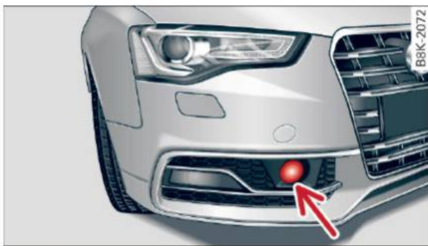
Fig. 93 Front of the vehicle: Position of radar sensor
