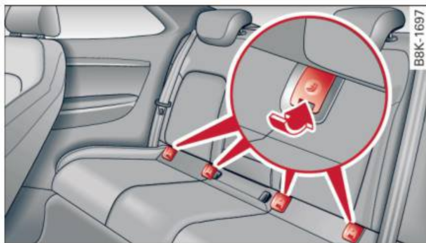
Fig. 148 Lower anchorages, covers marked
