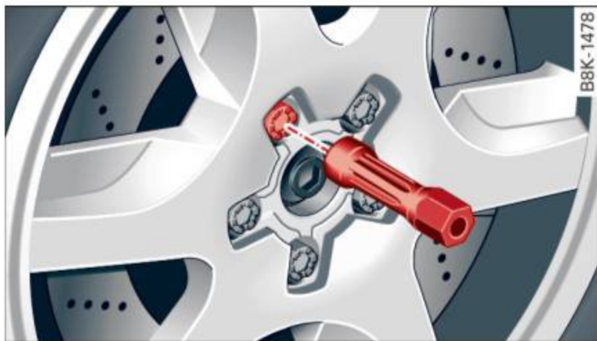
Fig. 180 Changing a wheel: using the screwdriver handle (with the blade removed) to turn the bolts
