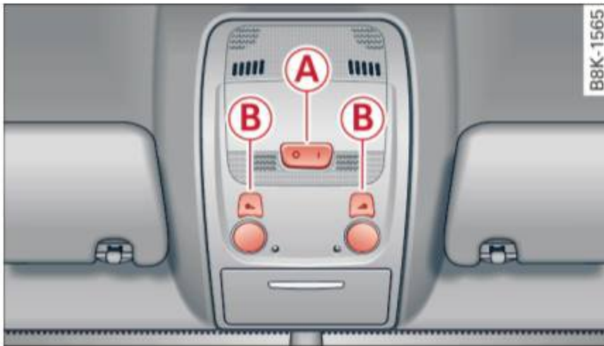
Fig. 40 Front headliner: interior lighting controls
