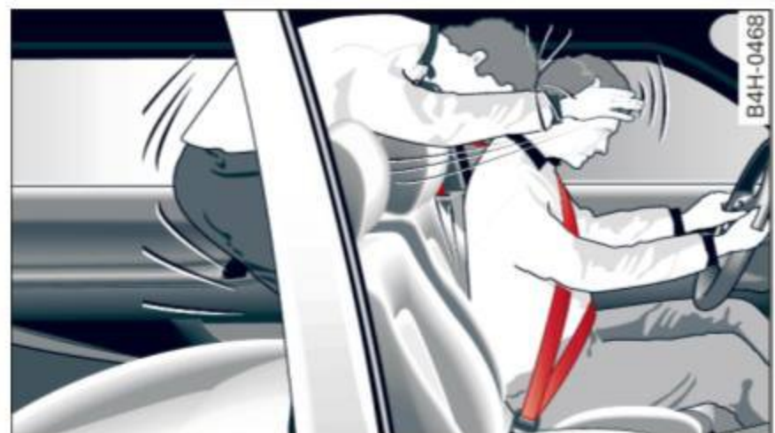
Fig. 126 A rear passenger not wearing a safety belt will fly forward and strike the driver
