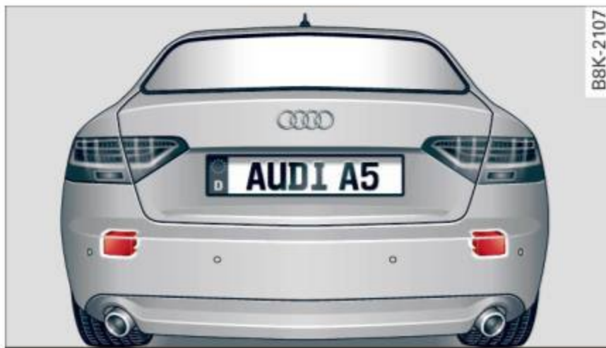
Fig. 107 Rear of the vehicle: position of the sensors
