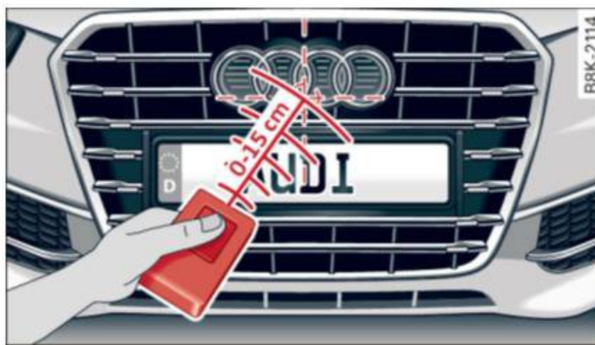
Fig. 35 Distance between the radiator grille and the hand transmitter
