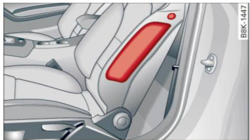
Fig. 137 Side airbag location in the driver's seat
