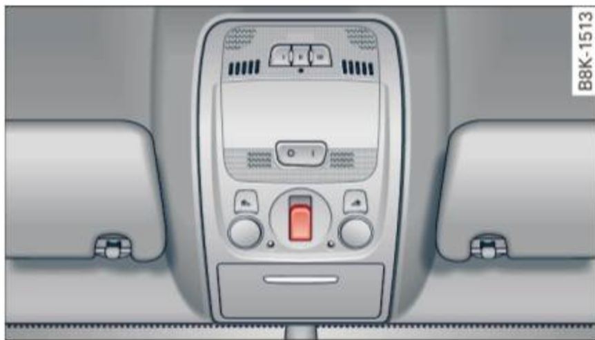
Fig. 31 Section of headliner: switch for sunroof
