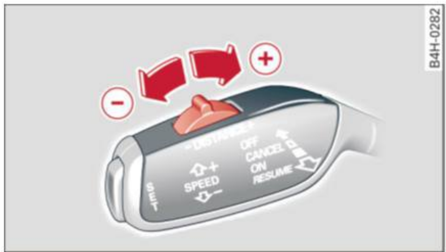
Fig. 100 Selector lever: setting the distance
