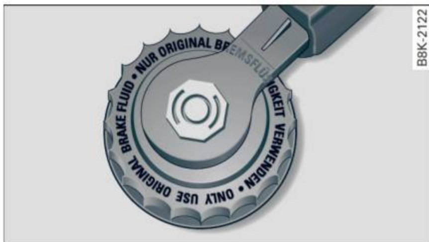
Fig. 164 Engine compartment: Cover on the brake fluid reservoir
