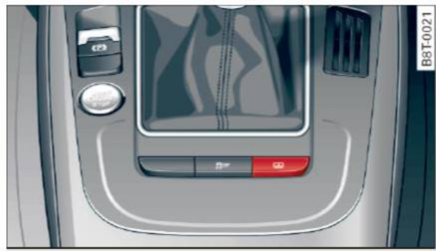
Fig. 46 Without MMI: Button for rear window sun shade
