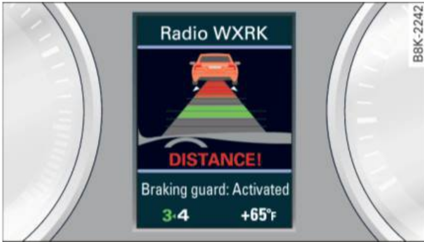
Fig. 102 Instrument cluster: approach warning
