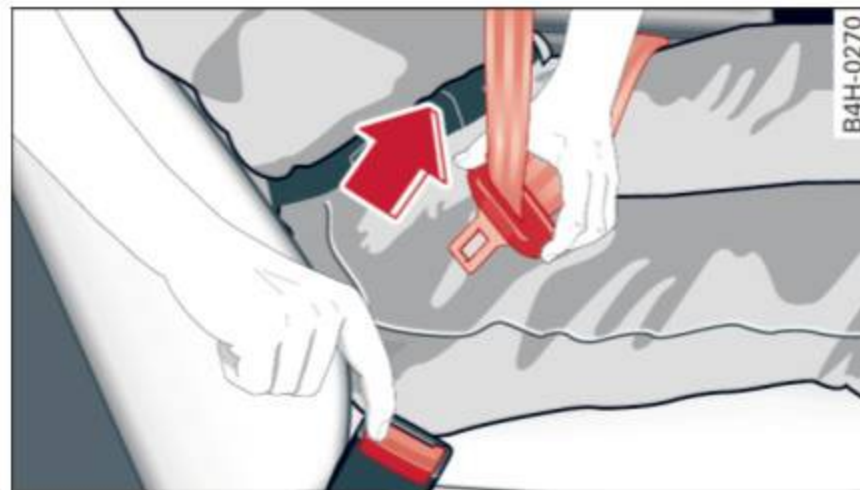
Fig. 130 Releasing the tongue from the buckle
