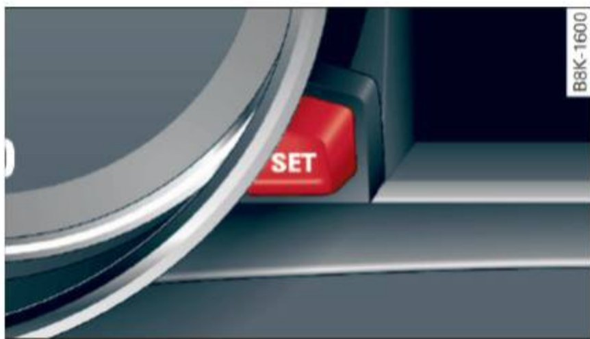
Fig. 81 SET button in the instrument cluster
