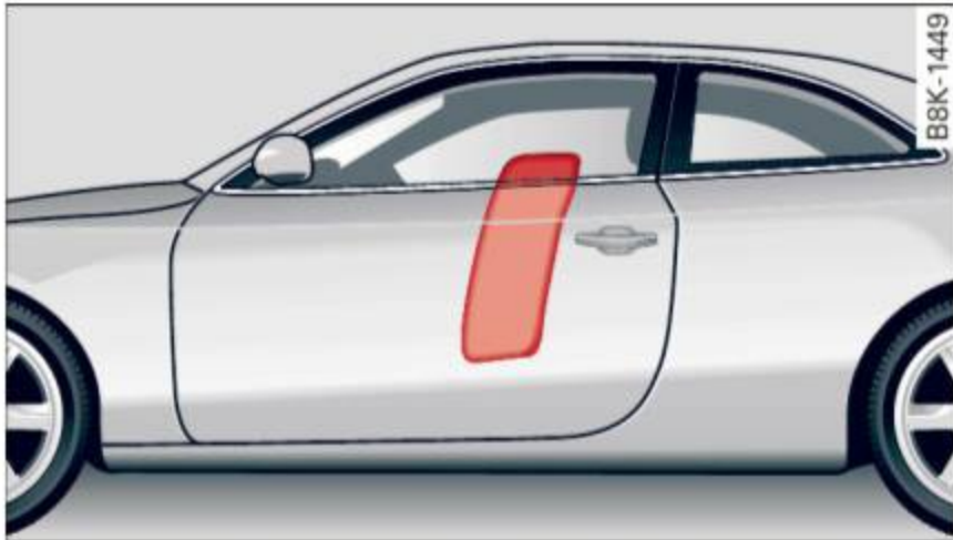
Fig. 138 Inflated side airbags on left side of vehicle
