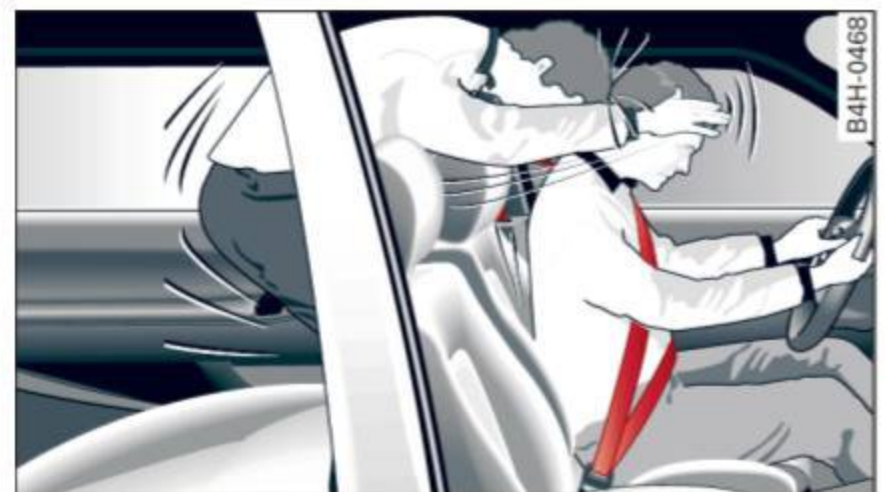
Fig. 125 A rear passenger not wearing a safety belt will fly forward and strike the driver
