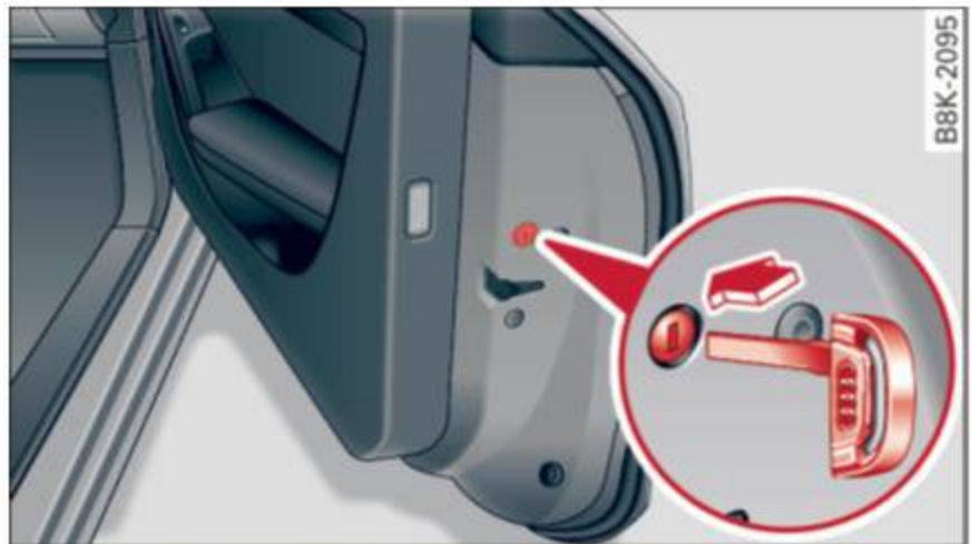
Fig. 25 Front passenger's door: emergency lock
