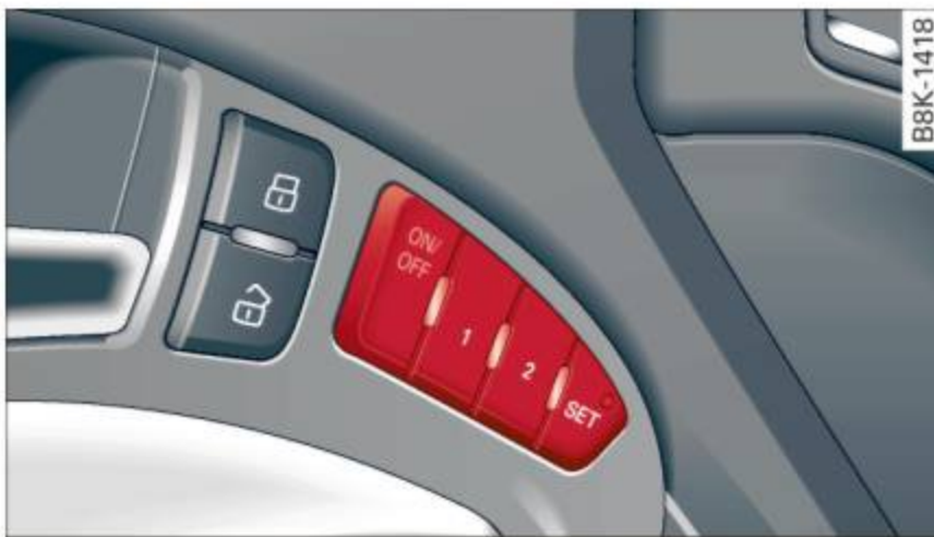
Fig. 59 Driver's door: memory function buttons
