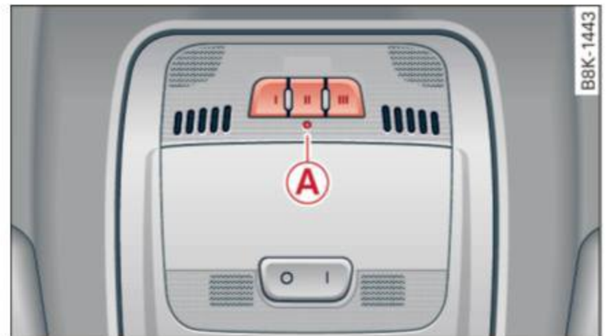
Fig. 34 Headliner: control unit
