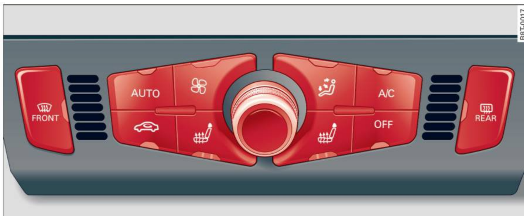
Fig. 73 Automatic climate control system: control
