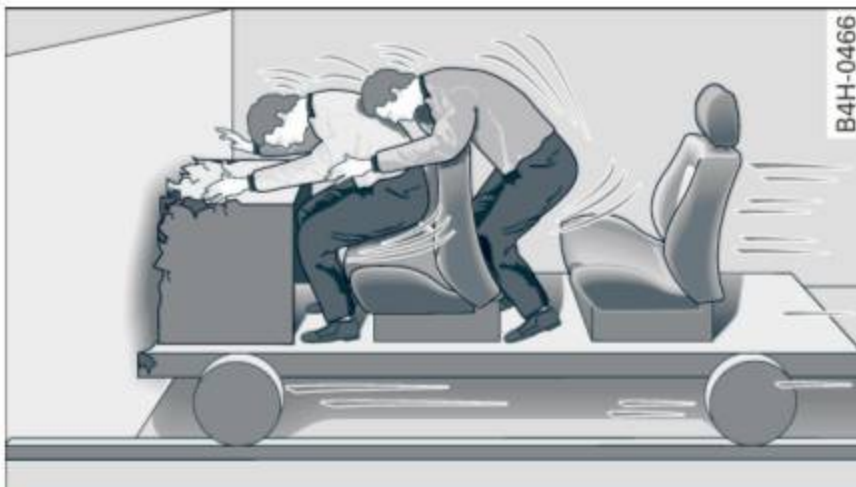
Fig. 123 The vehicle crashes into the wall
