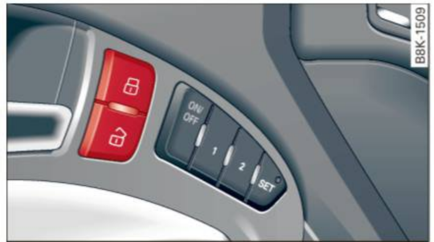
Fig. 23 Driver's door: power locking switch
