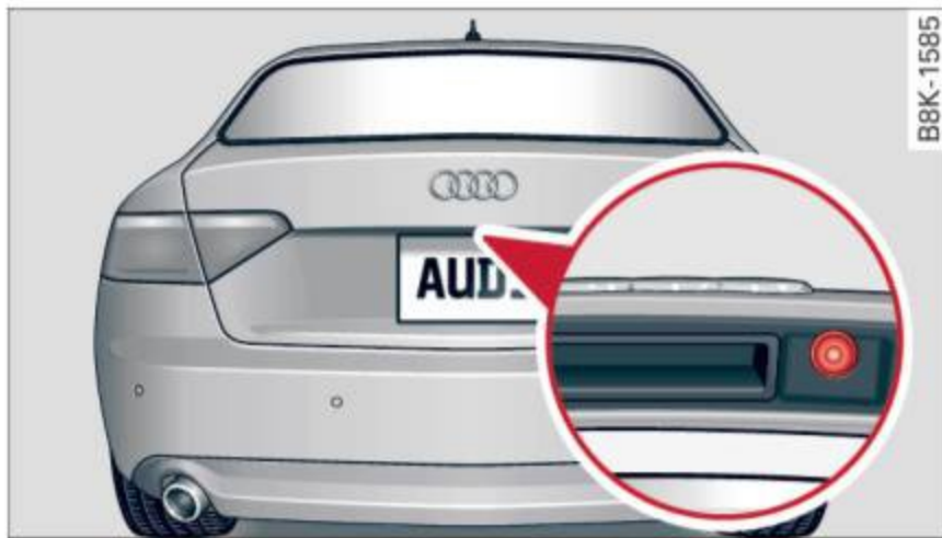
Fig. 113 Trunk lid: Location of the rear view camera
