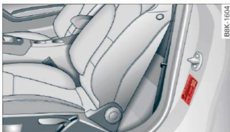
Fig. 169 Driver's side B-pillar: tire pressure label
