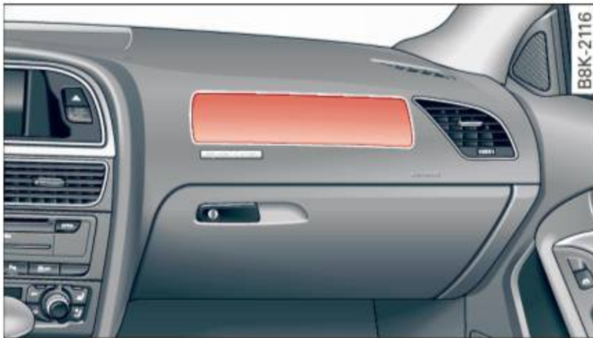
Fig. 132 Location of front passenger's airbag: in the instrument panel
