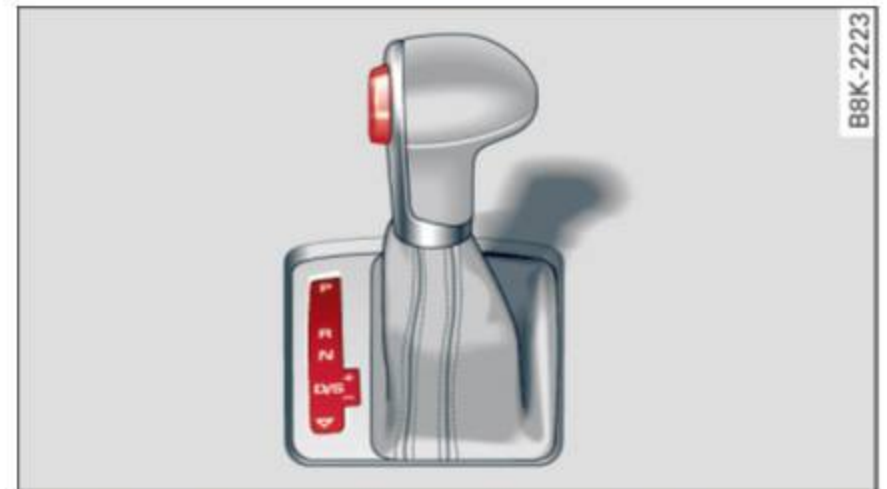
Fig. 87 Shift gate on the center console: selector lever with release button
