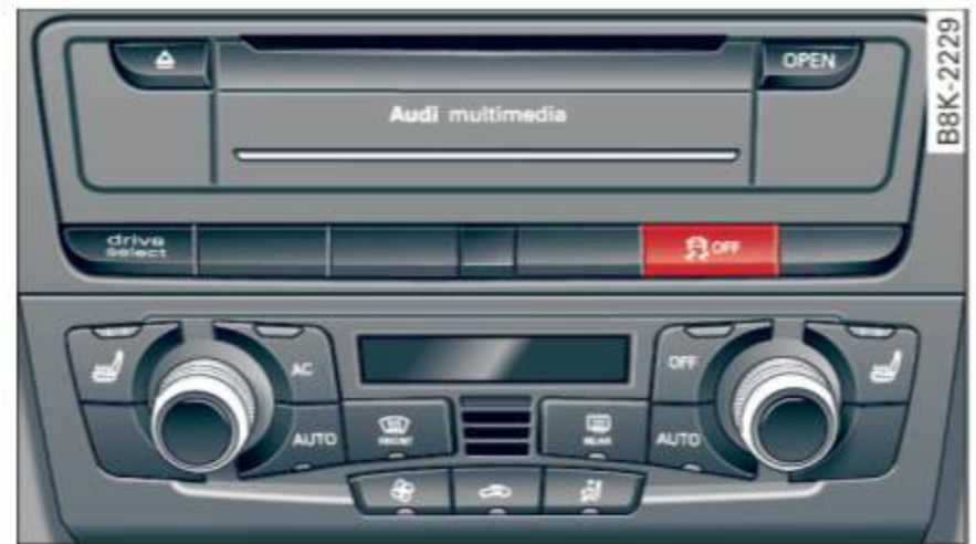
Fig. 153 Version B: upper center console, ESC OFF button
