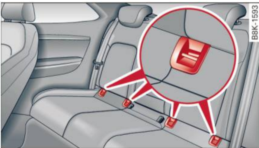
Fig. 148 Rear seats: lower anchorage bracket locations
