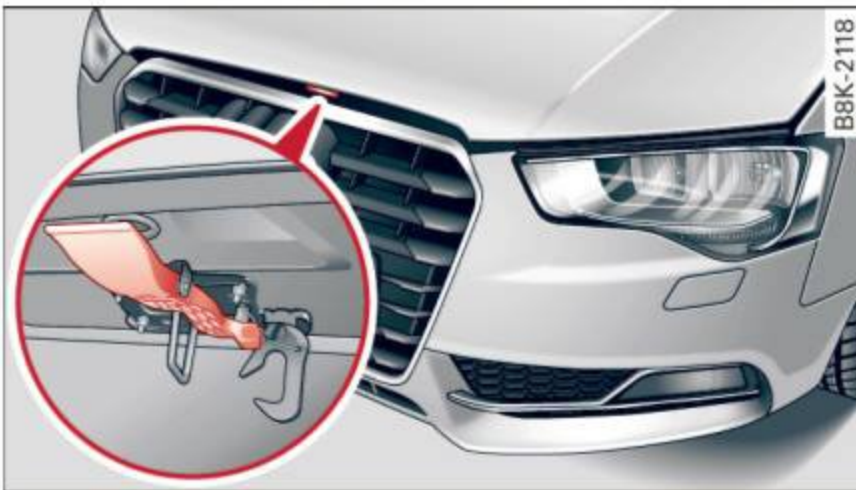
Fig. 159 Release lever under the engine hood
