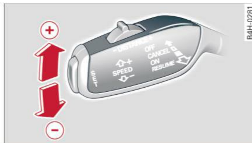
Fig. 98 Selector lever: changing the speed
