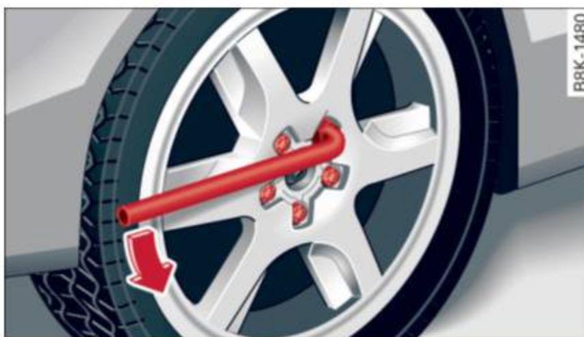
Fig. 176 Changing a wheel: loosening the wheel bolts
