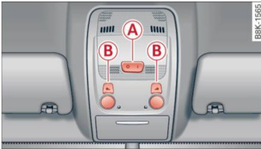
Fig. 39 Front headliner: interior lighting controls
