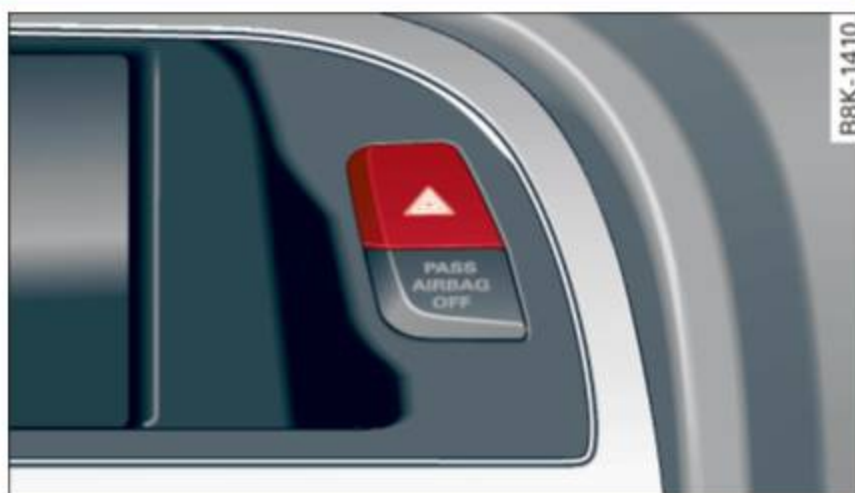
Fig. 38 Center console: emergency flasher switch
