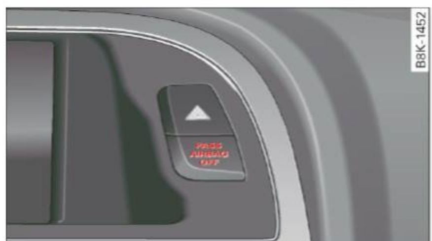
Fig. 134 Section from the instrument panel: PASSENGER AIR BAG OFF light
