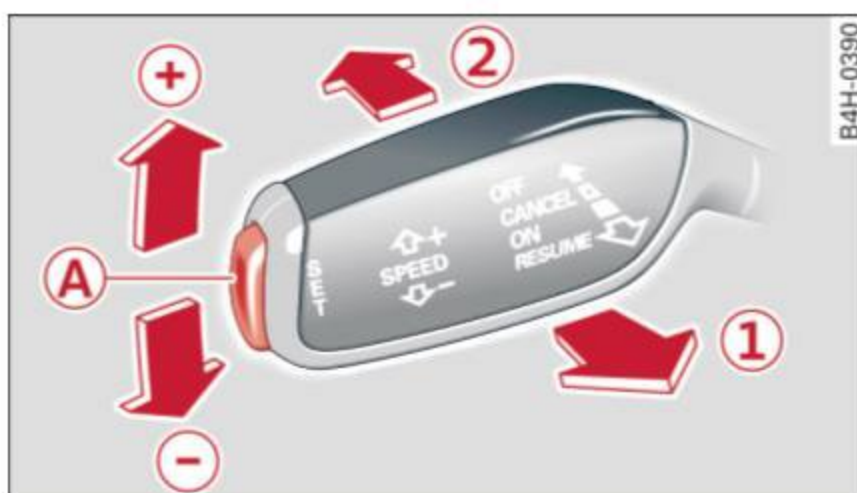
Fig. 82 Control lever with push-button
