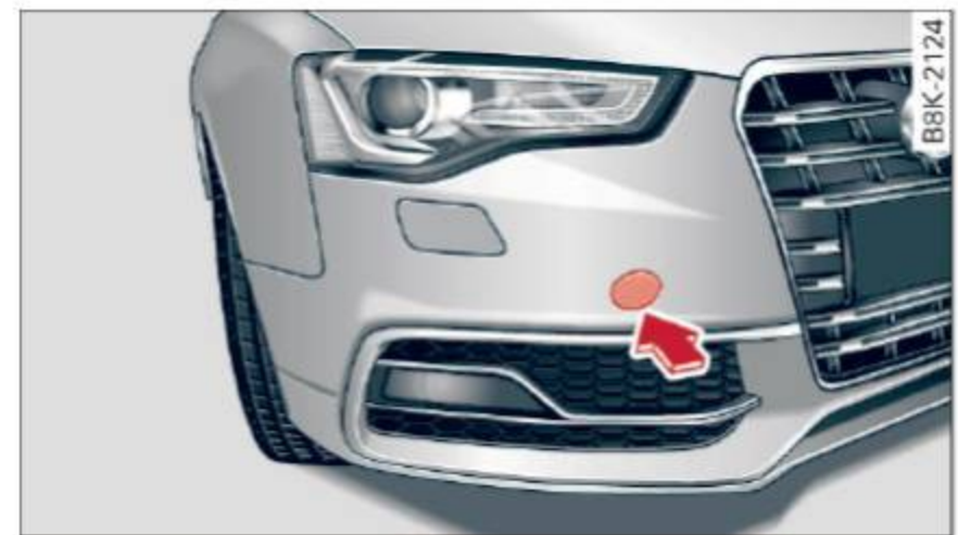
Fig. 187 Front bumper: removing the cover cap
