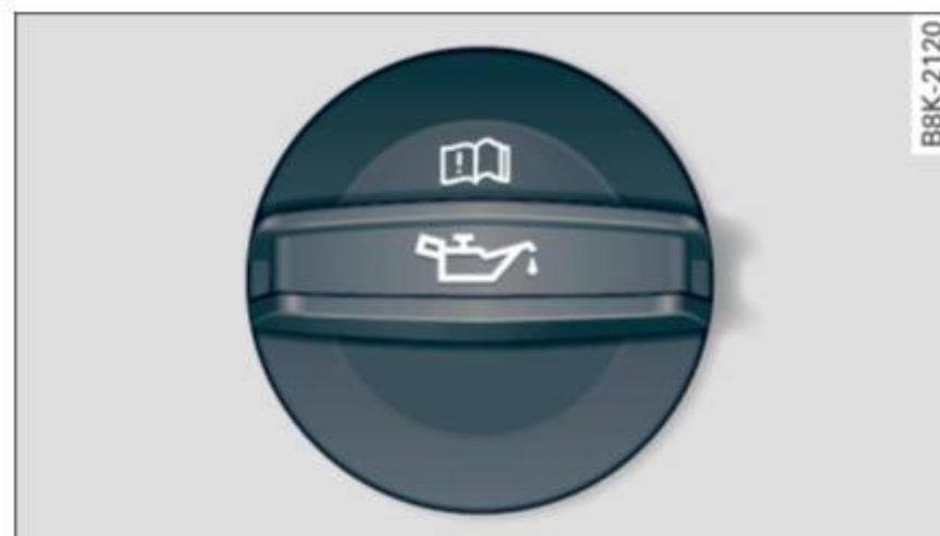
Fig. 162 Engine compartment: Cover on the oil filler neck
