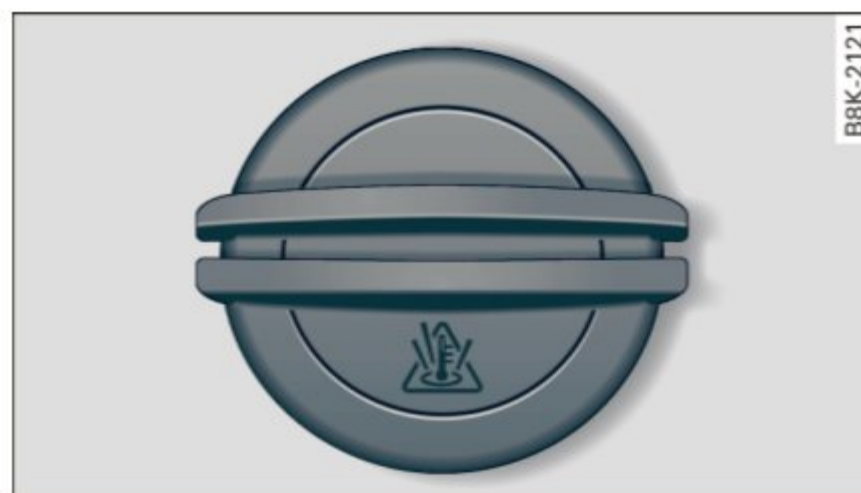
Fig. 163 Engine compartment: Cover on the coolant expansion tank
