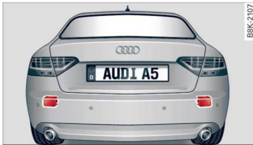
Fig. 106 Rear of the vehicle: position of the sensors
