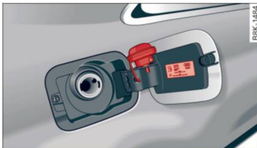
Fig. 155 Fuel filler flap with attached fuel cap
