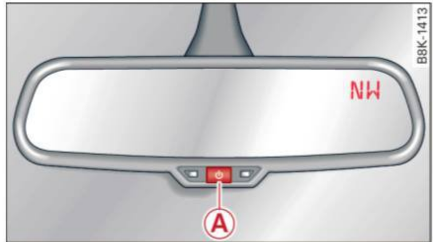
Fig. 49 Rearview mirror: Digital compass activated
