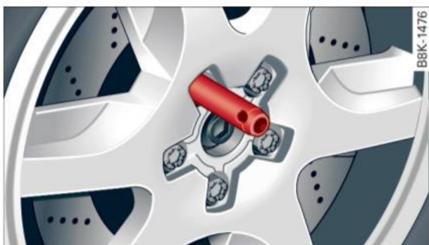
Fig. 180 Changing a wheel: alignment pin inside the top hole
