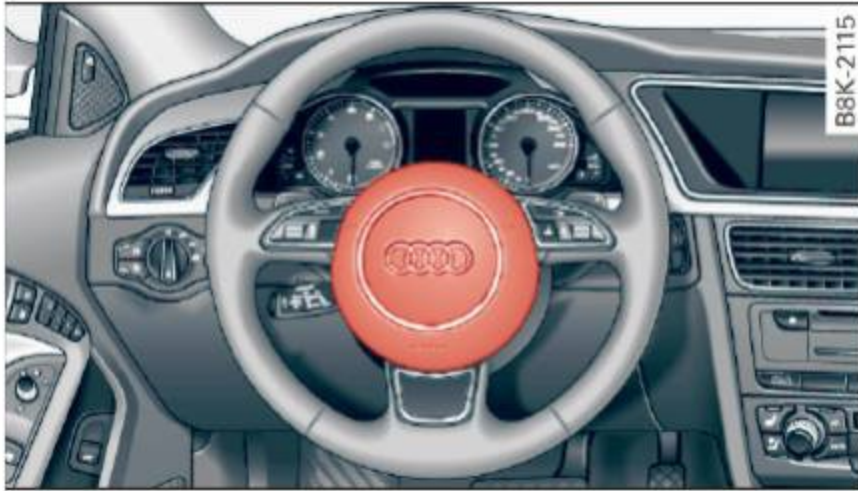
Fig. 131 Location of driver airbag: in steering wheel
