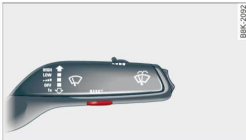
Fig. 8 Wiper lever: controls for the menu display
