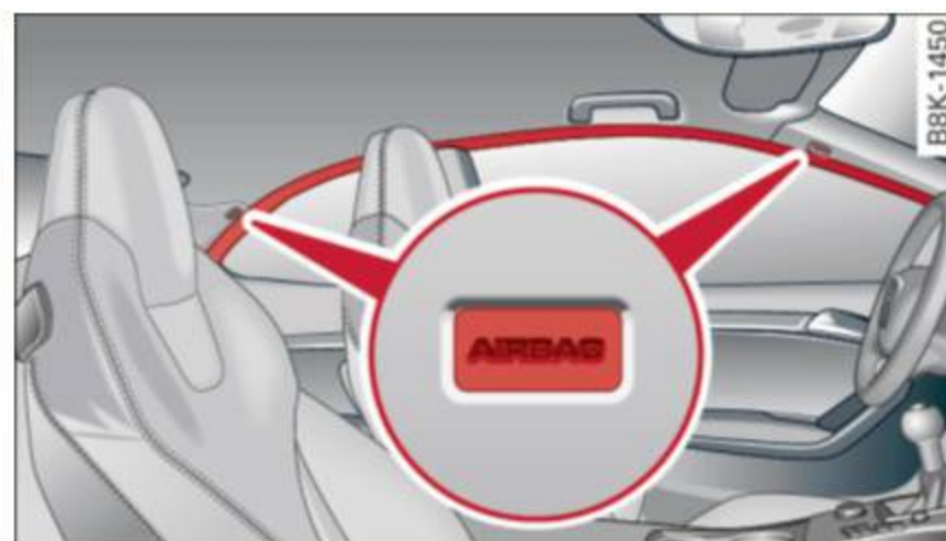
Fig. 139 Side curtain system, driver's side: side curtain airbag location
