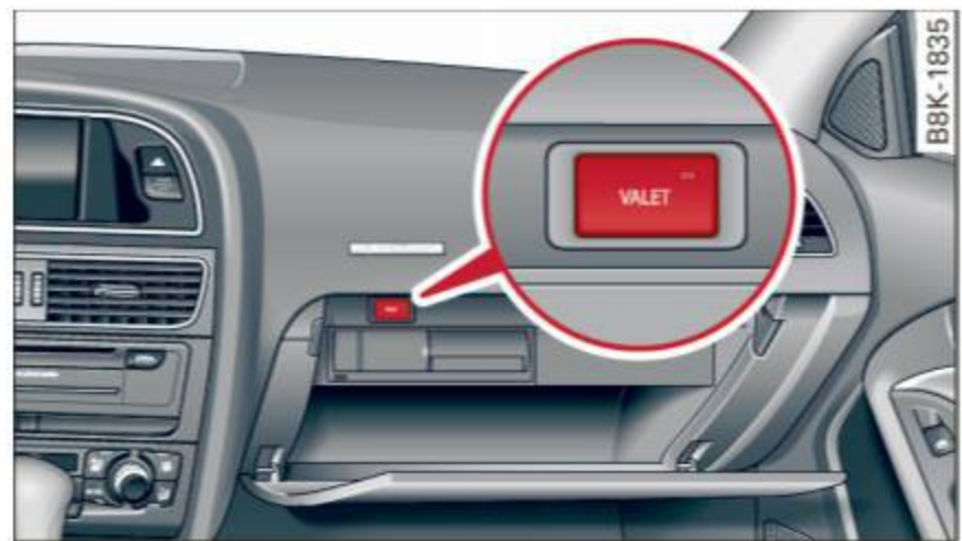
Fig. 32 Glove compartment: valet parking button
