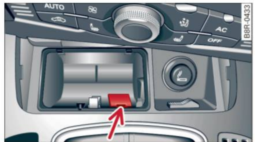
Fig. 91 Selector lever emergency release
