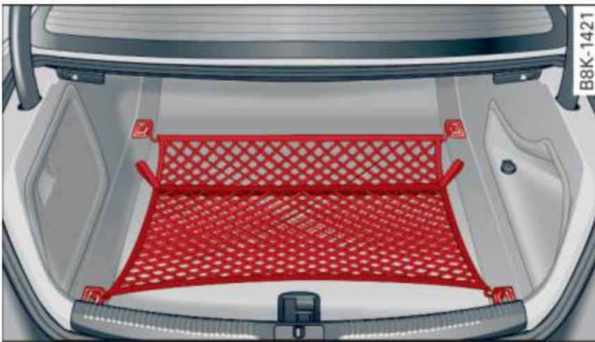
Fig. 68 Luggage compartment: cargo net stretched out
