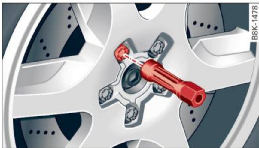
Fig. 179 Changing a wheel: using the screwdriver handle (with the blade removed) to turn the bolts
