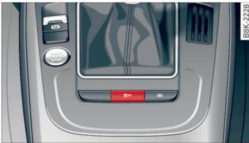
Fig. 152 Version A: lower center console, ESC OFF button
