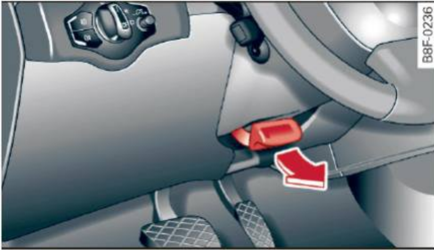
Fig. 75 Lever under the steering column
