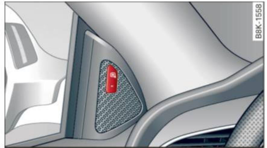
Fig. 107 Driver's door: Side assist button
