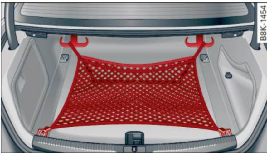
Fig. 69 Luggage compartment: cargo net at the top of the luggage compartment
