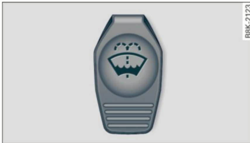
Fig. 166 Engine compartment: Cover on the windshield and headlight* washer fluid container
