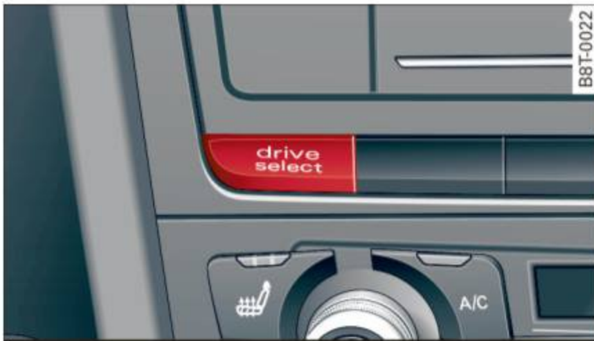
Fig. 108 Center console: Control for Audi drive select
