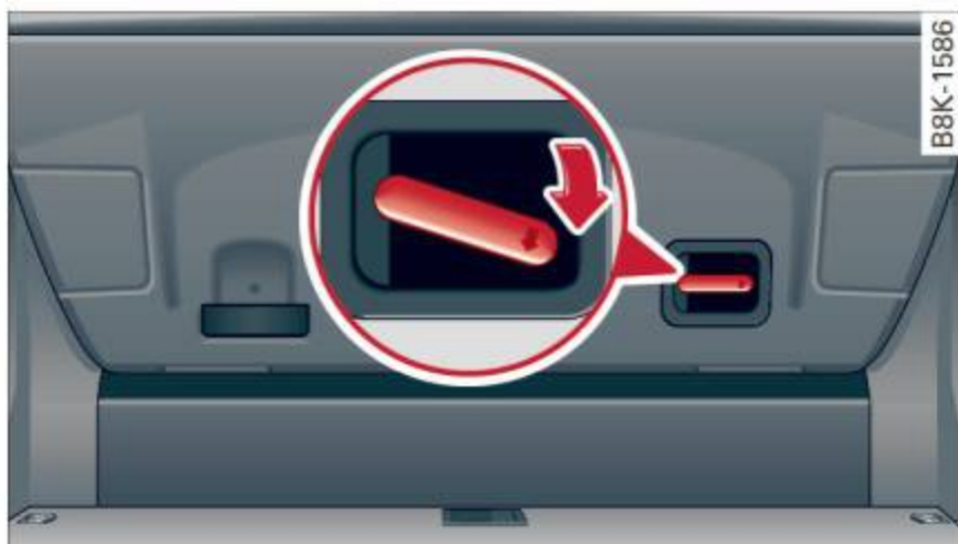
Fig. 28 Trunk escape handle: view from inside the closed rear lid
