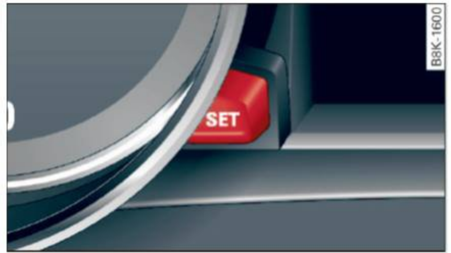
Fig. 4 SET button in the instrument cluster
