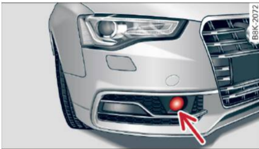
Fig. 92 Front of the vehicle: Position of radar sensor
