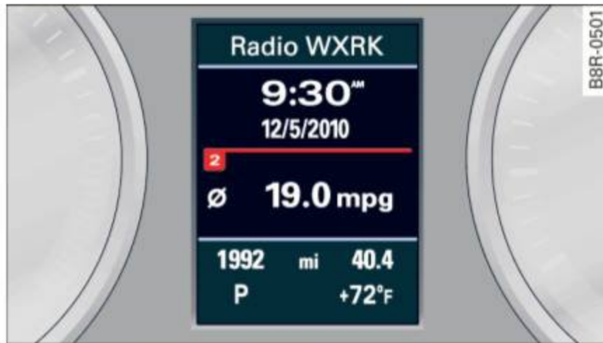
Fig. 7 Instrument cluster: center display
