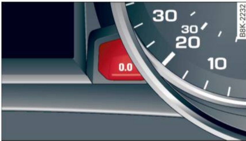
Fig. 6 Instrument cluster: reset button
