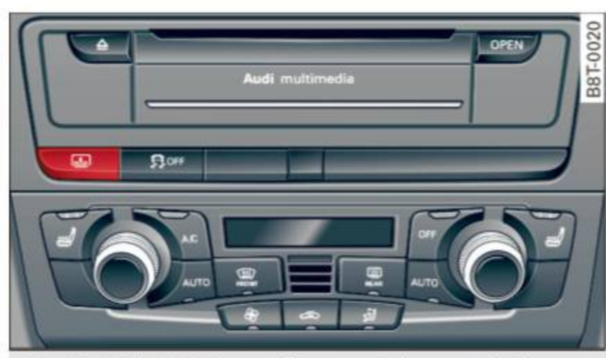
Fig. 45 With MMI: Button for rear window sun shade
