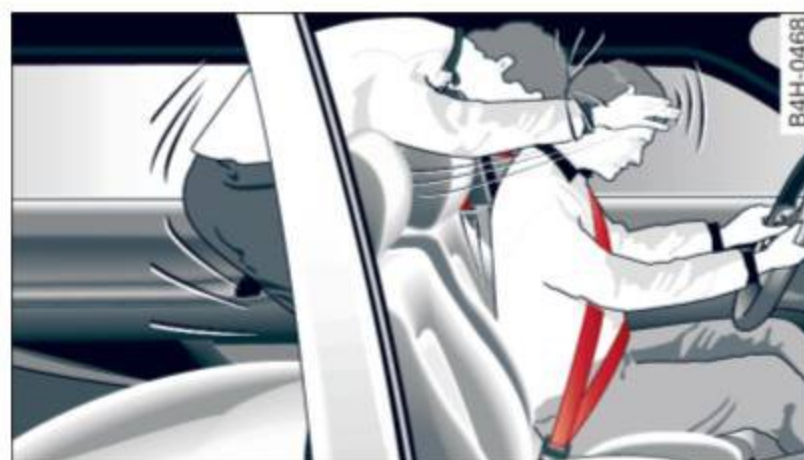
Fig. 126 A rear passenger not wearing a safety belt will fly forward and strike the driver
