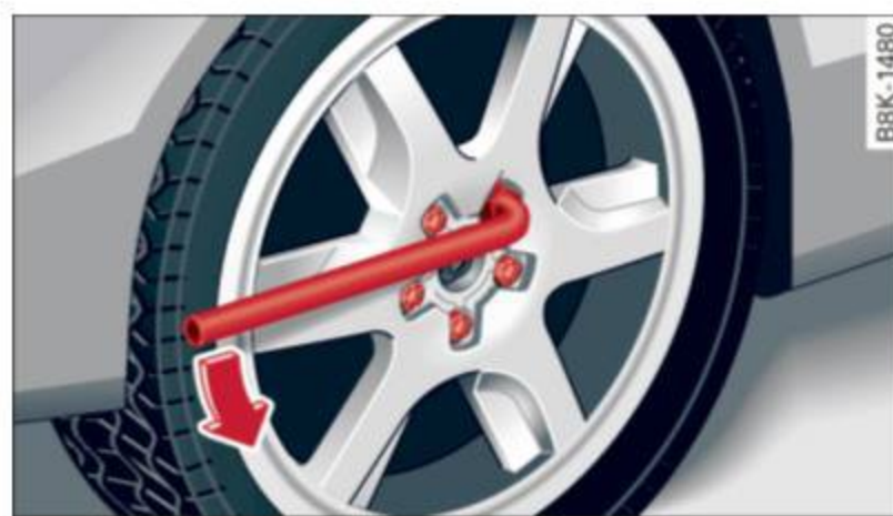
Fig. 178 Changing a wheel: loosening the wheel bolts
