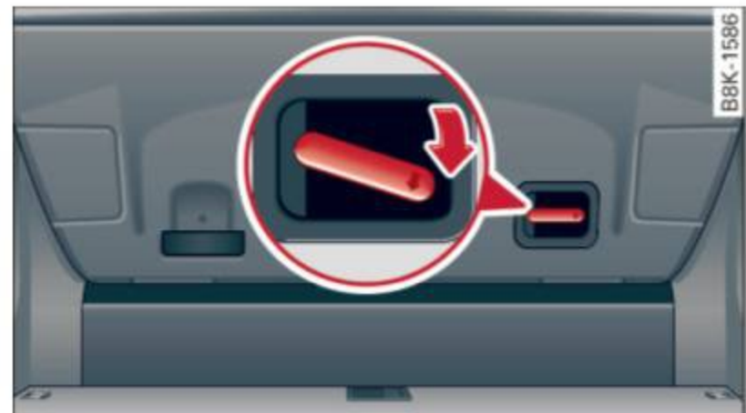
Fig. 29 Trunk escape handle: view from inside the closed rear lid
