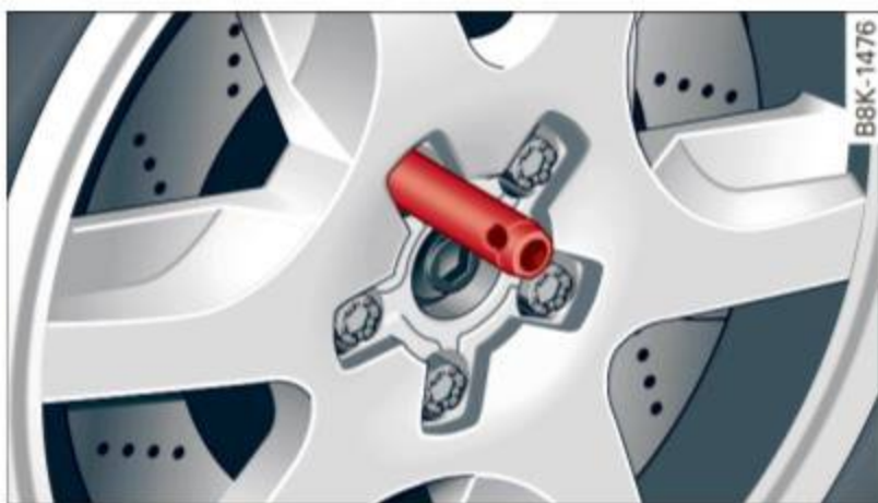
Fig. 182 Changing a wheel: alignment pin inside the top hole
