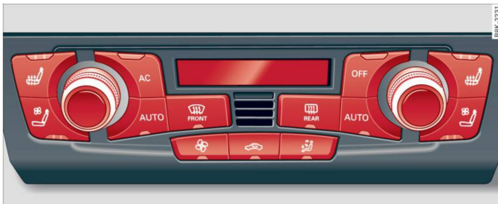
Fig. 72 3-zone deluxe automatic climate control*: controls
