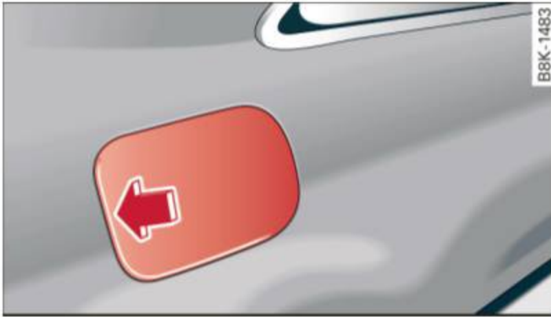
Fig. 155 Right rear vehicle side: Opening the fuel filler flap
