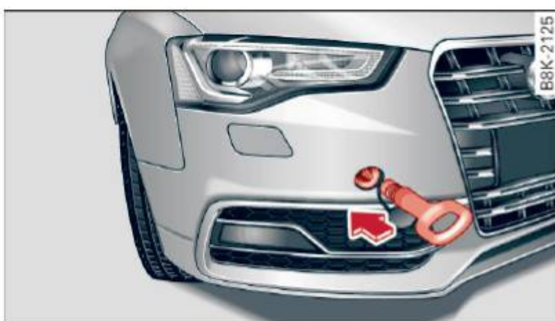
Fig. 190 Front bumper: screwing in the towing loop
