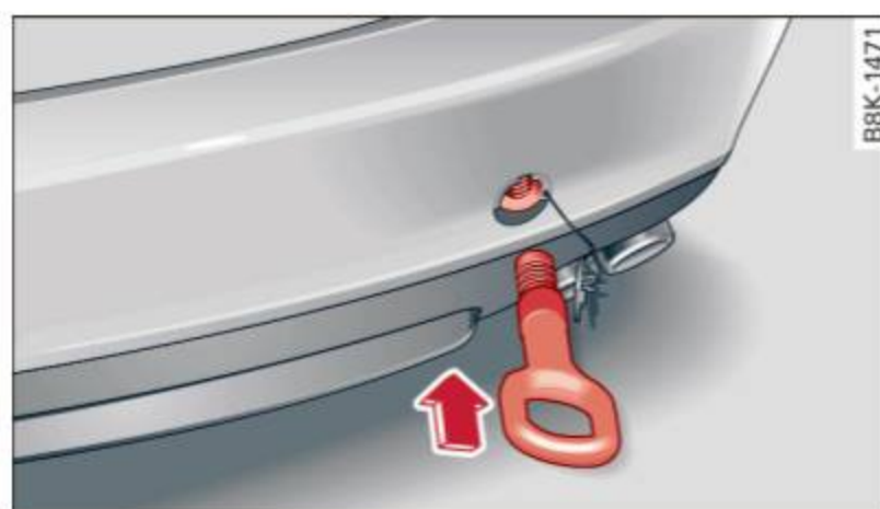
Fig. 192 Rear bumper: Screwing in towing loop
