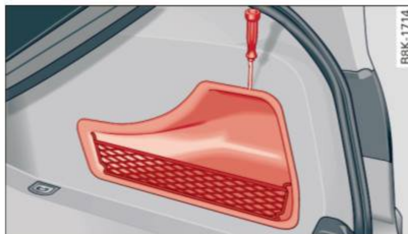
Fig. 157 Luggage compartment: opening the side trim
