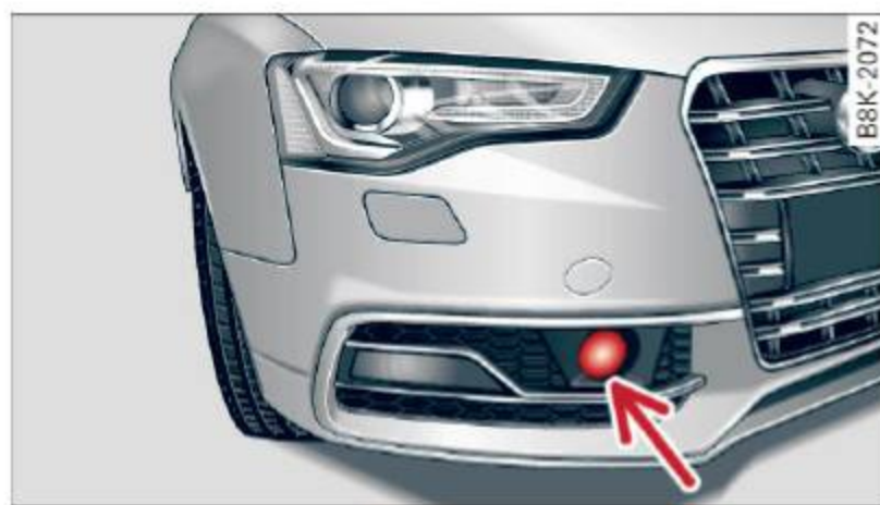
Fig. 90 Front of the vehicle: Position of radar sensor
