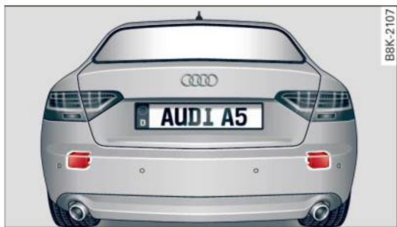
Fig. 104 Rear of the vehicle: position of the sensors
