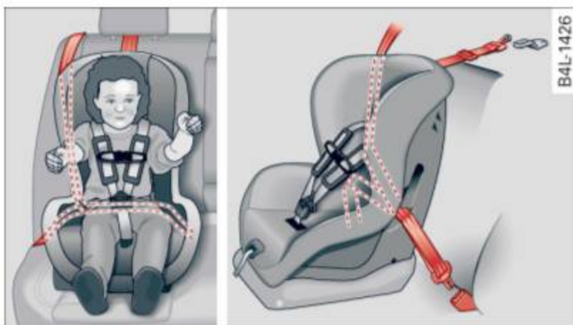
Fig. 145 Schematic overview: installation of the seat using the vehicle's safety belt system
