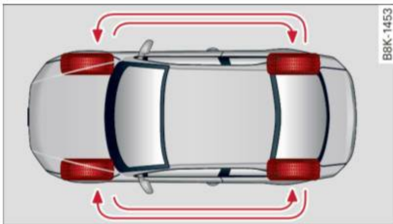
Fig. 171 Rotating tires for more even wear
