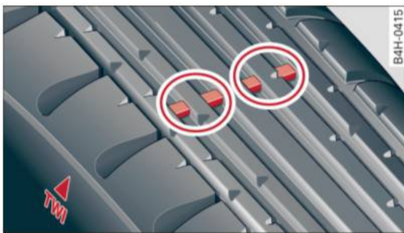
Fig. 170 Tire tread: tread wear indicators (TWI)
