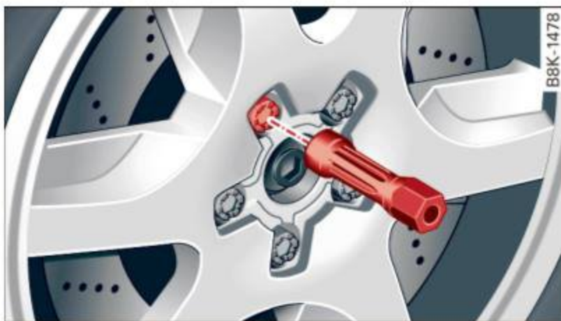
Fig. 181 Changing a wheel: using the screwdriver handle (with the blade removed) to turn the bolts
