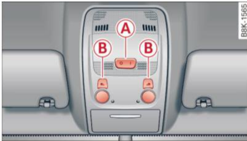
Fig. 37 Front headliner: interior lighting controls
