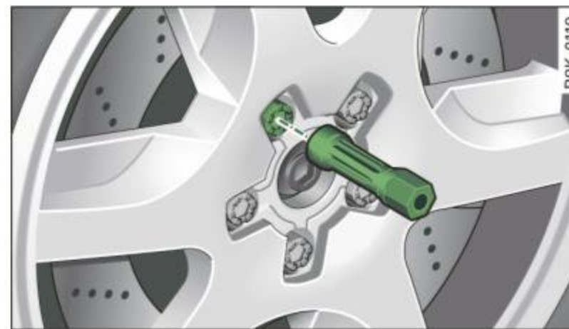
Fig. 226 Changing a wheel: using the screwdriver handle (with the blade removed) to turn the bolts
