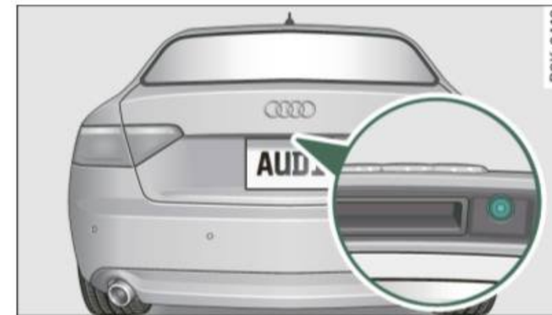
Fig. 156 Trunk lid: Location of the rear view camera
