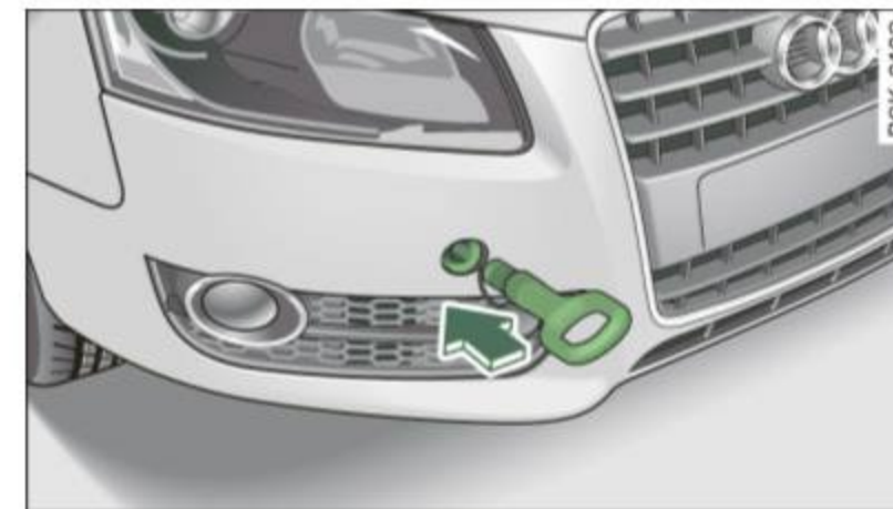
Fig. 235 Front bumper: screwing in the towing loop
