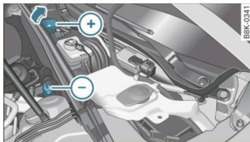
Fig. 210 Engine compartment: Connectors for charger and jumper cables
