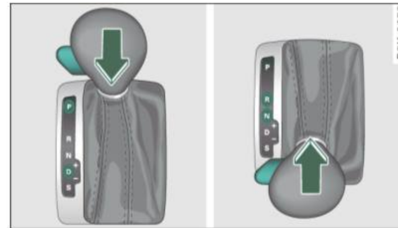
Fig. 147 Shift gate: selector lever lock positions and interlock button highlighted
