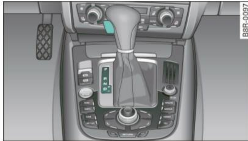
Fig. 145 Shift gate on the center console: selector lever with release button
