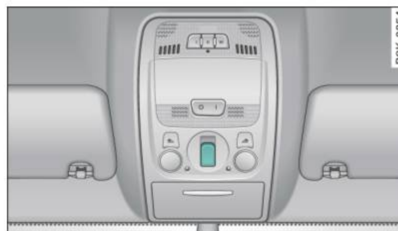
Fig. 47 Section of headliner: Switch for panoramic tilting sunroof
