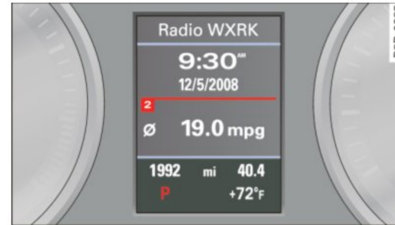
Fig. 146 Display in the instrument cluster: selector lever in position P
