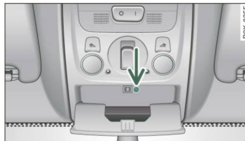
Fig. 48 Section of headliner: Unscrewing lighting unit
