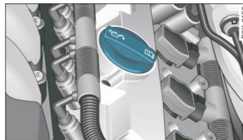
Fig. 207 Engine compartment: Oil filler cap location
