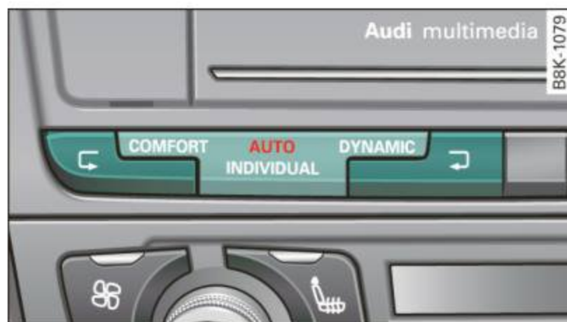
Fig. 143 Center console: Control for Audi drive select
