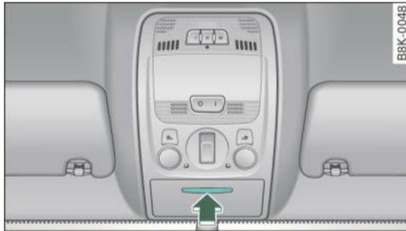
Fig. 95 Storage pocket in the roof
