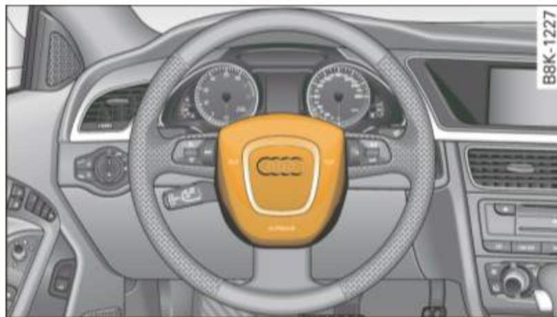
Fig. 177 Location of driver airbag: in steering wheel
