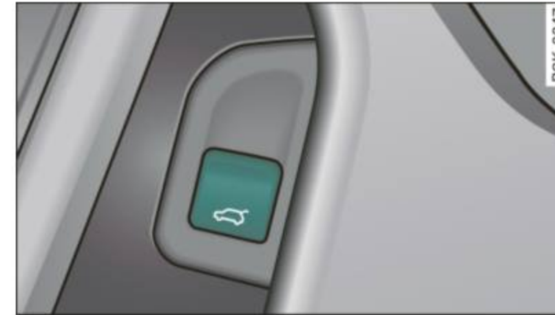
Fig. 41 Driver's door: remote rear lid release
