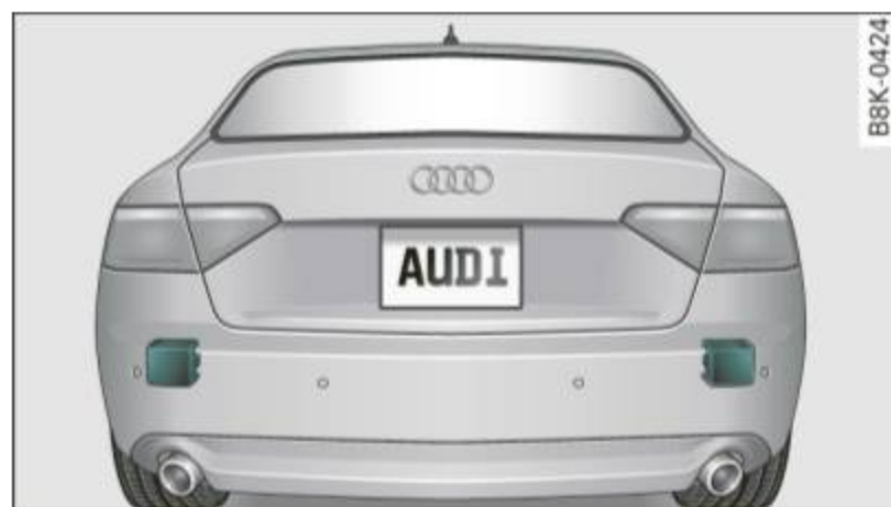
Fig. 132 Rear bumper: Position of radar sensors (not visible on outside)
