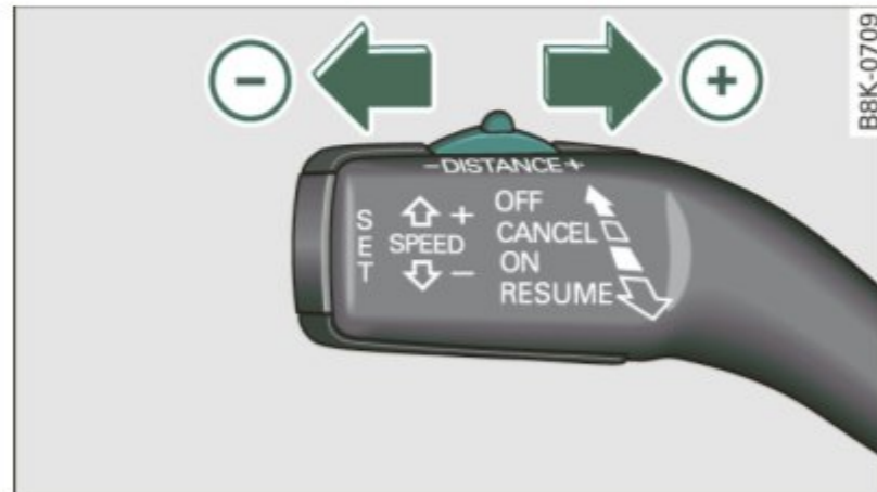
Fig. 118 Control lever: Setting distance
