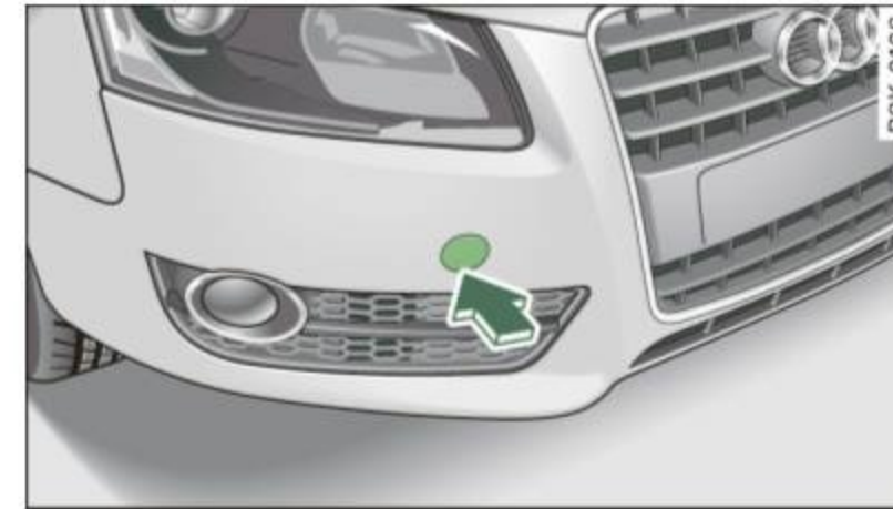
Fig. 234 Front bumper: removing the cover cap
