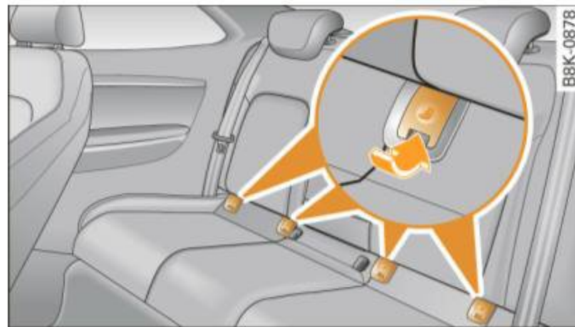
Fig. 192 Lower anchorages, covers marked
