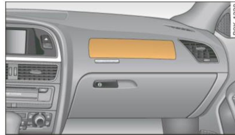
Fig. 178 Location of front passenger's airbag: in the instrument panel
