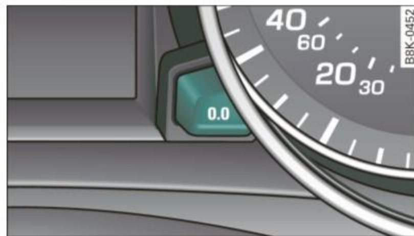
Fig. 6 Instrument cluster: reset button
