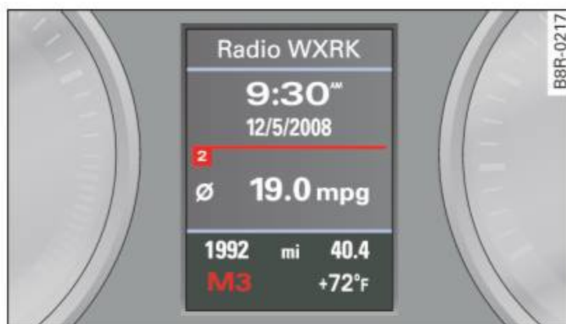
Fig. 149 Display: manual shift program, selected gear high-lighted
