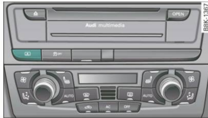
Fig. 59 with MMI: Button for rear window sun shade
