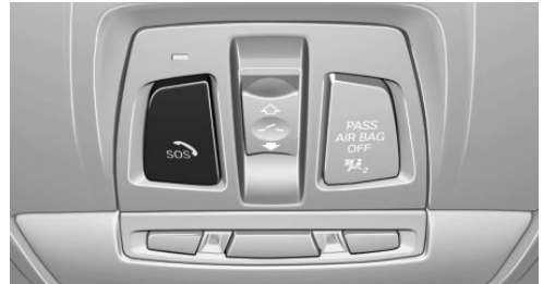
SOS button in the roofliner
