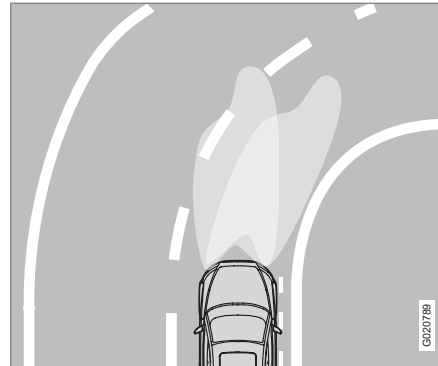
Headlamp pattern for active/non-active headlamps.
