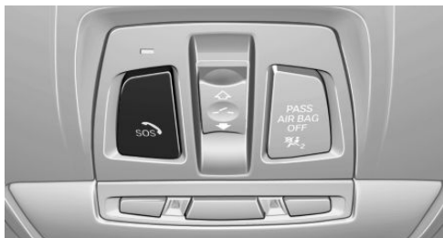
SOS button in the roofliner
