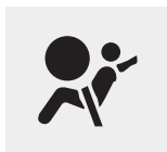
SRS warning light
