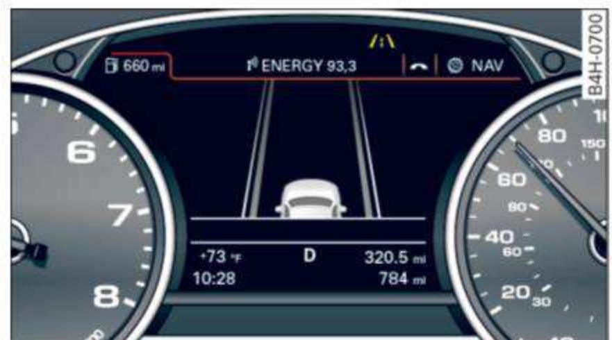
Fig. 103 Instrument cluster: active lane assist is switched on but not ready to provide warnings
