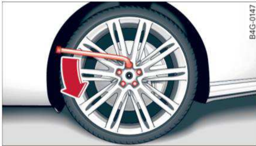
Fig. 200 Changing a wheel: loosening the wheel bolts
