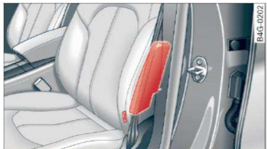
Fig. 159 Side airbag location in the driver's seat
