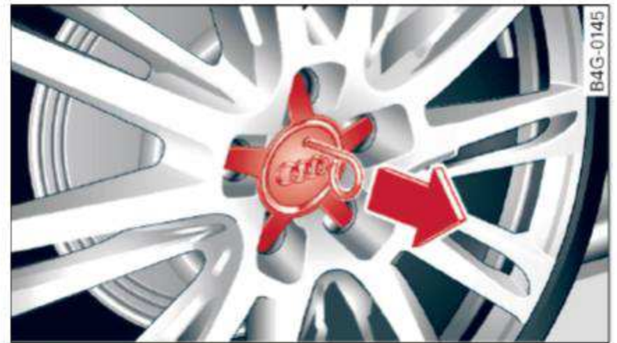
Fig. 198 Changing a wheel: Removing the wheel cover
