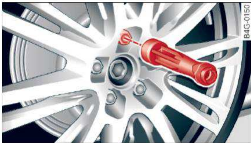
Fig. 204 Changing a wheel: using the screwdriver handle (with the blade removed) to turn the bolts
