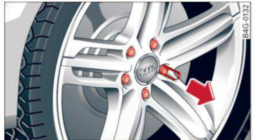
Fig. 199 Changing a wheel: removing the wheel bolt caps
