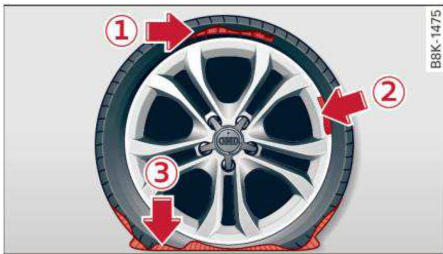
Fig. 195 Tire: tire damage that cannot be repaired
