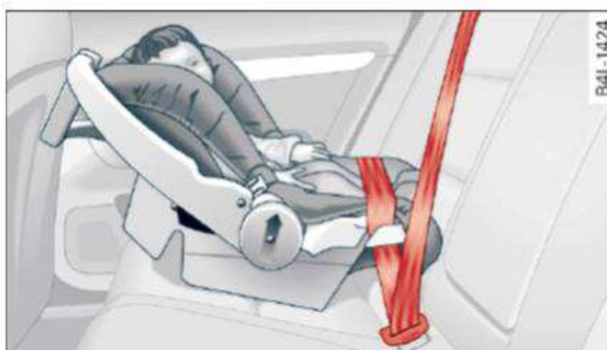
Fig. 164 Schematic overview: rearward-facing infant seat, properly installed on the rear seat
