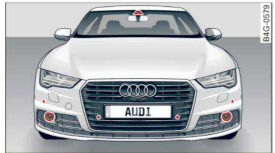
Fig. 90 Front of the vehicle: sensors and video camera
