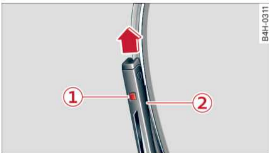
Fig. 44 Removing windshield wiper blades
