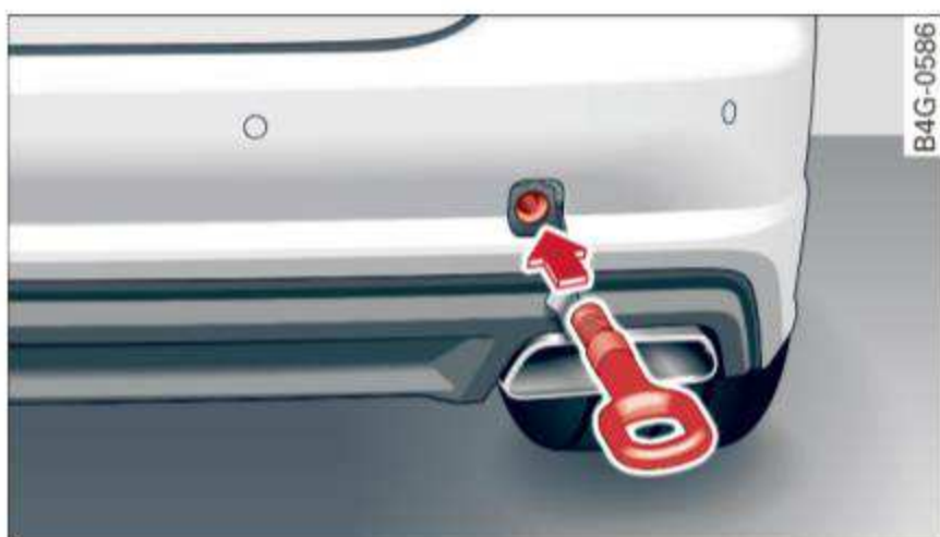
Fig. 216 Rear bumper: installing the towing loop
