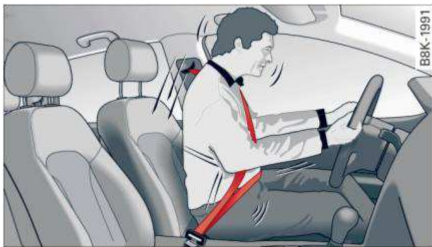
Fig. 147 Driver is correctly restrained in a sudden braking maneuver
