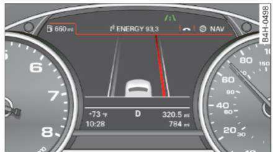
Fig. 102 Instrument cluster: active lane assist is switched on and providing warnings
