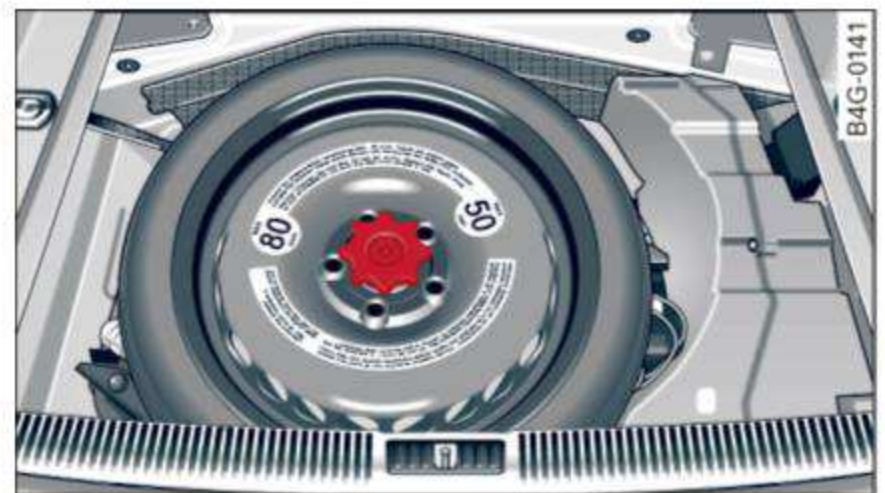
Fig. 206 Luggage compartment: space-saving spare tire
