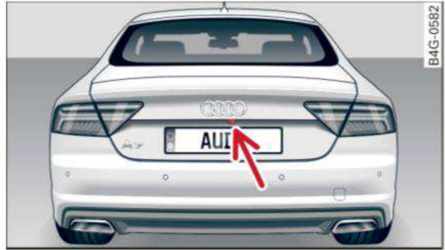
Fig. 120 Luggage compartment lid: location of the rearview camera
