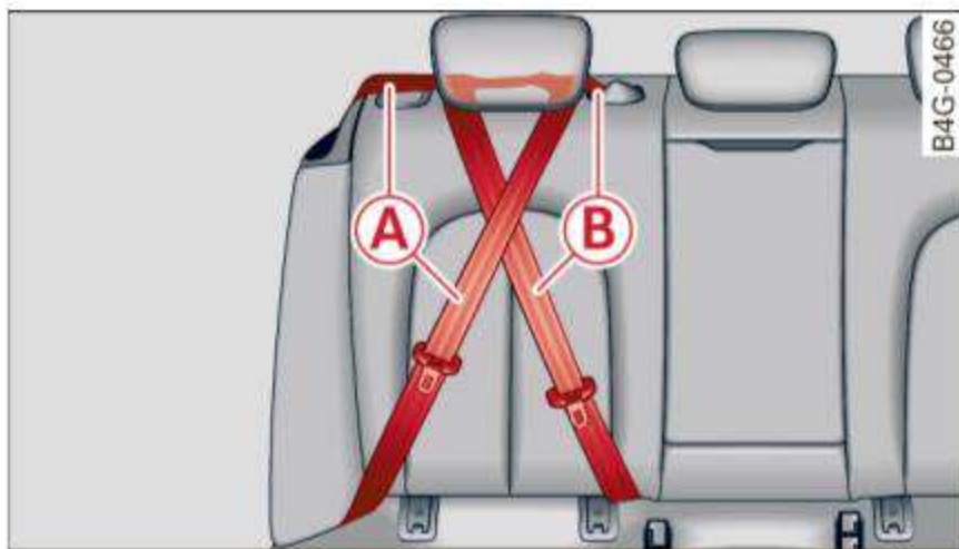
Fig. 163 Schematic overview: keep unused safety belts away from children in child safety seats. (A) - outer rear safety belt, (B) - center rear safety belt*
