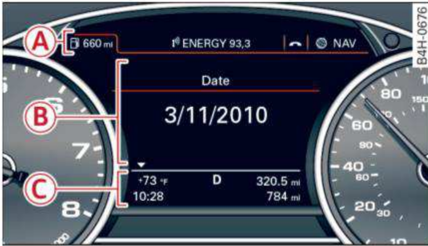
Fig. 4 Driver information system in the instrument cluster
