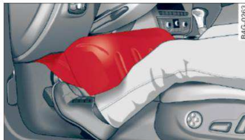
Fig. 158 Inflated airbags protecting in a frontal collision
