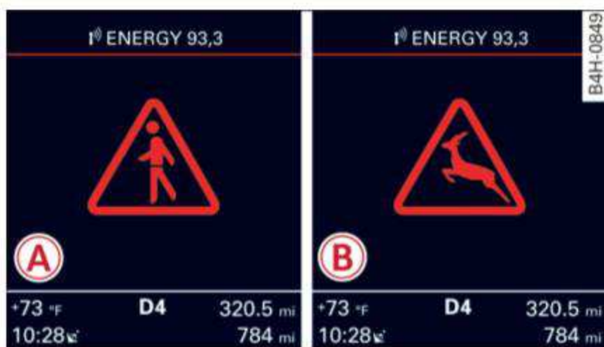
Fig. 112 Instrument cluster: (A) pedestrian warning/(B) wild animal warning, when the night vision assist image is not selected in the instrument cluster display
