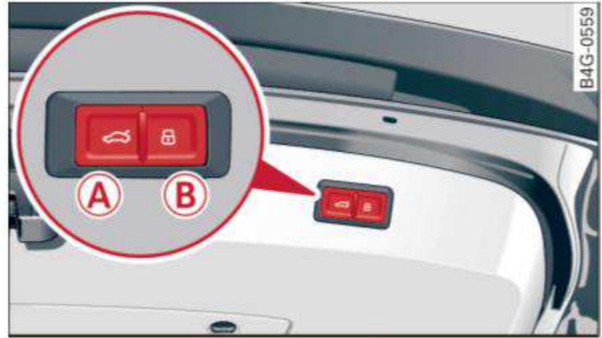
Fig. 25 Luggage compartment lid: (A) closing button, (B) lock button (vehicles with convenience key*)
