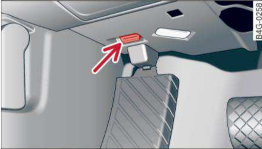
Fig. 178 Footwell on left side of the vehicle: connection port for the On-Board Diagnostic System (OBD)
