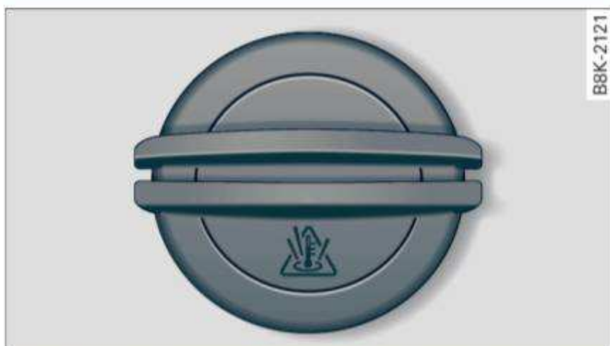
Fig. 183 Engine compartment: coolant expansion tank cover
