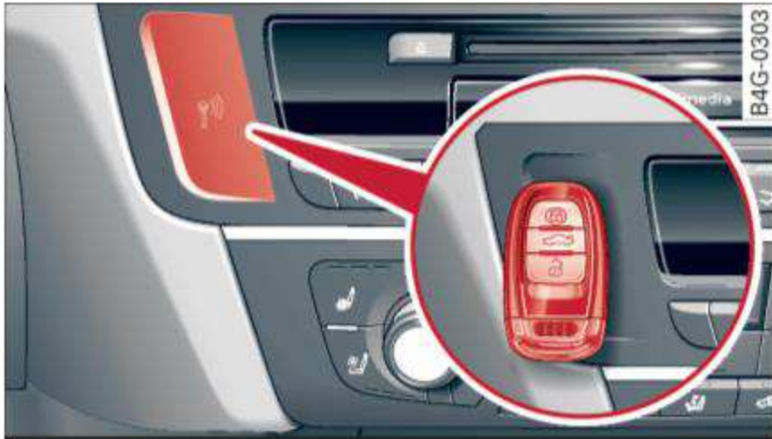
Fig. 77 Center console/remote control key: starting the engine if there is a malfunction
