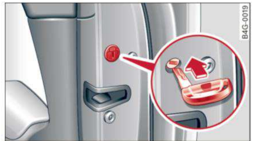
Fig. 23 Door: emergency locking
