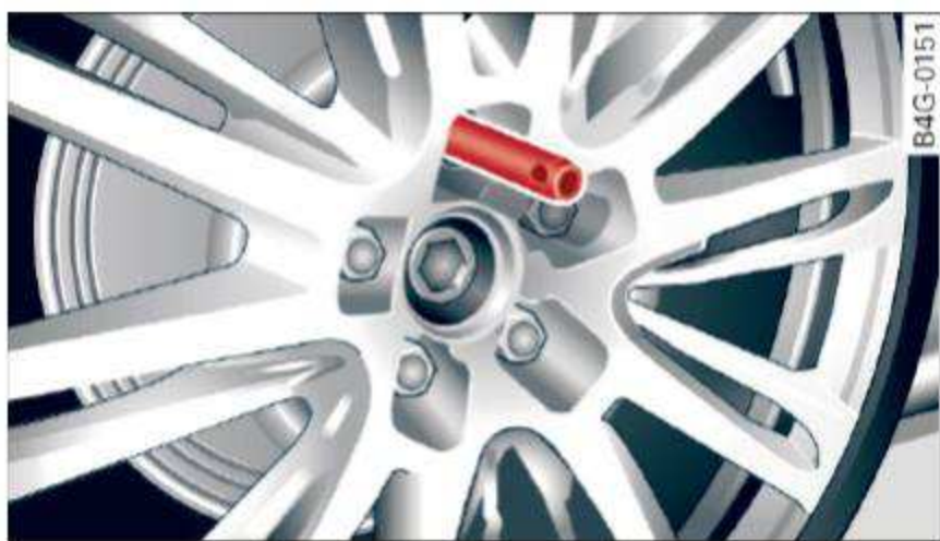
Fig. 205 Changing a wheel: alignment pin inside the top hole
