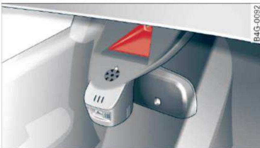
Fig. 101 Windshield: camera window for active lane assist
