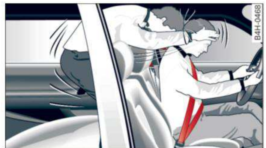
Fig. 146 A rear passenger not wearing a safety belt will fly forward and strike the driver
