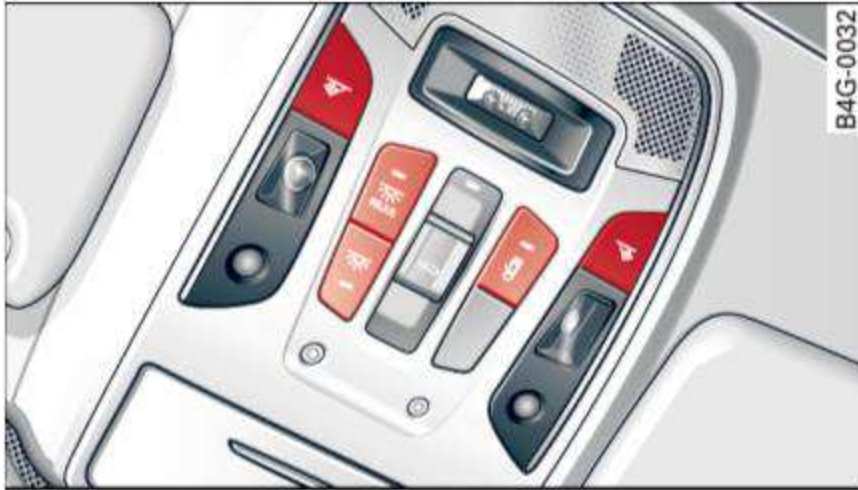
Fig. 36 Front headliner: interior lighting controls
