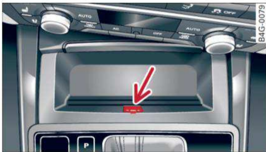
Fig. 85 Front center console: emergency release for the selector lever
