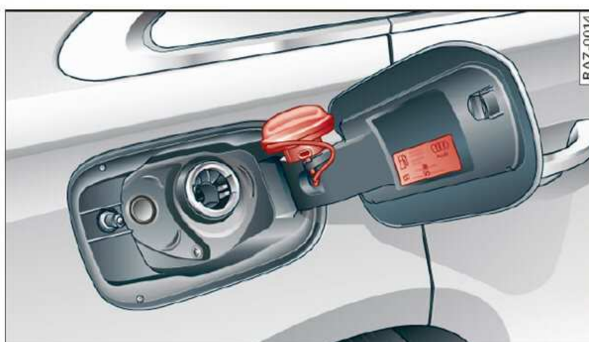
Fig. 138 Fuel filler door with attached fuel cap
