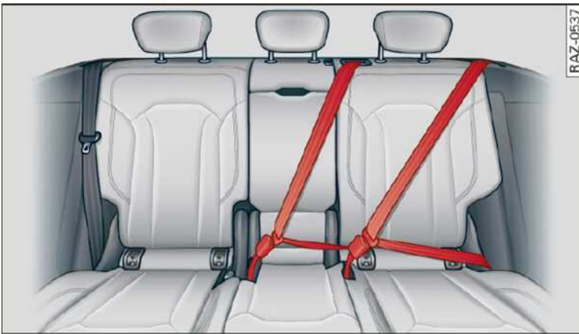
Fig. 68 Rear bench seat: securing unused safety belts
