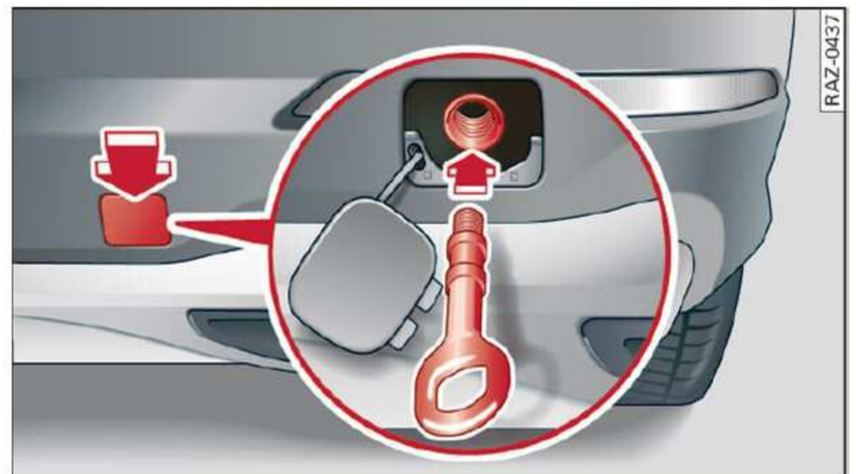
Fig. 165 Rear bumper: installing the towing loop
