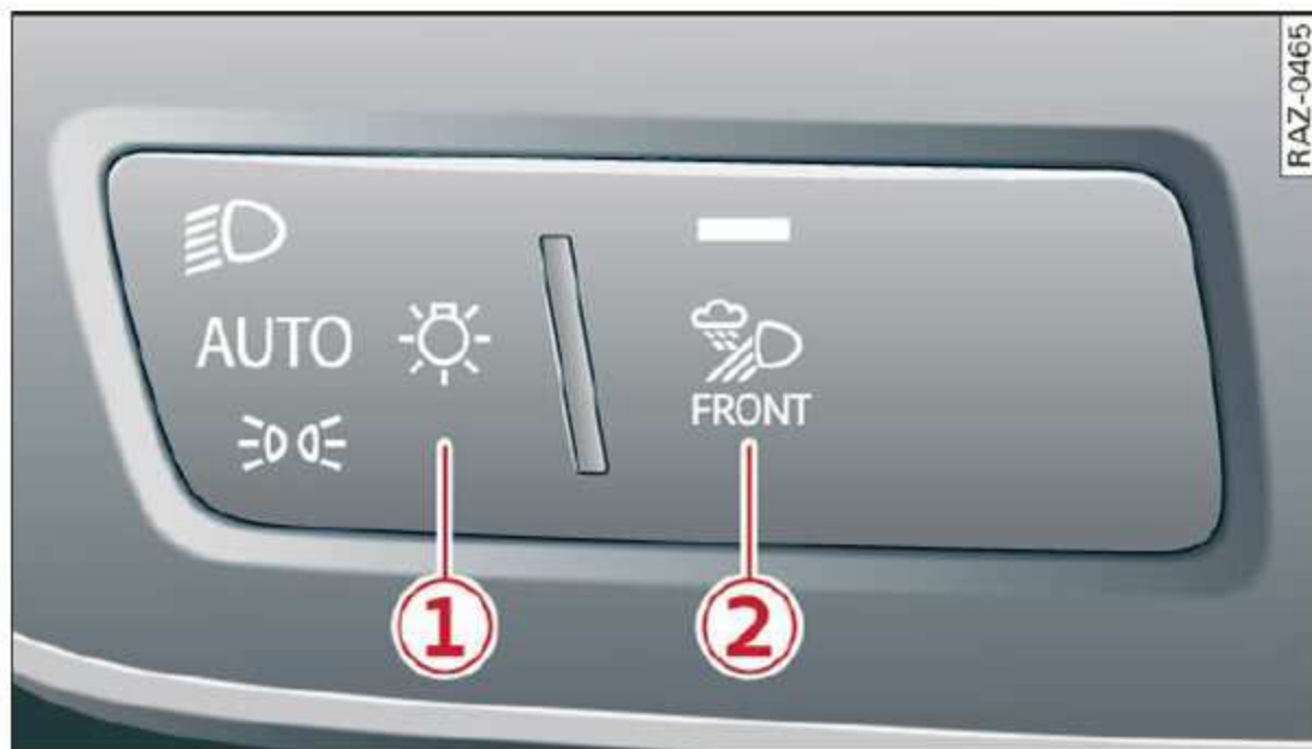
Fig. 37 Instrument panel: light switch module
