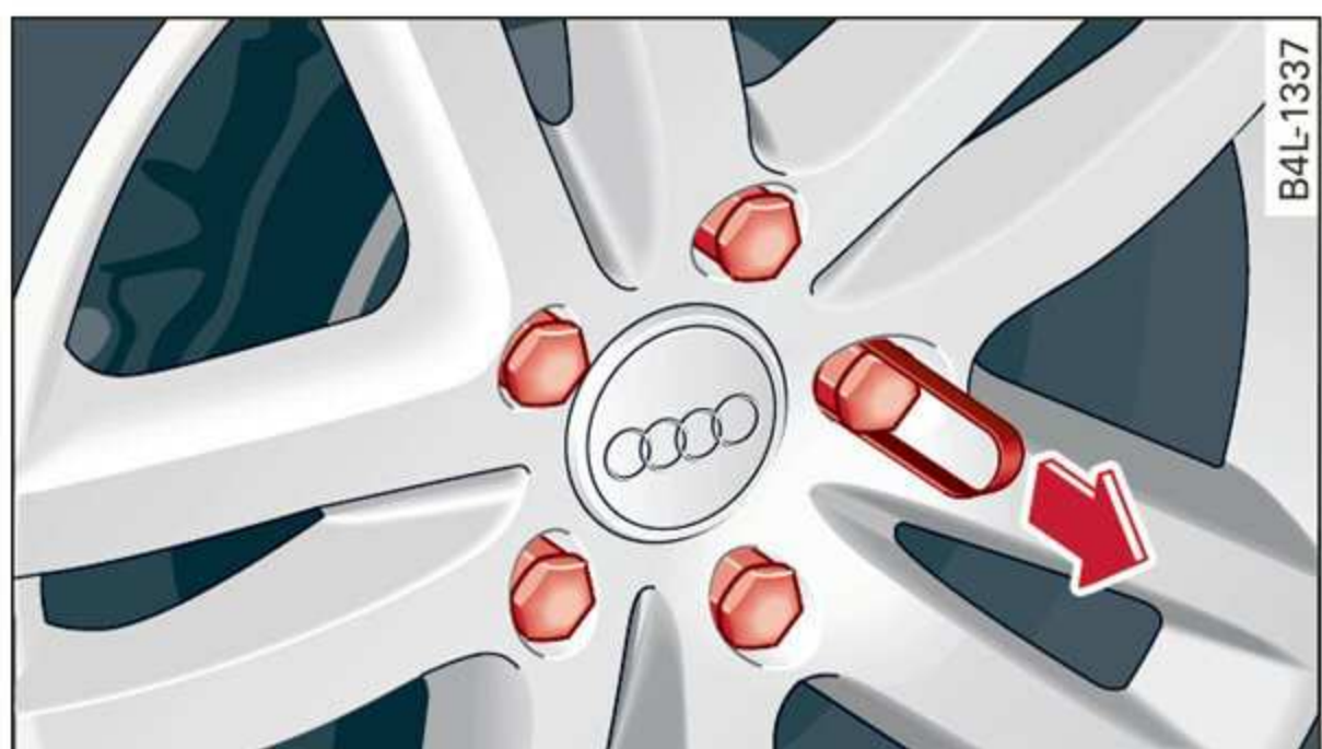
Fig. 154 Wheel: Wheel bolts with caps
