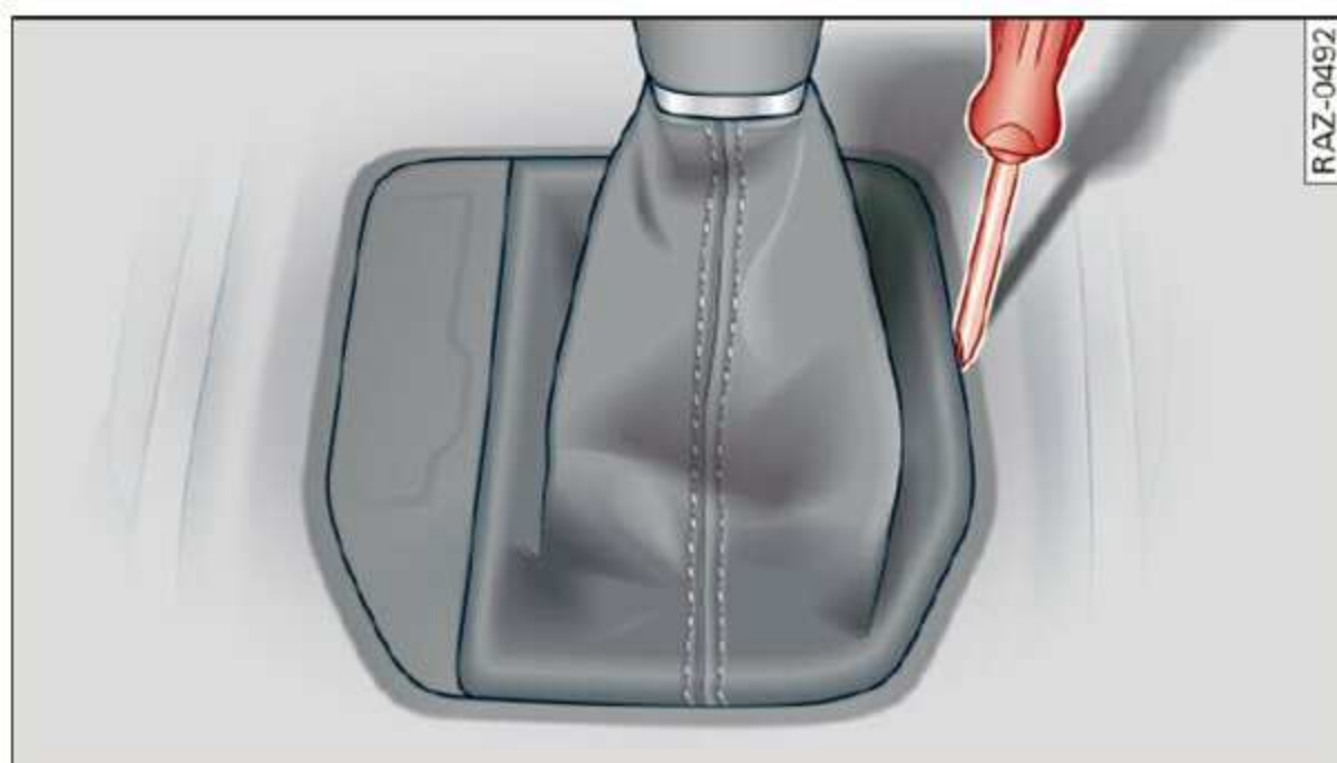
Fig. 84 Selector lever: Removing the shifter boot
