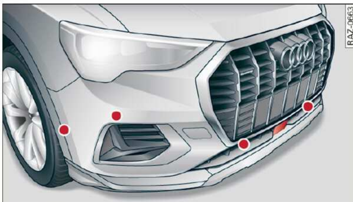
Fig. 87 Positions of the outer front sensors
