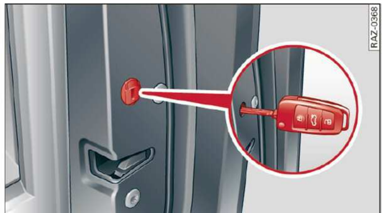
Fig. 23 Door: Emergency locking
