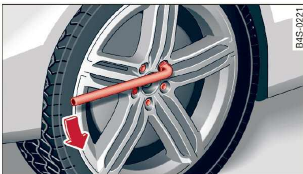
Fig. 156 Wheel: Loosening the wheel bolts
