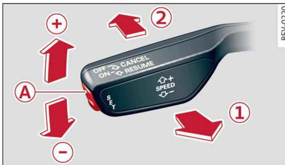
Fig. 91 Operating lever: Switching on the cruise control system
