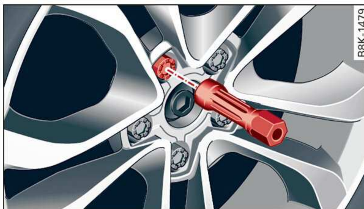
Fig. 159 Wheel: internal hex socket to turn the wheel bolts
