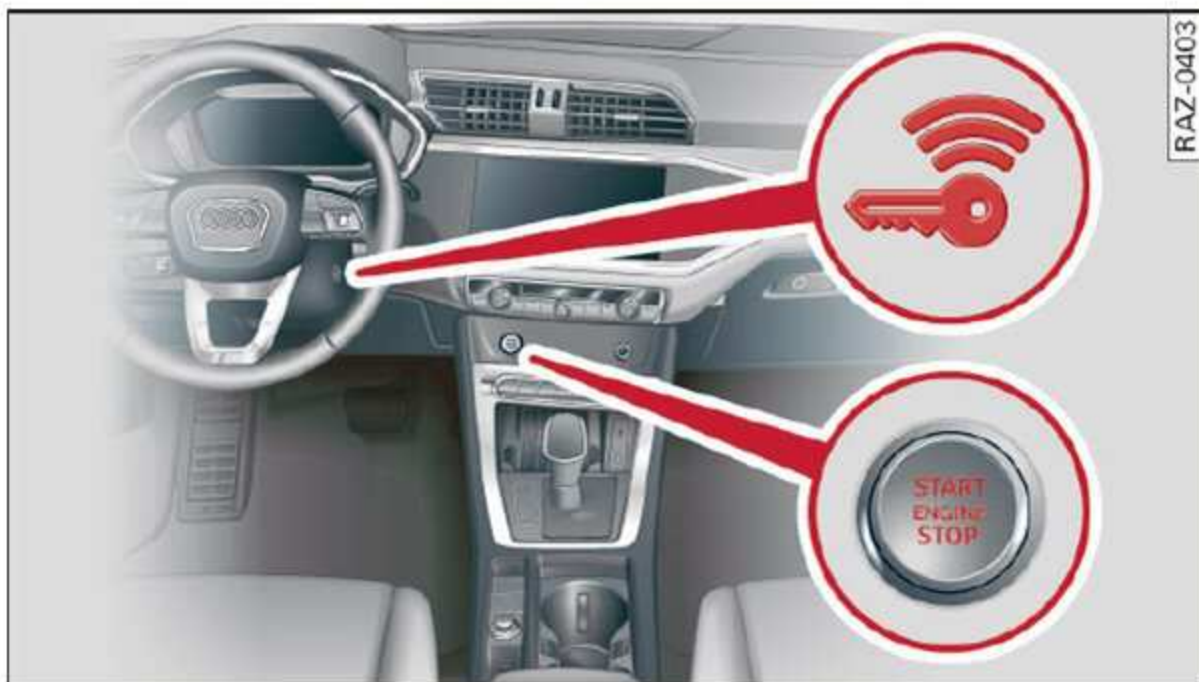
Fig. 79 Center console: Starting the engine
