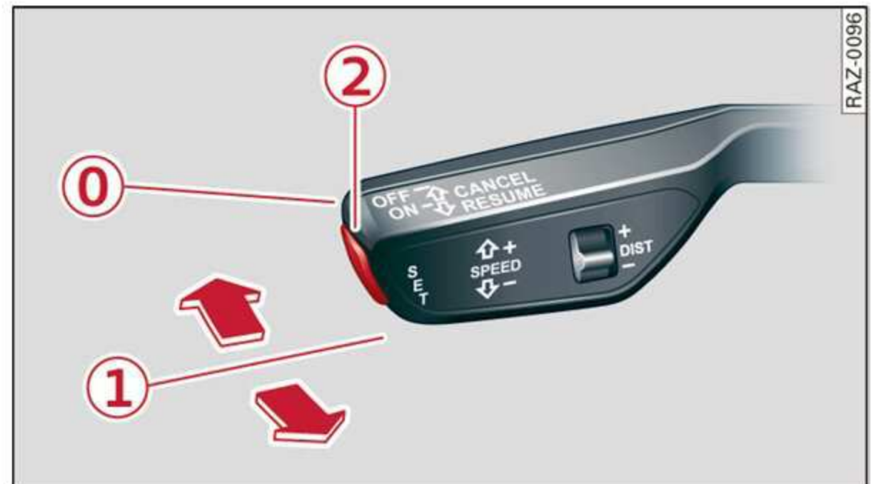
Fig. 99 Operating lever: Overriding control
