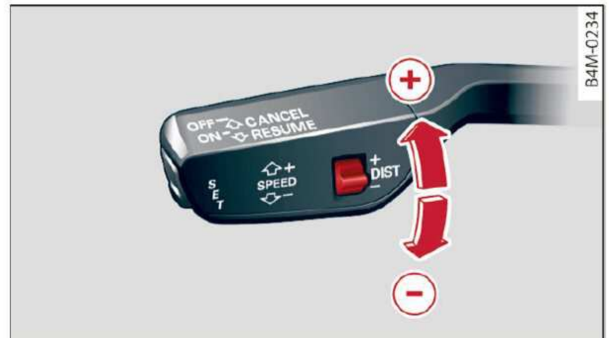
Fig. 98 Operating lever: Setting the distance
