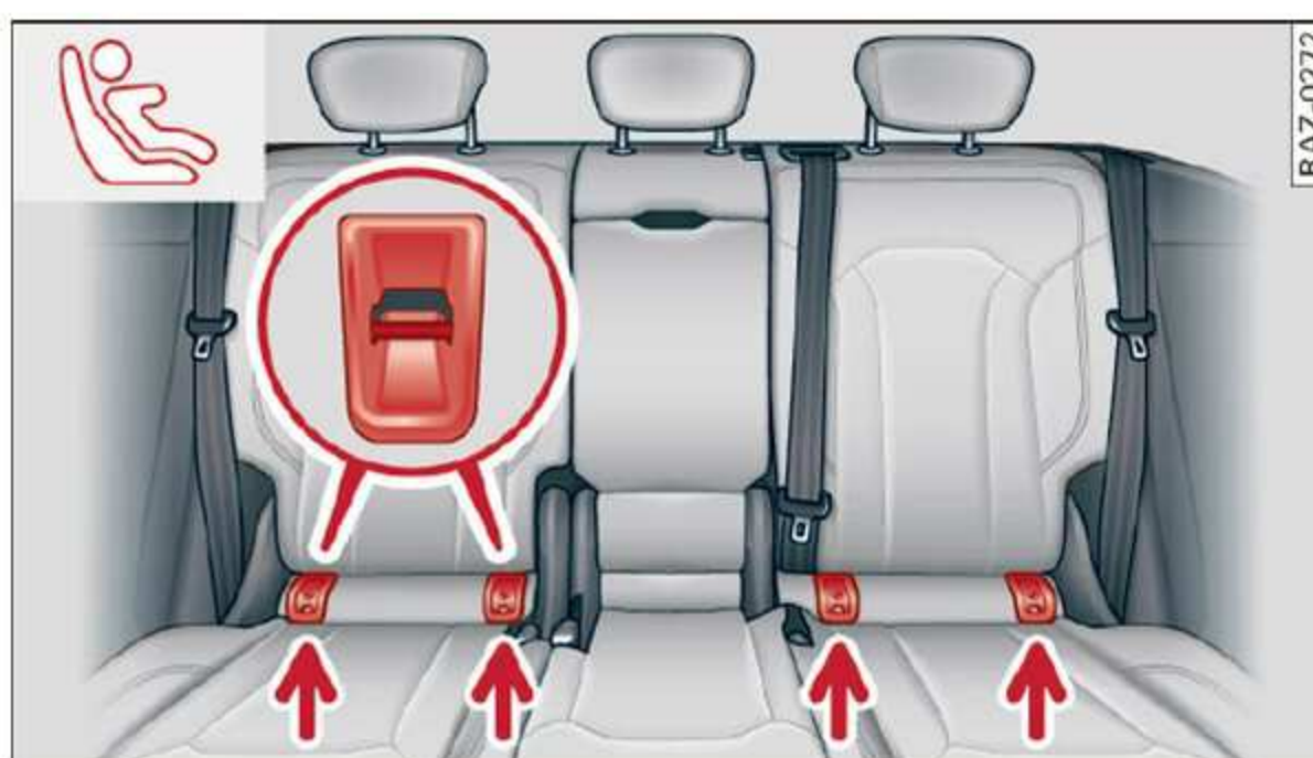
Fig. 65 Rear bench seat: lower LATCH anchors
