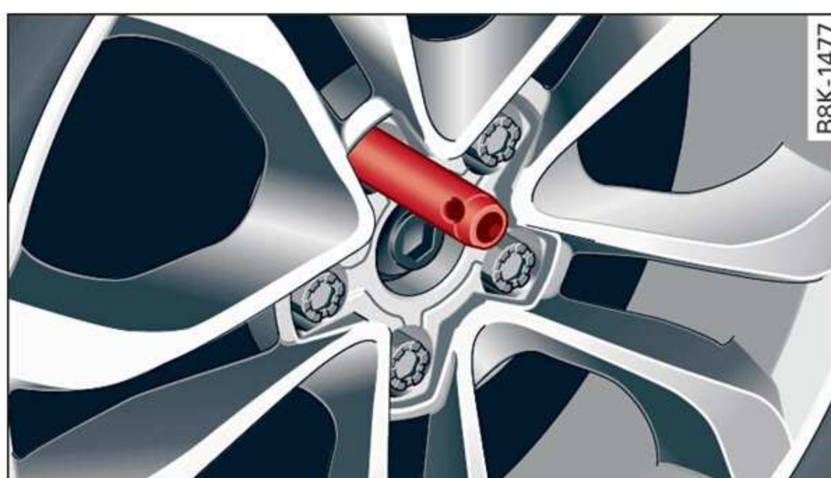
Fig. 160 Wheel: alignment pin in the top hole
