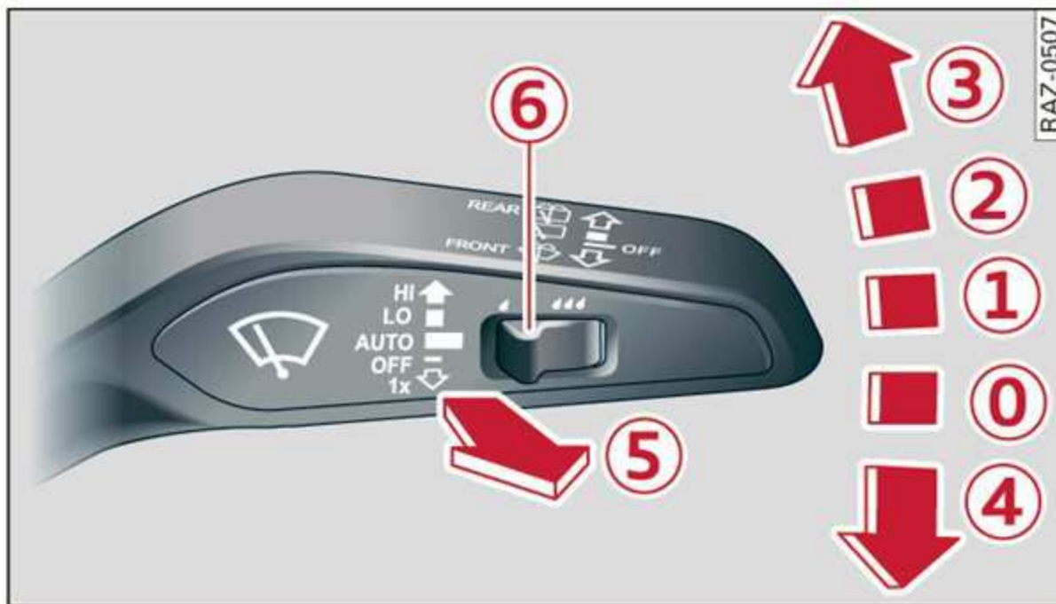
Fig. 44 Operating lever: Windshield wipers
