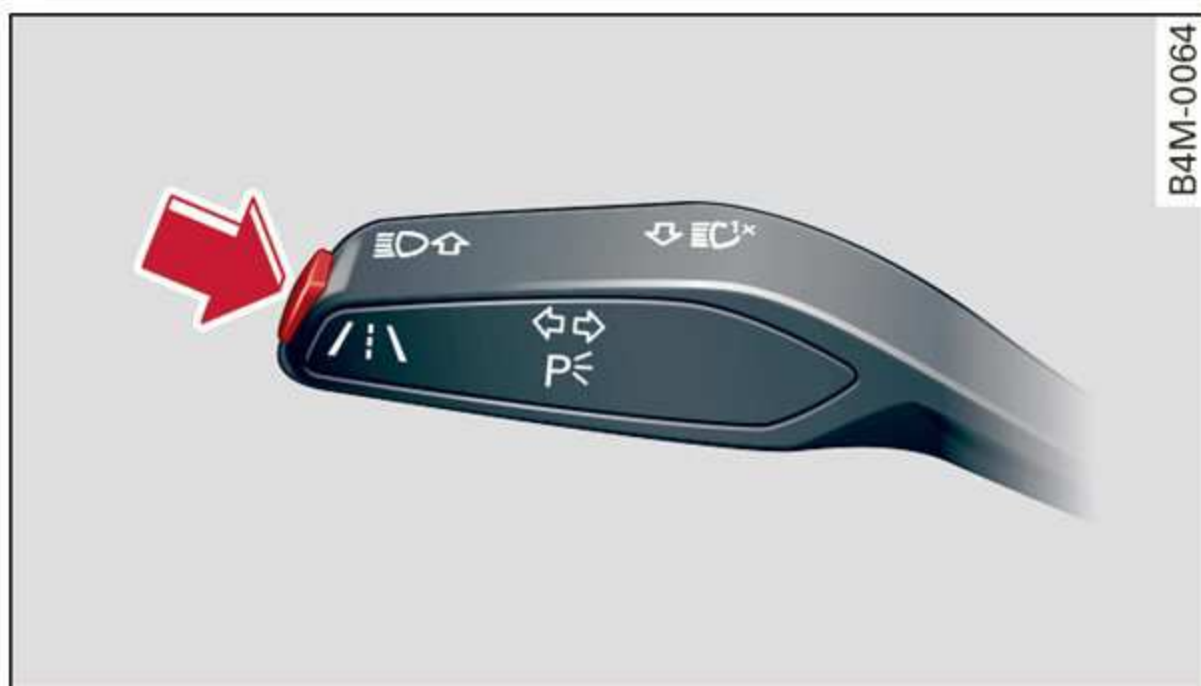
Fig. 104 Turn signal lever: Switches the lane departure warning on or off
