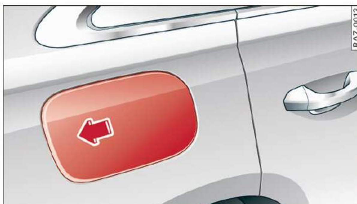
Fig. 137 Right rear side of the vehicle: opening the fuel filler door
