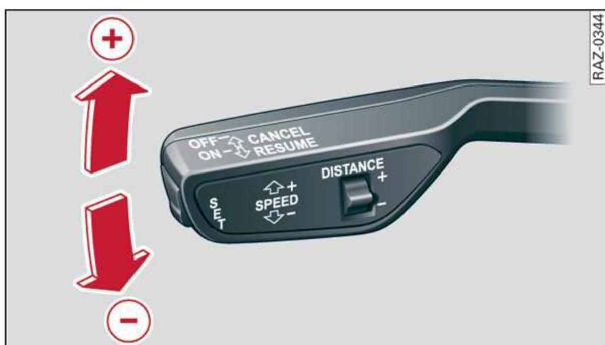
Fig. 97 Operating lever: Changing the speed
