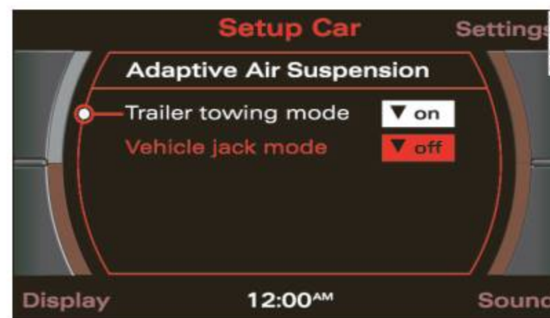
Fig. 184 MMI display: Activate towing operation
