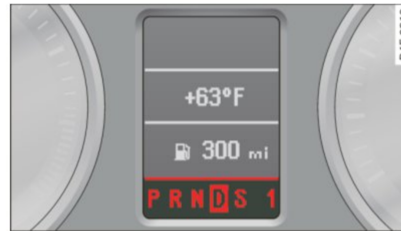
Fig. 151 Display in the instrument cluster: selector lever in position D
