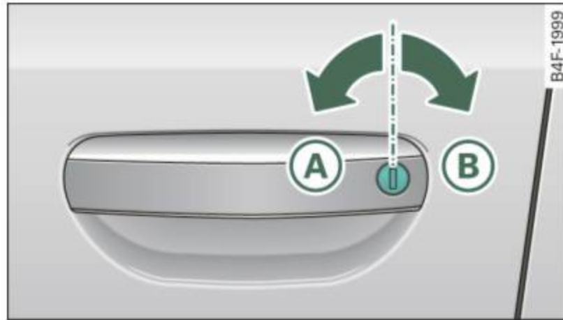
Fig. 35 Key turns for opening and closing.
