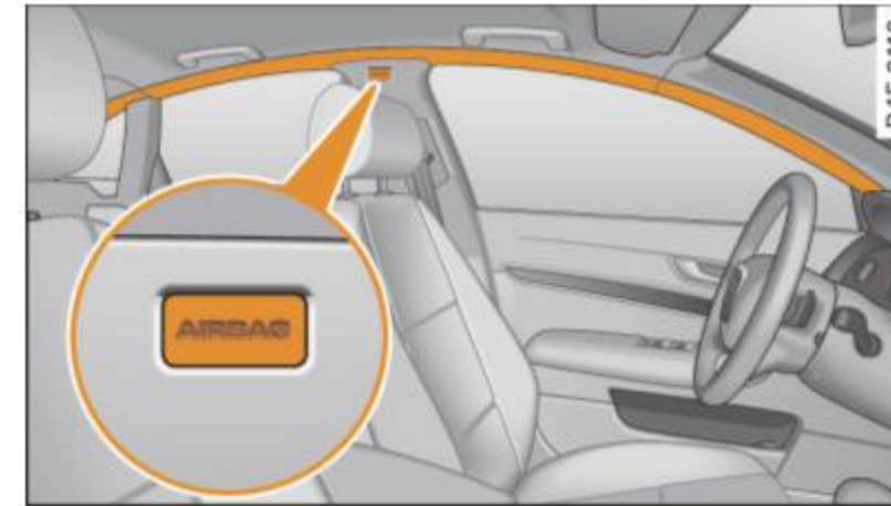
Fig. 209 SIDEGUARD™ system, driver's side: side curtain airbag location
