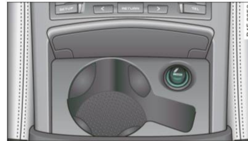
Fig. 102 Open front beverage storage compartment with cigarette lighter
