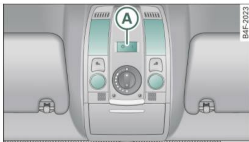
Fig. 61 Headliner: Front interior lights
