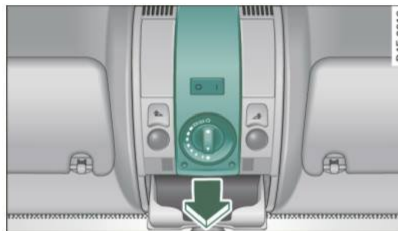
Fig. 50 Section from headliner: removing the cover
