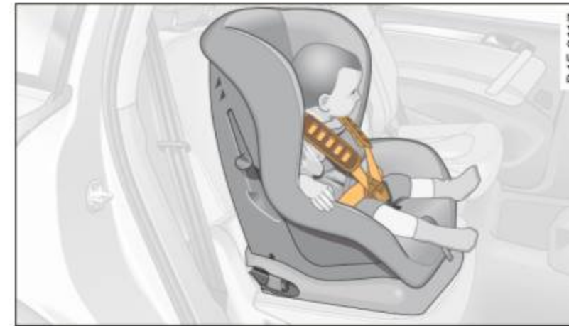
Fig. 212 Rear seat: smaller child in a properly installed forward-facing convertible child safety seat
