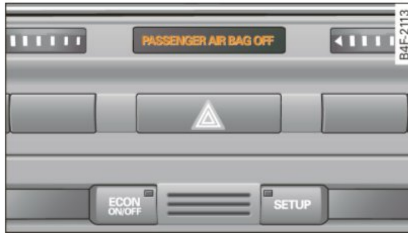
Fig. 206 Section from the instrument panel: PASSENGER AIR BAG OFF light
