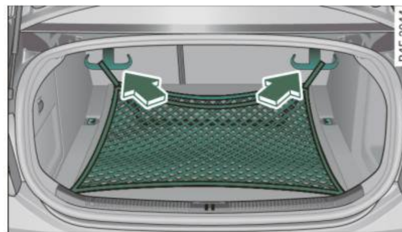
Fig. 91 Luggage compartment cargo net attached to mounting hooks*
