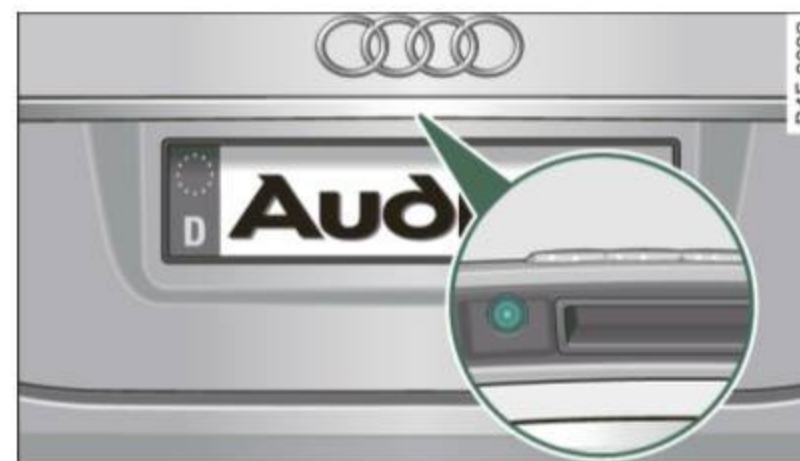
Fig. 167 Rear lid: Location of the rear-view camera
