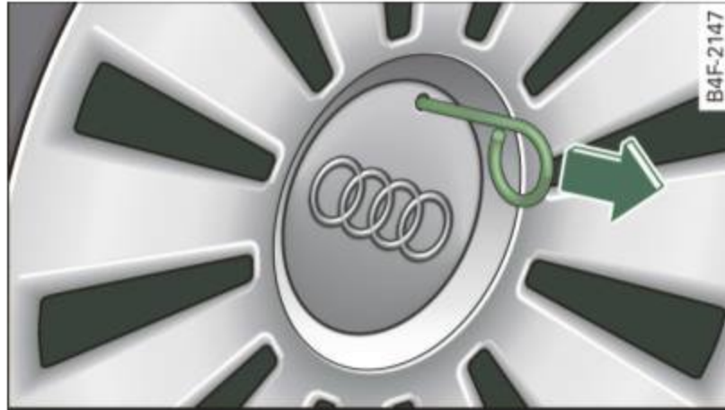
Fig. 249 Changing a wheel: Removing the wheel cover
