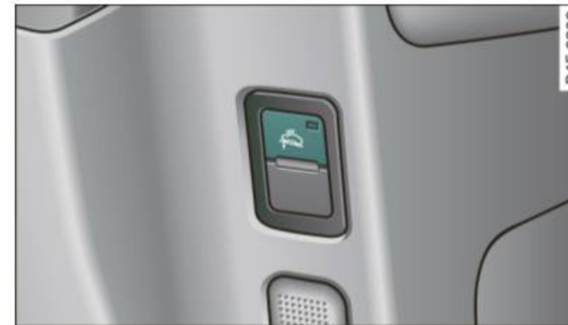
Fig. 45 Driver's door: tilt sensor switch
