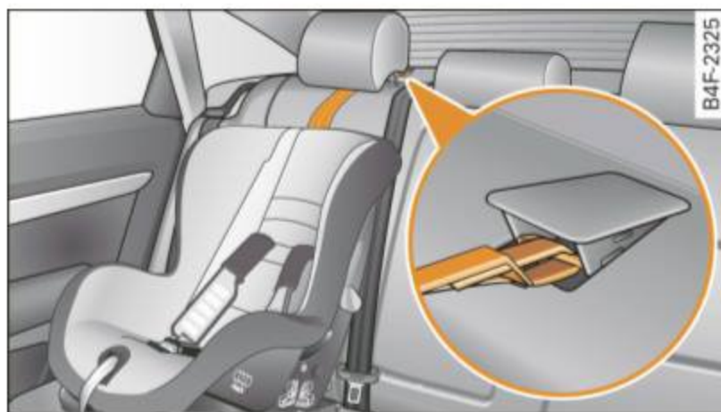
Fig. 223 Tether strap: proper routing and mounting
