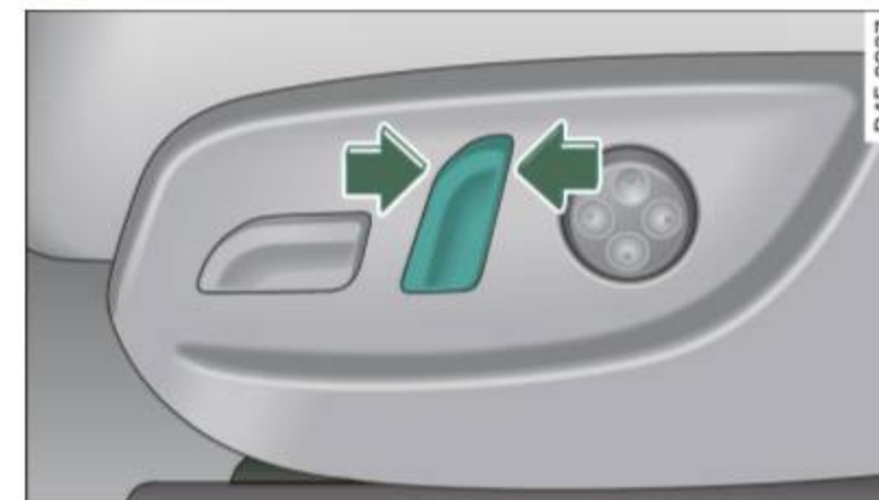
Fig. 79 Power seat: Switch for seat back angle
