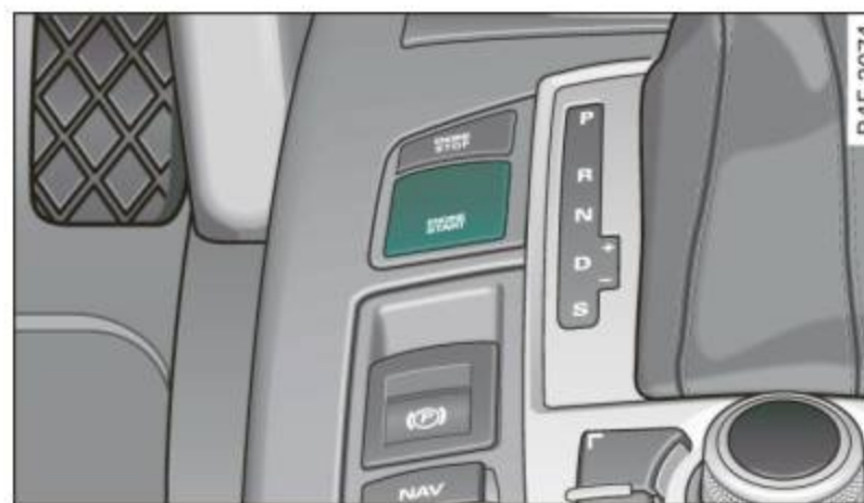
Fig. 124 Advanced Key: ENGINE START button
