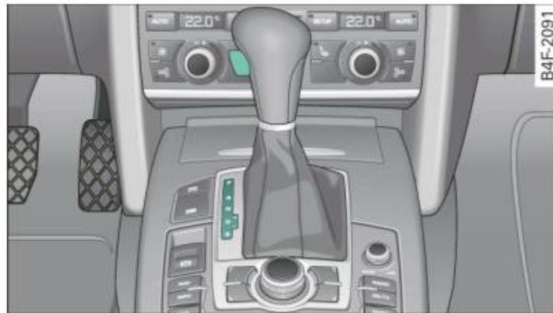
Fig. 150 Shift gate on the center console: selector lever with release button
