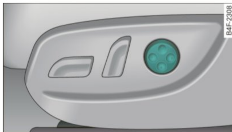
Fig. 80 Power seat: Switch shell for lumbar support
