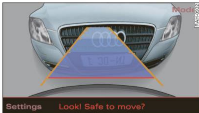
Fig. 177 MMI Display: displayed red line touches the bumper
