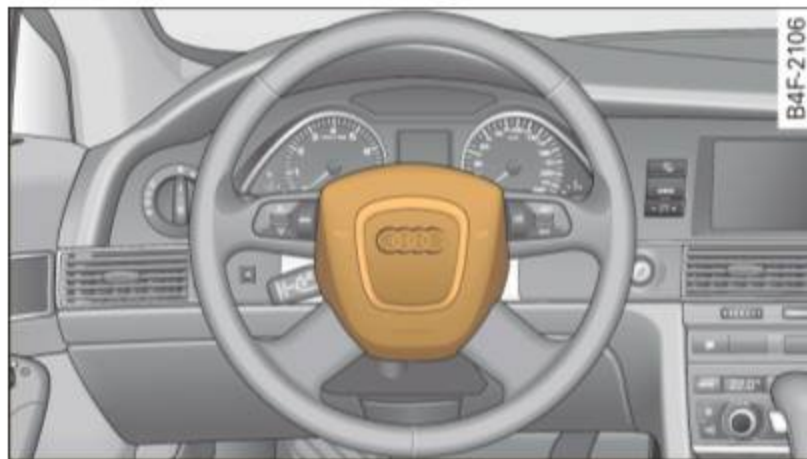
Fig. 203 Location of driver airbag: in steering wheel
