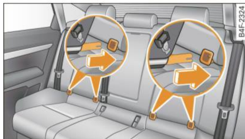
Fig. 221 Installation of child safety seat with rigid latches on bars
