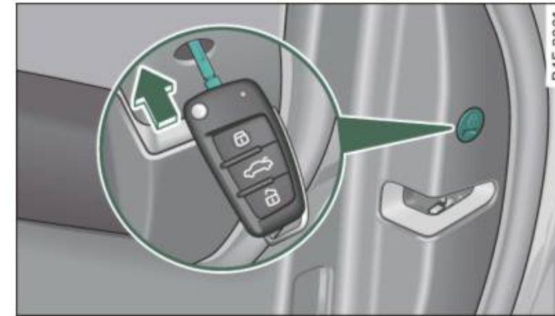
Fig. 39 Emergency locking of the front passenger's door
