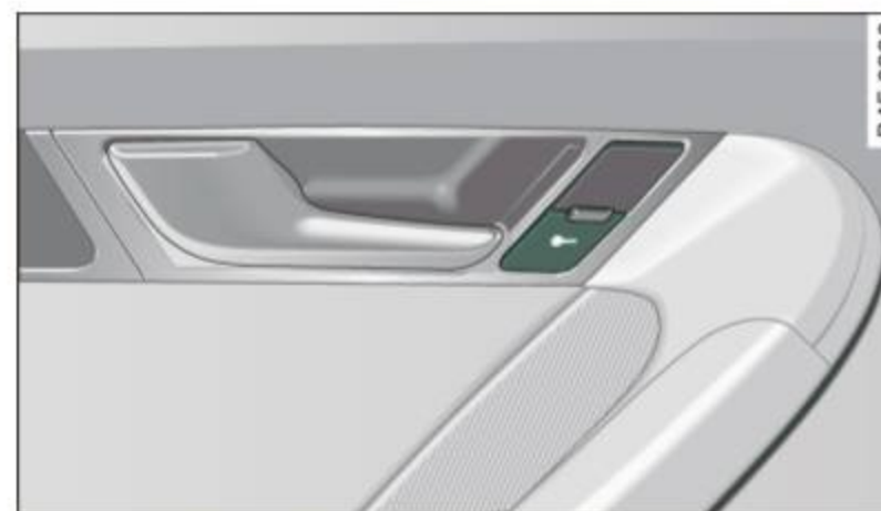
Fig. 38 Rear doors: power locking switch
