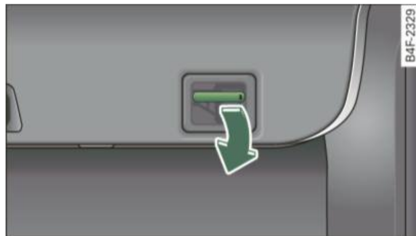
Fig. 245 Trunk escape handle: View from inside the closed trunk
