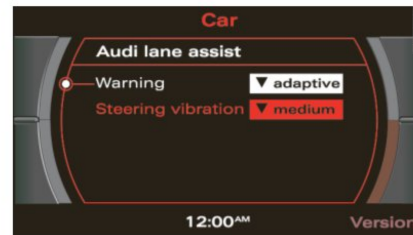
Fig. 149 MMI Display: Setting the warning time and steering wheel vibration
