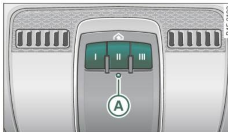
Fig. 185 Overhead console: HomeLink® keypad
