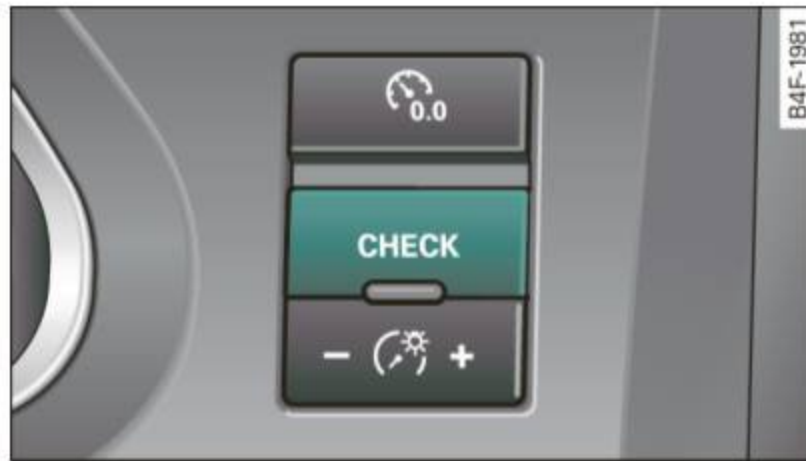
Fig. 20 CHECK button in the instrument cluster
