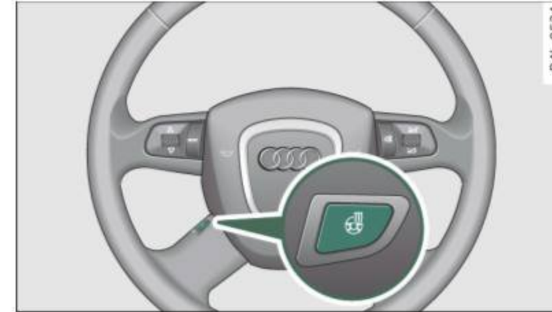
Fig. 113 Multifunction steering wheel: Button for steering wheel heating
