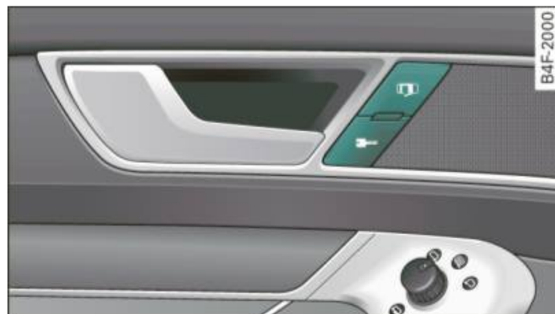
Fig. 37 Front doors: power locking switch
