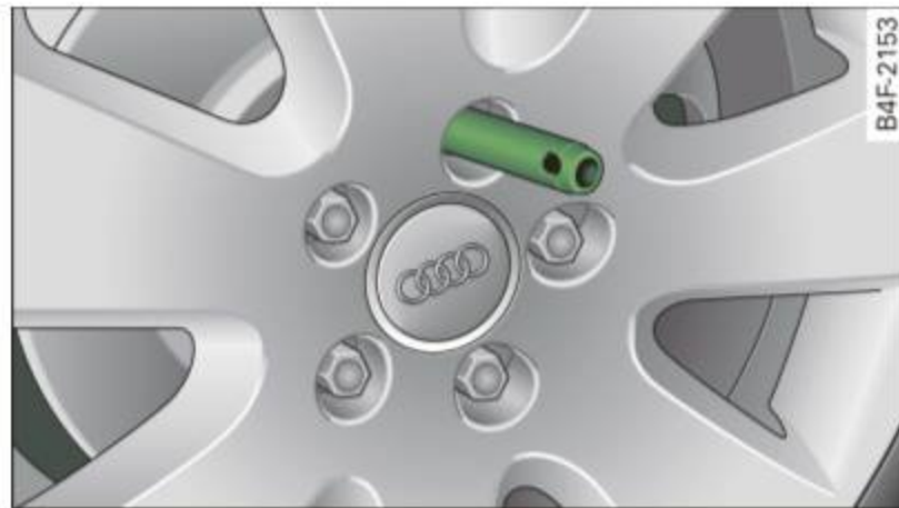
Fig. 255 Changing a wheel: alignment pin inside the top hole
