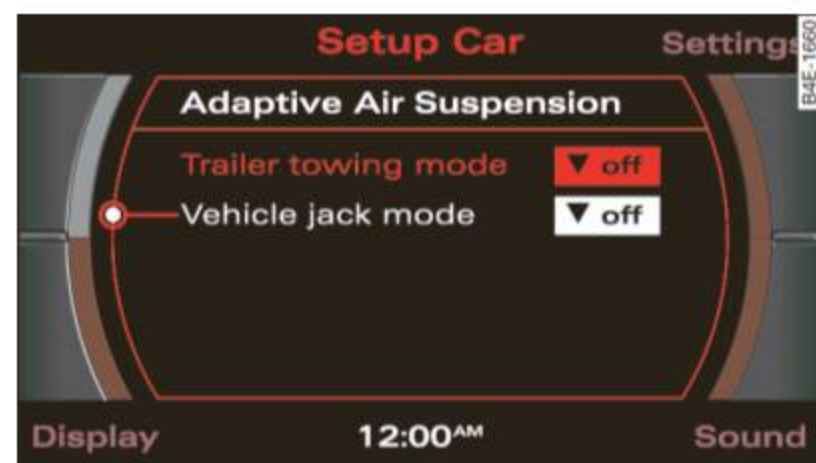
Fig. 183 MMI display: Activate jacking mode
