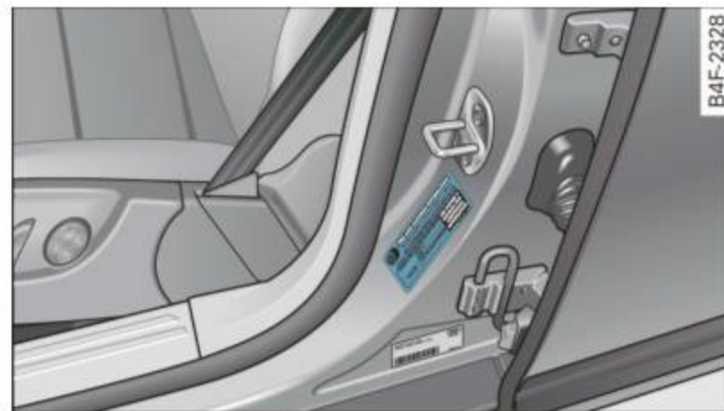
Fig. 240 Tire pressure label: located either on driver's side B-pillar or inside the fuel filler flap
