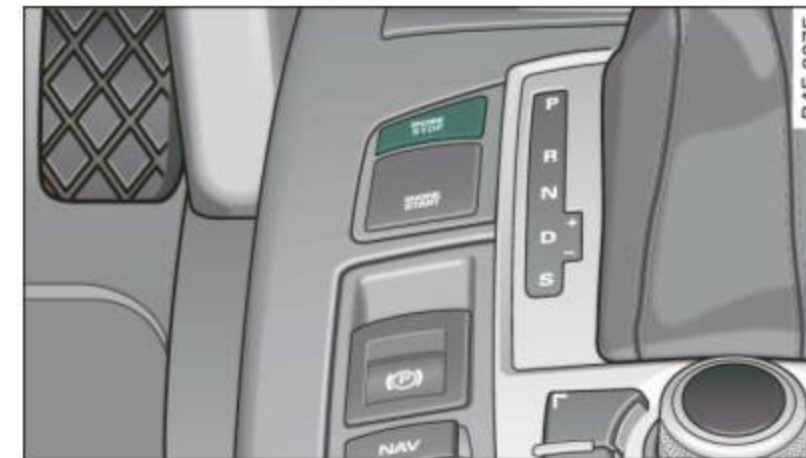
Fig. 125 Advanced Key: ENGINE STOP button
