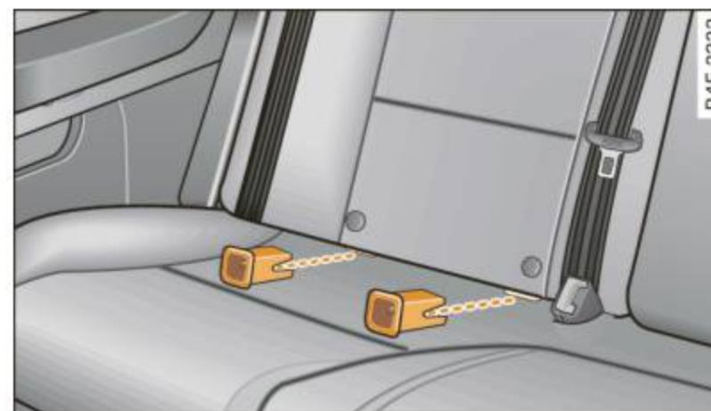
Fig. 218 Outer rear seats: installing the guidance fixtures
