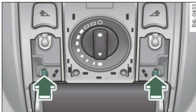
Fig. 52 Section from headliner: unscrewing the lighting unit
