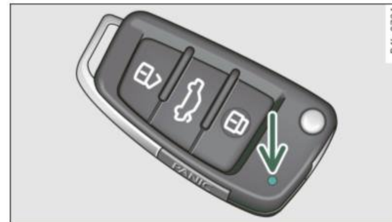
Fig. 31 Check light in the master key
