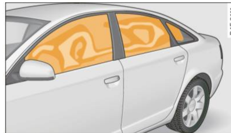
Fig. 210 Illustration of principle: Inflated side curtain airbags on the left side
