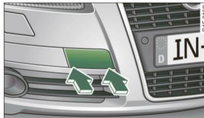
Fig. 263 Front bumper: removing the cover cap
