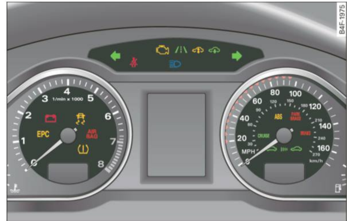
Fig. 7 Instrument cluster with warning/indicator lights
