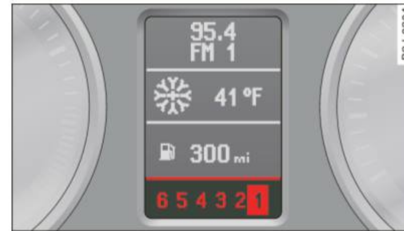
Fig. 154 Display: manual shift program, selected gear highlighted
