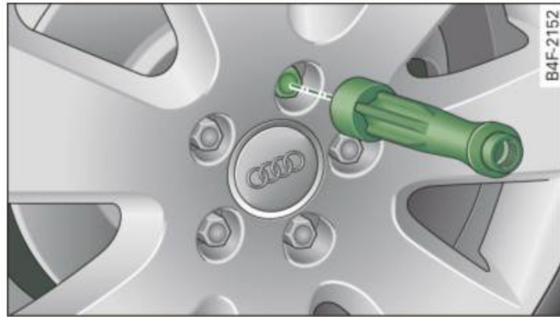
Fig. 254 Changing a wheel: using the screwdriver handle (with the blade removed) to turn the bolts
