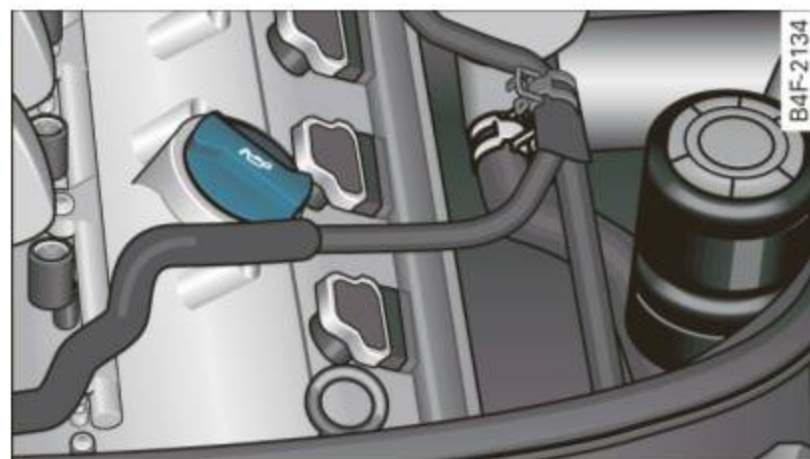
Fig. 234 Engine compartment: Oil filler cap location
