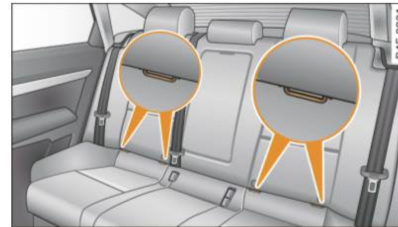
Fig. 217 Rear seats: lower anchorage bracket locations
