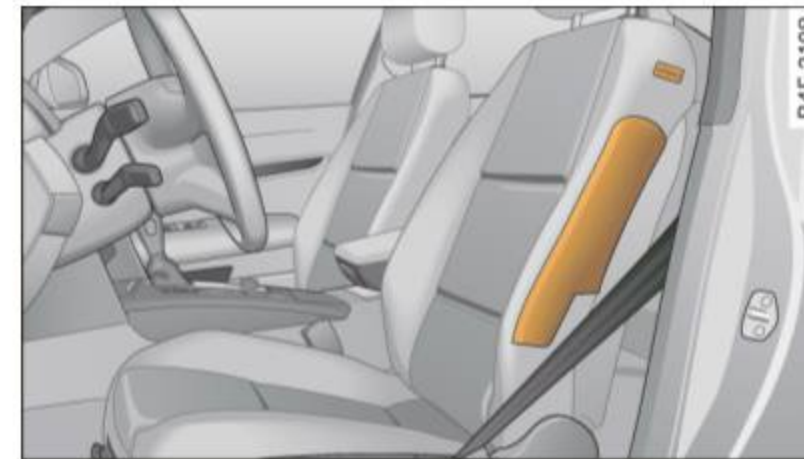
Fig. 207 Side airbag location in the driver's seat
