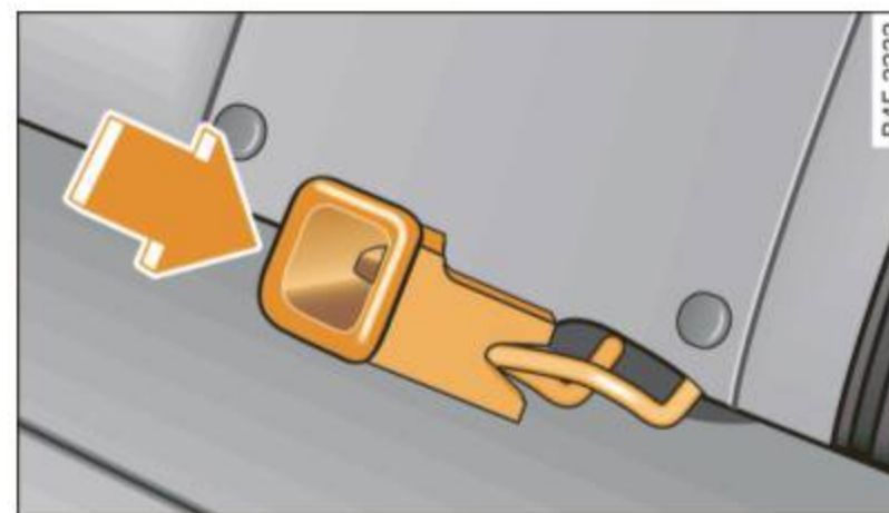
Fig. 219 Close-up: fitting the guidance fixture over the lower anchorage bracket
