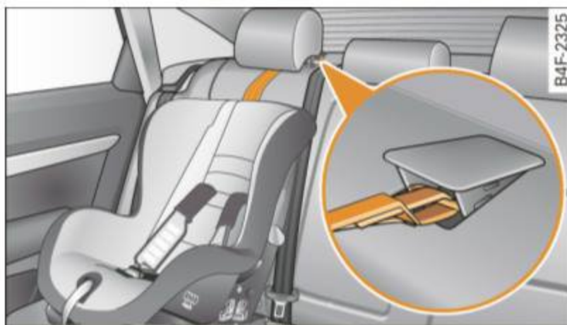
Fig. 224 Tether strap: proper routing and mounting
