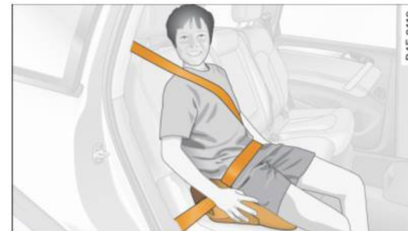
Fig. 214 Child taller than 4 ft. 9 in. properly restrained on the rear seat
