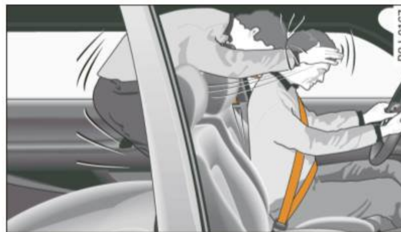
Fig. 196 A rear passenger not wearing a safety belt will fly forward and strike the driver
