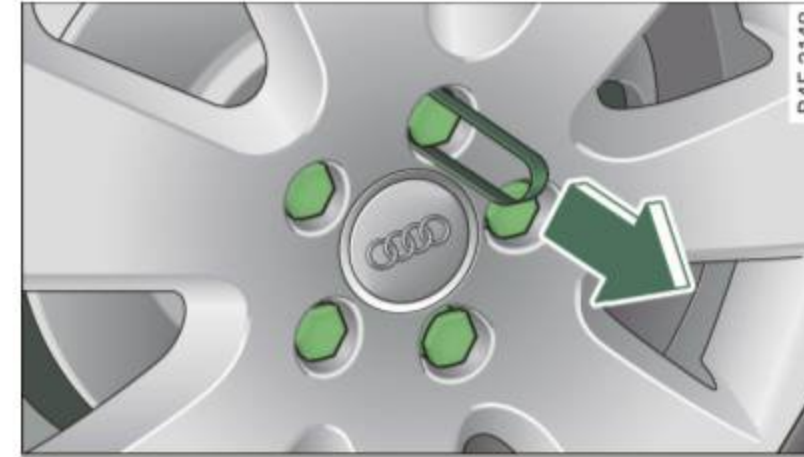
Fig. 250 Changing a wheel: removing the wheel bolt caps
