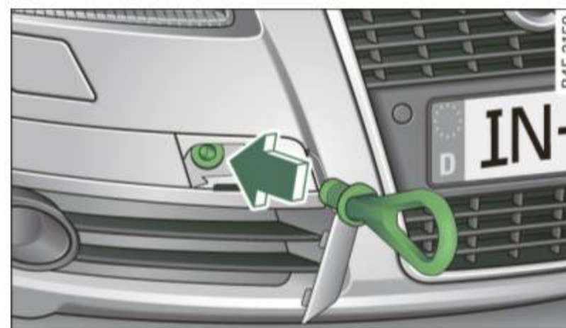
Fig. 264 Front bumper: screwing in the towing loop
