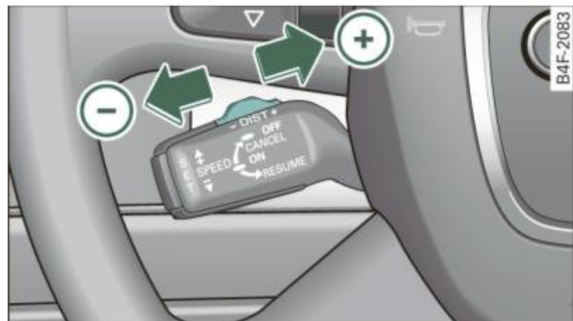
Fig. 135 Control lever: Setting distance
