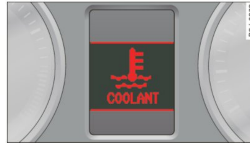
Fig. 18 Display: engine coolant level warning (priority 1)
