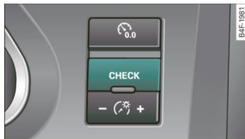
Fig. 5 CHECK button in the instrument cluster
