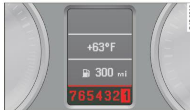
Fig. 162 Display: manual shift program, selected gear highlighted
