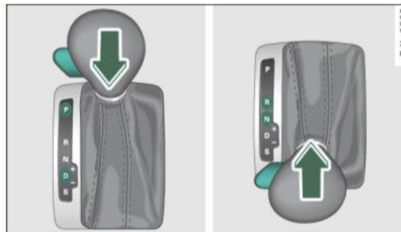
Fig. 160 Shift gate: selector lever lock positions and interlock button highlighted
