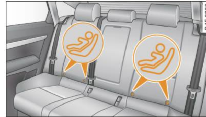
Fig. 216 Rear seat-backs: locator buttons for lower anchorages
