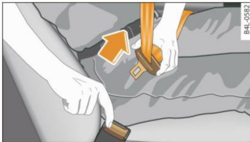
Fig. 201 Releasing the tongue from the buckle
