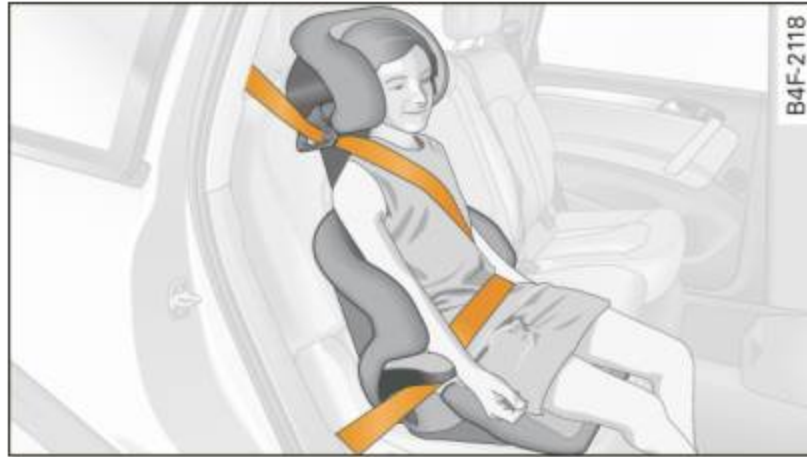
Fig. 213 Rear seat: child properly restrained in a booster seat
