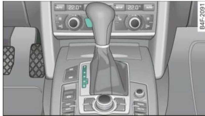
Fig. 158 Section of the center console: selector lever with lock button
