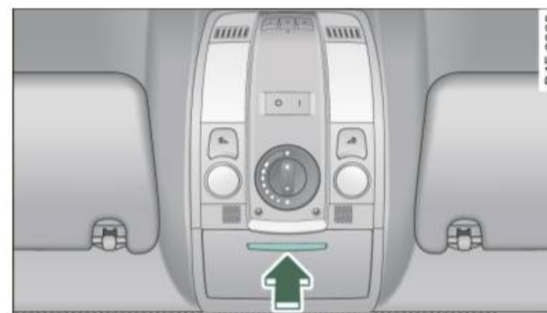
Fig. 107 Storage compartment in roof
