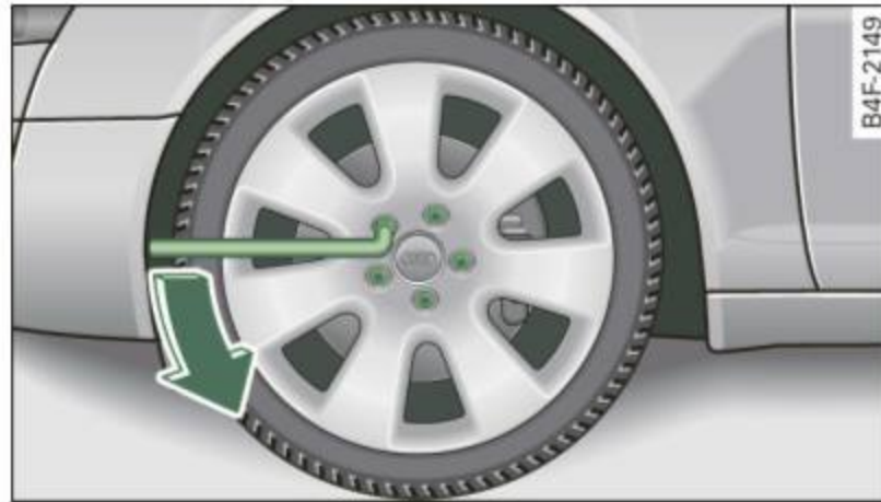
Fig. 251 Changing a wheel: loosening the wheel bolts
