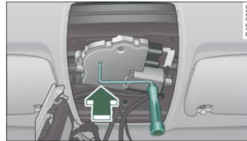
Fig. 53 Section from headliner: crank for emergency operation
