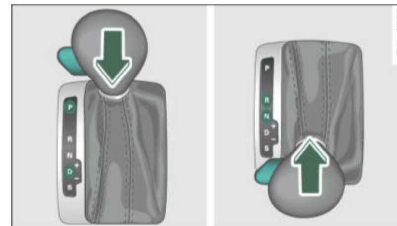
Fig. 152 Shift gate: selector lever lock positions and interlock button highlighted
