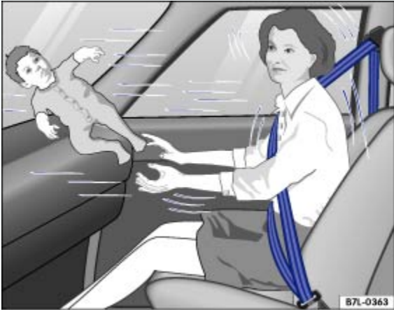
Fig. 75 Never let babies or older children ride in a vehicle while sitting on the lap of another passenger.
