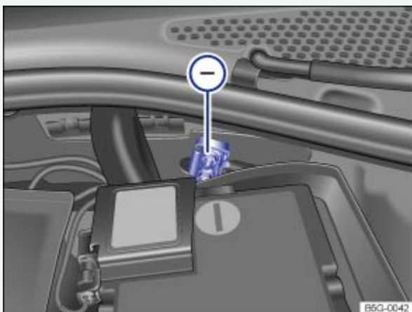
Fig. 235 In the engine compartment: Negative jump-start terminal ⊖.
