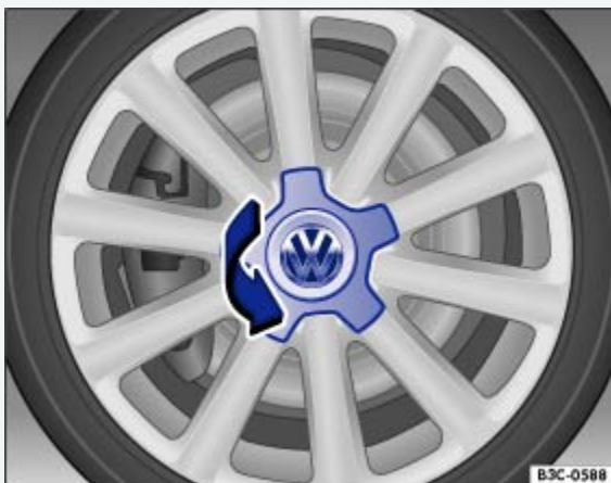
Fig. 218 Pulling the hubcap off.
