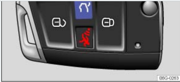
Fig. 34 On the remote control vehicle key: Button to unlock the trunk lid.
