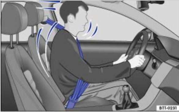
Fig. 61 Belted driver secured by the correctly worn safety belt in the event of a sudden braking maneuver.
