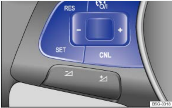
Fig. 155 Left-hand side of the multi-function steering wheel (if equipped): Buttons for operating the cruise control.
