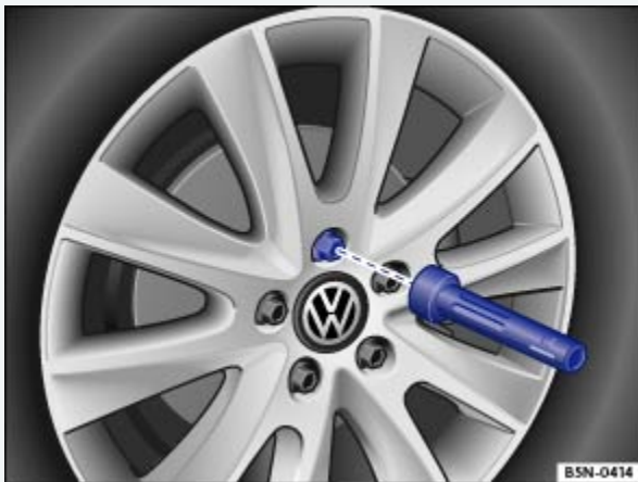
Fig. 229 Changing a wheel: Remove previously loosened wheel bolts using the screwdriver handle.
