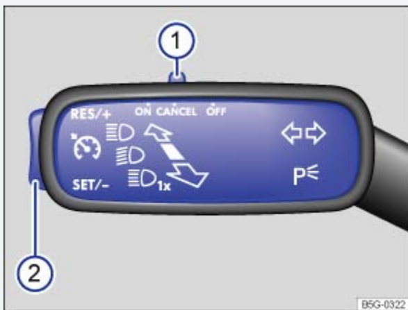
Fig. 154 On the turn signal lever: Cruise control buttons and switches (if equipped).
