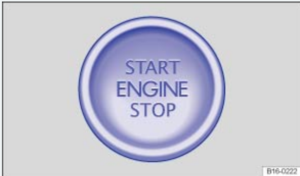
Fig. 135 In the lower center console: Starter button for the Keyless Access system.
