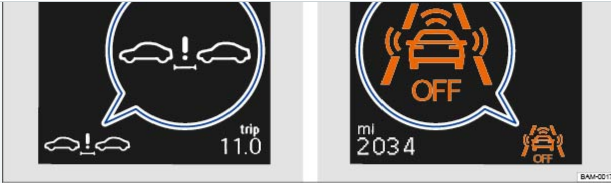
Fig. 163 Symbols in the instrument cluster display. : Distance warning. : System switched off (symbol displayed in color on an instrument cluster with color display).
