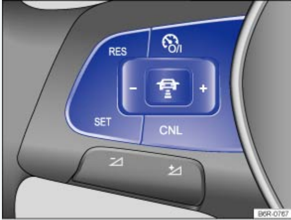
Fig. 160 Left-hand side of the multifunction steering wheel: Buttons for operating the Adaptive Cruise Control (ACC).
