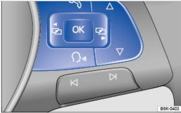
Fig. 17 Right side of the multi-function steering wheel (if equipped): Controls for the menus and information in the instrument cluster display.
