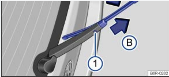
Fig. 205 Changing the rear window wiper blades.
