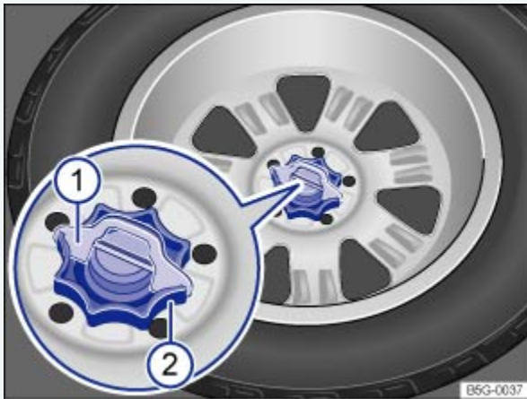
Fig. 114 In the luggage compartment: Handwheel holding the spare wheel in place (if equipped).
