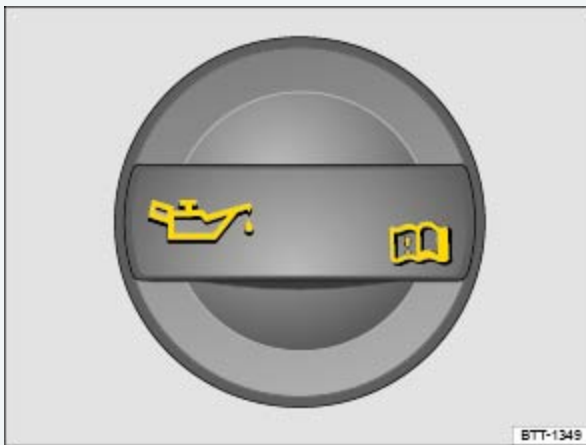
Fig. 199 In the engine compartment: Engine oil filler cap (cap design may vary depending on vehicle equipment).
