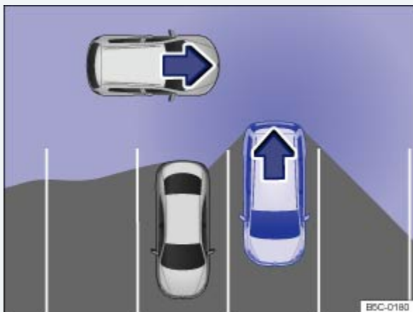
Fig. 185 Rear Traffic Alert: Monitored area around the vehicle that is backing out of a parking space.
