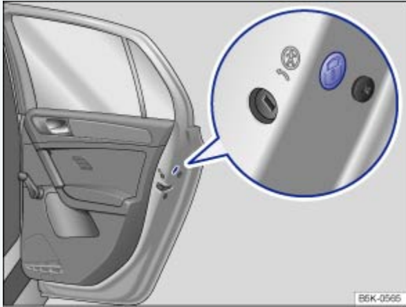
Fig. 210 On the front side of the passenger side rear door: Manual lock, covered by a rubber seal.
