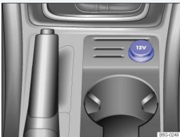
Fig. 132 In the lower center console: 12 Volt socket (vehicles with parking brake lever).
