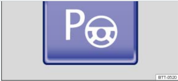
Fig. 178 In the lower center console: Button for switching on the Park Assist system.
