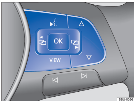
Fig. 16 Right side of the multi-function steering wheel: Controls for the menus and information in the instrument cluster display.
