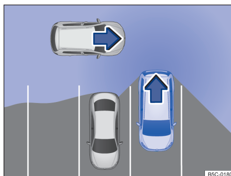
Fig. 123 Rear Traffic Alert: Monitored area around the vehicle that is backing out of a parking space.
