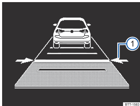
Fig. 111 In the instrument cluster display: ACC active, vehicle detected ahead, time interval is being set (displayed in color on an instrument cluster with color display).
