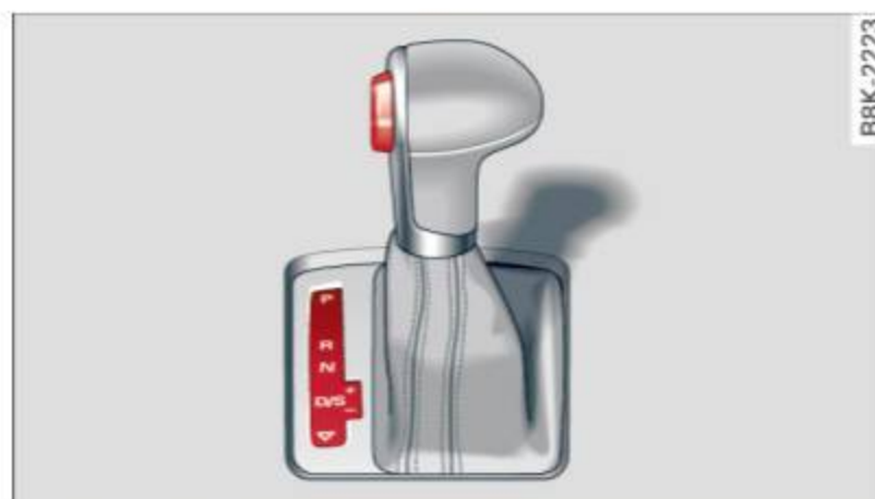
Fig. 83 Shift gate on the center console: selector lever with release button
