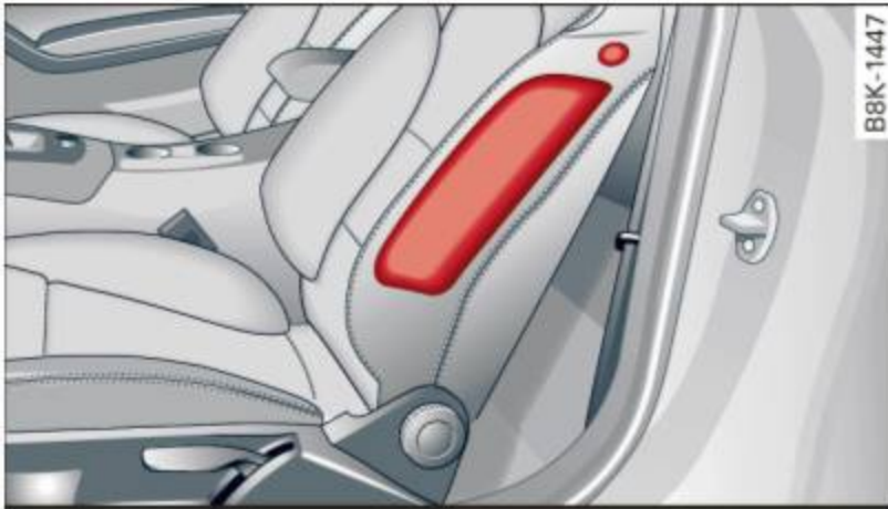
Fig. 146 Side airbag location in the driver's seat
