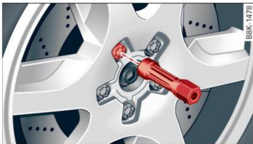
Fig. 189 Changing a wheel: using the screwdriver handle (with the blade removed) to turn the bolts
