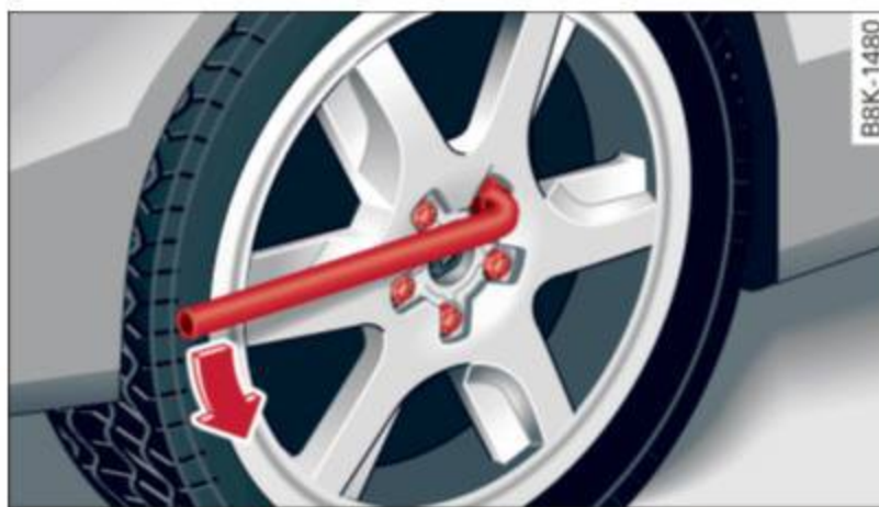
Fig. 186 Changing a wheel: loosening the wheel bolts
