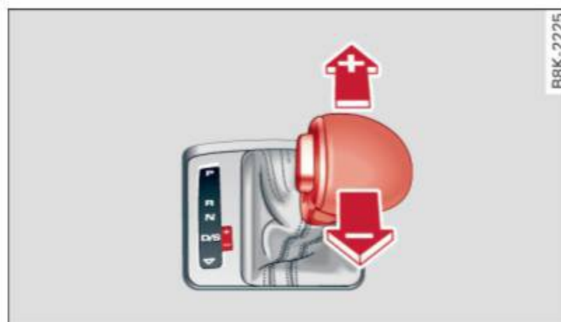
Fig. 86 Center console: shifting the multitronic/tiptronic manually
