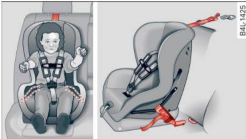
Fig. 152 Schematic overview: installation of the attachments applicable to a LATCH seat
