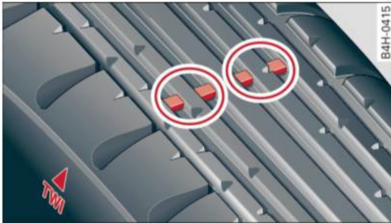
Fig. 178 Tire tread: tread wear indicators (TWI)
