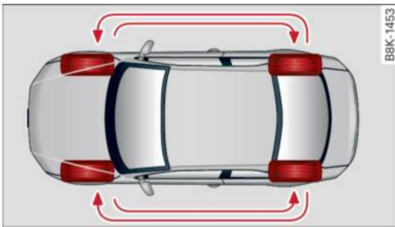
Fig. 179 Rotating tires for more even wear
