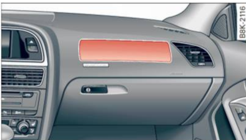
Fig. 141 Location of front passenger's airbag: in the instrument panel
