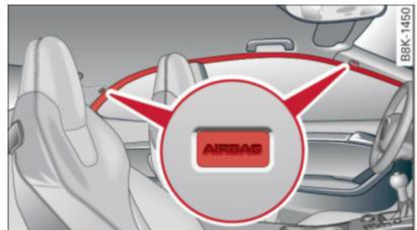
Fig. 148 Side curtain system, driver's side: side curtain airbag location
