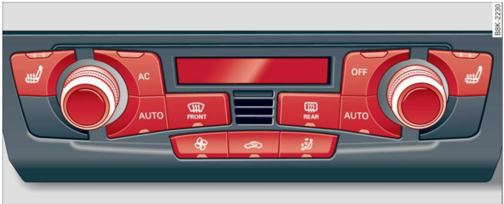
Fig. 72 3-zone deluxe automatic climate control*: controls
