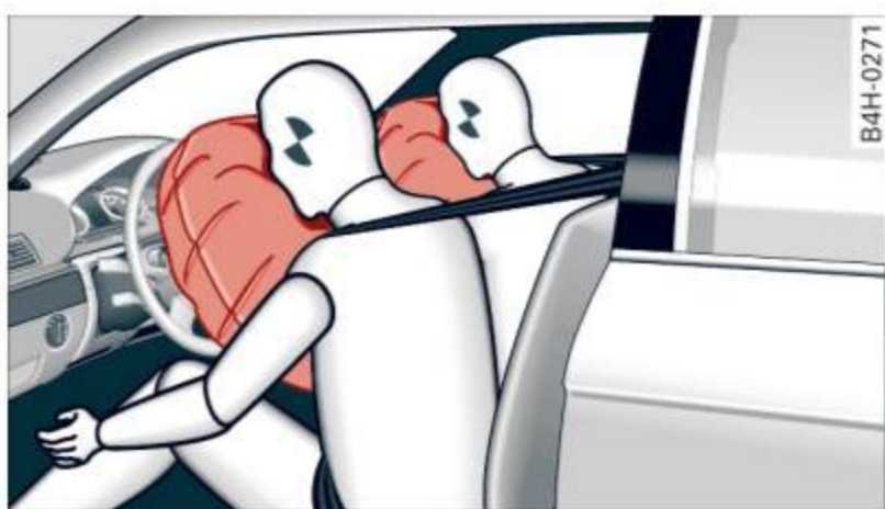
Fig. 142 Inflated front airbags
