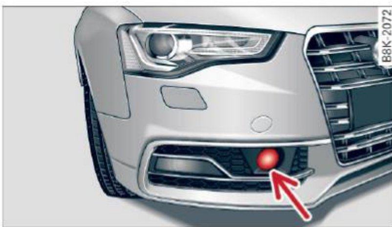
Fig. 97 Front of the vehicle: Position of radar sensor
