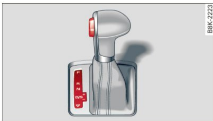
Fig. 92 Section of the center console: Selector lever with interlock button
