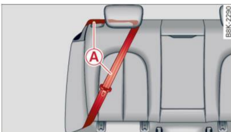
Fig. 150 Schematic overview: keep unused safety belts away from children in child safety seats. A - outer rear safety belt
