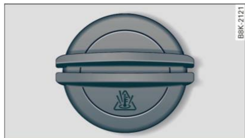
Fig. 172 Engine compartment: Cover on the coolant expansion tank
