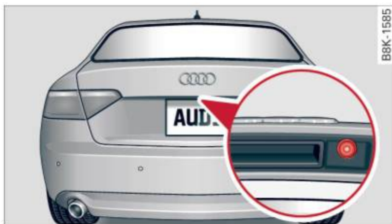
Fig. 118 Trunk lid: Location of the rear view camera
