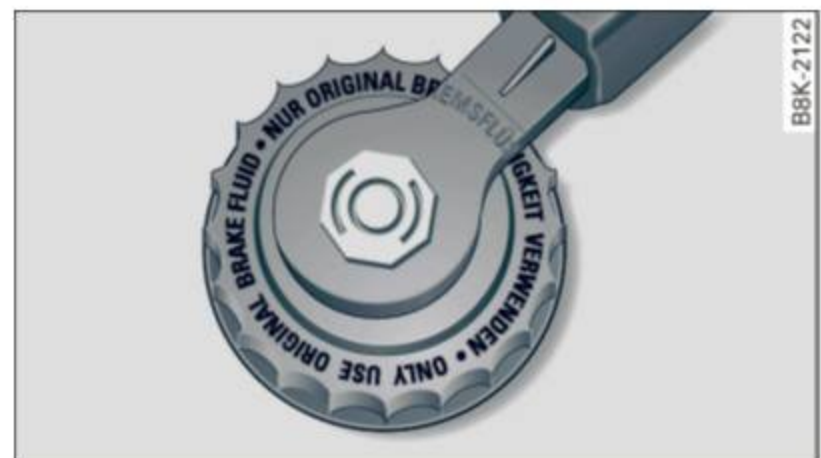
Fig. 173 Engine compartment: Cover on the brake fluid reservoir
