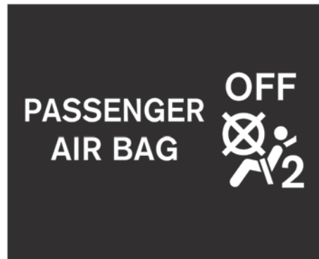
Front passenger air bag status light Front passenger air bag and status light
