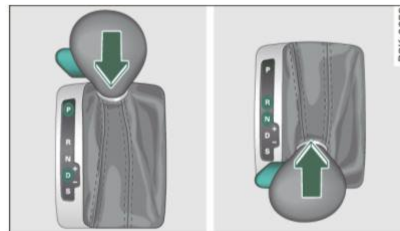
Fig. 138 Shift gate: selector lever lock positions and interlock button highlighted
