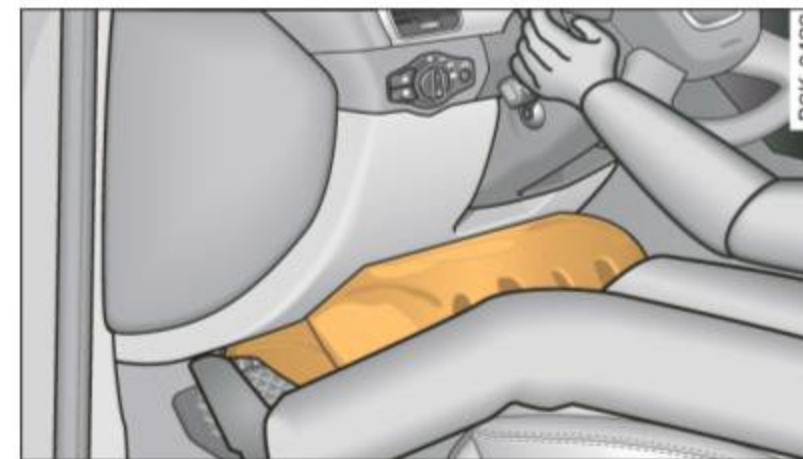
Fig. 177 Inflated airbags protecting in a frontal collision
