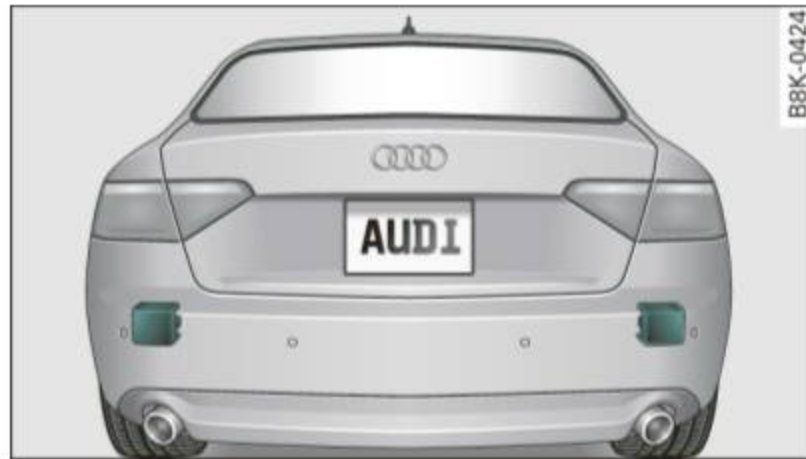
Fig. 123 Rear bumper: Position of radar sensors (not visible on outside)
