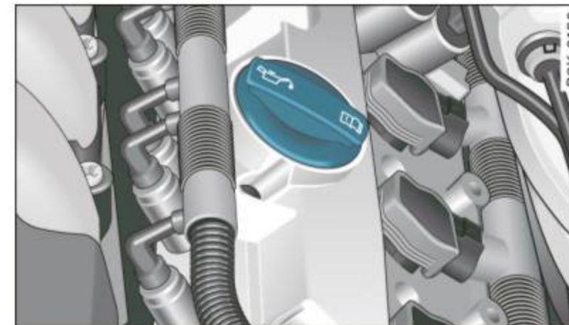
Fig. 205 Engine compartment: Oil filler cap location
