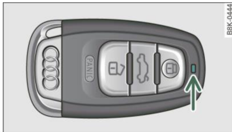
Fig. 32 Check light in the master key
