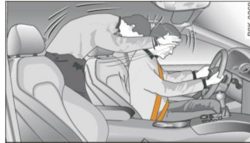
Fig. 166 A rear passenger not wearing a safety belt will fly forward and strike the driver
