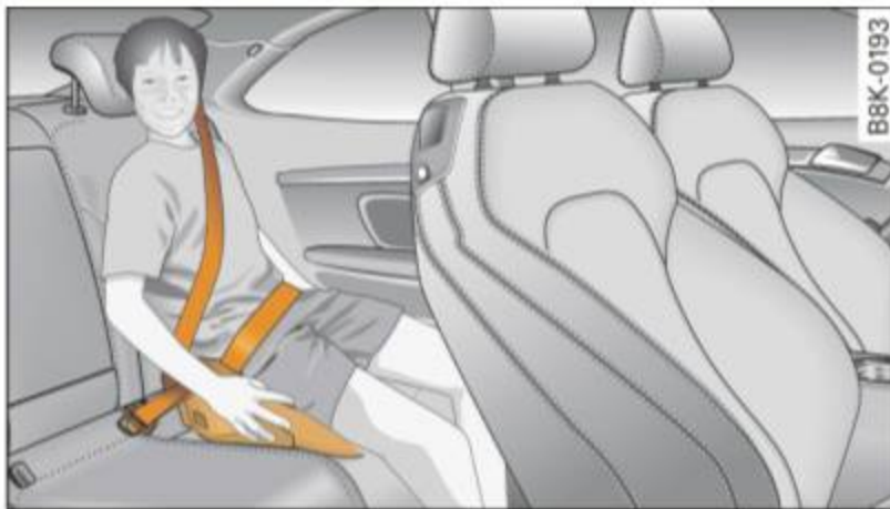
Fig. 185 Rear seat: child properly restrained in a booster seat (without seat-back)
