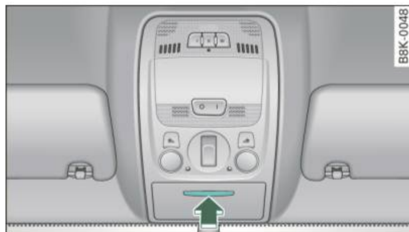
Fig. 105 Storage pocket in the roof
