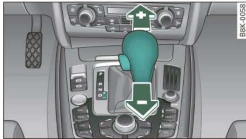
Fig. 139 Center console: shifting the tiptronic® manually
