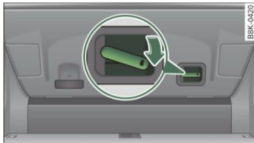
Fig. 215 Trunk escape handle: view from inside the closed trunk
