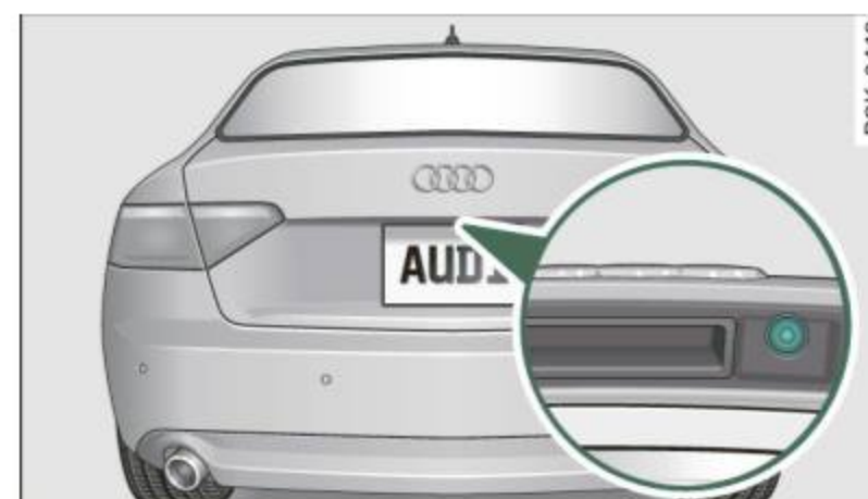
Fig. 149 Trunk lid: Location of the rear- view camera
