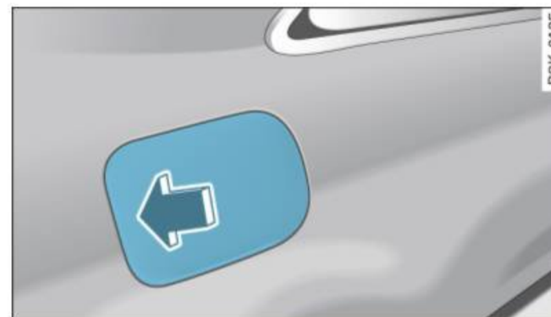
Fig. 196 Right rear vehicle side: Opening the fuel filler flap
