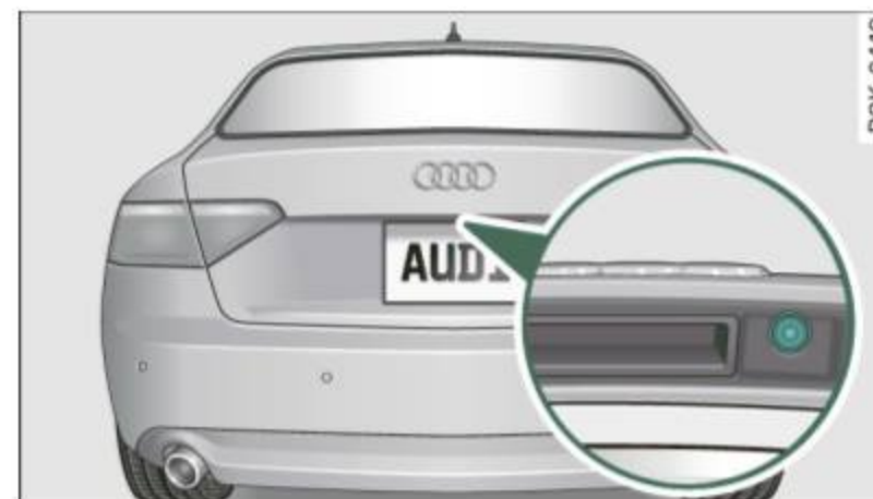
Fig. 144 Rear lid: Location of the rear-view camera
