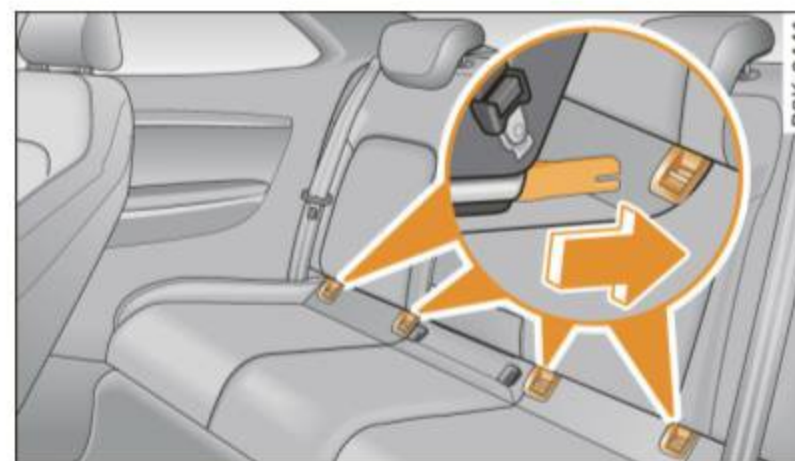
Fig. 190 Installation of child safety seat with rigid latches on bars
