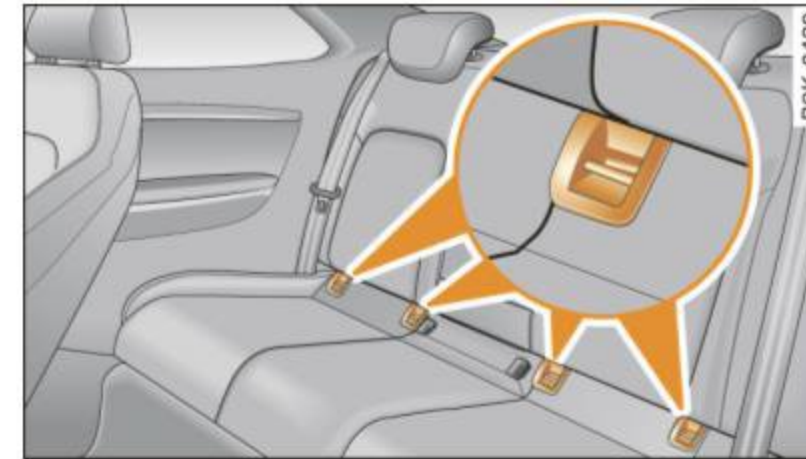
Fig. 188 Rear seats: lower anchorage bracket locations
