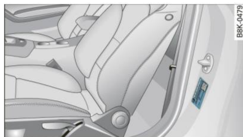
Fig. 210 Tire pressure label: located either on driver's side B-pillar or inside the fuel filler flap
