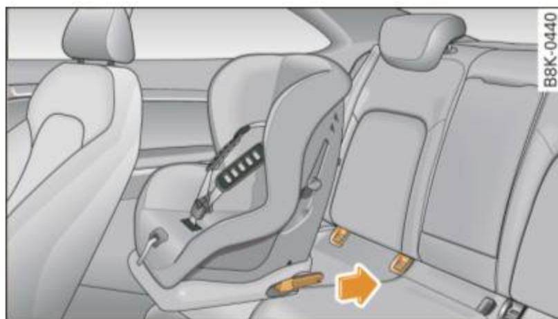
Fig. 189 LATCH-type seat with both latch bars extended
