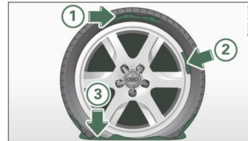
Fig. 219 Tire damage for which the tire mobility system is not suited
