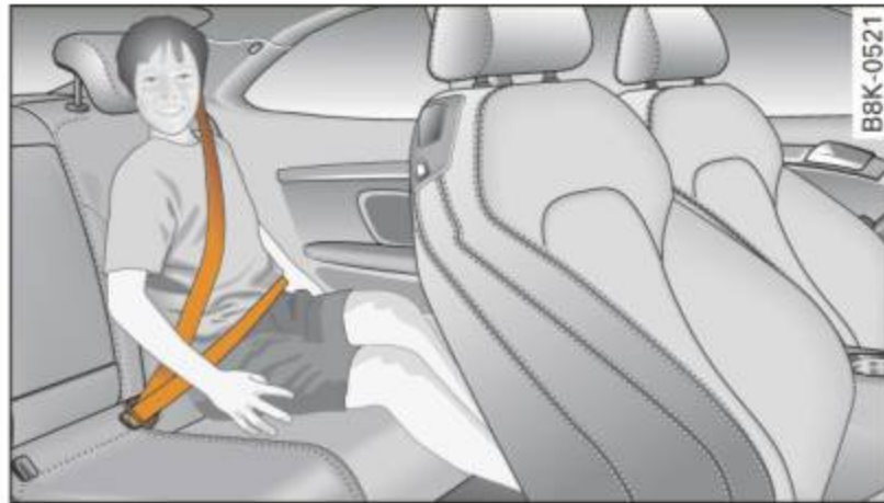
Fig. 186 Child taller than 4 ft. 9 in. properly restrained on the rear seat
