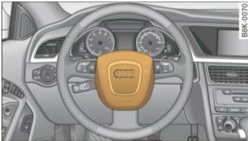
Fig. 172 Location of driver airbag: in steering wheel
