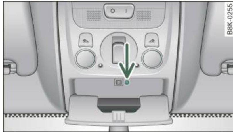
Fig. 52 Section from headliner: Unscrewing lighting unit
