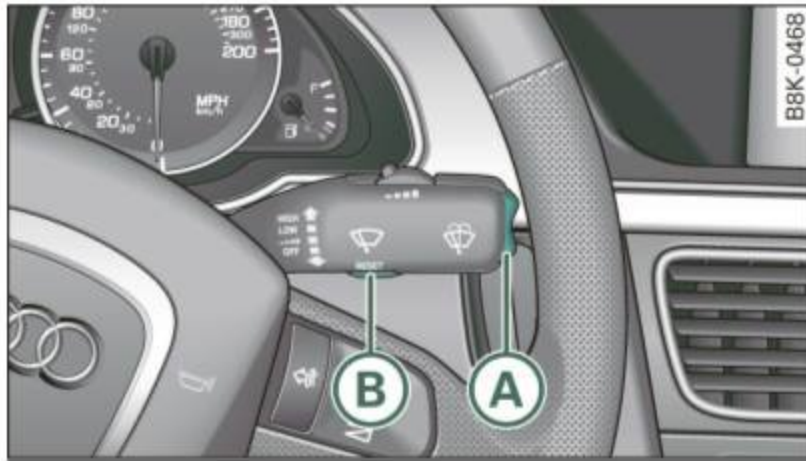
Fig. 21 Windshield wiper lever: controls for the trip computer
