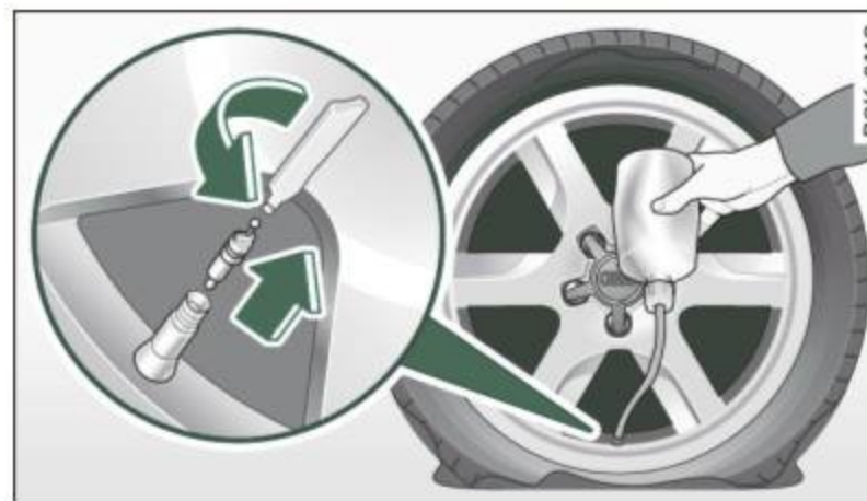
Fig. 220 Tire mobility system: filling a tire
