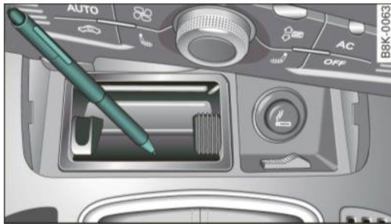
Fig. 143 Emergency release for selector lever
