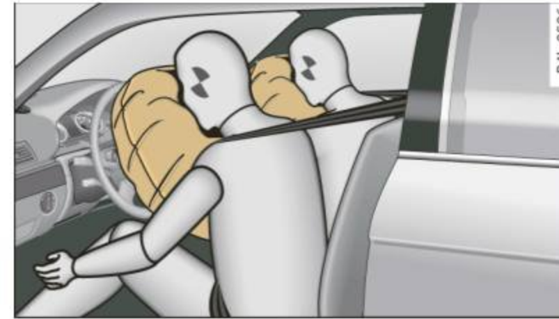
Fig. 174 Inflated front airbags
