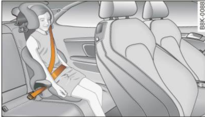
Fig. 184 Rear seat: child properly restrained in a booster seat (with seatback)
