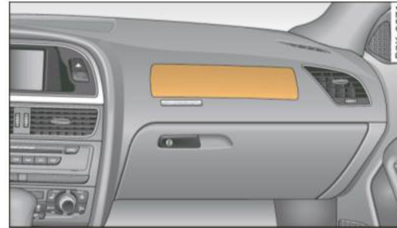
Fig. 173 Location of front passenger's airbag: in the instrument panel
