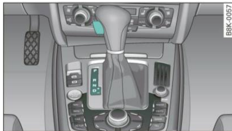
Fig. 136 Shift gate on the center console: selector lever with release button
