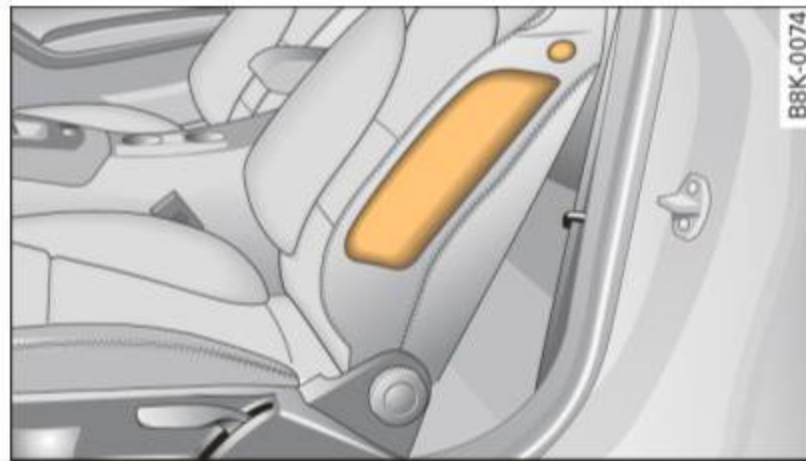
Fig. 178 Side airbag location in the driver's seat
