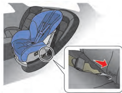
Forward-facing web-mounted — step 2
