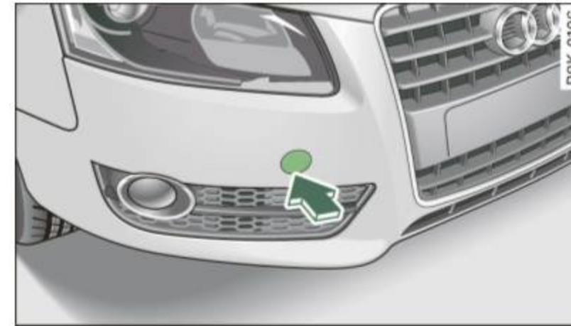
Fig. 241 Front bumper: removing the cover cap
