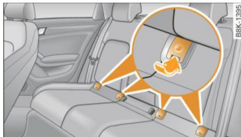
Fig. 199 Lower anchorages, covers marked
