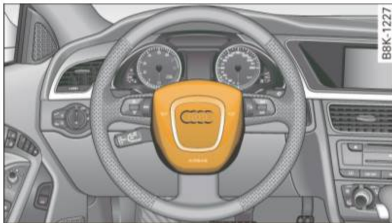
Fig. 186 Location of driver airbag: in steering wheel
