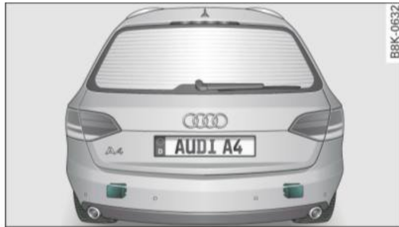
Fig. 141 Rear bumper: Position of radar sensors (not visible on outside)
