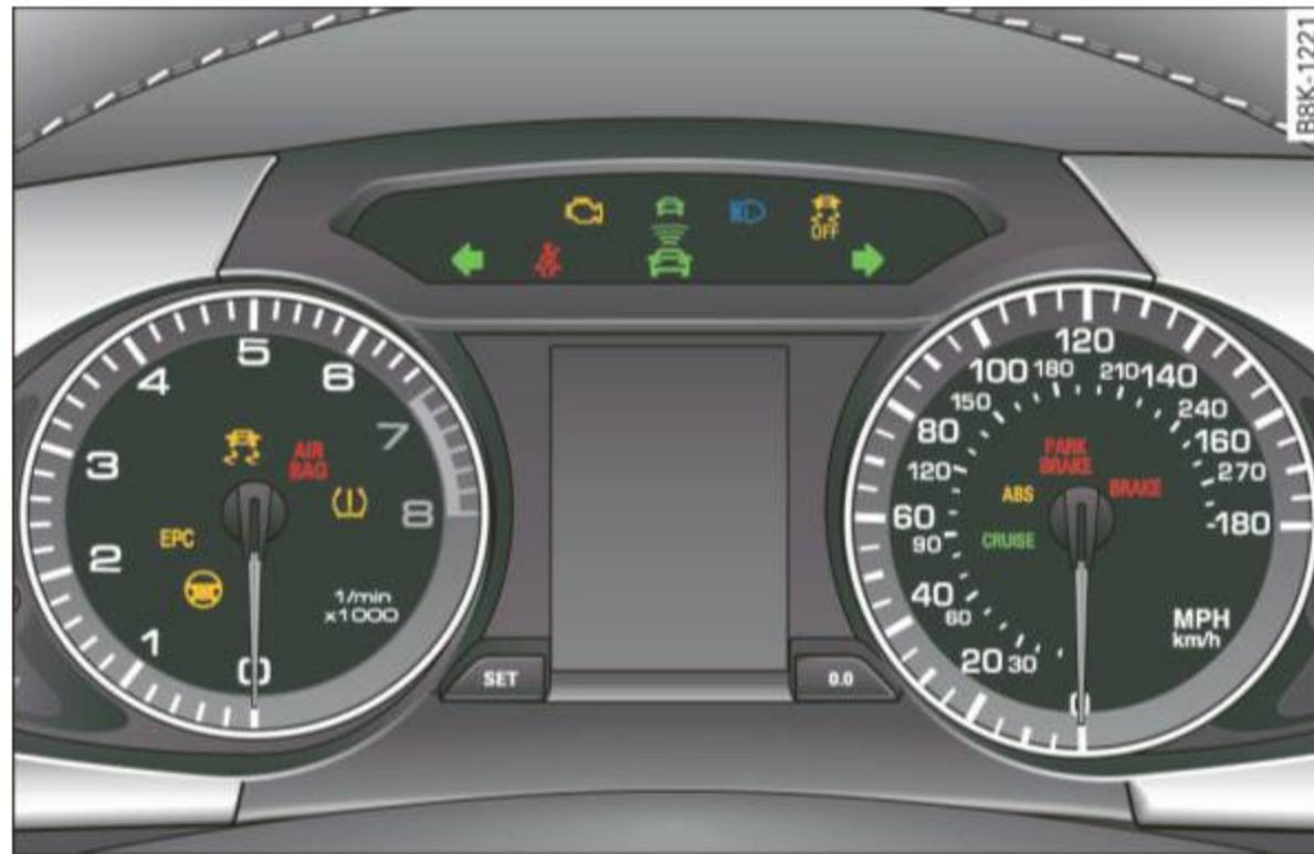
Fig. 7 Instrument cluster with warning/indicator lights
