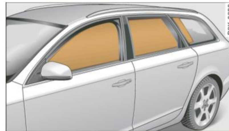
Fig. 193 Illustration of principle: Inflated side curtain airbags on the left side
