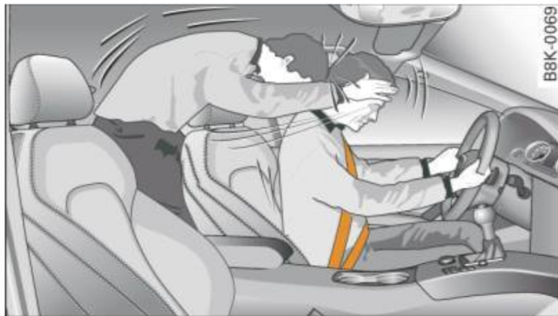
Fig. 179 A rear passenger not wearing a safety belt will fly forward and strike the driver
