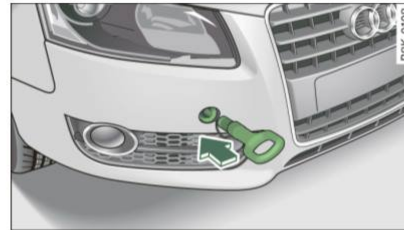
Fig. 242 Front bumper: screwing in the towing loop
