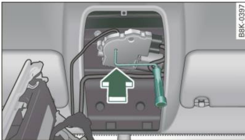
Fig. 49 Section from headliner: Crank for emergency operation
