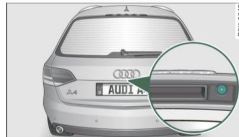
Fig. 164 Trunk lid: Location of the rear view camera
