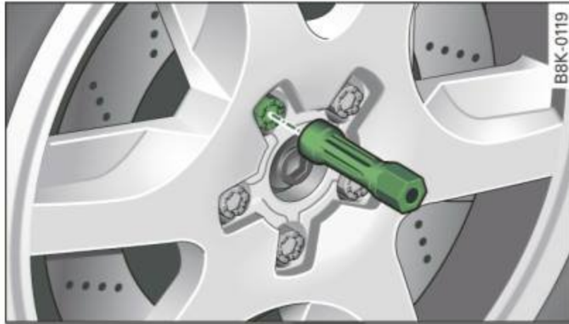
Fig. 233 Changing a wheel: using the screwdriver handle (with the blade removed) to turn the bolts
