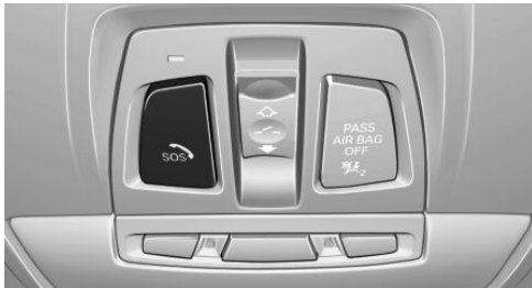
SOS button in the roof lining.
