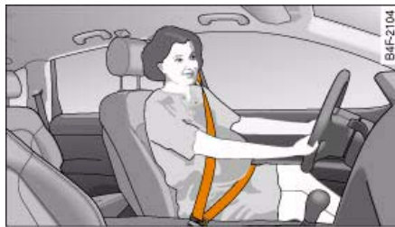
Fig. 211 Positioning seat belts during pregnancy
