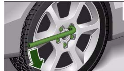
Fig. 272 Changing a wheel: Loosening wheel bolts
