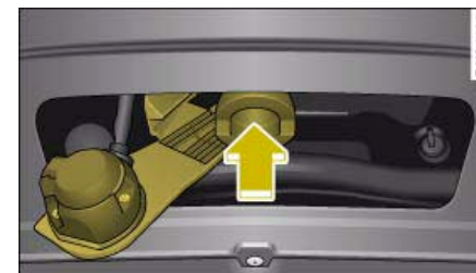
Fig. 240 Removable towing bracket: Inserting the ball joint
