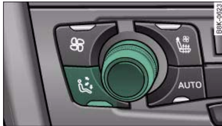
Fig. 117 Air distribution button and rotary control
