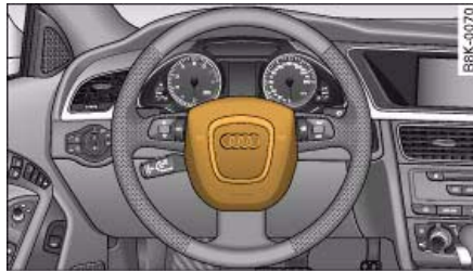
Fig. 214 Driver's airbag in steering wheel
