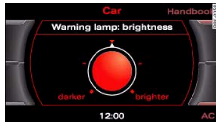
Fig. 171 Display: Adjusting brightness of warning lamp
