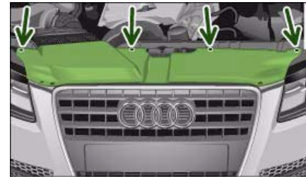
Fig. 288 Trim panel: Attachment points are marked by arrows
