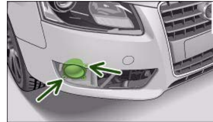
Fig. 299 Screws securing fog light
