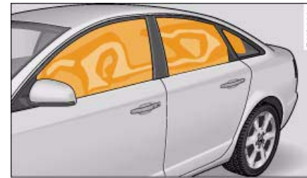
Fig. 221 Head-protection airbags in inflated condition
