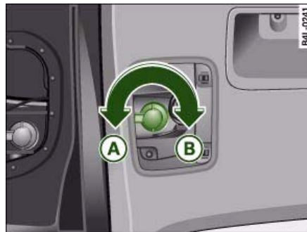
Fig. 287 Diagram: Bulb holder with a bayonet fastener
