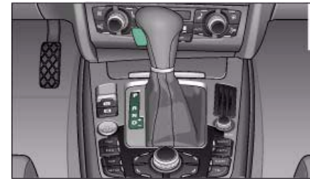
Fig. 177 Detail of the centre console: Selector lever with interlock button
