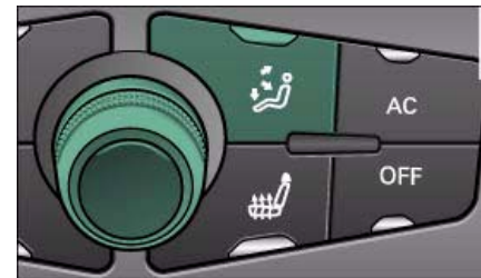
Fig. 108 Air distribution button and rotary control
