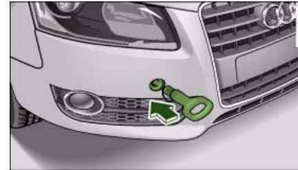
Fig. 281 Front bumper: Fitting the towing eye
