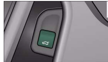
Fig. 45 Driver's door: Unlocking the boot lid ►
