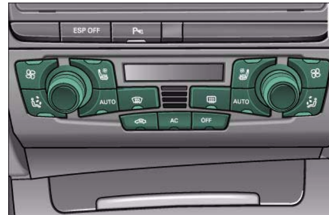
Fig. 112 Air conditioner controls
