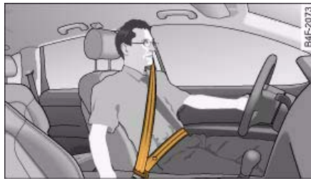
Fig. 208 Positioning of head restraints and seat belts
