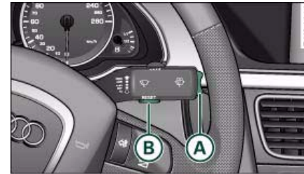
Fig. 20 Windscreen wiper lever: On-board computer controls
