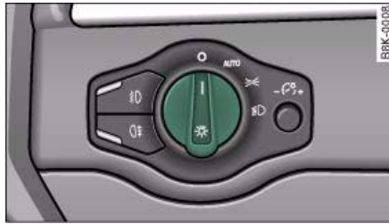
Fig. 54 Dashboard: Light switch
