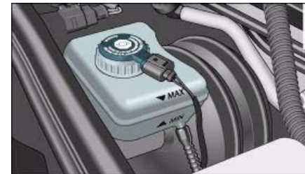
Fig. 258 Engine compartment: Markings on brake fluid reservoir
