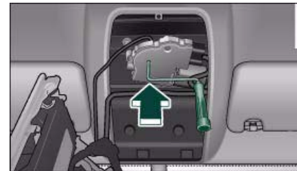
Fig. 53 Detail of headliner: Crank for manual operation
