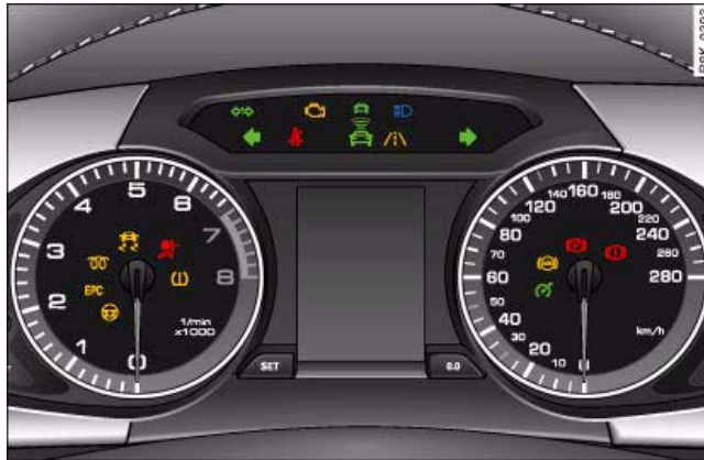
Fig. 7 Instrument cluster with warning and indicator lamps
