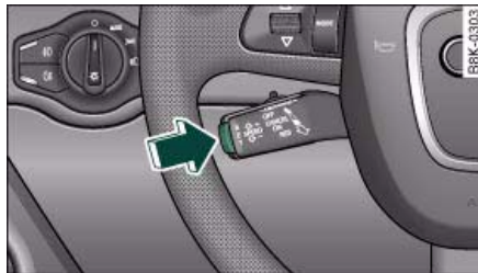
Fig. 139 Control lever for: Setting speed
