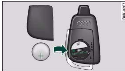
Fig. 126 Remote control: Changing battery
