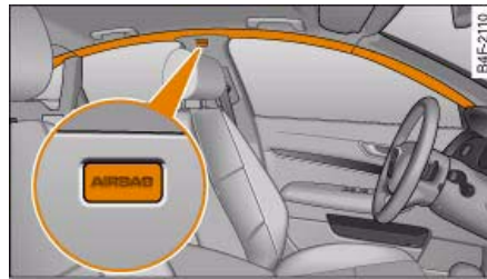
Fig. 220 Location of head-protection airbags above the doors
