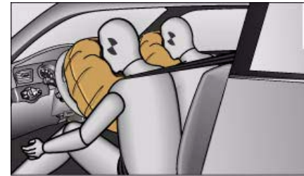
Fig. 216 Front airbags in inflated condition
