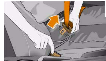
Fig. 213 The latch plate of the belt springs out of the buckle
