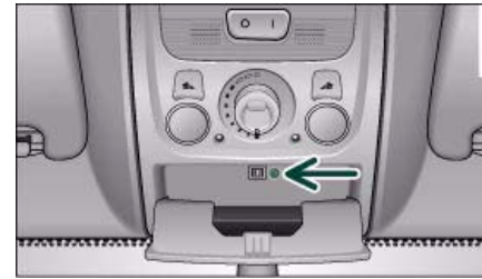
Fig. 52 Detail of headliner: Unscrewing the light housing
