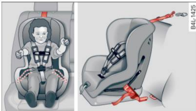
Fig. 163 Schematic overview: installation of the attachments applicable to a LATCH seat
