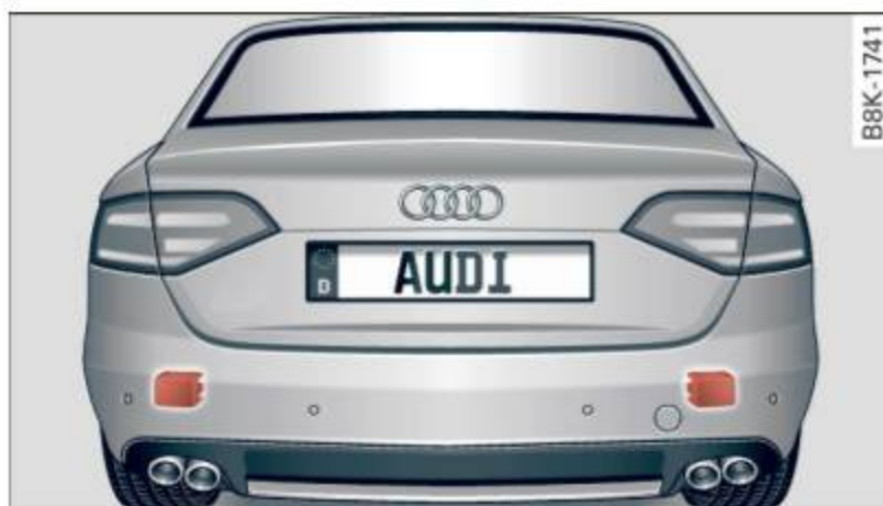
Fig. 124 Rear of the vehicle: position of the sensors
