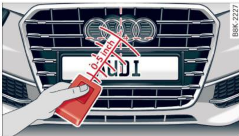
Fig. 137 Distance between the radiator grille and the hand transmitter
