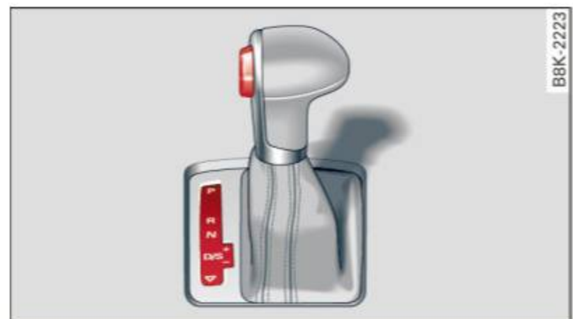
Fig. 105 Shift gate on the center console: selector lever with release button
