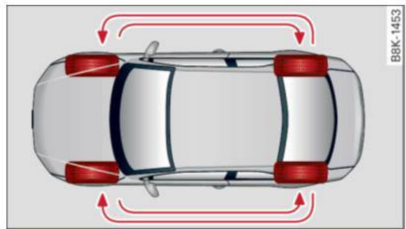
Fig. 192 Rotating tires for more even wear
