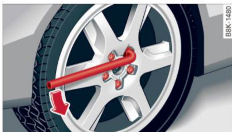
Fig. 202 Changing a wheel: loosening the wheel bolts
