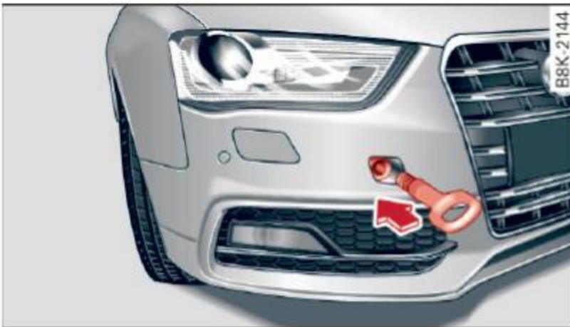
Fig. 214 Front bumper: screwing in the towing loop
