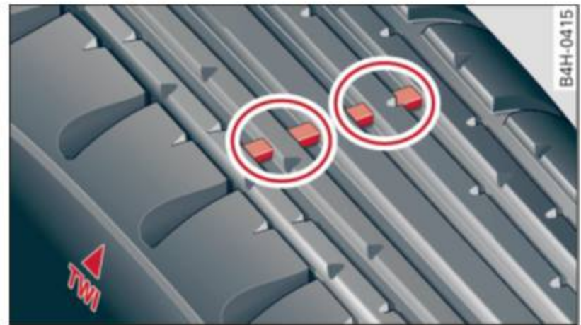
Fig. 191 Tire tread: tread wear indicators (TWI)
