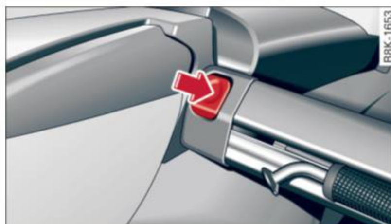
Fig. 78 Behind the backrest: removing the partition net
