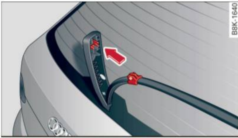
Fig. 55 Rear wiper: Removing the wiper blade
