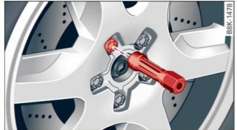
Fig. 205 Changing a wheel: using the screwdriver handle (with the blade removed) to turn the bolts
