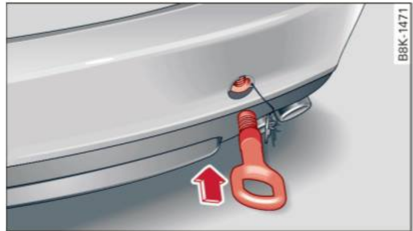
Fig. 216 Rear bumper: Screwing in towing loop
