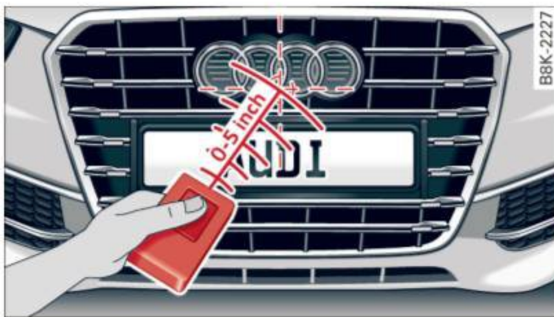
Fig. 138 Distance between the radiator grille and the hand transmitter
