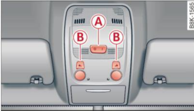
Fig. 43 Front headliner: interior lighting controls
