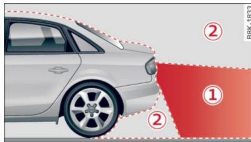
Fig. 133 Covered area ① and uncovered area ② of the rear view camera
