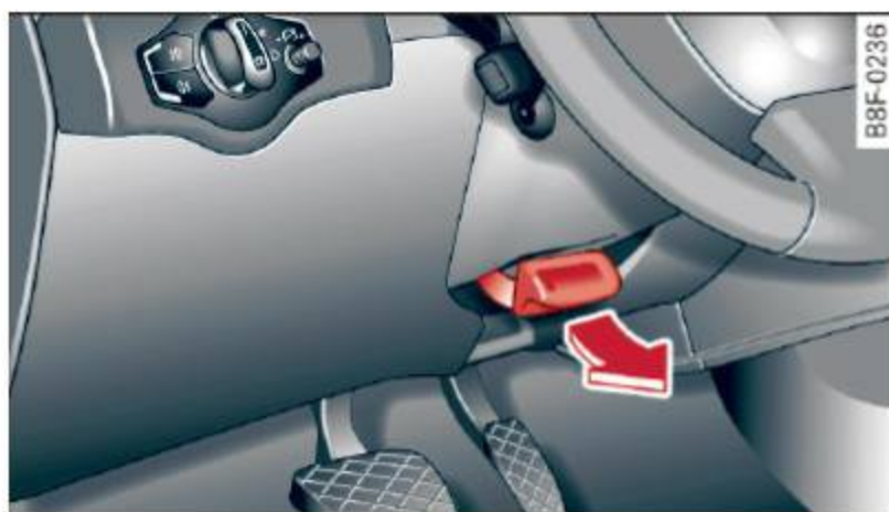
Fig. 96 Lever under the steering column
