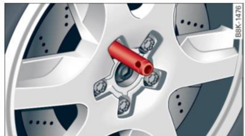
Fig. 206 Changing a wheel: alignment pin inside the top hole
