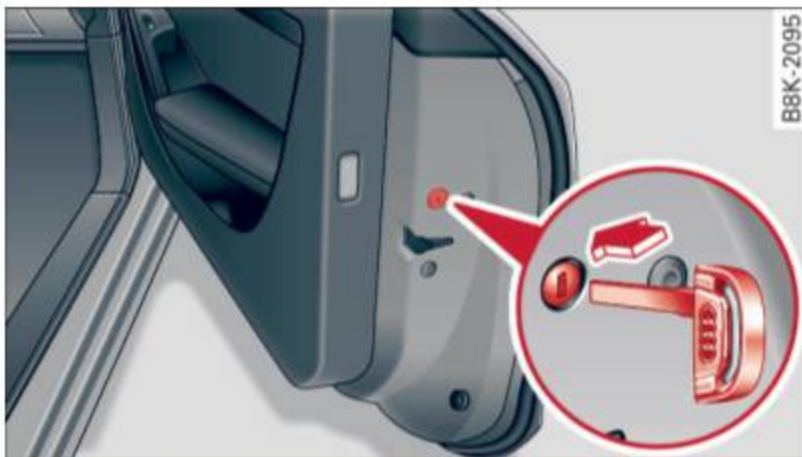
Fig. 26 Front passenger's door/rear doors*: emergency lock
