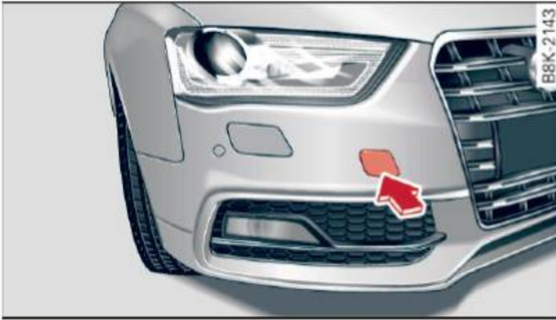
Fig. 213 Front bumper: removing the cover cap
