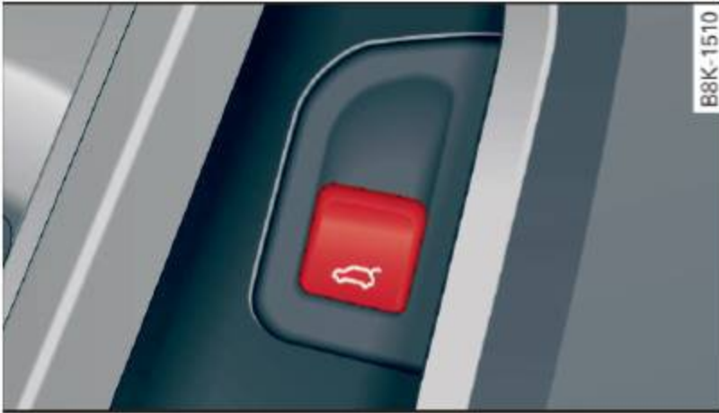
Fig. 29 Driver's door: Unlocking the rear lid
