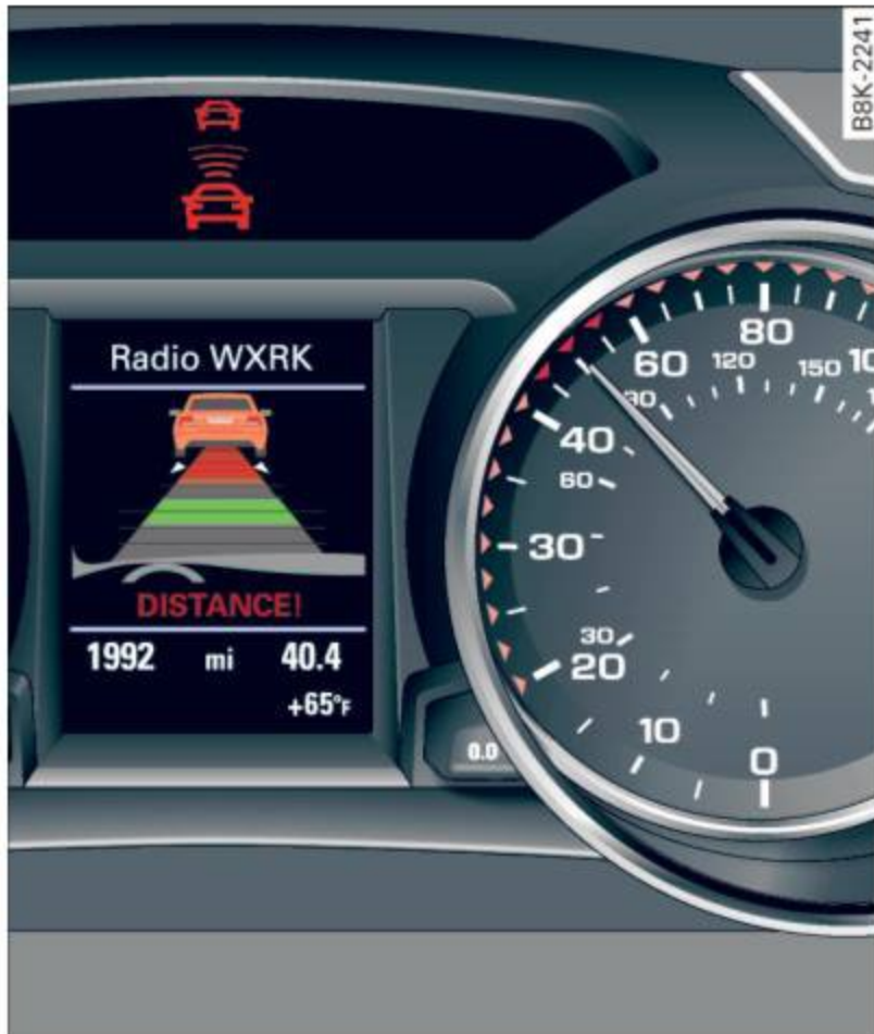
Fig. 122 Instrument cluster: request for driver intervention
