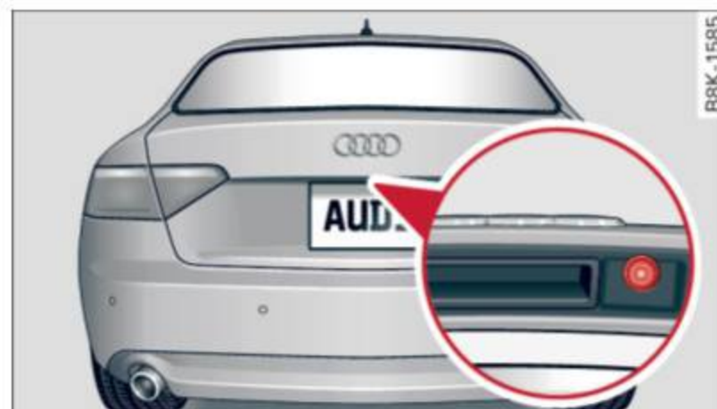
Fig. 134 Trunk lid: Location of the rear view camera
