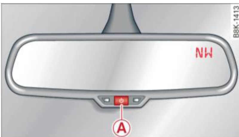
Fig. 59 Rearview mirror: Digital compass activated
