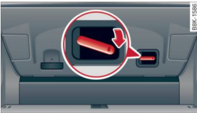
Fig. 33 Trunk escape handle: view from inside the closed rear lid
