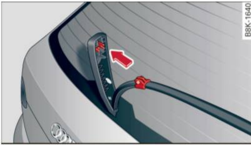
Fig. 58 Rear wiper: Removing the wiper blade
