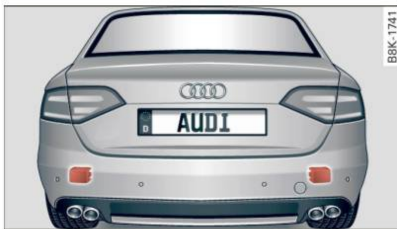
Fig. 127 Rear of the vehicle: position of the sensors
