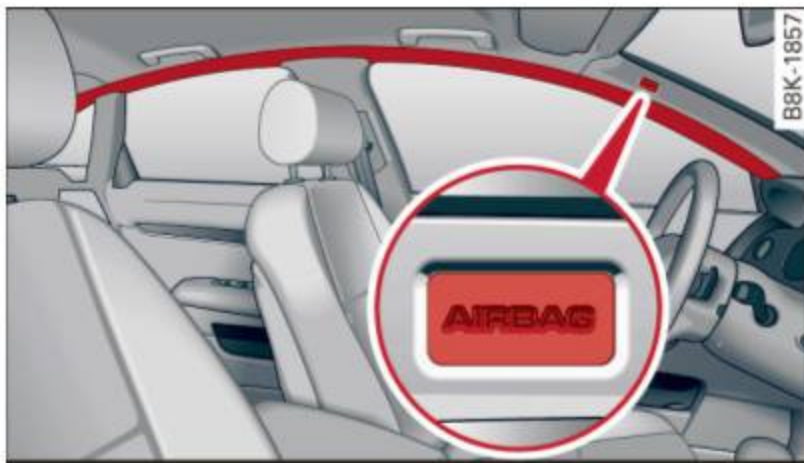
Fig. 159 Side curtain system, driver's side: side curtain airbag location
