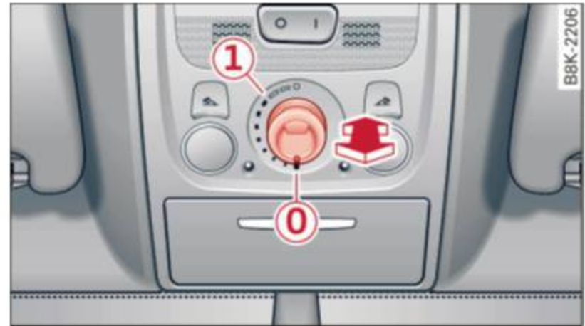
Fig. 37 Section of headliner: knob for sunroof
