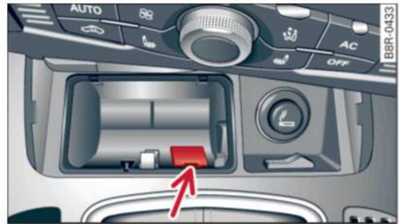
Fig. 112 Selector lever emergency release
