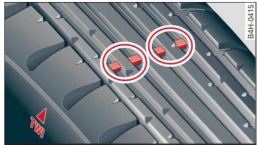
Fig. 191 Tire tread: tread wear indicators (TWI)
