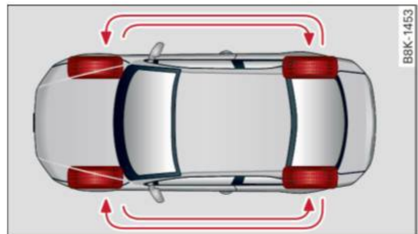
Fig. 192 Rotating tires for more even wear
