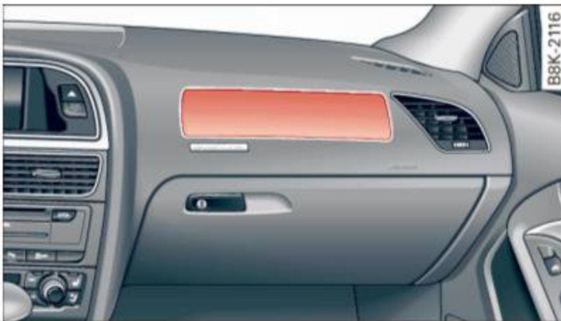
Fig. 154 Location of front passenger's airbag: in the instrument panel
