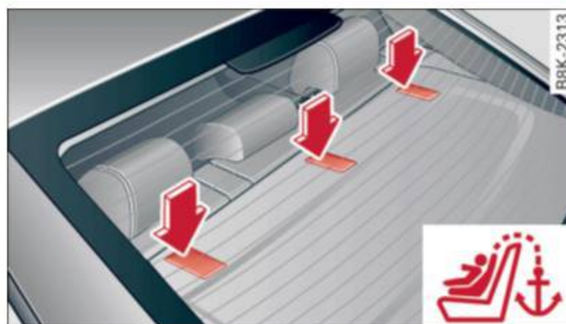
Fig. 170 Sedan Tether anchors: recess flaps behind the rear seatbacks
