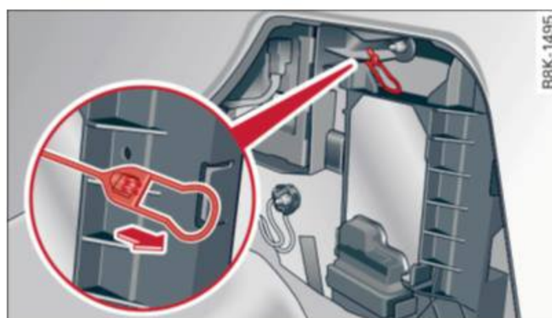
Fig. 179 Luggage compartment: Emergency opening of fuel filler flap
