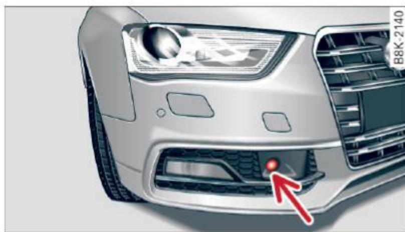
Fig. 113 Front of the vehicle: Position of radar sensor
