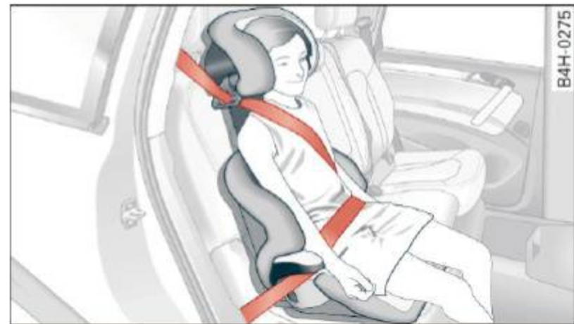
Fig. 165 Rear seat: child properly restrained in a booster seat
