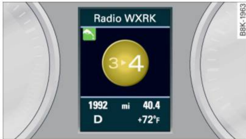
Fig. 14 Display: enhanced shift indicator
