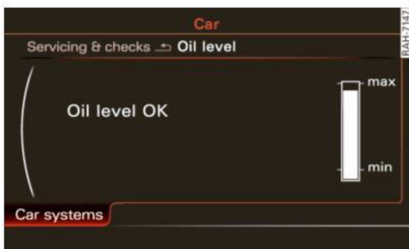
Fig. 183 MMI Display: Oil level indicator
