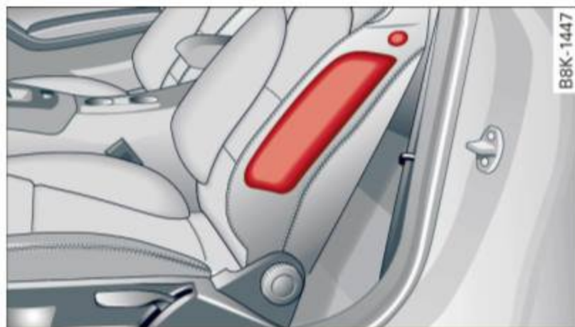
Fig. 157 Side airbag location in the driver's seat
