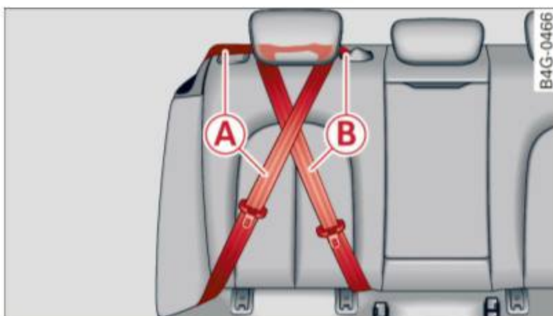
Fig. 161 Schematic overview: keep unused safety belts away from children in child safety seats. (A) - outer rear safety belt, (B) - center rear safety belt
