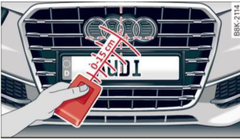
Fig. 42 Distance between the radiator grille and the hand transmitter
