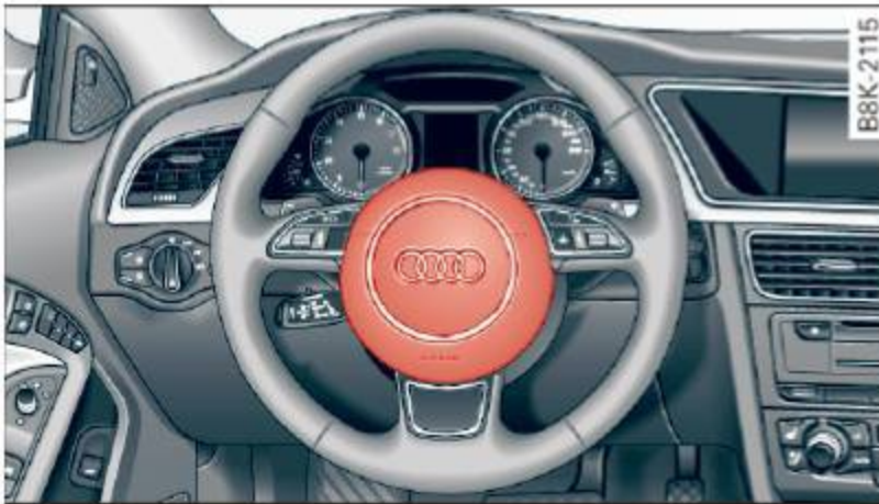
Fig. 153 Location of driver airbag: in steering wheel
