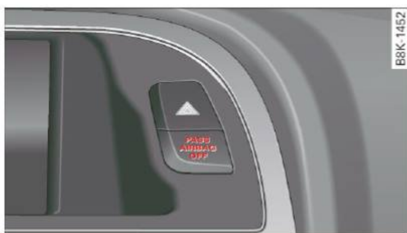
Fig. 156 Section from the instrument panel: PASSENGER AIR BAG OFF light
