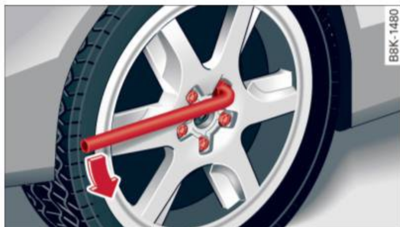
Fig. 202 Changing a wheel: loosening the wheel bolts
