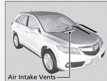
Air Intake Vents
