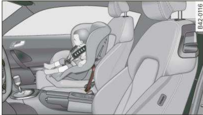
Fig. 107 Passenger seat: smaller child in a properly installed forward-facing convertible child safety seat
