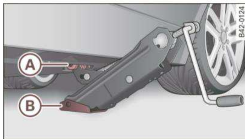
Fig. 134 Close-up: proper positioning of lifting jack
