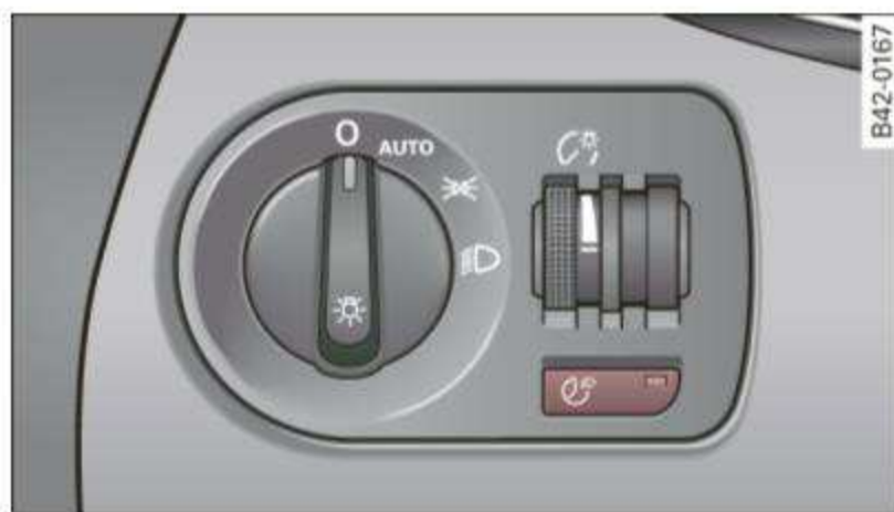
Fig. 44 Dashboard detail: coming home/leaving home switch
