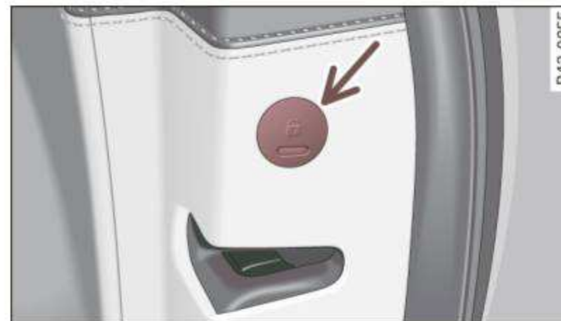
Fig. 34 Emergency lock location on the front passenger's door
