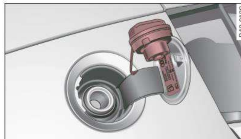
Fig. 115 Fuel cap hooked on the opened fuel filler flap
