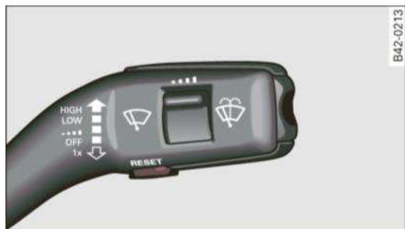
Fig. 7 Wiper lever: controls for the menu display
