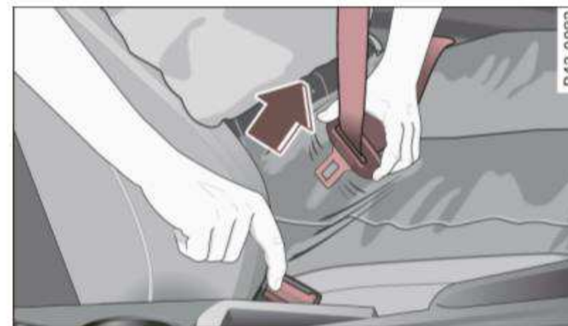
Fig. 96 Releasing the tongue from the buckle
