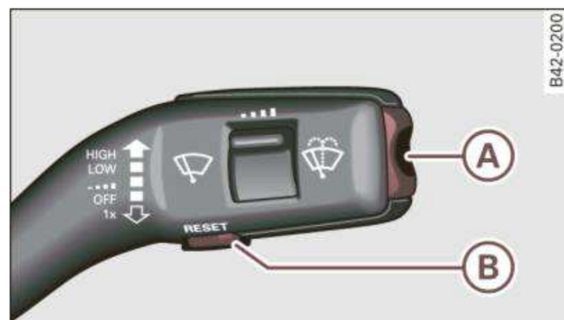
Fig. 14 Wiper lever: Controls for the menu display
