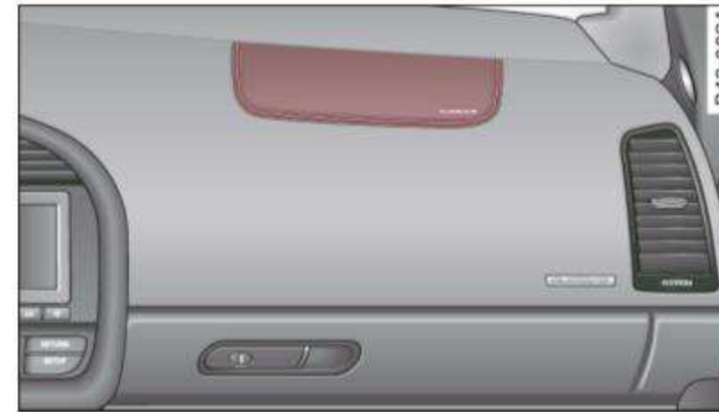
Fig. 98 Location of front passenger's airbag: in the instrument panel
