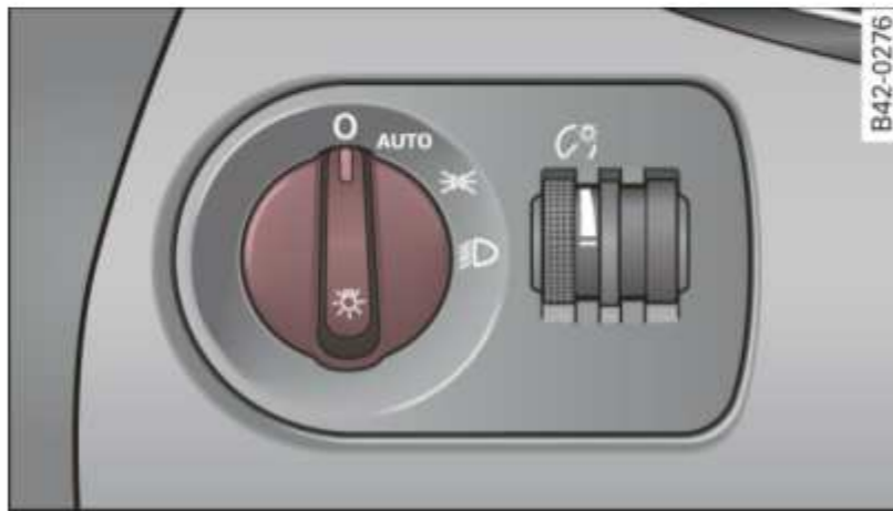
Fig. 42 Instrument panel: light switch (automatic head- and taillight control)
