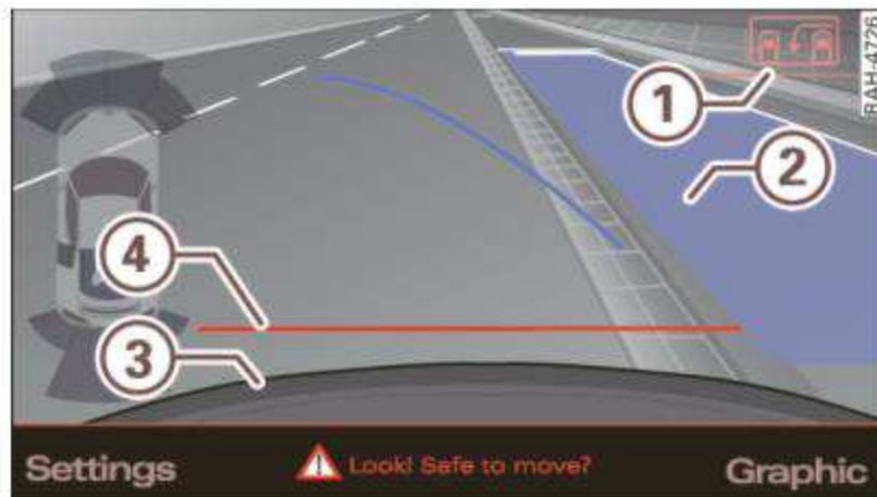
Fig. 78 Navigation system display: Blue surface aligned with parking spot
