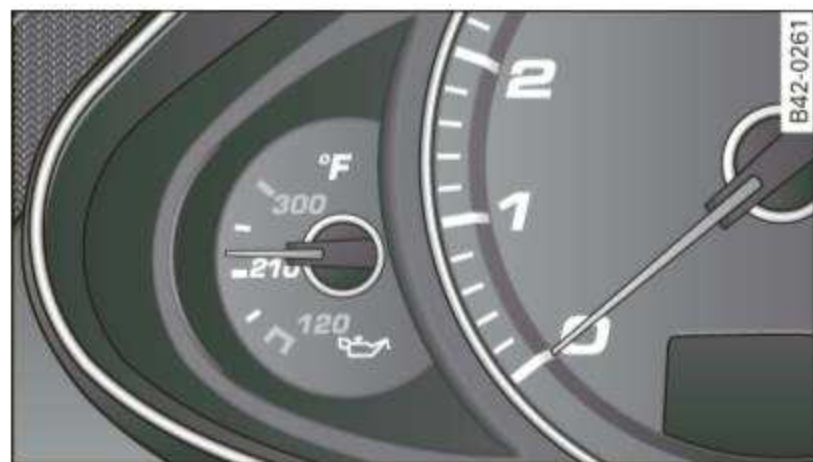
Fig. 118 Instrument cluster: Engine oil temperature display
