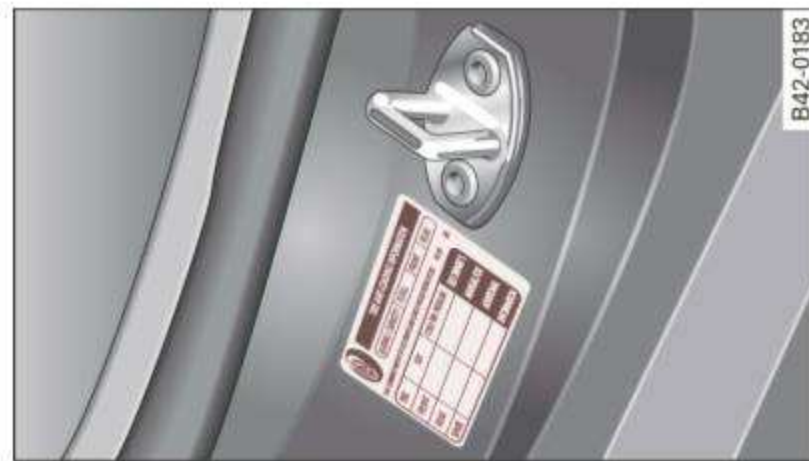
Fig. 123 Tire pressure label: located on driver's side B-pillar
