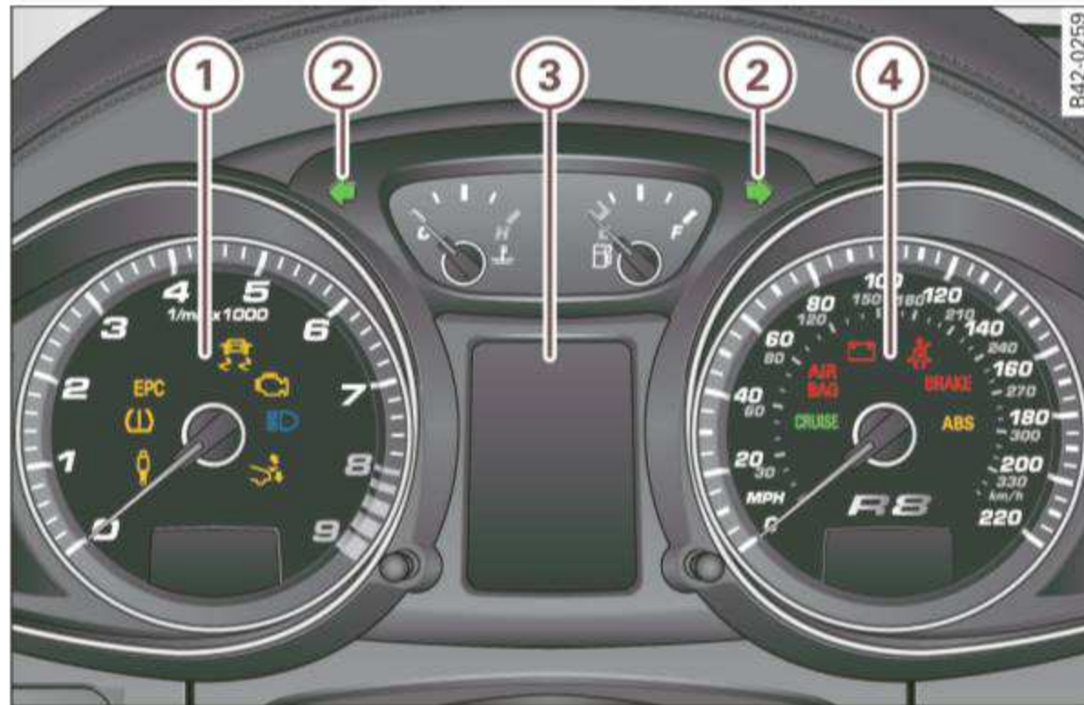
Fig. 5 Instrument cluster with warning/indicator lights
