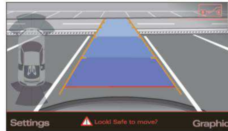
Fig. 77 Navigation system display: Aligning the vehicle
