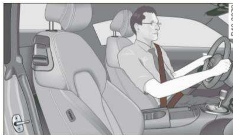
Fig. 92 Head restraint adjustment and belt position
