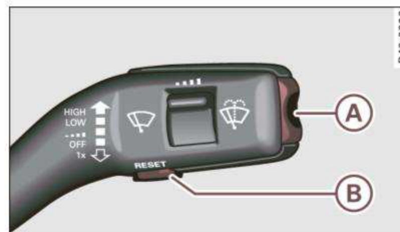
Fig. 12 Wiper lever: Controls for the menu display
