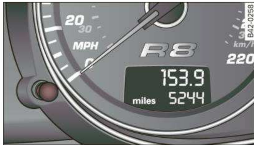
Fig. 4 Speedometer close-up: odometer display
