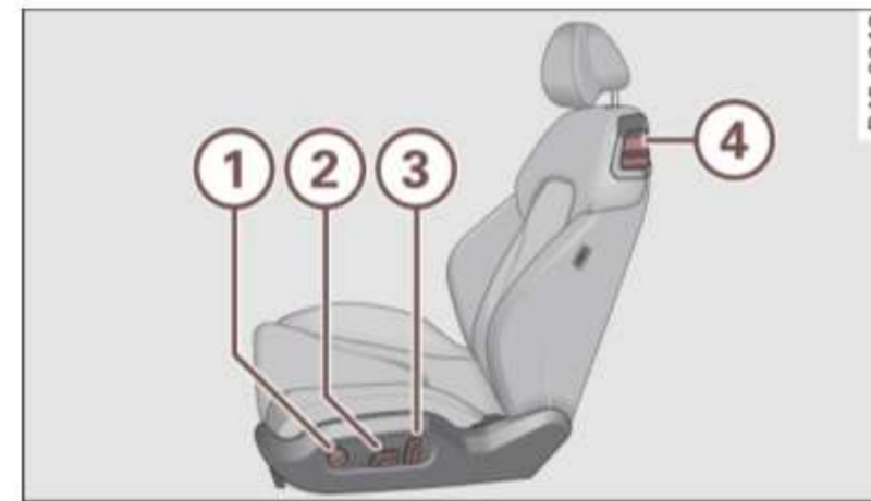
Fig. 55 Adjustment switches: locations on driver seat
