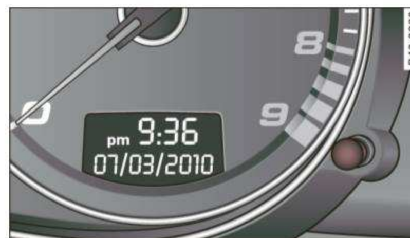
Fig. 27 Section of instrument cluster: Set/Check button
