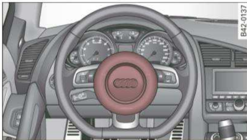
Fig. 97 Location of driver airbag: in steering wheel
