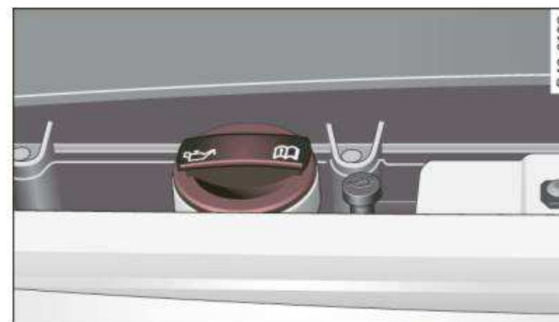
Fig. 120 Engine compartment: Oil filler cap location
