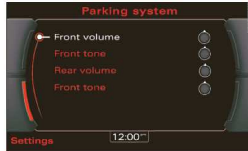
Fig. 80 Navigation system display: adjusting the parking system
