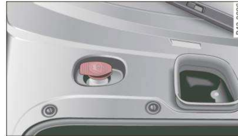
Fig. 122 Luggage compartment: Windshield washer fluid reservoir
