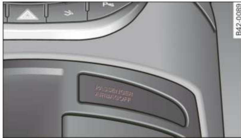
Fig. 100 Section from the instrument panel: PASSENGER AIR BAG OFF light
