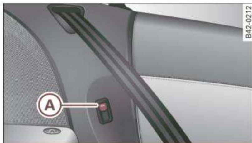
Fig. 115 Driver's side: releasing the engine compartment lid
