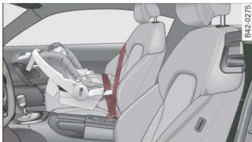
Fig. 105 Rearward-facing infant seat, properly installed on the passenger seat
