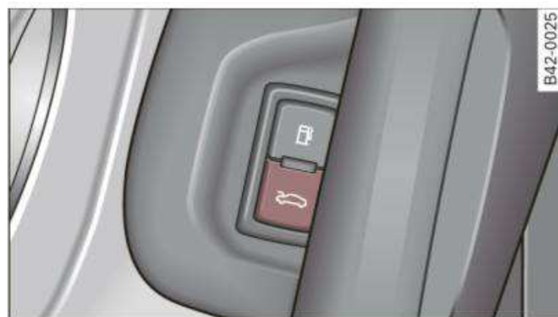
Fig. 36 Drivers door: remote front lid release
