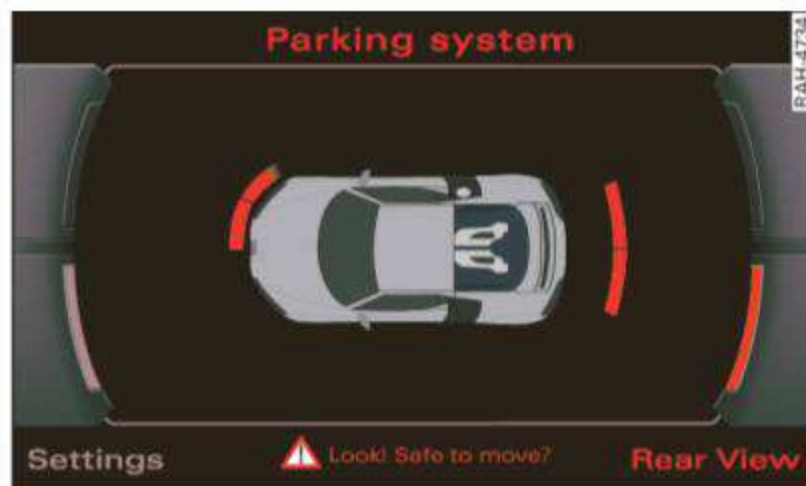
Fig. 75 Navigation system display: visual distance display
