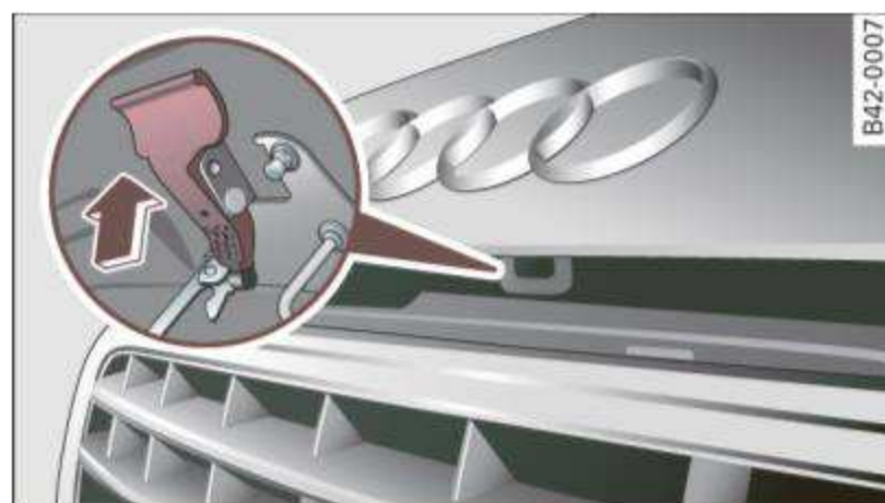
Fig. 37 Release lever under the front lid
