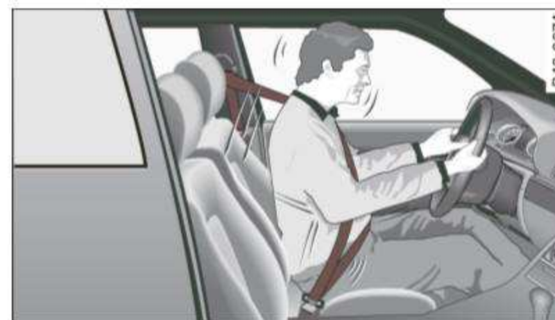
Fig. 88 Driver is properly restrained in a sudden braking maneuver.
