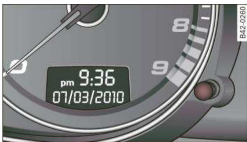
Fig. 25 Section of instrument cluster: Set/Check button
