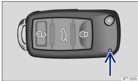
Fig. 27 Indicator light in the remote control vehicle key (version 1).
