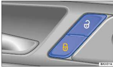
Fig. 37 In the driver and front passenger doors: power locking button.
