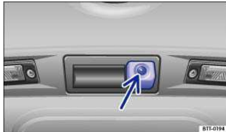
Fig. 166 In the luggage compartment lid: Location of the Rear Assist camera.
