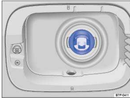
Fig. 175 With open fuel cap: Misfueling guard in the fuel filler neck.
