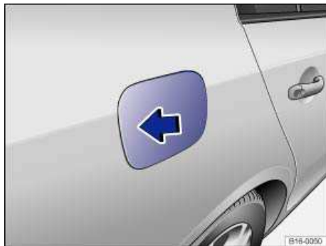
Fig. 173 Right rear side of vehicle: Opening the fuel filler flap.
