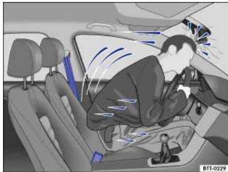
Fig. 72 The unbelted driver is thrown forward.
