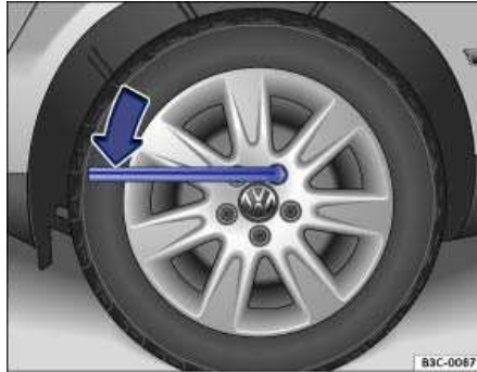
Fig. 208 Changing a wheel: Loosening wheel bolts.
