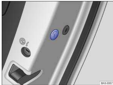
Fig. 196 On the front side of the right rear door: Emergency lock, covered by a rubber seal.
