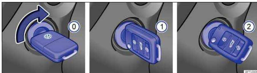
Fig. 147 In the ignition switch: Vehicle key positions.
