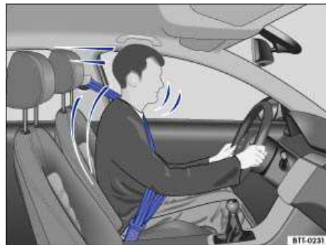
Fig. 74 Belted driver secured by the correctly worn safety belt in the event of a sudden braking maneuver.
