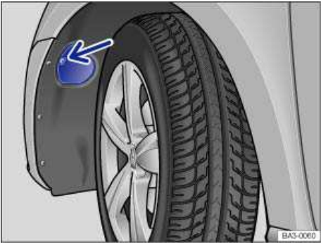
Fig. 218 In the wheel housing: Removing cover.
