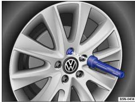
Fig. 212 Changing a wheel: remove previously loosened wheel bolts using the screwdriver handle.
