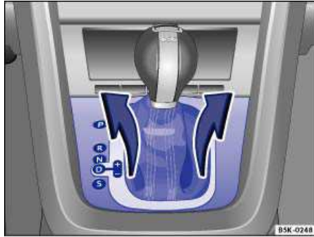
Fig. 202 Removing the selector gate cover.
