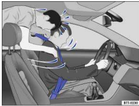
Fig. 73 Unbelted passengers in the rear seats are thrown forward on top of the belted driver.
