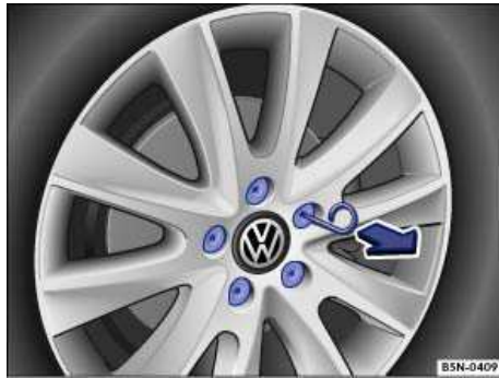
Fig. 206 Pulling cover caps off wheel bolts.
