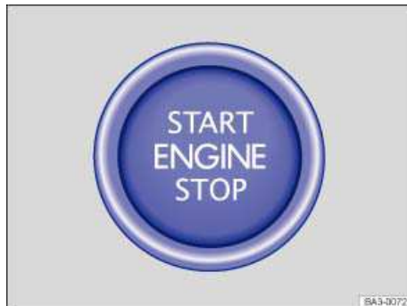
Fig. 148 In the center console: Starter button of the Keyless Access locking and starting system.
