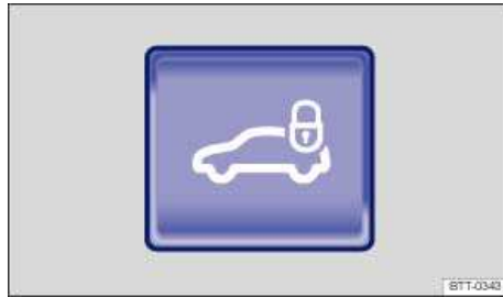
Fig. 36 In the glove compartment: Button for Valet Parking feature.
