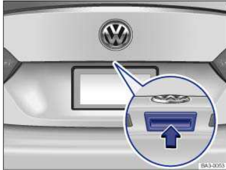
Fig. 43 Opening luggage compartment lid from the outside.
