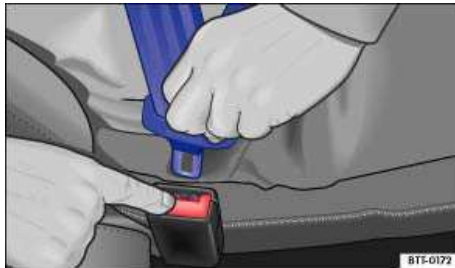
Fig. 76 Releasing the buckle tongue from the belt buckle.
