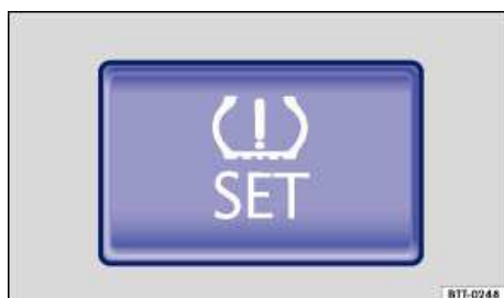
Fig. 130 In the glove compartment: SET button for the Tire Pressure Monitoring System.
