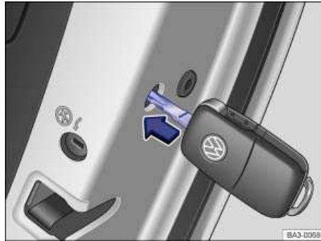
Fig. 197 On the front side of the right rear door: Manual vehicle locking with the key bit in the vehicle key.
