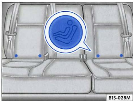
Fig.1 The illustration above shows the location of the circular seat markings for the lower anchorages for the outboard rear seating positions.
