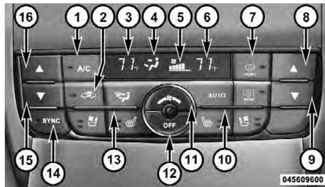
Automatic Temperature Control (ATC) Panel
