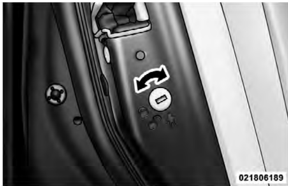
Child-Protection Door Lock Function
