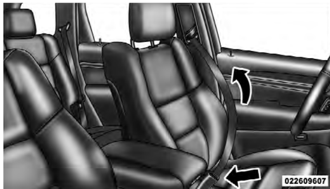
Removing Slack from Belt
