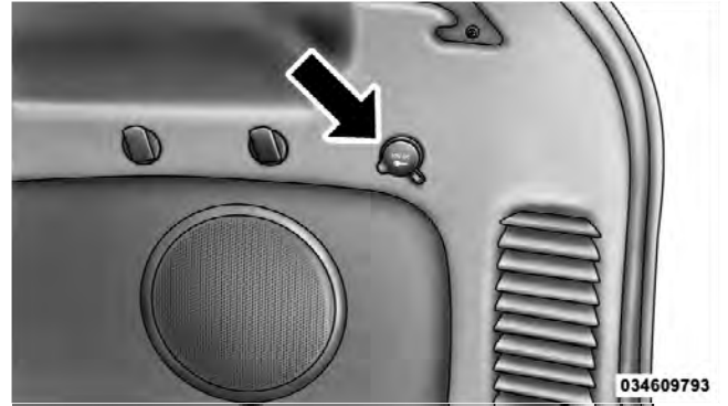
Rear Power Outlet
