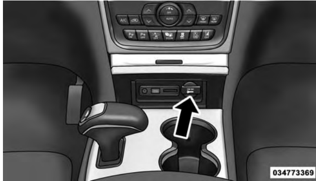
Front Power Outlet
