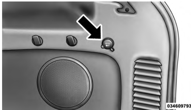
Rear Power Outlet
