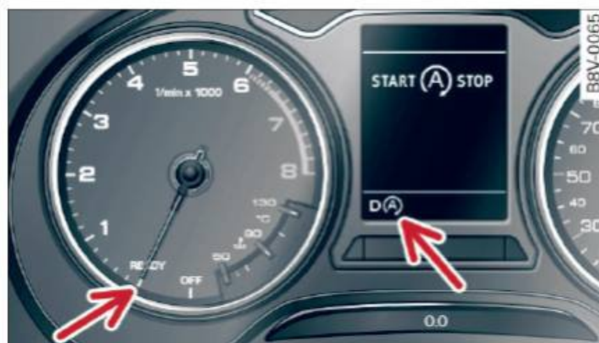
Fig. 92 Instrument cluster: engine switched off (stop phase)
