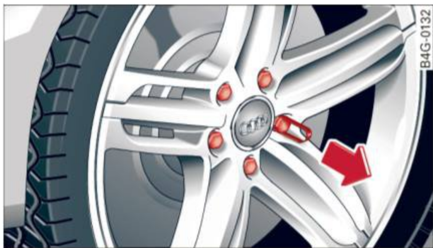
Fig. 289 Changing a wheel: removing the wheel bolt caps
