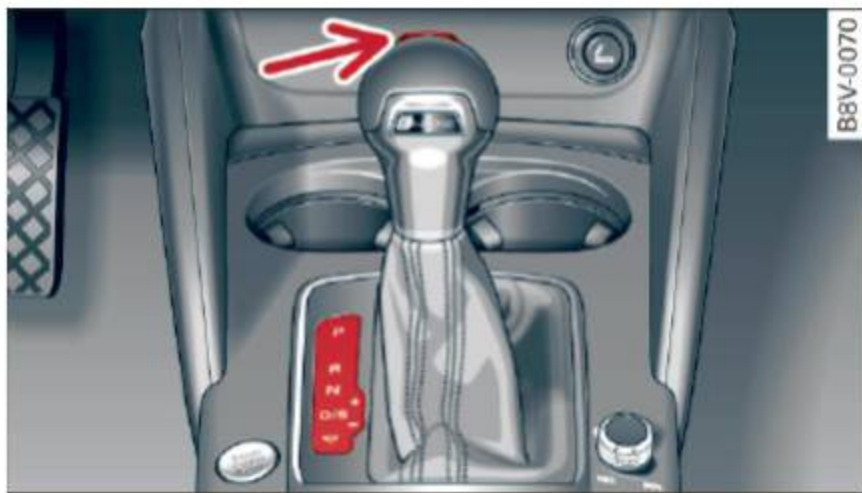
Fig. 97 Section of the center console: selector lever with interlock button
