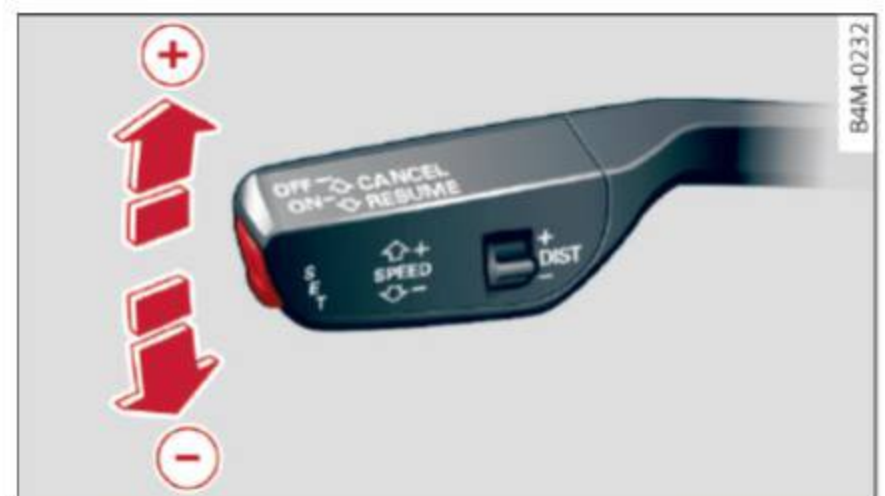
Fig. 134 Operating lever: changing the speed
