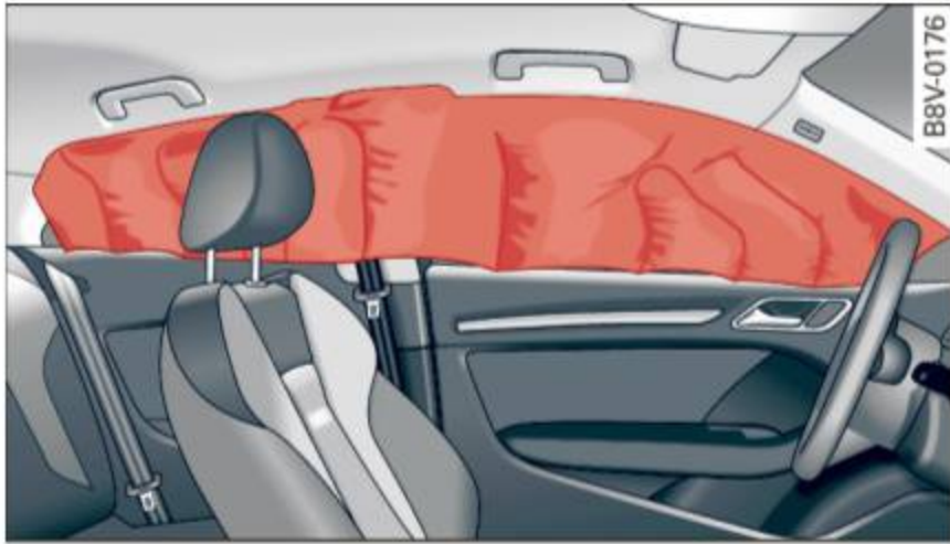
Fig. 251 Illustration of principle: Inflated side curtain airbags on the left side (example)
