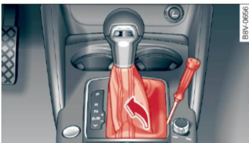
Fig. 100 Selector lever: removing the shifter boot
