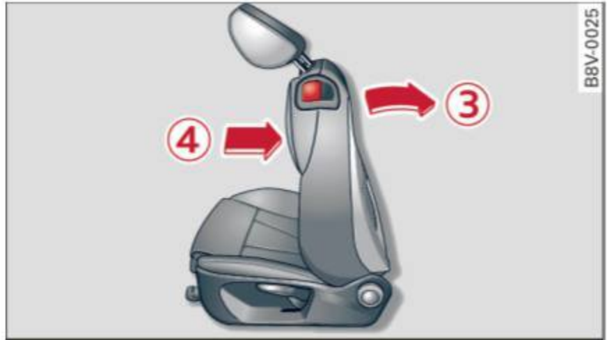
Fig. 68 Easy seat entry operation (example), seat returning to the original position with seat memory
