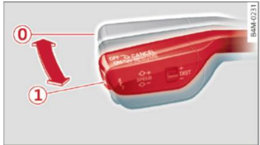
Fig. 132 Operating lever: switching on and off
