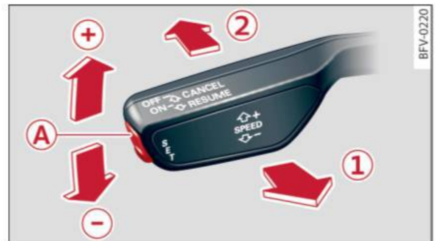
Fig. 127 Operating lever: cruise control system
