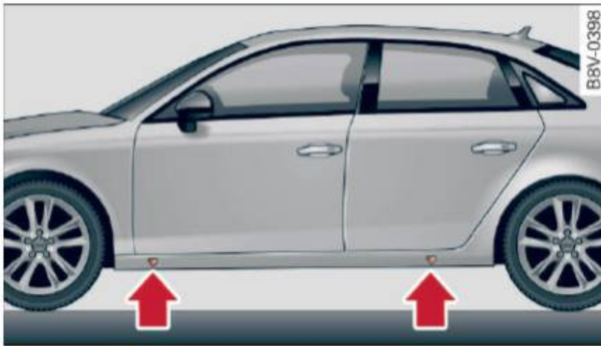
Fig. 291 Sill panels: markings (example)
