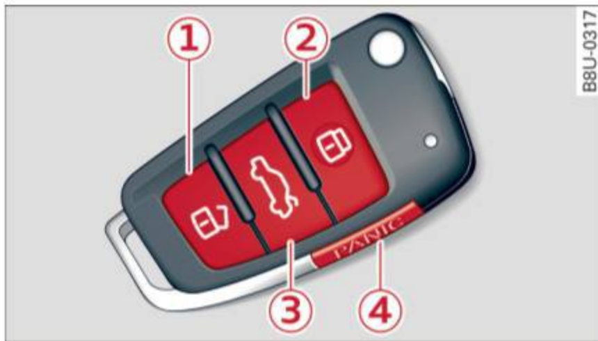
Fig. 22 Remote control key or convenience key: button programming
