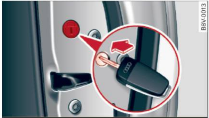
Fig. 26 Front side of the door: emergency release
