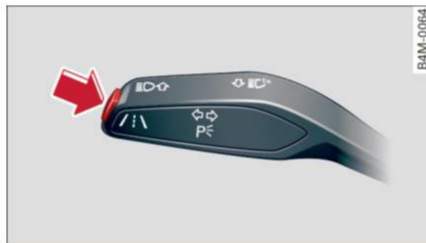
Fig. 141 Turn signal lever: button for active lane assist
