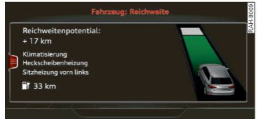
Fig. 105 Infotainment system: e-tron range monitor
