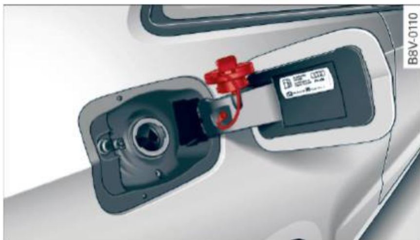
Fig. 266 Fuel filler door with attached fuel cap
