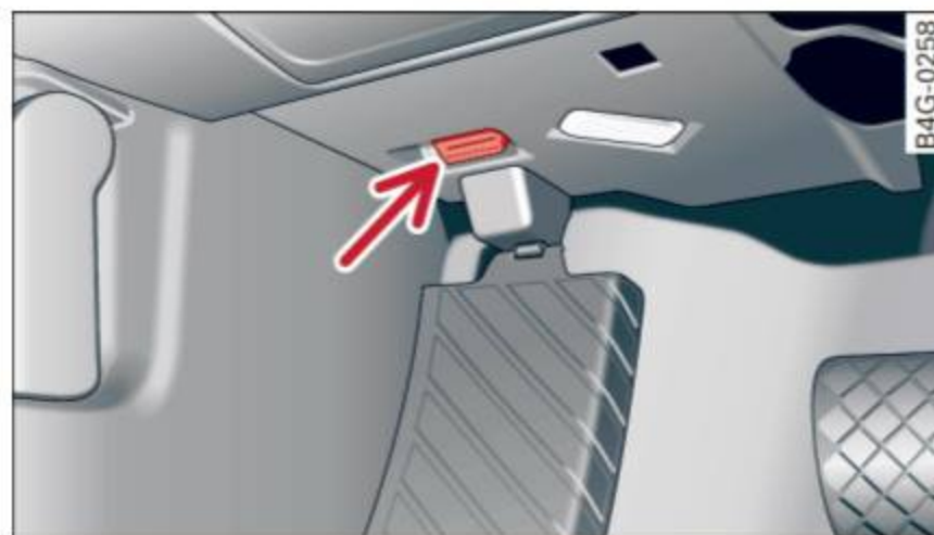
Fig. 19 Location of Data Link Connector (DLC)
