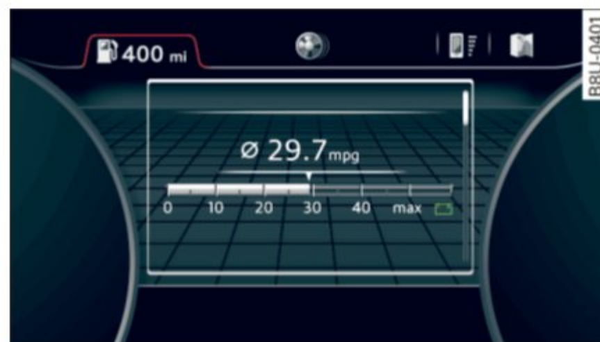
Fig. 14 Instrument cluster: fuel consumption display
