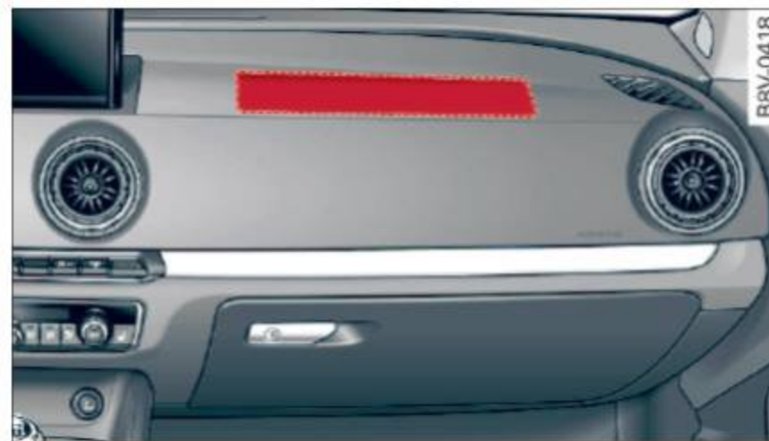
Fig. 242 Location of front passenger's airbag: in the instrument panel
