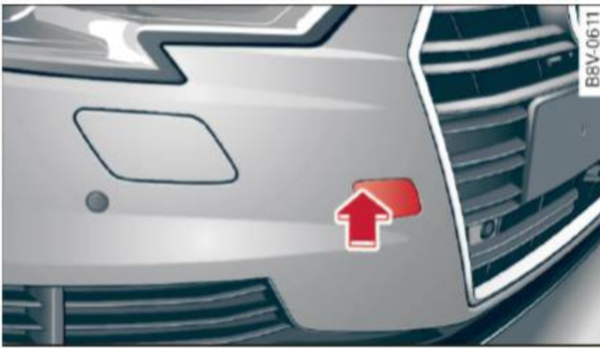
Fig. 305 Right front bumper: removing the cover
