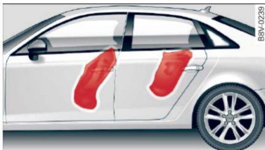
Fig. 248 Side impact protection: inflated side airbags (example)
