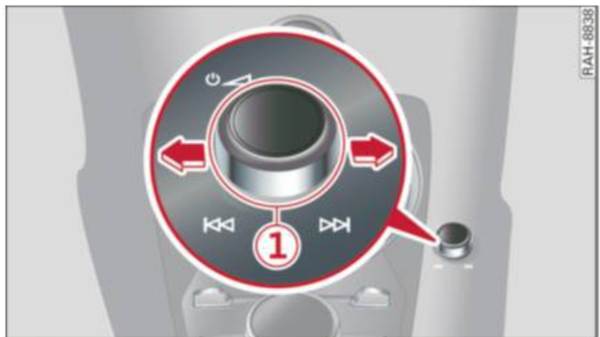
Fig. 161 MMI On/Off knob with joystick function
