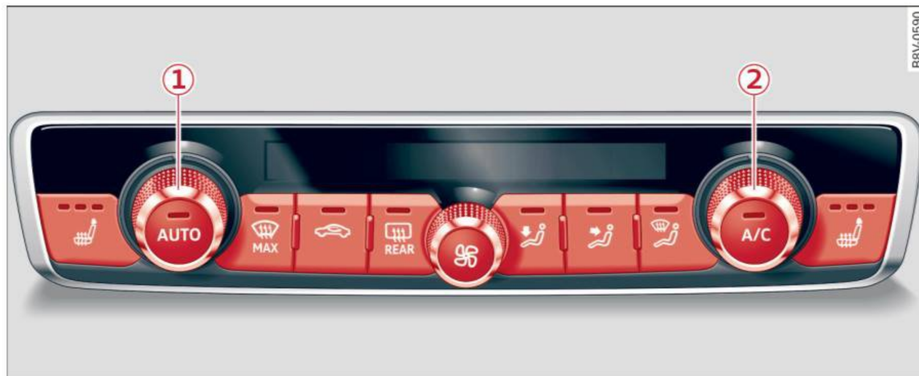
Fig. 86 Automatic climate control system: controls (example)
