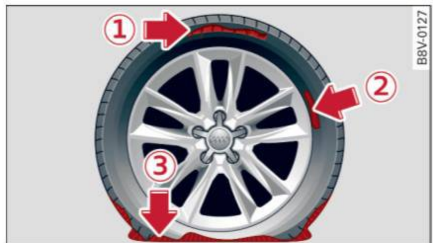
Fig. 285 Tire: tire damage that cannot be repaired
