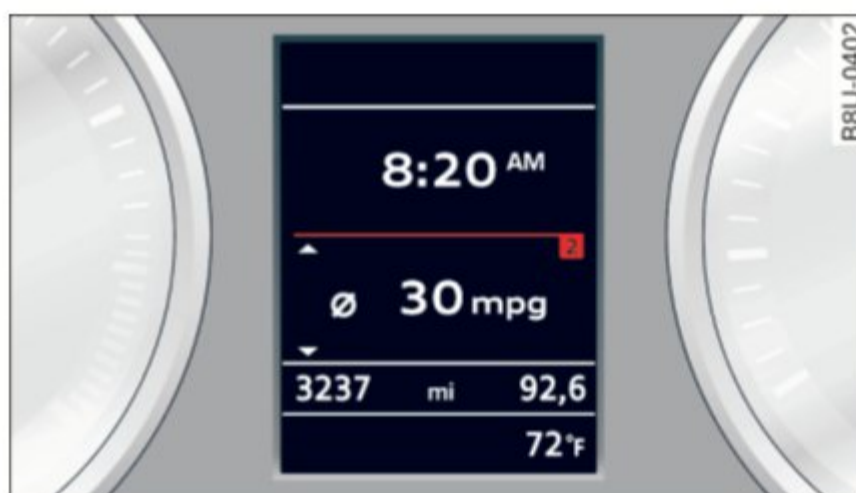
Fig. 15 Instrument cluster: fuel consumption display
