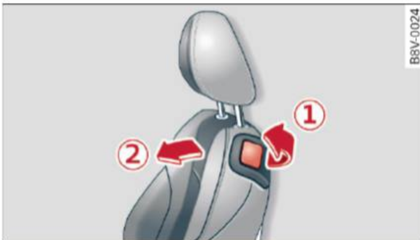
Fig. 67 Driver's seat: easy seat entry controls (example)
