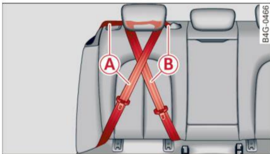
Fig. 252 Schematic overview: keep unused safety belts away from children in child safety seats. A - outer rear safety belt, B - center rear safety belt*
