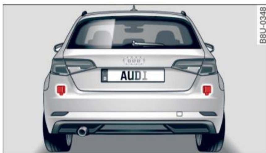
Fig. 147 Rear of the vehicle: position of the sensors
