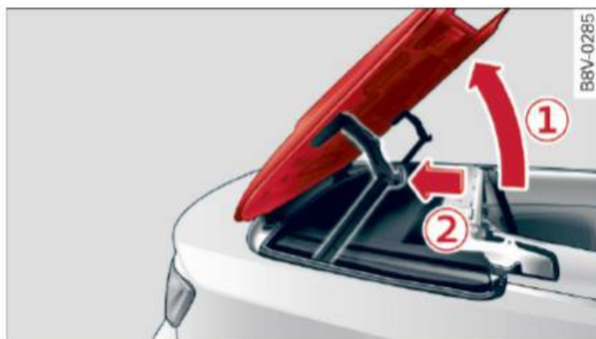
Fig. 43 Lifting the power top storage compartment cover out and setting up the supports
