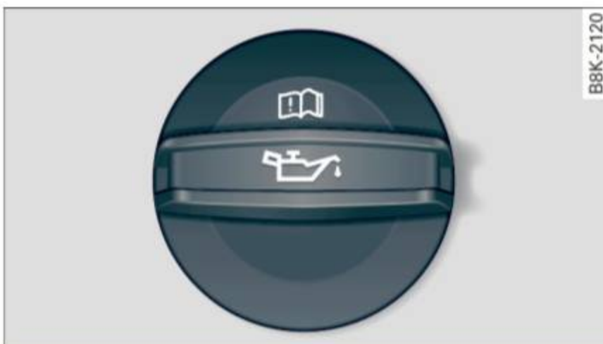
Fig. 273 Engine compartment: engine oil filling opening cover (example)
