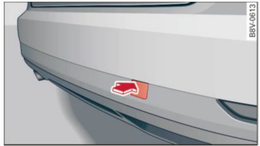
Fig. 307 Right rear towing loop: removing the cover
