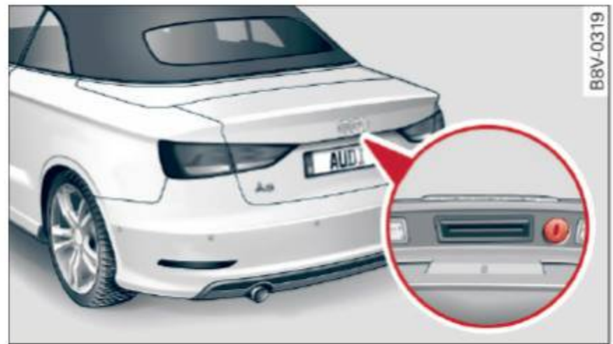
Fig. 30 Rear lid: emergency release lock cylinder
