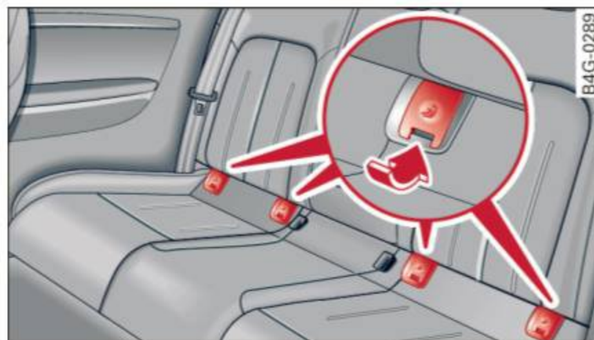
Fig. 258 Lower anchorages, covers marked
