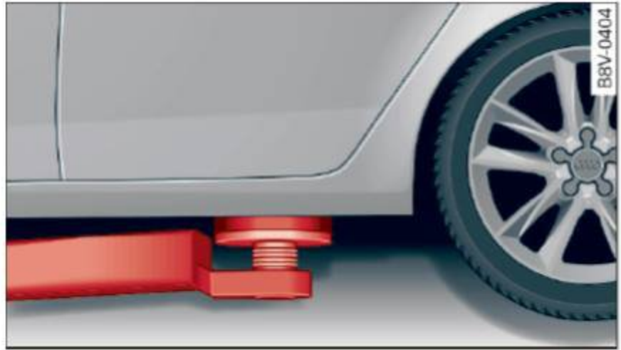
Fig. 311 Rear lifting point (example)
