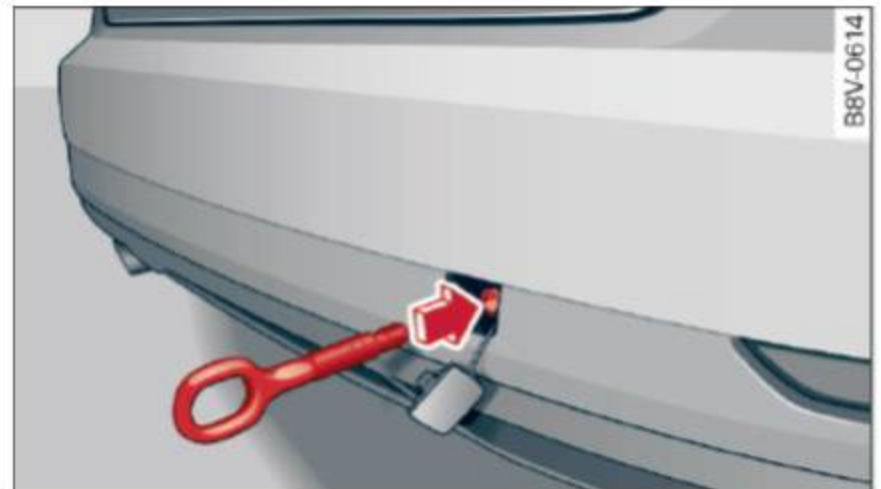
Fig. 308 Right rear towing loop: towing loop installed
