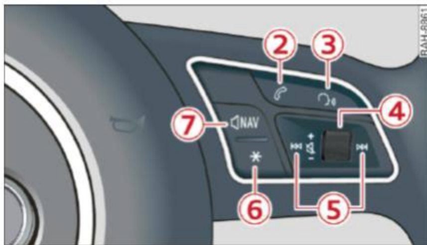
Fig. 13 Right side of the multifunction steering wheel
