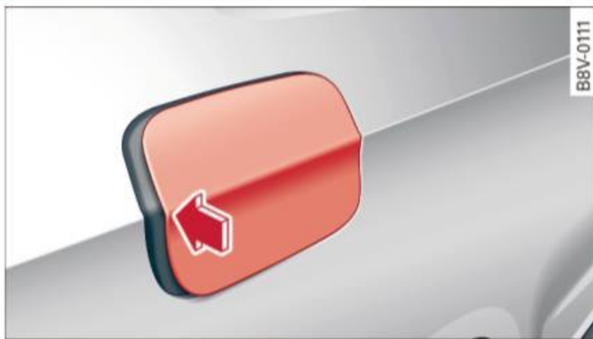
Fig. 265 -Applies to: vehicles without plug-in hybrid drive- right rear side of the vehicle: opening the fuel filler door
