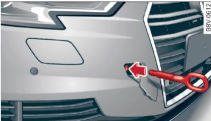
Fig. 306 Right front bumper: towing loop installed
