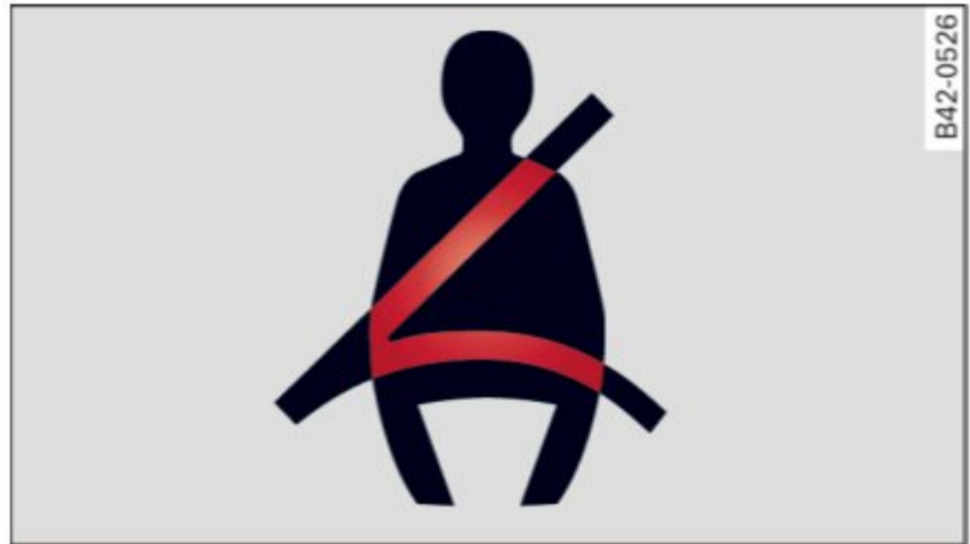
Fig. 229 Safety belt warning light in the instrument cluster - enlarged
