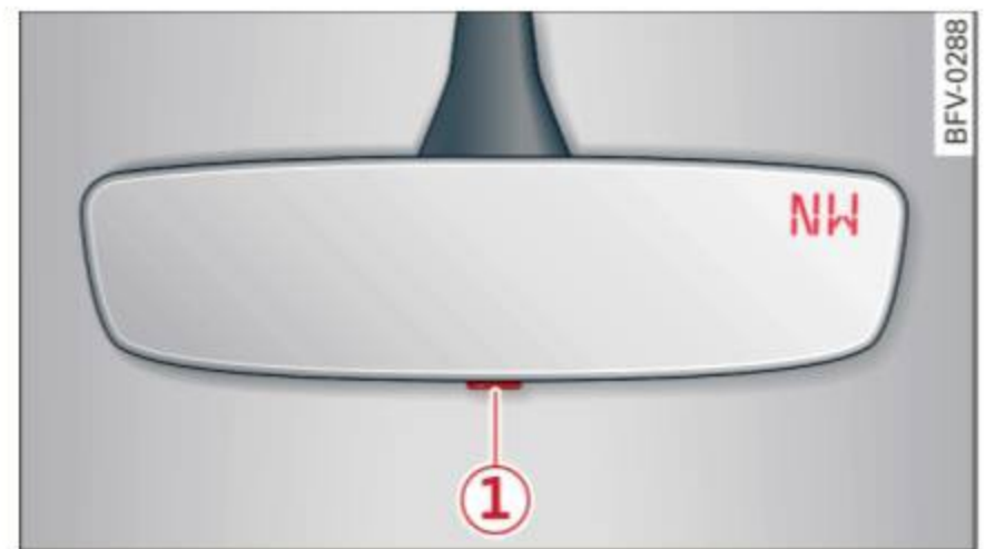
Fig. 63 Rearview mirror: digital compass is switched on
