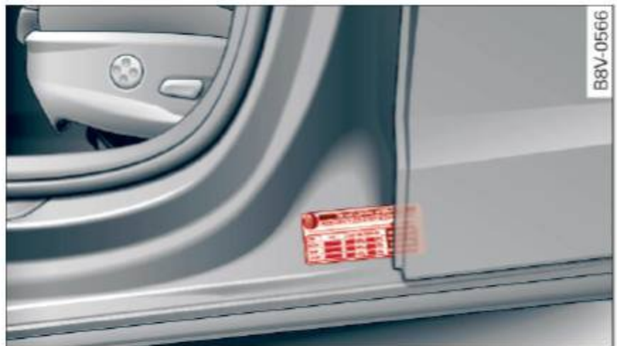
Fig. 280 Driver's side B-pillar (example): tire pressure label
