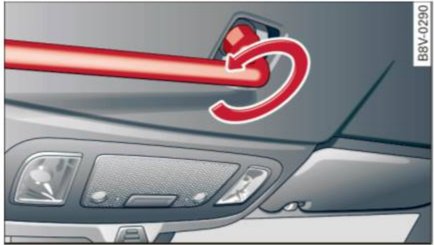
Fig. 49 Inside of the power top: locking the power top
