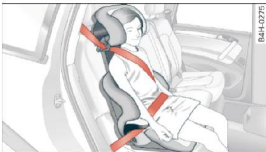
Fig. 256 Rear seat: child properly restrained in a booster seat
