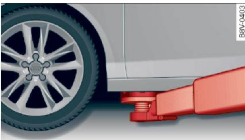
Fig. 310 Front lifting point (example)
