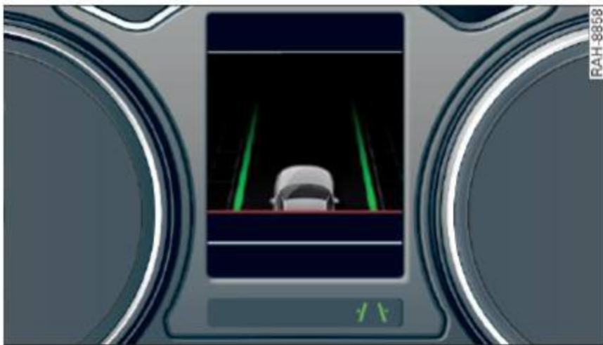
Fig. 143 Instrument cluster: active lane assist is switched on and ready to provide warnings
