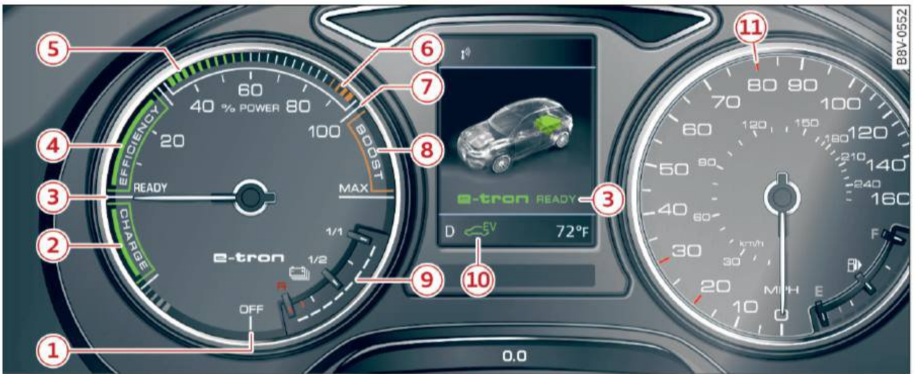
Fig. 103 -Applies to: vehicles with analog instrument cluster-Power meter overview (diagram)
