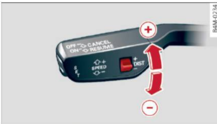
Fig. 137 Operating lever: setting the distance
