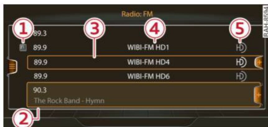
Fig. 201 FM station list (HD Radio technology FM)
