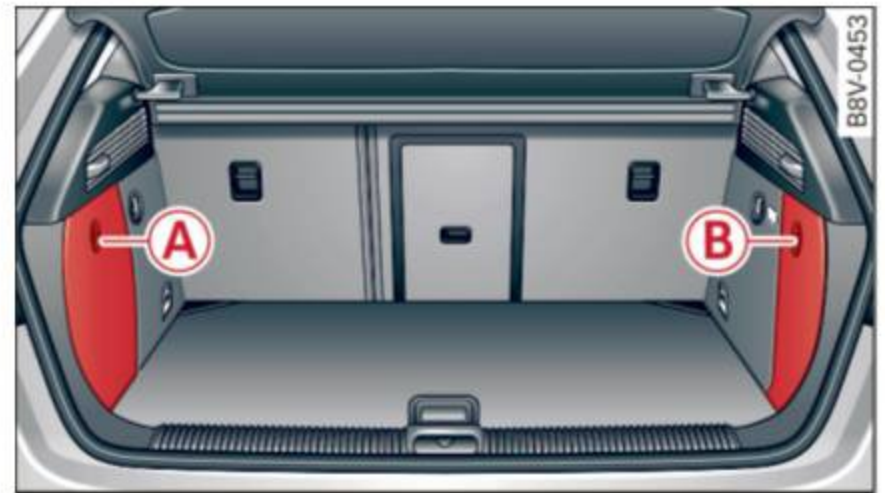
Fig. 109 Luggage compartment: vehicle tool kit and tire mobility kit
