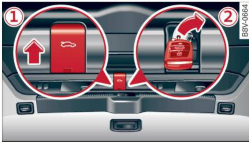
Fig. 28 Section of the luggage compartment: access to the emergency release
