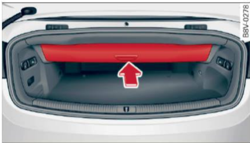
Fig. 37 Luggage compartment: power top storage compartment lowered
