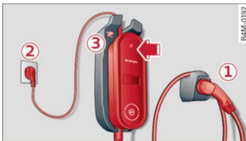
Fig. 119 Charging clip: charging system connected
