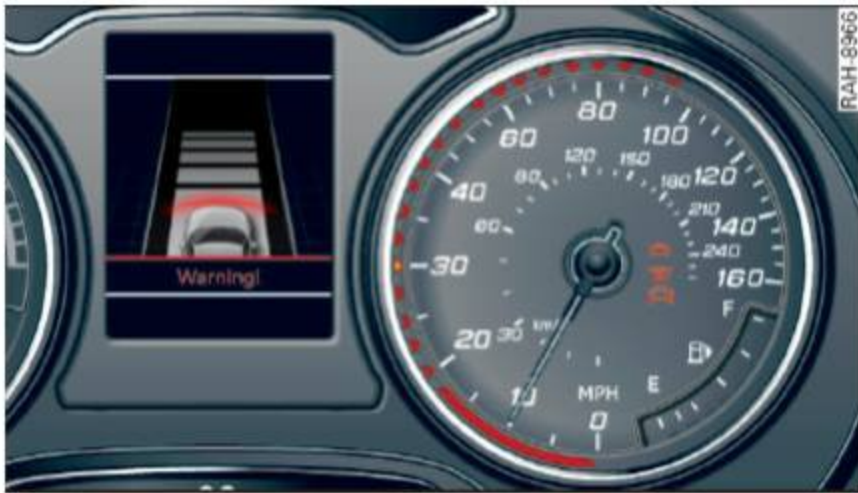
Fig. 135 Instrument cluster: safe start monitor
