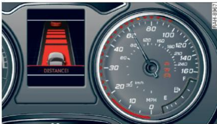
Fig. 138 Instrument cluster: request for driver intervention
