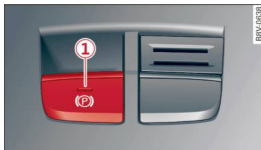
Fig. 94 Center console: parking brake
