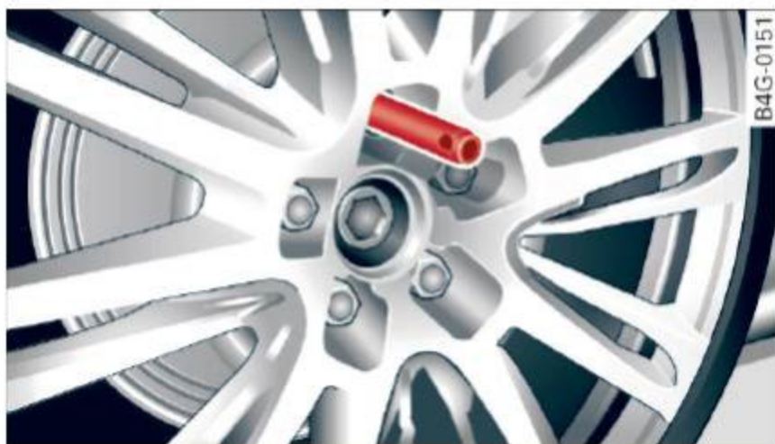
Fig. 294 Changing a wheel: alignment pin inside the top hole
