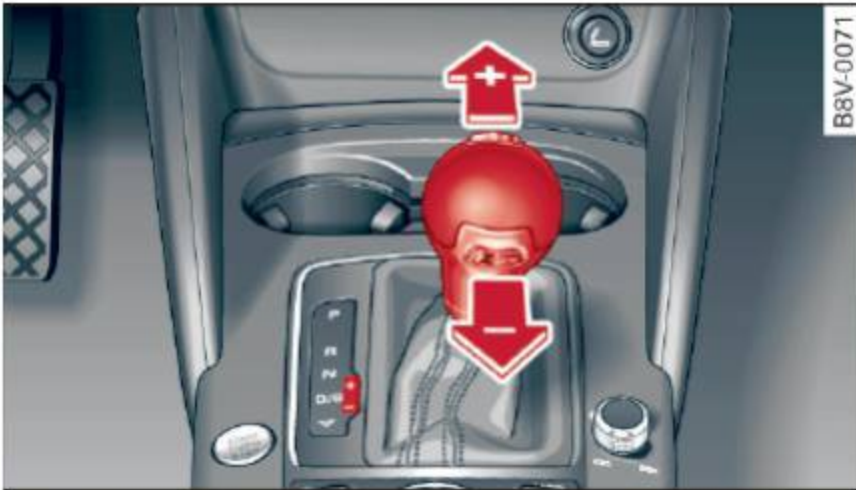
Fig. 98 Center console: shifting manually with the selector lever
