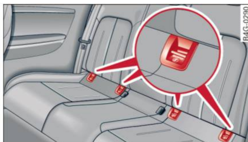
Fig. 259 Rear seats: lower anchorage bracket locations
