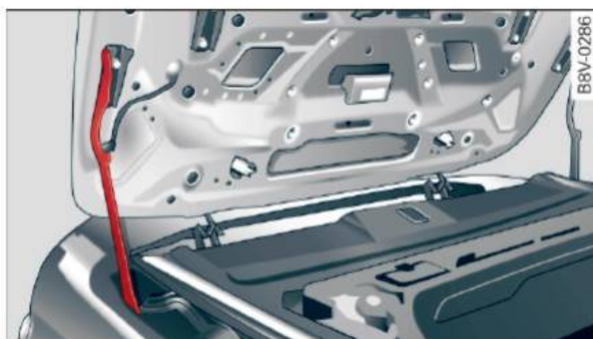
Fig. 44 Power top storage compartment cover: supports set up
