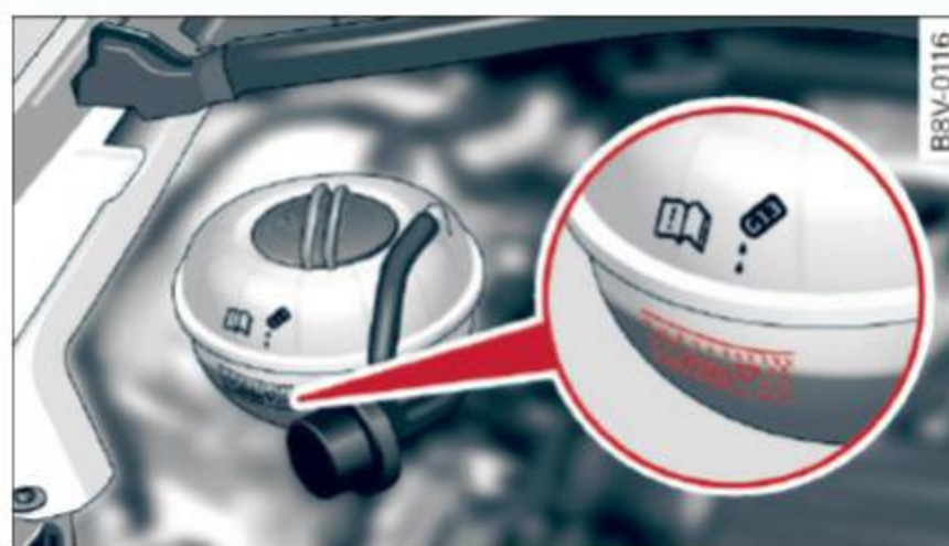
Fig. 274 Engine compartment: markings on the coolant expansion tank
