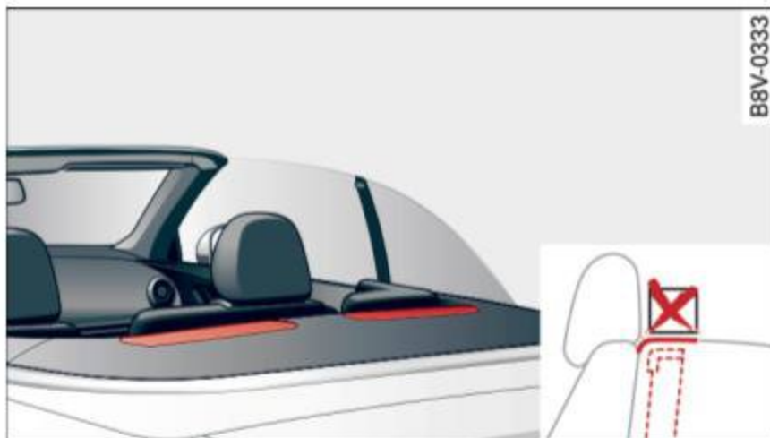
Fig. 225 Rear seats: rollbar deployment range
