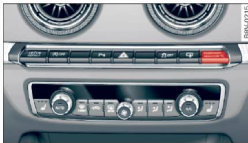
Fig. 244 Center console: passenger airbag off warning light
