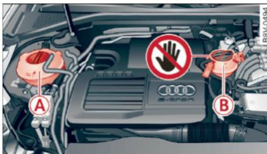
Fig. 111 Engine compartment: coolant expansion tank
