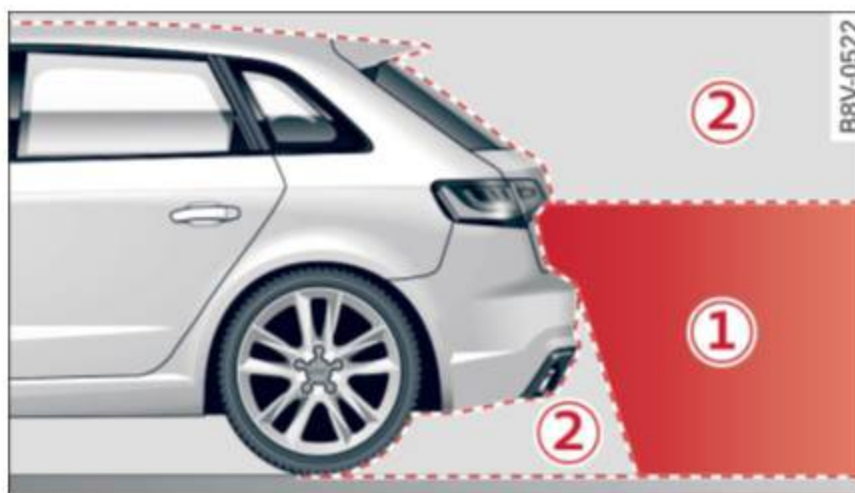
Fig. 155 Area covered ① and area not covered ② by the rearview camera (example)
