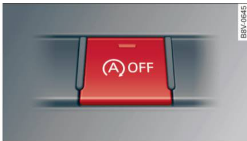
Fig. 93 Center console: Start/Stop system button
