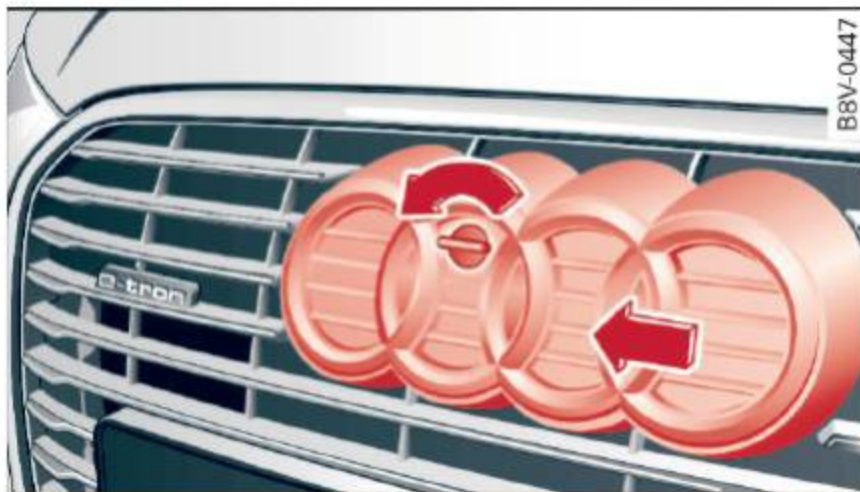
Fig. 123 Radiator grille: opening the charging unit cover
