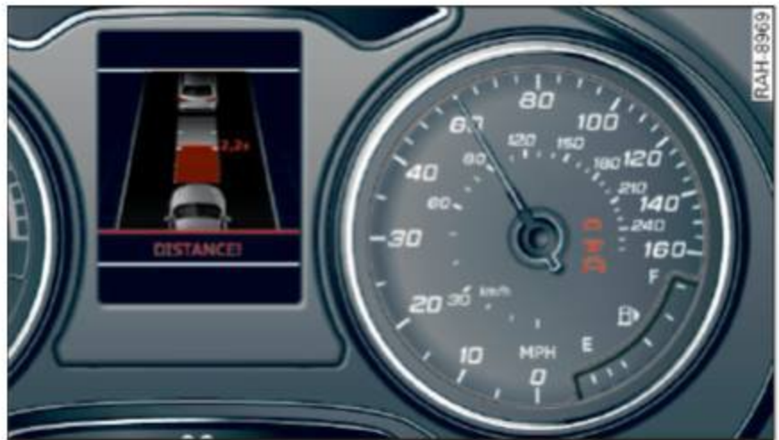
Fig. 139 Instrument cluster: distance indicator/warning
