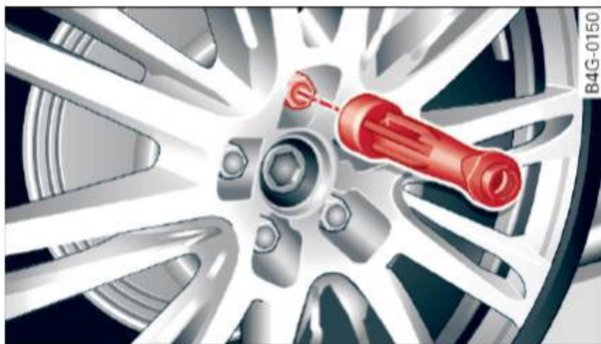
Fig. 293 Changing a wheel: using the screwdriver handle (with the blade removed) to turn the bolts
