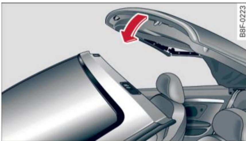
Fig. 48 Windshield: closing the power top
