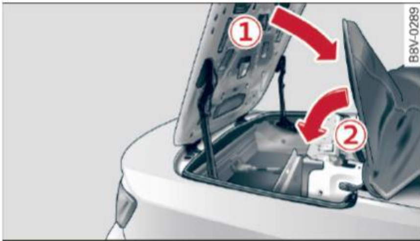
Fig. 47 Rear of vehicle: closing the power top (2)
