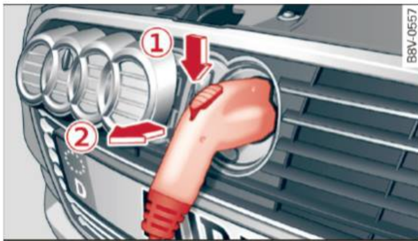
Fig. 125 Radiator grille: unlocking and removing the vehicle charging connector
