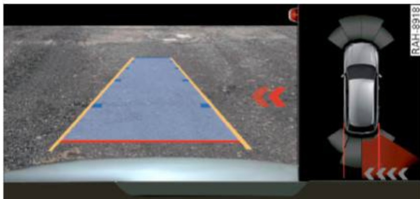
Fig. 149 Infotainment system: rear cross-traffic assist display
