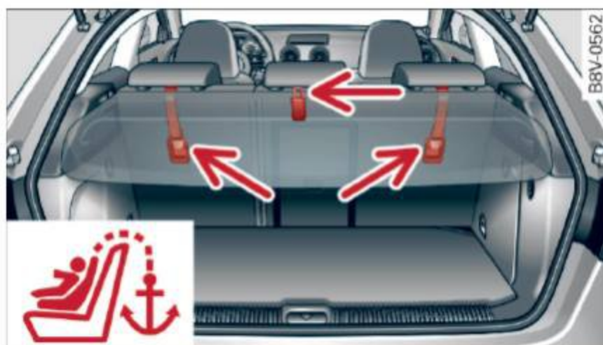
Fig. 262 Tether anchors: recess flaps behind the rear seat-backs
