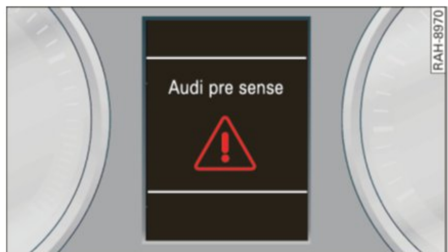
Fig. 140 Instrument cluster: approach warning
