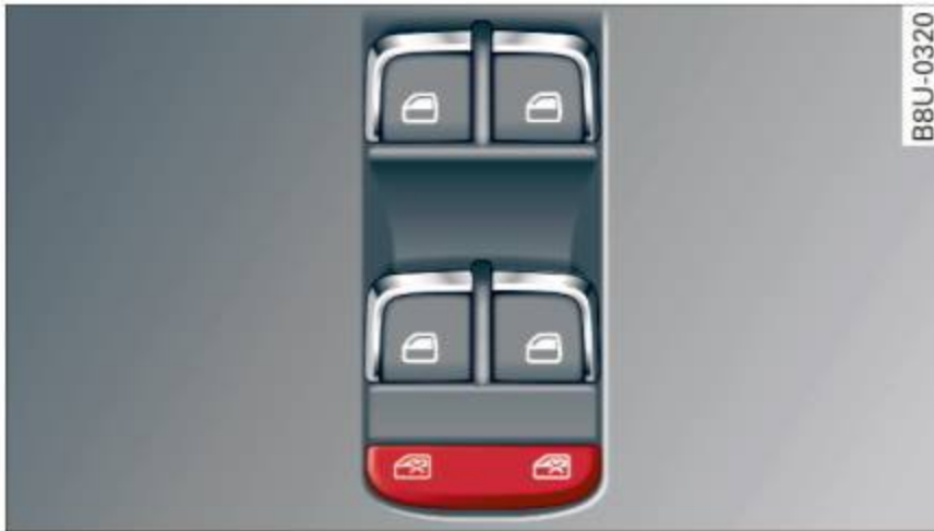
Fig. 31 Section of driver's door: controls
