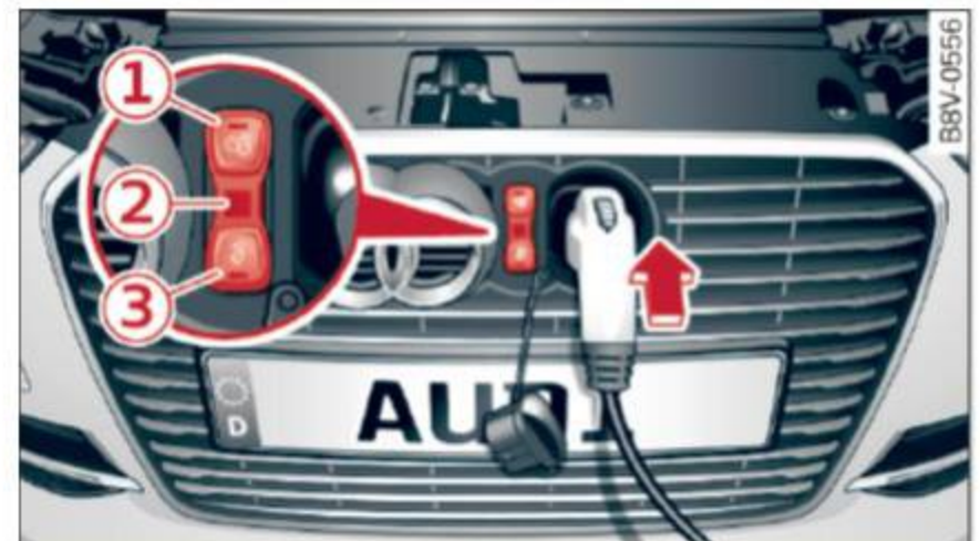
Fig. 122 Radiator grille: vehicle charging port and button module
