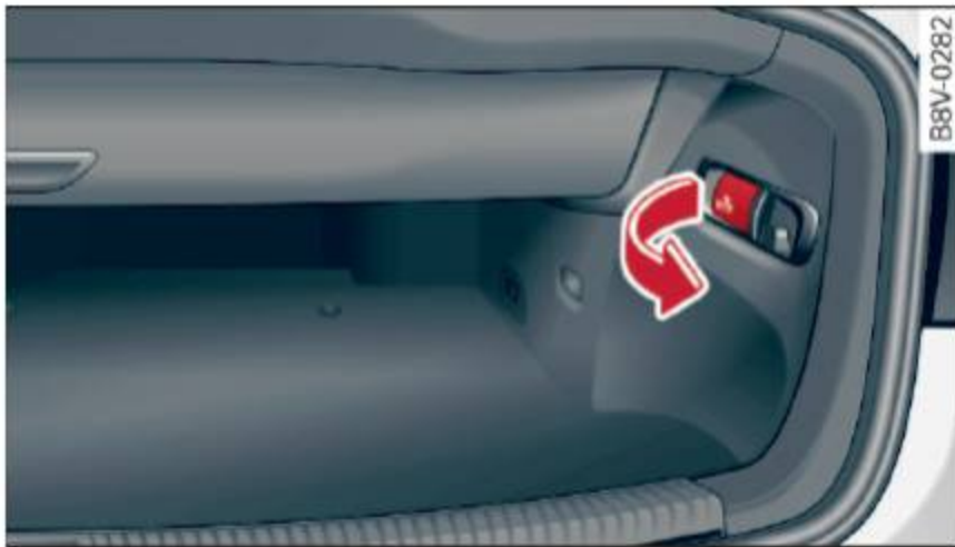
Fig. 83 Luggage compartment: release lever in the luggage compartment (example on the right side)
