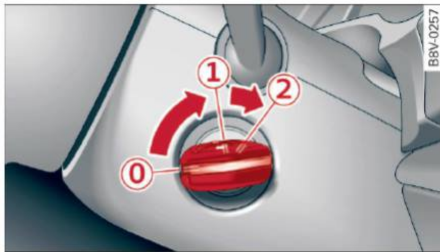
Fig. 89 Ignition lock: position of the ignition key
