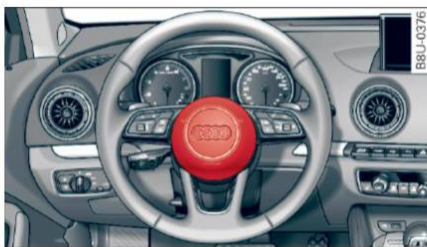
Fig. 241 Location of driver airbag: in steering wheel
