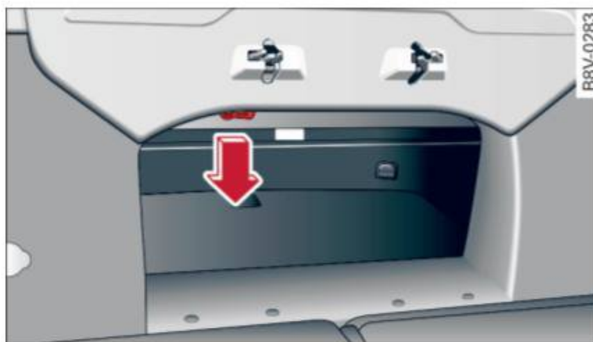
Fig. 41 Rear seats folded forward: release loop for the power top storage compartment cover
