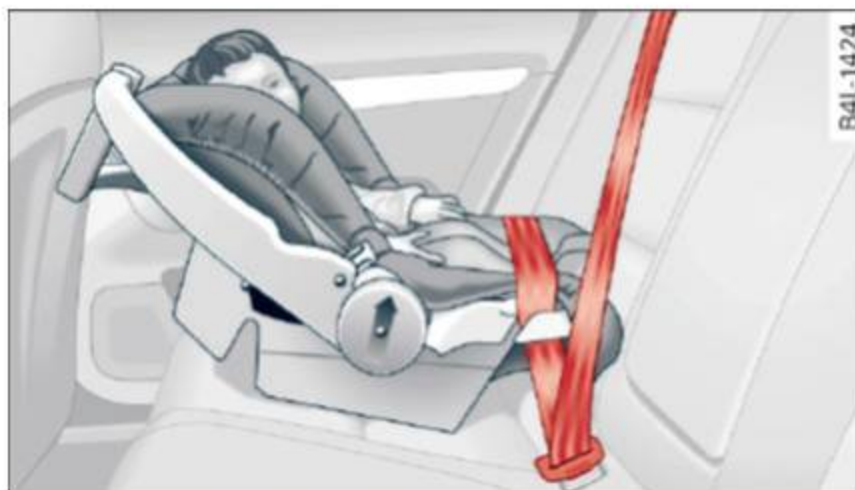
Fig. 253 Schematic overview: rearward-facing infant seat, properly installed on the rear seat
