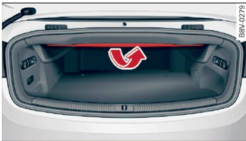
Fig. 38 Luggage compartment: power top storage compartment raised
