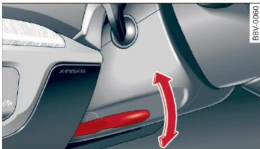
Fig. 88 Steering column: steering column adjustment lever
