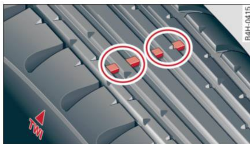
Fig. 279 Tire profile: treadwear indicator
