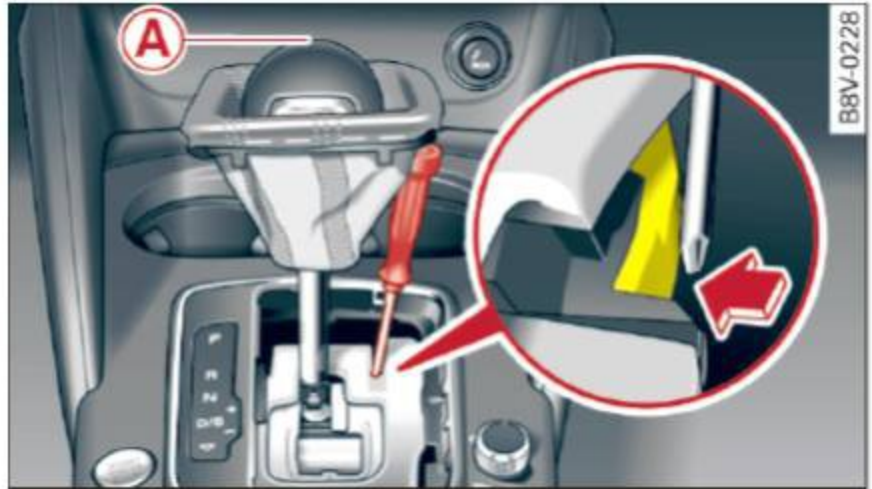
Fig. 101 Selector lever: using the emergency release to move out of the Park position
