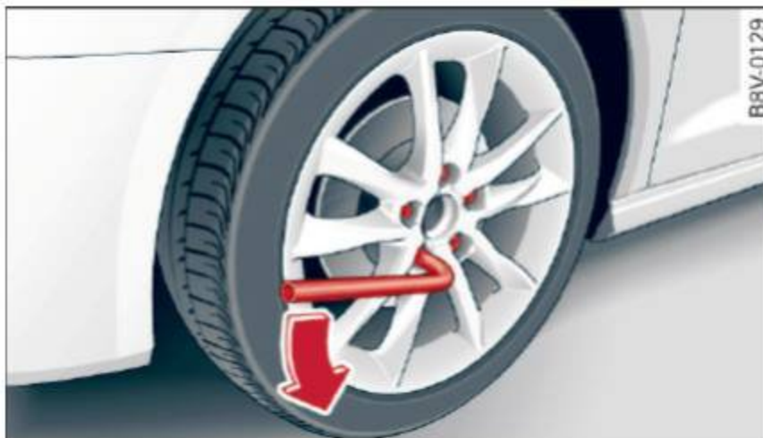
Fig. 290 Changing a wheel: loosening the wheel bolts
