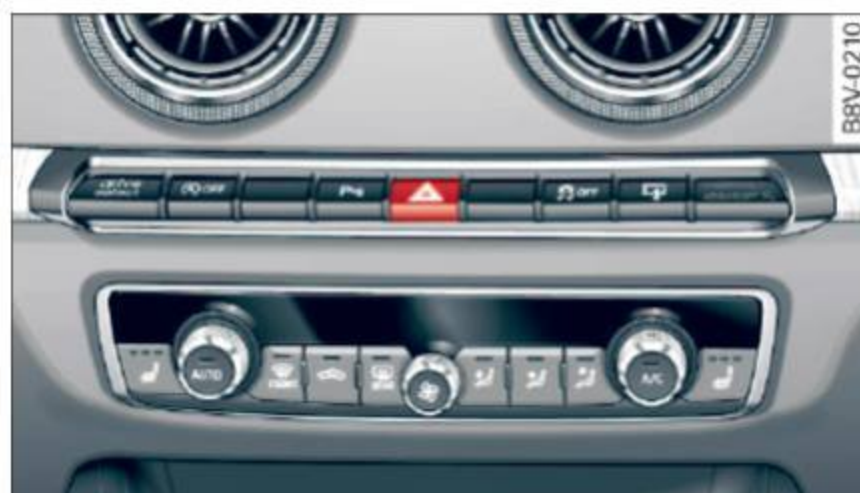
Fig. 52 Instrument panel: emergency flasher button
