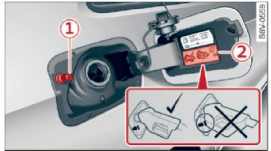
Fig. 113 Fueling procedure: insert the fuel pump nozzle correctly
