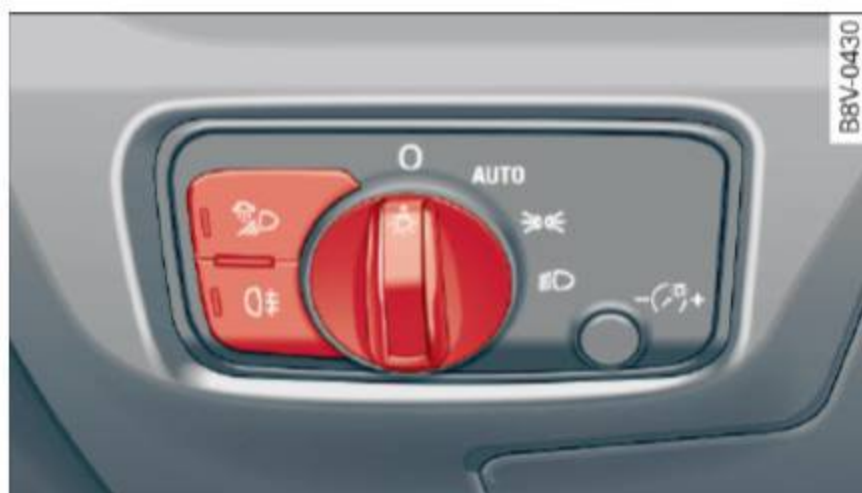
Fig. 50 Instrument panel: light switch with buttons
