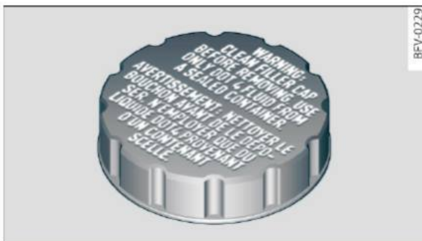
Fig. 275 Engine compartment: cap on brake fluid reservoir
