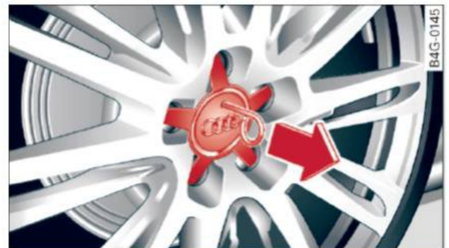
Fig. 288 Changing a wheel: Removing the wheel cover
