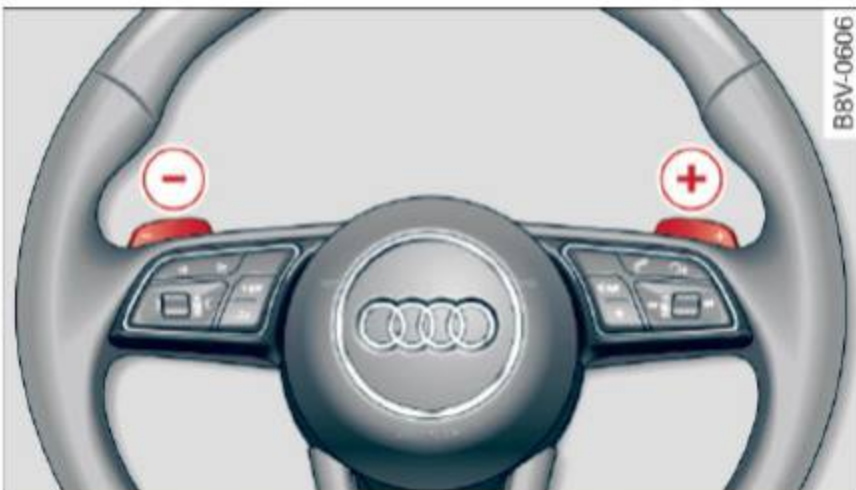
Fig. 99 Steering wheel: shifting manually with the shift paddles*
