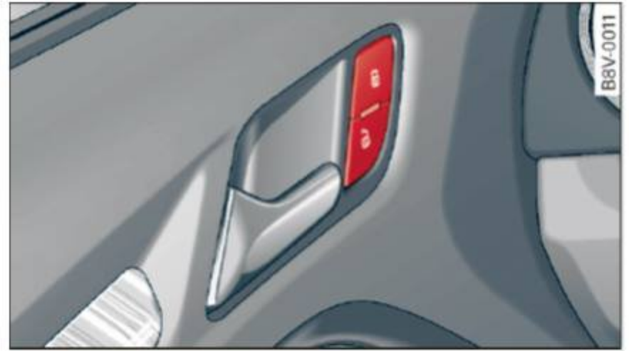
Fig. 24 Driver's door: central locking switch
