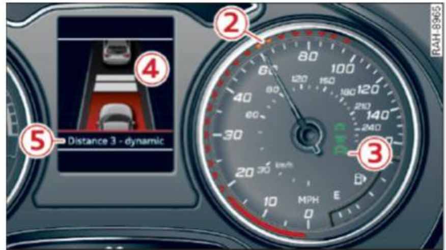
Fig. 133 Instrument cluster: adaptive cruise control
