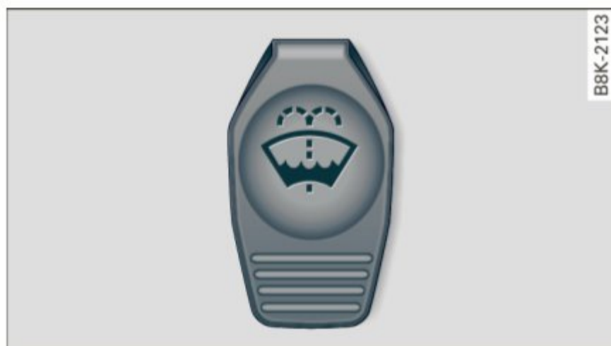
Fig. 277 Engine compartment: washer fluid reservoir cap
