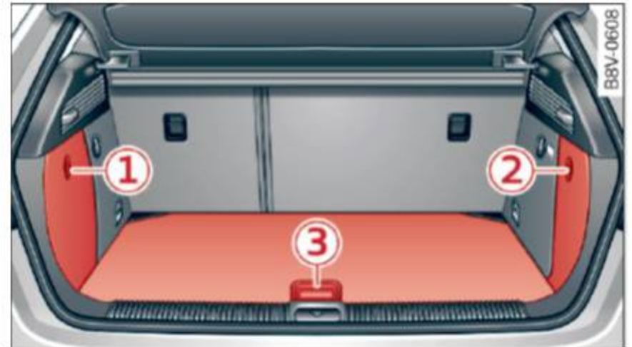
Fig. 283 Luggage compartment (example): vehicle tool kit housing, tire mobility kit and vehicle jack*
