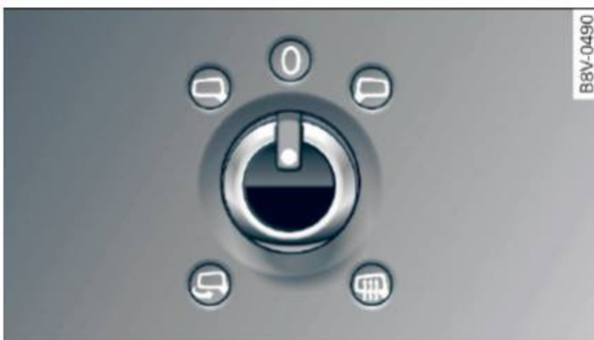
Fig. 57 Driver's door: knob for the exterior mirrors (example)
