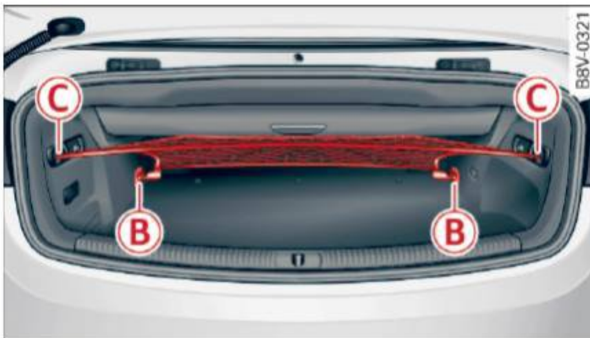
Fig. 80 Luggage compartment: cargo bag hung in place (example)
